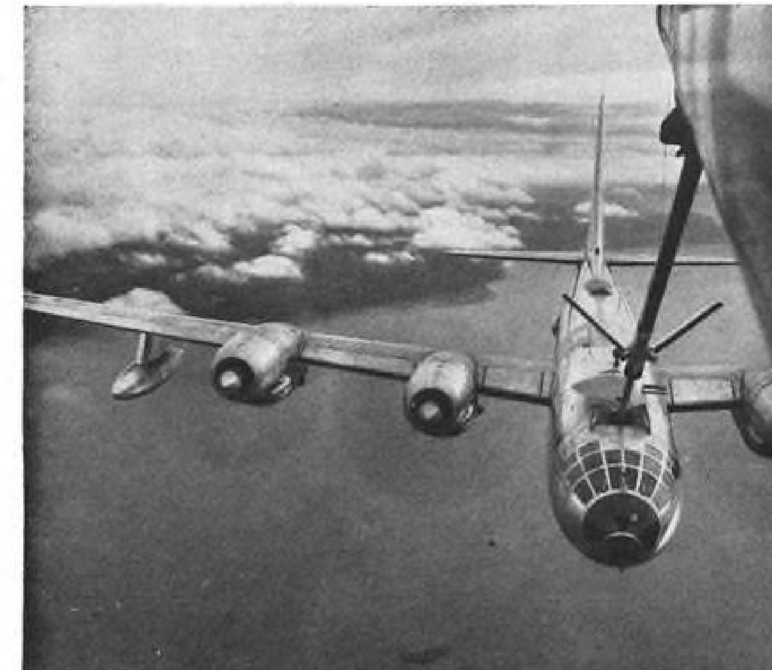
STEP-BY-STEP PICTURES , just released, show details of new Boeing Flying Boom aerial refueling system in actual mid-air operation. Above photo, taken from side sighting blister of B-29 tanker, shows B-50D taking on fuel load through telescopic boom.
