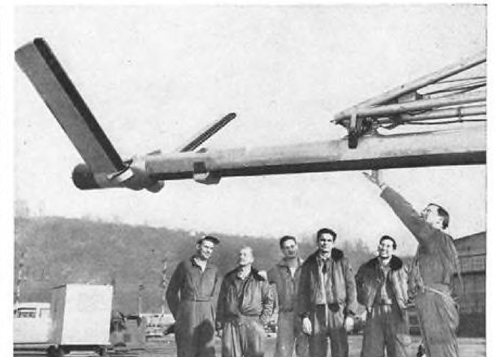
STOWED AWAY , the Boeing-developed Flying Boom refueling pipe is shown in a close-up as it is inspected by a flight test crew. Support rigging, holding boom in place, also can be seen in side and rear views of tanker in flight. Note anti-icing strips.
