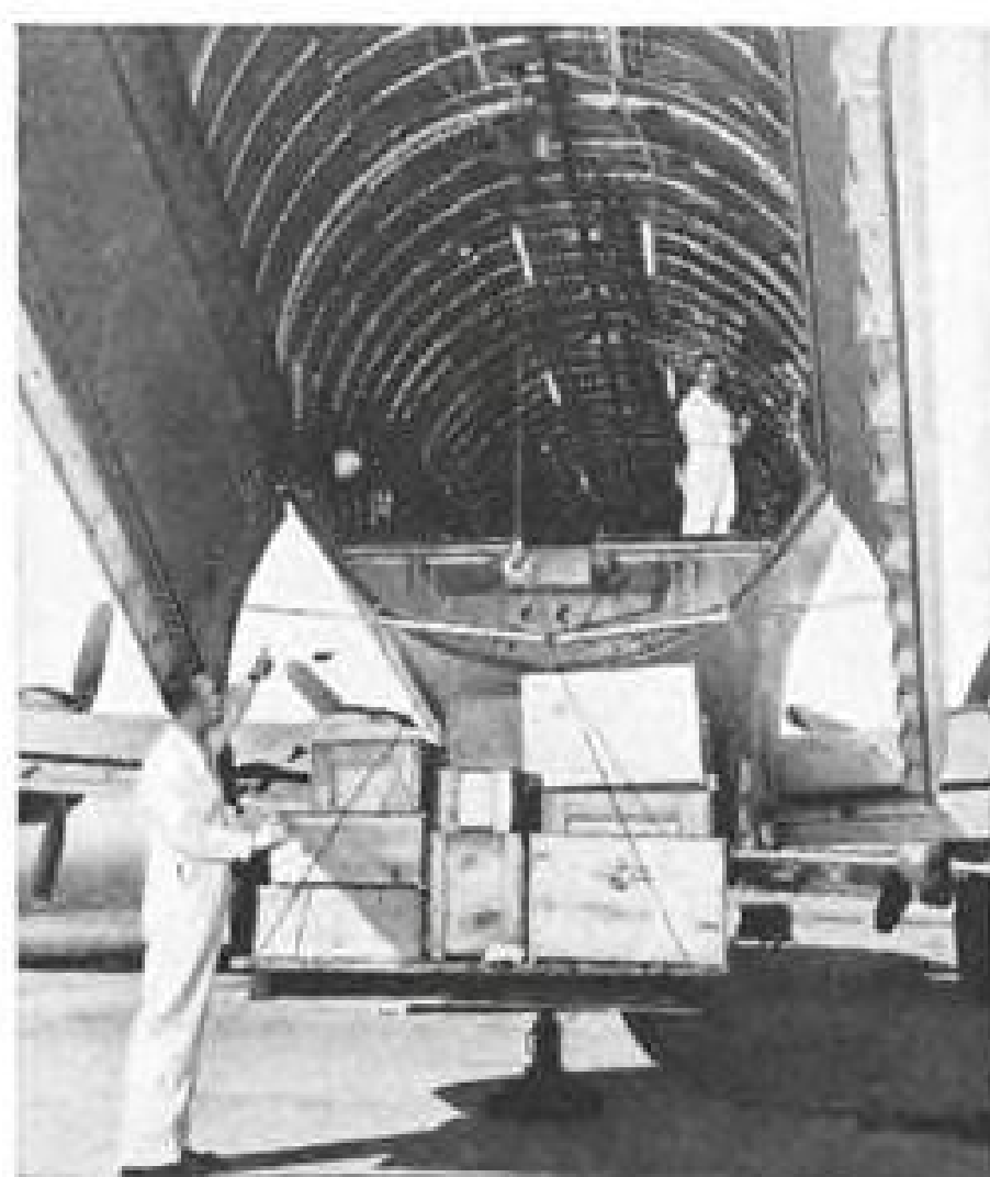
HOOK AND HOIST! Self-contained 5,000-pound capacity hoist and overhead rail facilitate positioning of heavy cargo in cavernous main cabin.
