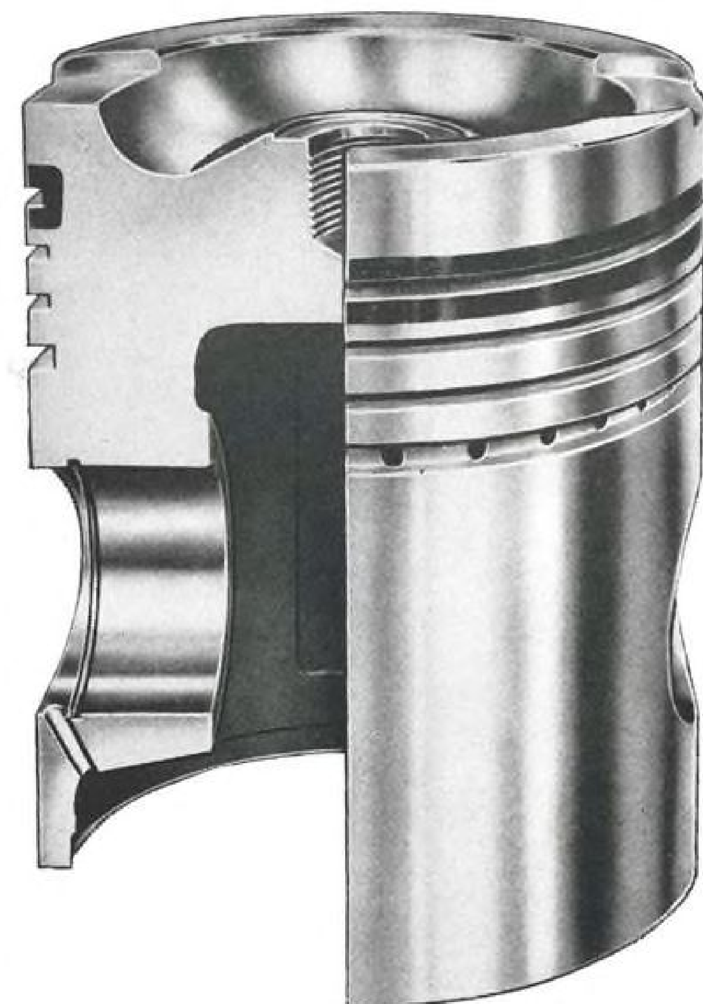
A NI-RESIST INSERT . . . bonded into aluminum alloy piston by the Al-Fin process.
