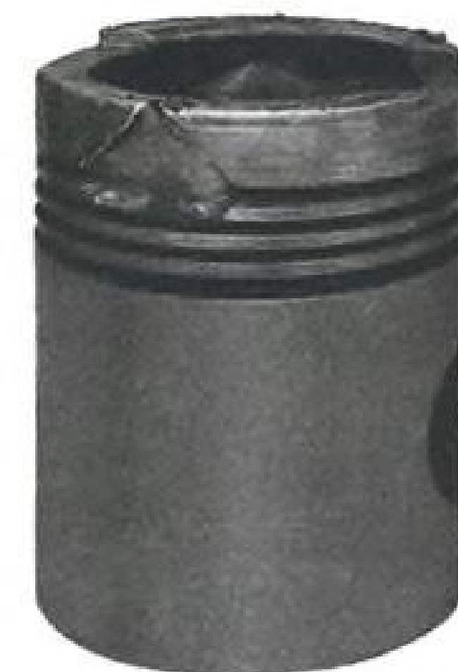
Standard aluminum alloy piston which failed in the top ring groove.
