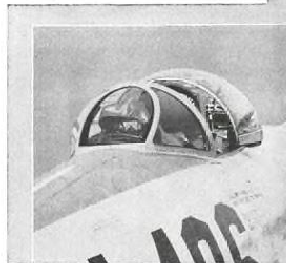
◀ One of the toughest glazing problems ever encountered was the windshield of the Shooting Star. It was solved by Pittsburgh specialists, with center panel of bird-resisting, bullet-resisting Pittsburgh Safety Plate Glass.
