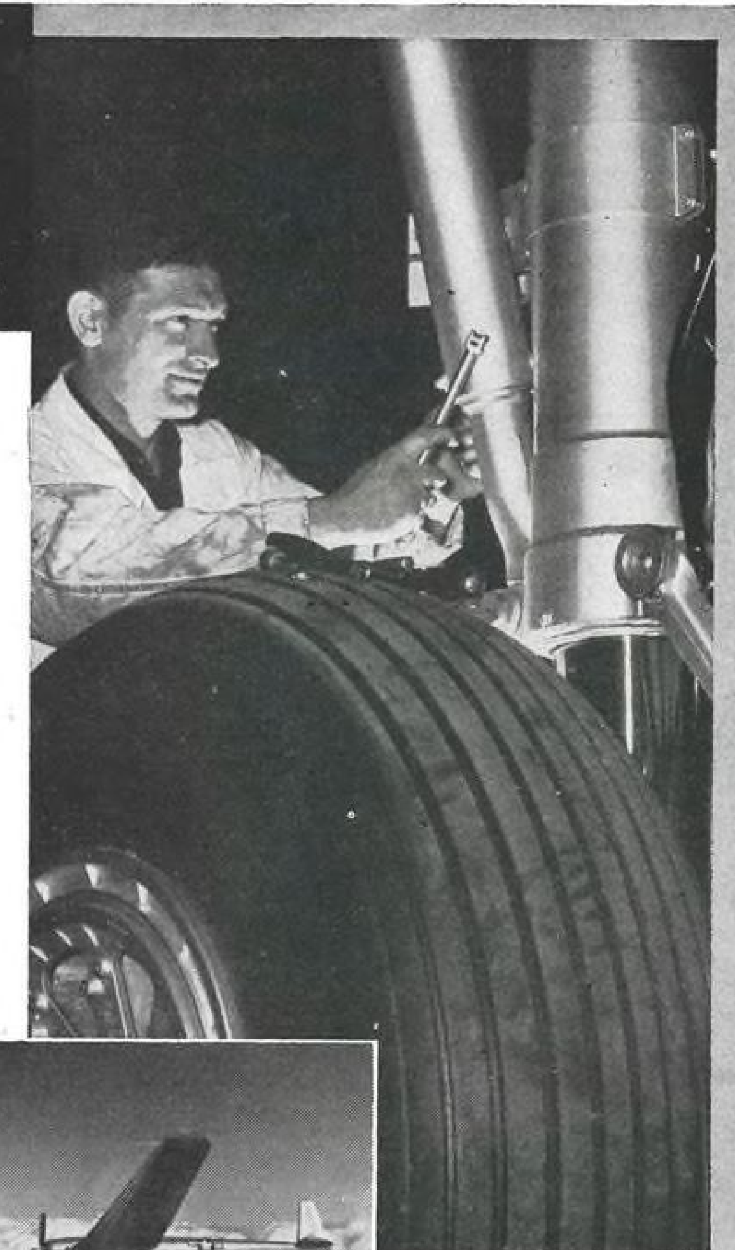
Breeze screw-jack actuator retracts the gear in 7 seconds.
