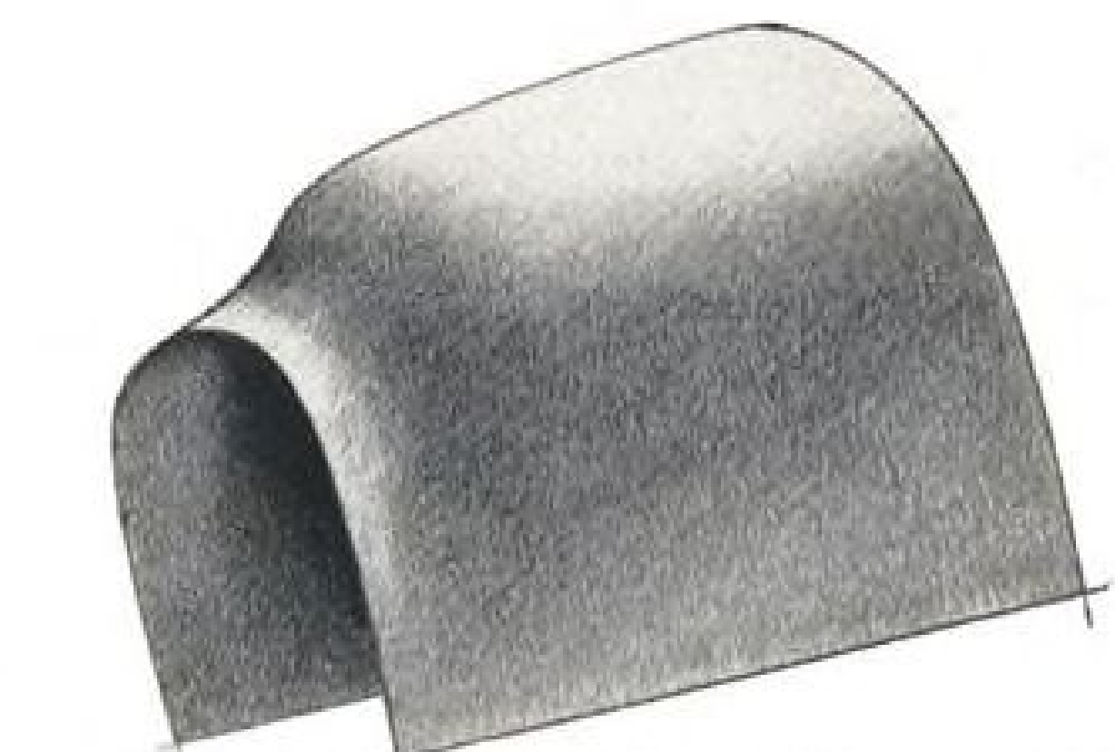
INTER DUCT NACELLE SKIN Formerly made of 24 SQ, now formed true at a time of 24 ST on a Hufford. Excessive breakage, heat treatment, refrigeration and straightening of parts experienced with original forming method now completely eliminated.
