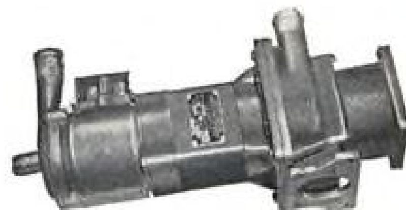
EXPLOSION-PROOF HYDRAULIC PUMP DRIVE Equipped with inline gear reduction. Gearbox designed to keep acoustic noise level at an absolute minimum. For continuous duty operation with duty cycle varying from 1-1/2 to 5 H.P. load. Designed to operate for 2000 hours without maintenance. Operates in a vertical position. Weight, 20-1/2 lbs.
