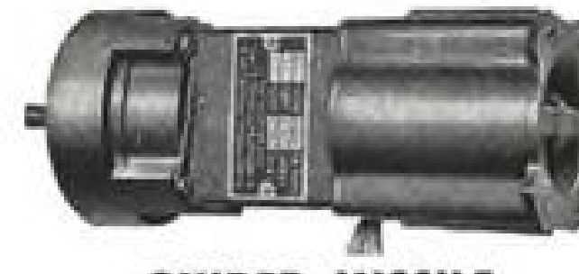
GUIDED MISSILE CONTROL MOTOR 3/4 H. P., 25,000 RPM, 10 minute duty cycle. Weight, 2.9 lbs. Silicone insulated. High temperature materials throughout. Temperature on outside of case at end of run, 250°C without damage to materials.
