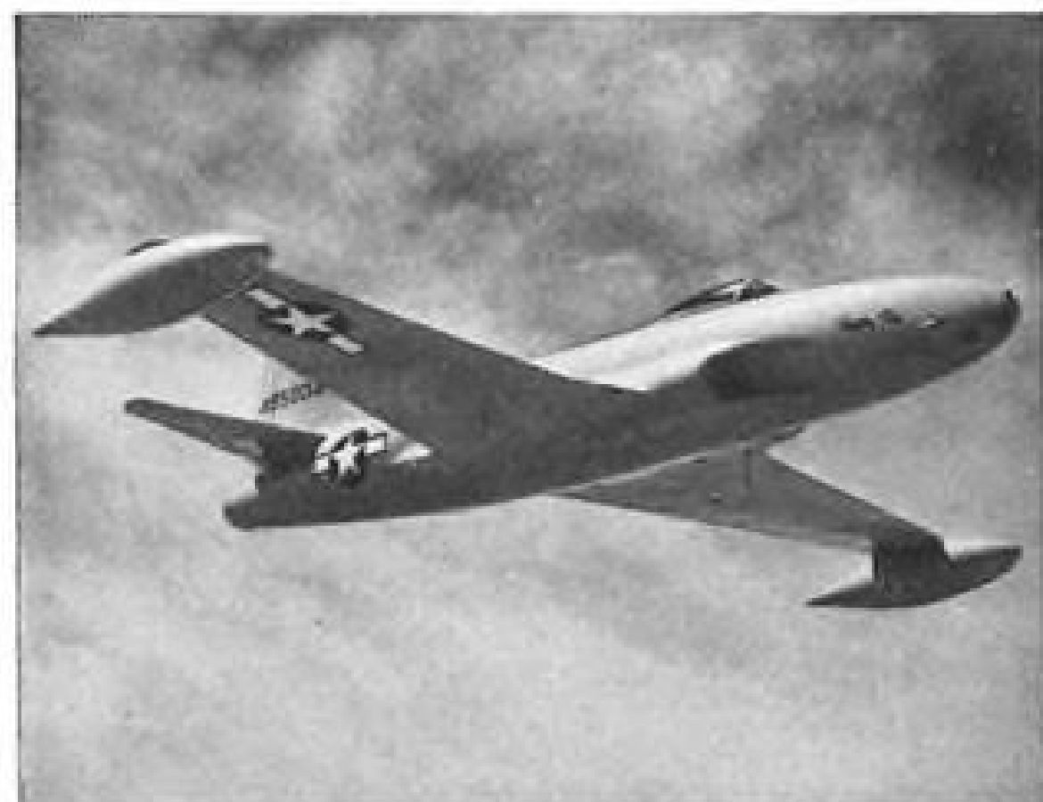
The J33 Turbo-Jet powers Lockheed's famous P-80 "Shooting Star." Inconel combustion chamber linings help extend engine life and reduce maintenance costs.
