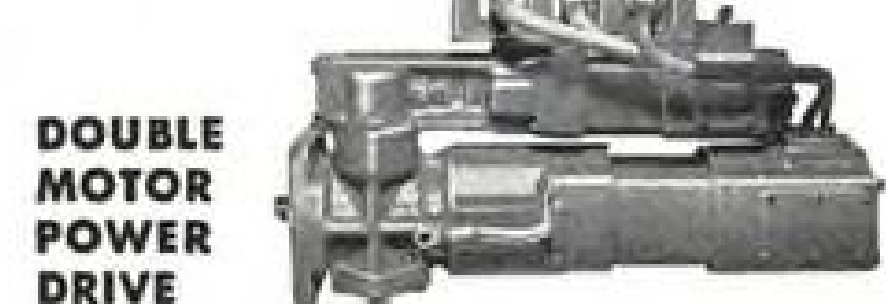
DOUBLE MOTOR POWER DRIVE Small motor operates in conjunction with automatic pilot. Large motor used for manual control. Small motor—helical and worm gear reduction. Large motor—no reduction. Outputs: Small motor, 1/15 h.p. continuous; large motor, 3.3 h.p., 6 sec. duty cycle. Output RPM: driven by small motor, 1000; driven by large motor, 10,000. Radio noise suppressors. 26 volts d. c. Weight, 16-1/2 lbs.
