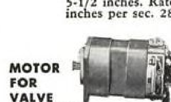
MOTOR FOR VALVE ACTUATOR Weight, 11.7 ounces. 2-5/8" long by 1-5/8" by 1-13/16". 20 watts output at 18,000 RPM, intermittent duty. 28 volts d. c.
