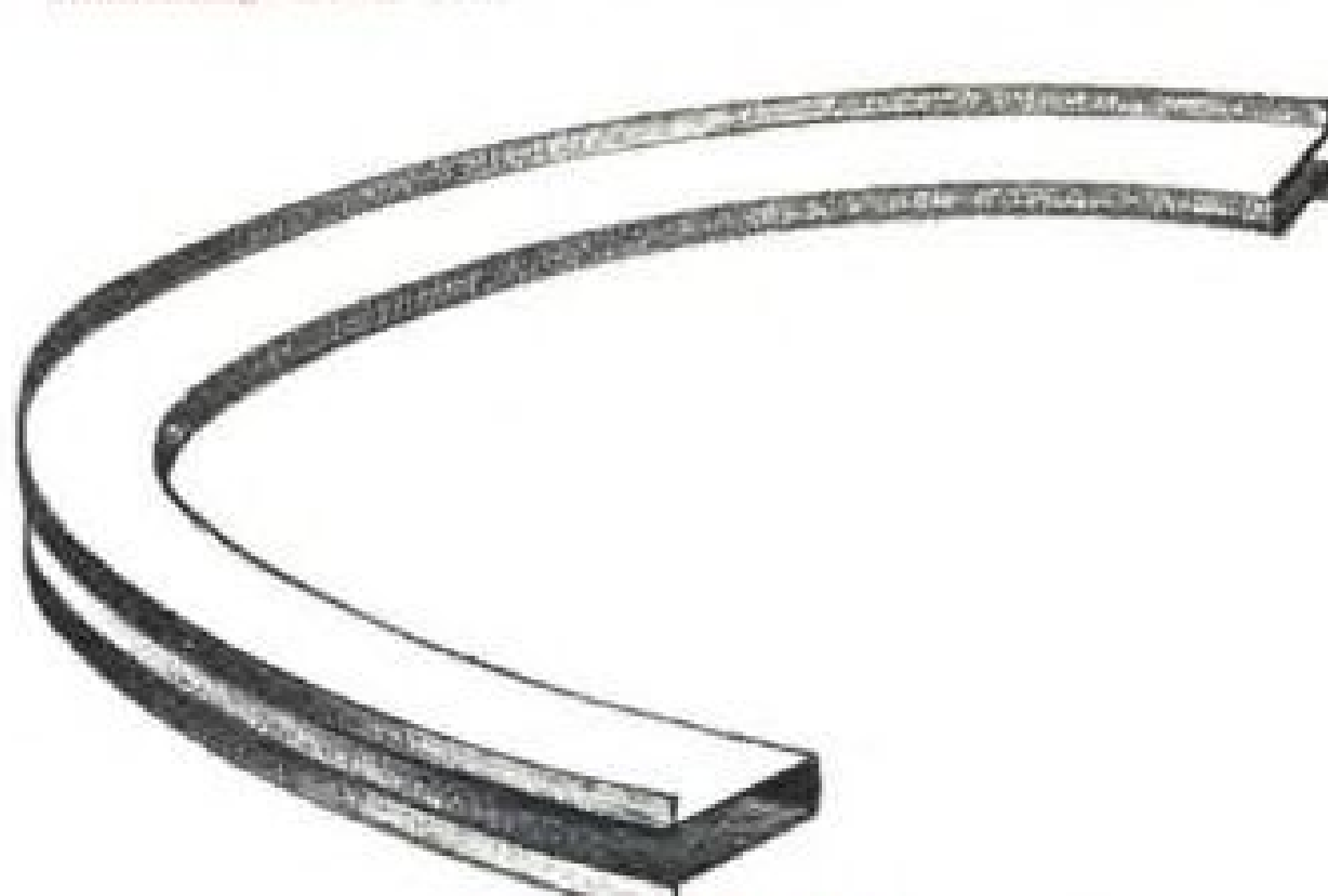
FUSELAGE FRAME Formerly made of two 1/2" sections welded together, this 1 1/2" hard stainless steel frame is now stretch-wrap formed in one operation from a blank formed hat section.
