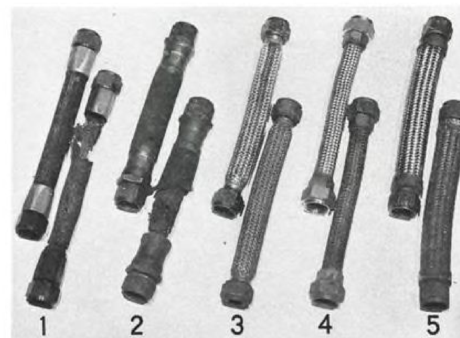
can occur in vacuum system, which can attain 1600-1800 F. temperature. Hose 1 withstood fire for approximately 1½ min.; hose 2, for about 5 min. Hoses 3 (stainless steel), 4 (Inconel), and 5 (stainless steel) withstood test fire for 10 hours without damage.
