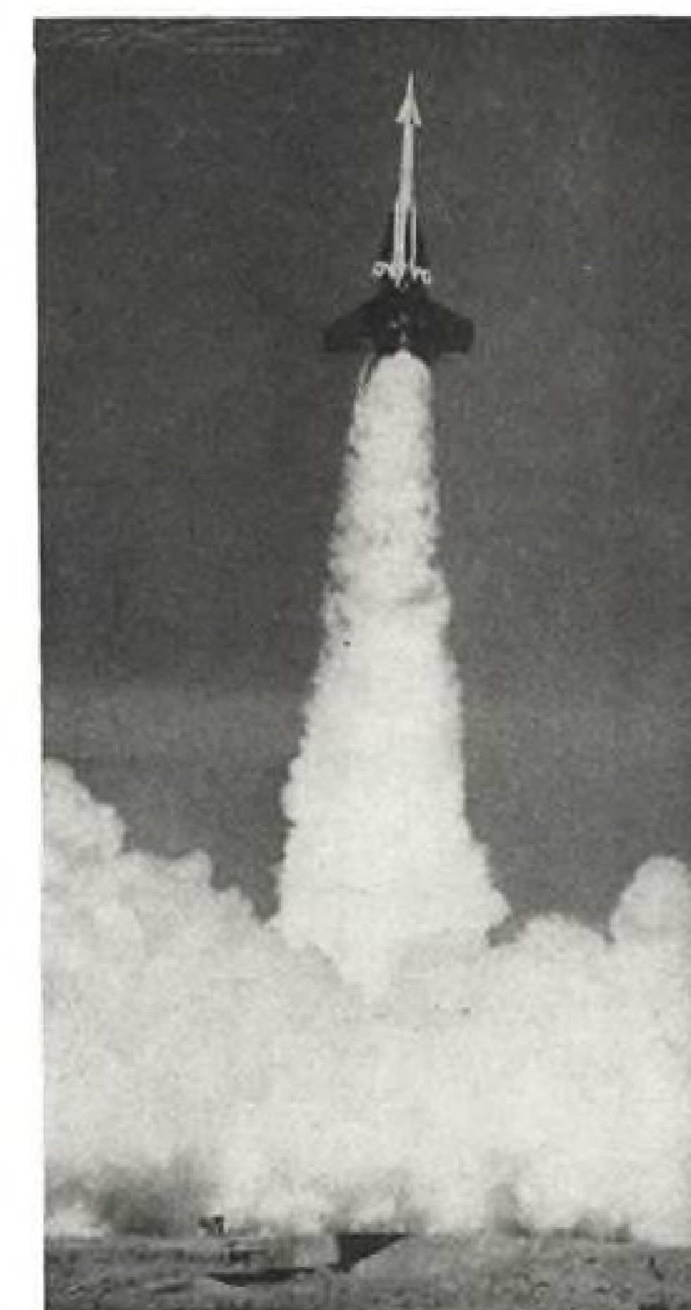
NIKE, rocket-powered army anti-aircraft missile, has four-finned booster rocket on tail.
