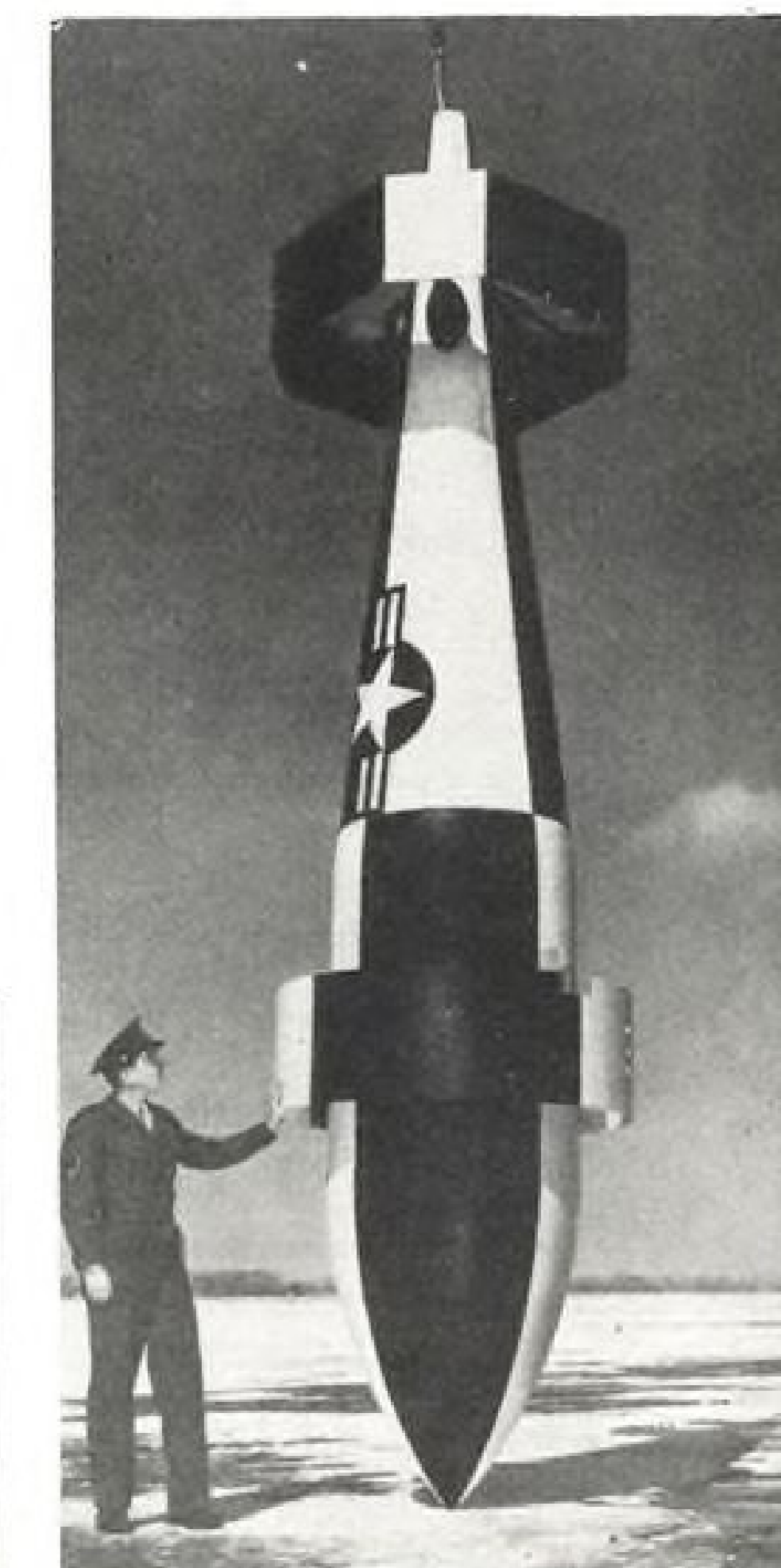
TARZON, Bell Aircraft Corp.'s 12,000-lb. bomb, can be guided during descent by electronic commands from bombardier.
