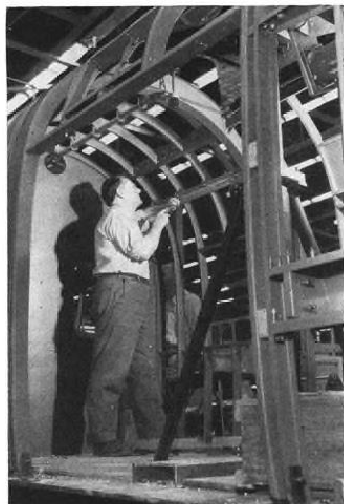
ALUMINUM ARCHES for the H-19's skeleton are bolted to the fuselage jig. Note ample working room.
