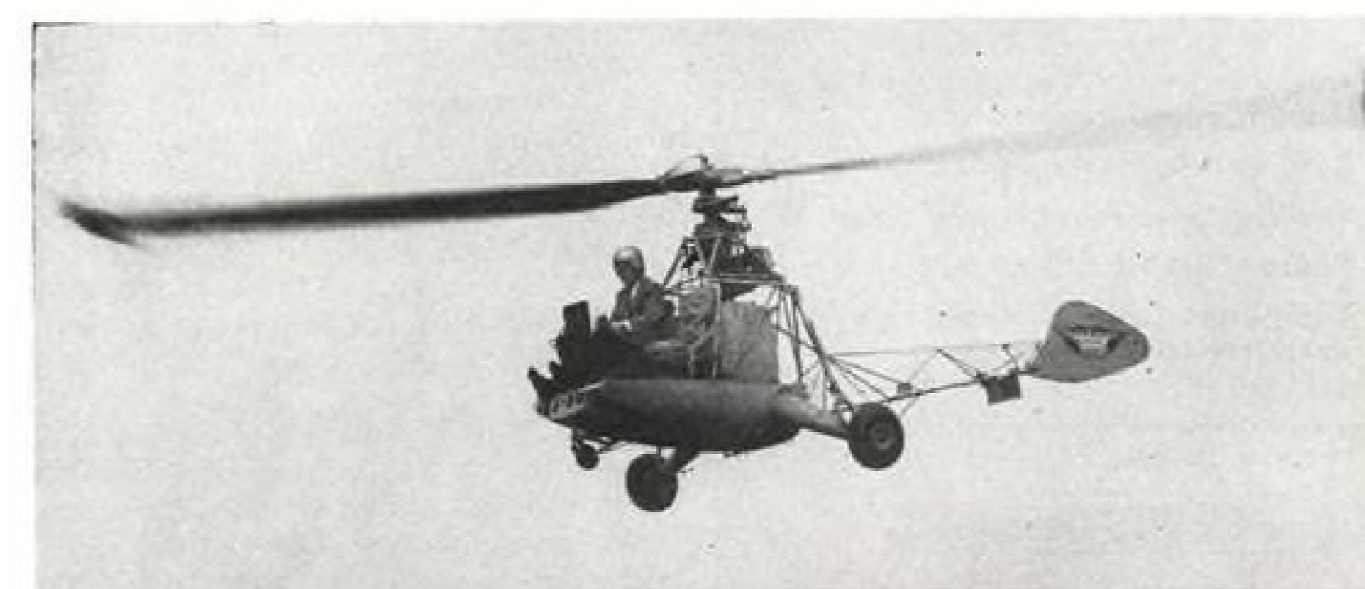
TOP SERGEANT XA-5 pulsejet copter has 33-ft. rotor turned by engines at tips.
