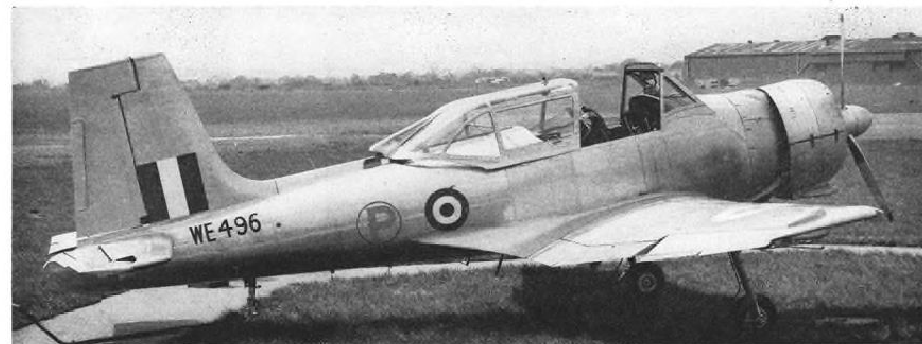
HANDLEY PAGE H.P.R. 2 side-by-side, all-metal construction trainer combines slow stalling speed and quick takeoff characteristics.
