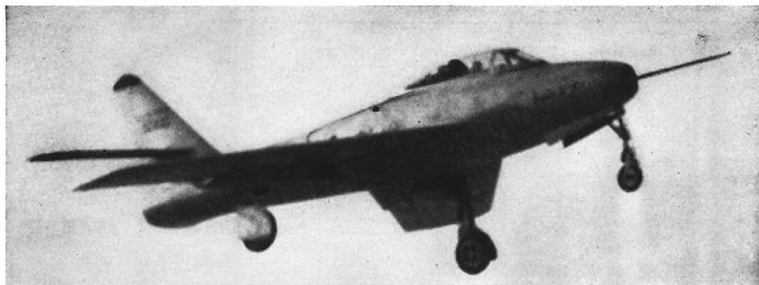
YF-96A Takes off from Muroc on first flight piloted by Republic's O. P. Hass. Flight lasted an hour. Craft uses 60 percent of F-84 tooling, has a 5200-lb. thrust Allison J-35-A-25.
