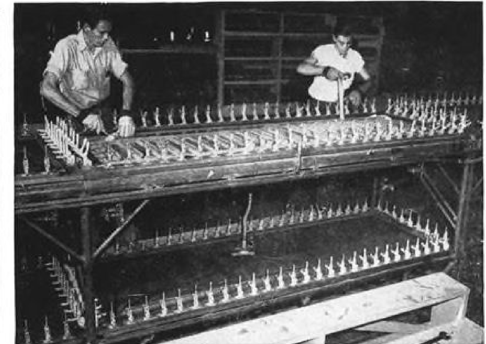
REMOVING the cured assembly from pressure fixture is quickly done, although care in handling magnesium alloys is necessary to avoid deformation due to temperature.
