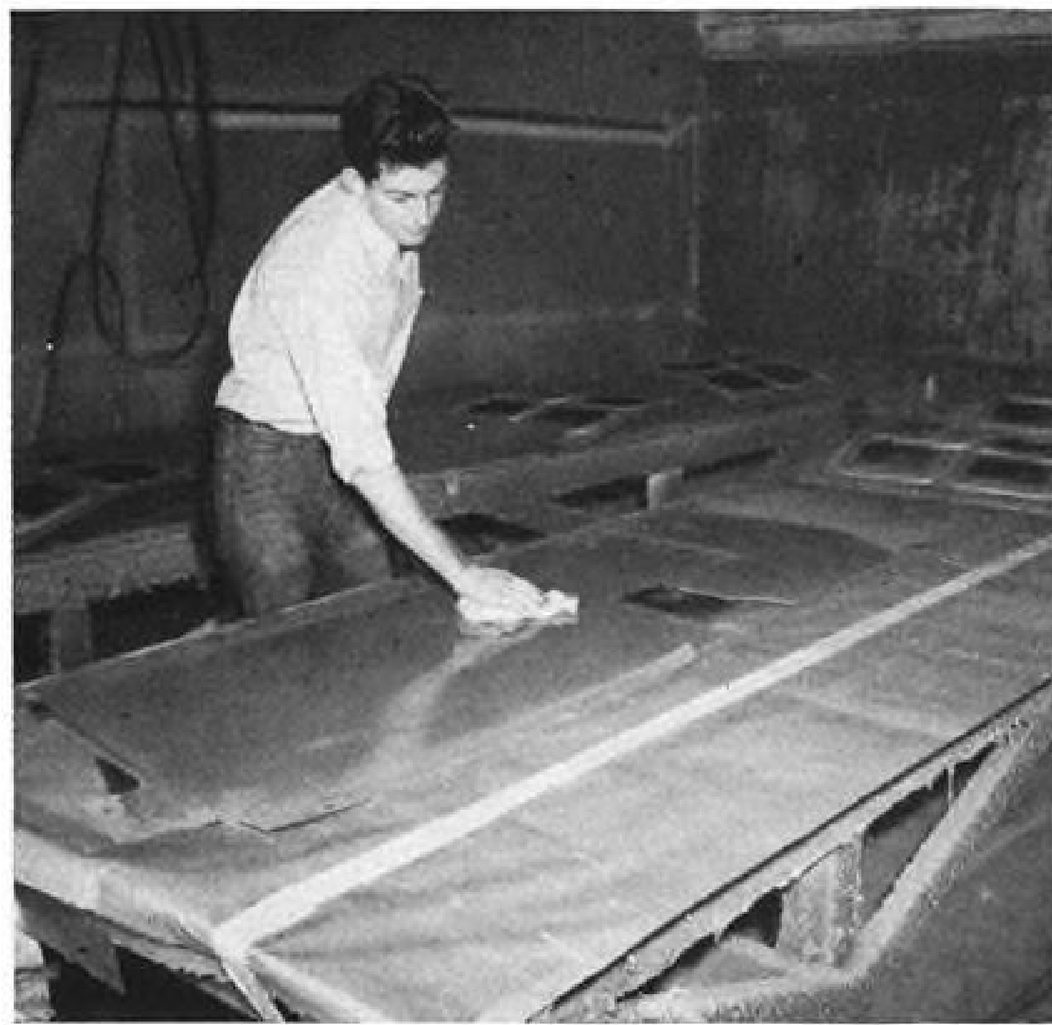
CLEANING process for magnesium alloy requires wiping with low-flash naphtha. Primer previously applied is not softened if low-aromatic cleaner is used.
