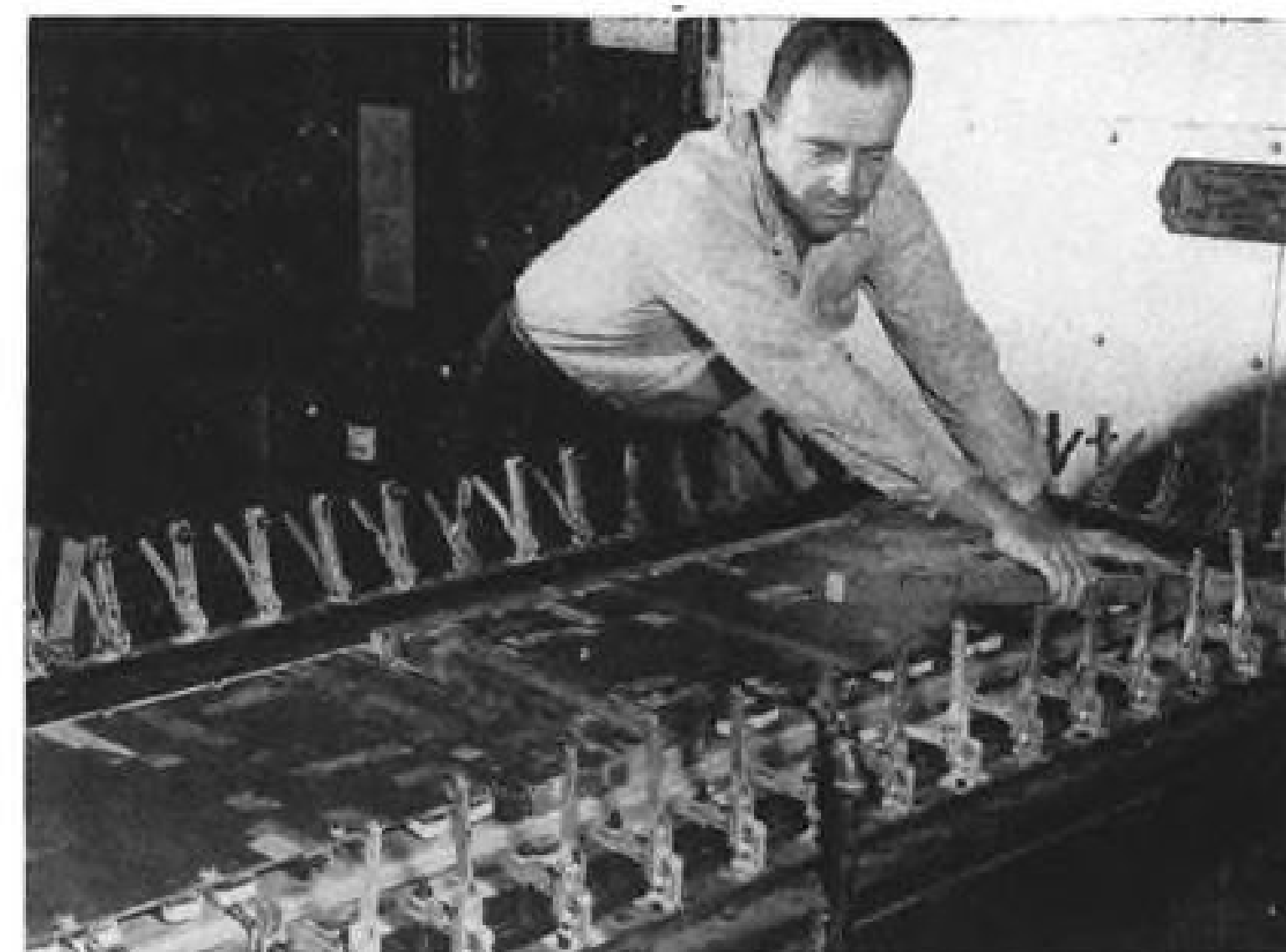
LOADING assembly in pressure fixture requires extra blocks for doubler edges. Locating jig, shown inverted here, must be flexible for uniform loading of filmed parts.
