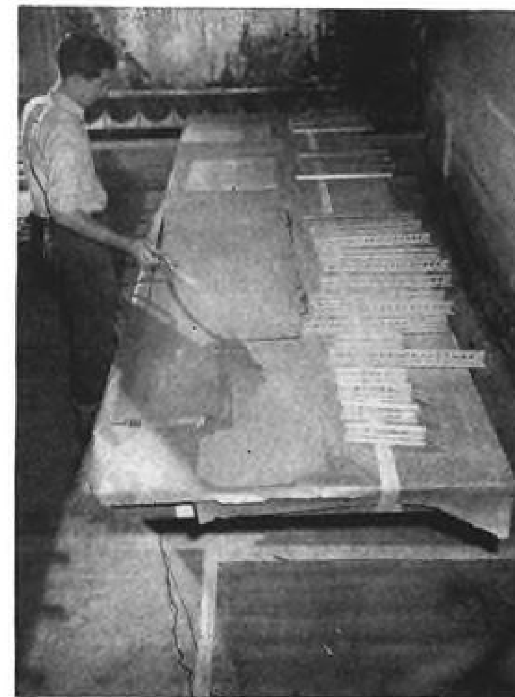
SPRAYING of two thin coats of M3C cement follows cleaning. Laboratory tests now being made may eventually eliminate this phase of Metlbonding.
