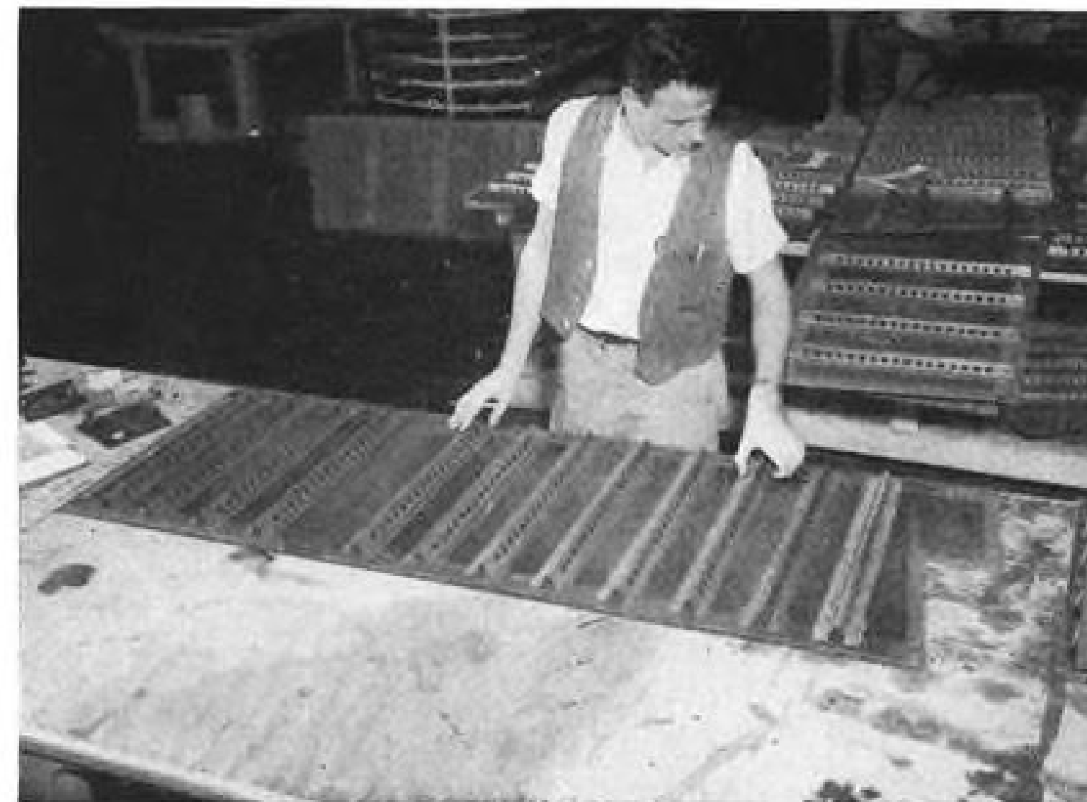
INSPECTING of B-36 elevator panel includes visual check for voids, delaminations or poor bonding. Magnesium alloy parts get dip coat of zinc chromate after inspection.
