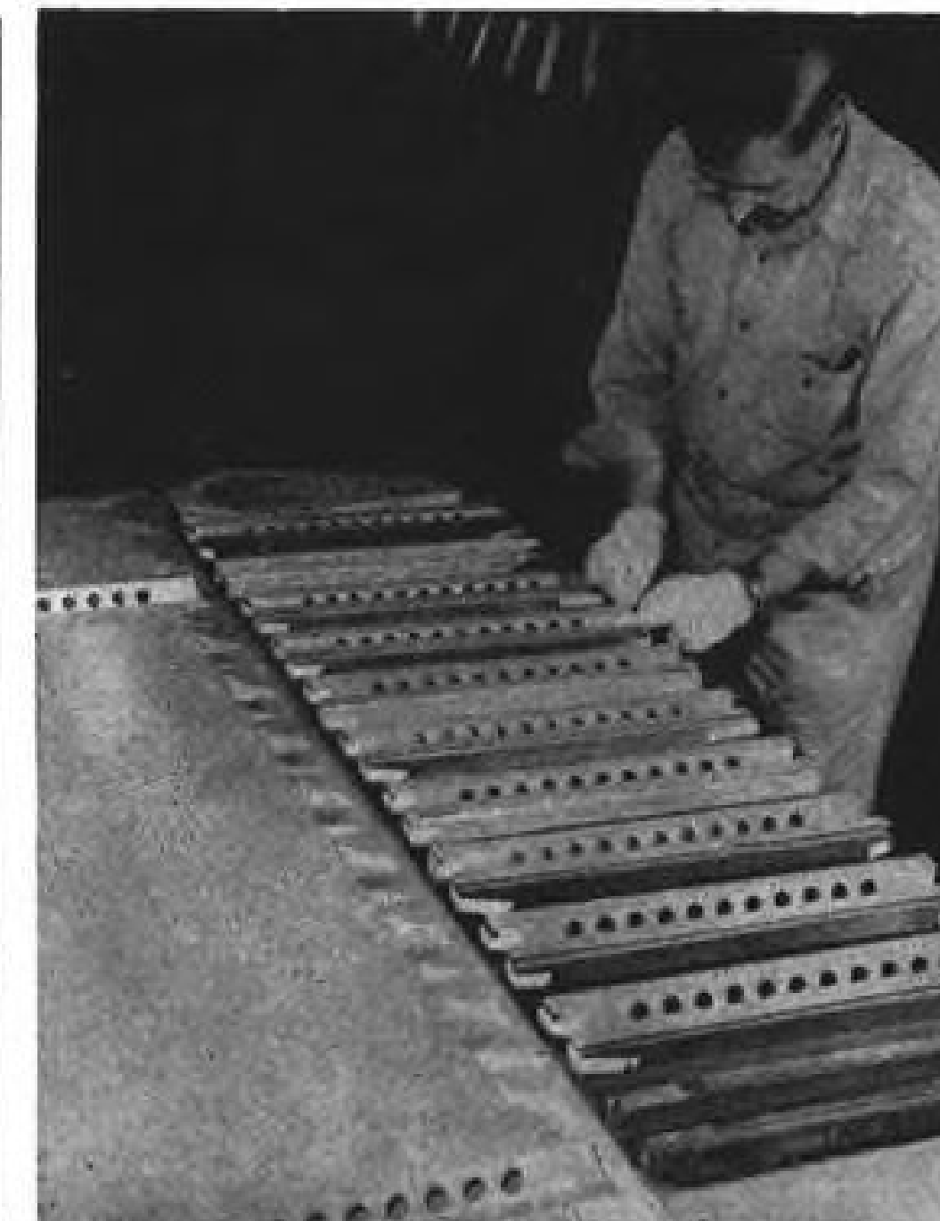
FILMING is shown being done on legs of hat-section stiffeners. Jig blocks distribute pressures uniformly on parts when rubber blanket is used.
