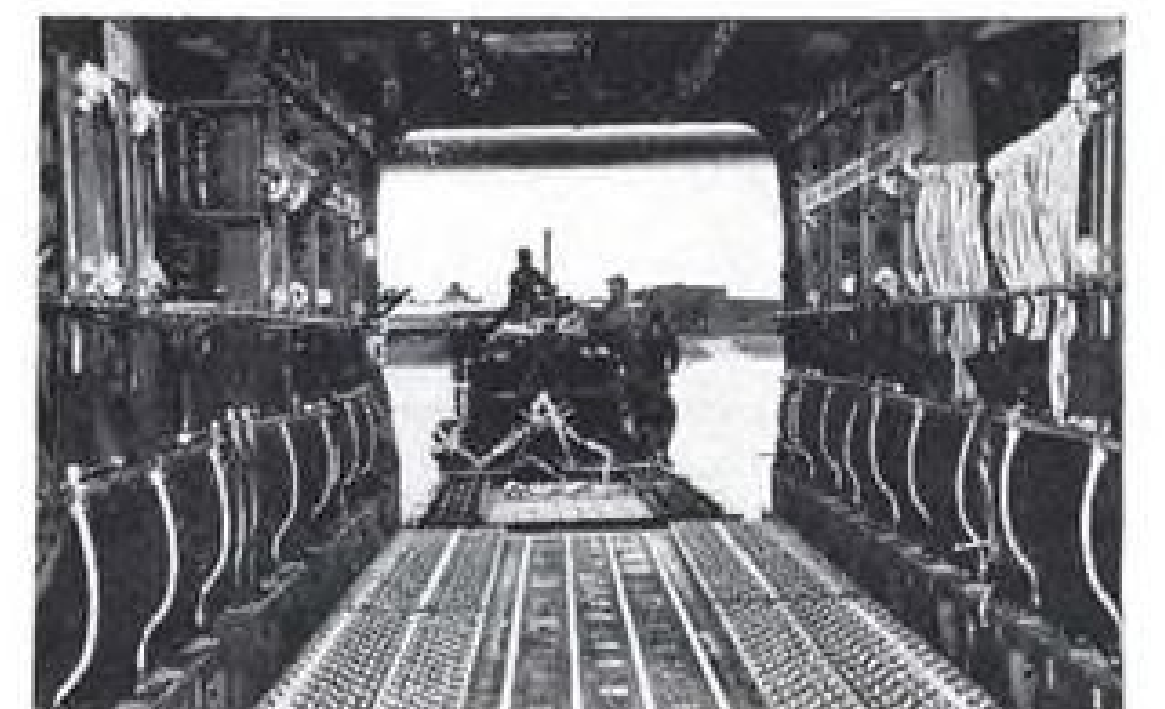
BOXCAR FUSELAGE permitted rapid loading of large, bulky equipment . . . no dismantling or ground handling equipment needed. Vehicles loaded and unloaded under their own power!
