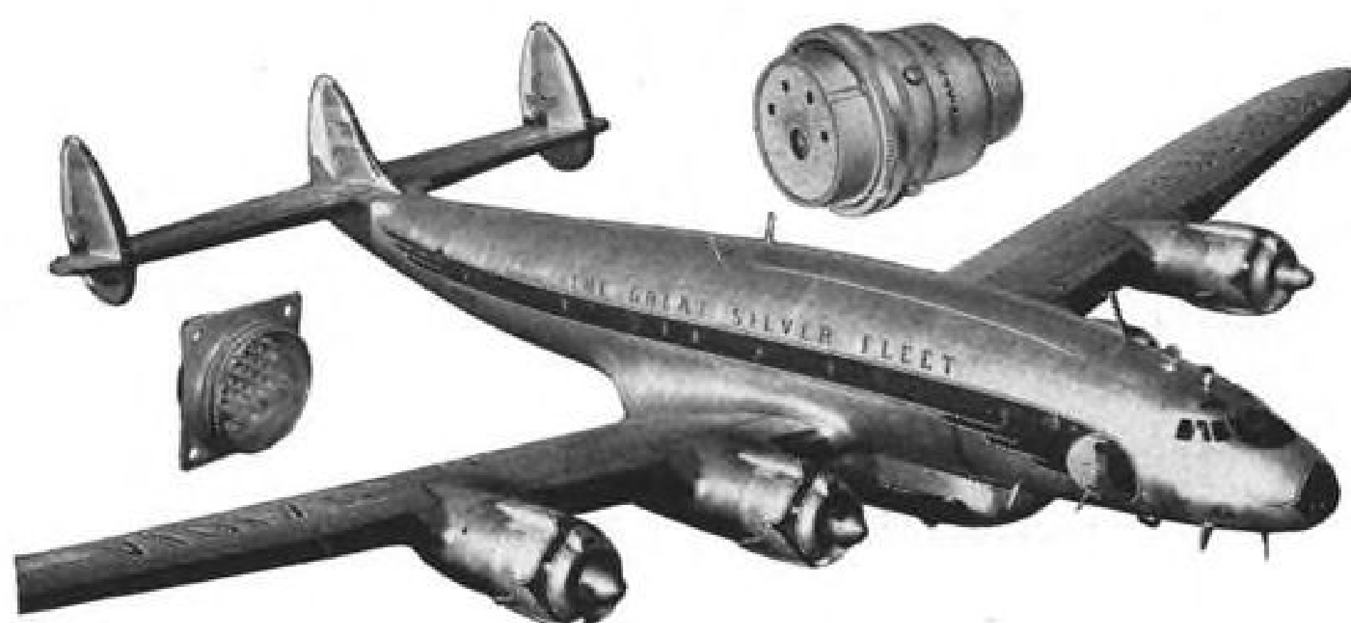
Arrows point to several Cannon Type K Firewall Connectors on portion of Constellation Engine Firewall. Included are Flame Barrier and Fireproof Types.
