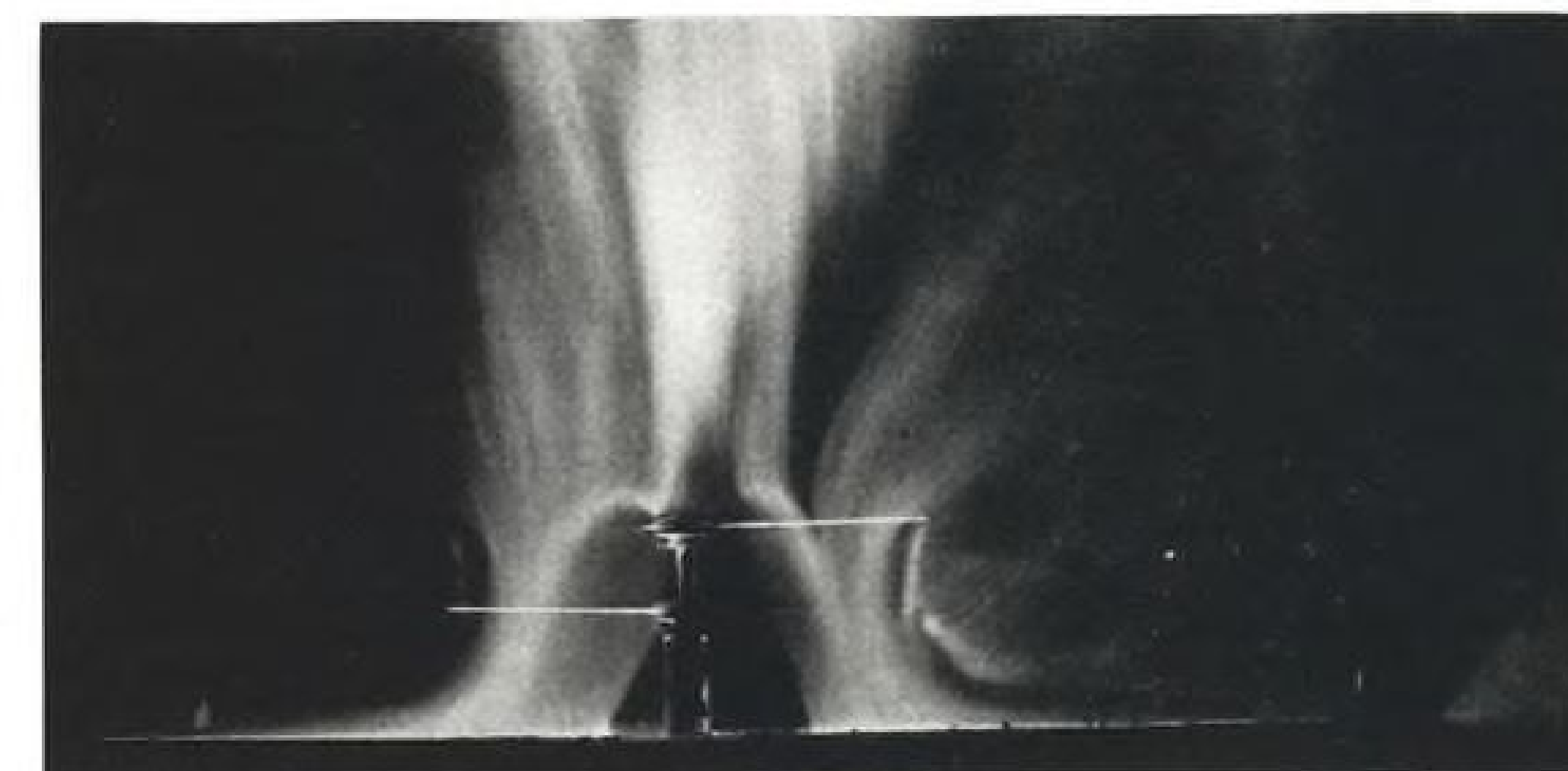
METHOD SHOWS static thrust geometry of rotor wake and trailing vortices from blade tips of coaxial rotor. Balsa particles show . . .
