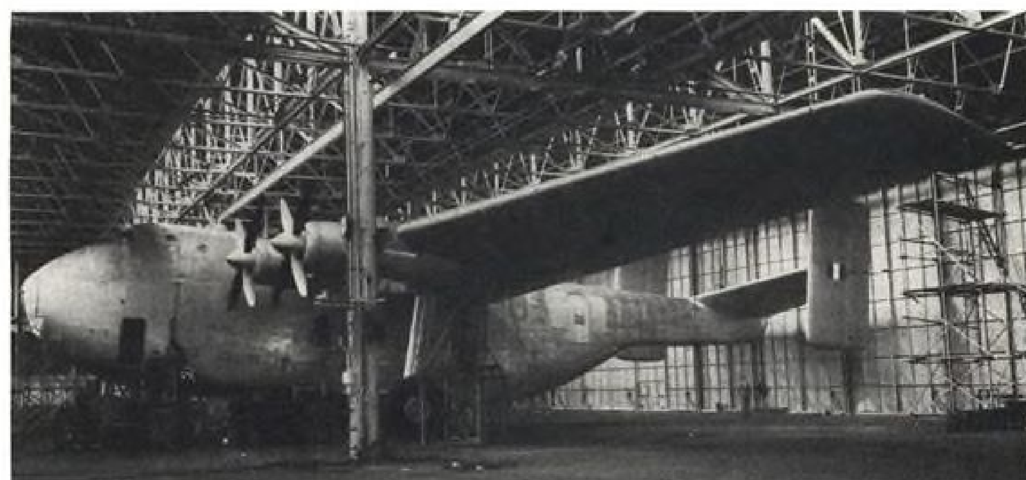
UNIVERSAL FREIGHTER'S upswept aft end has integral ramp. With ramp down . . .
