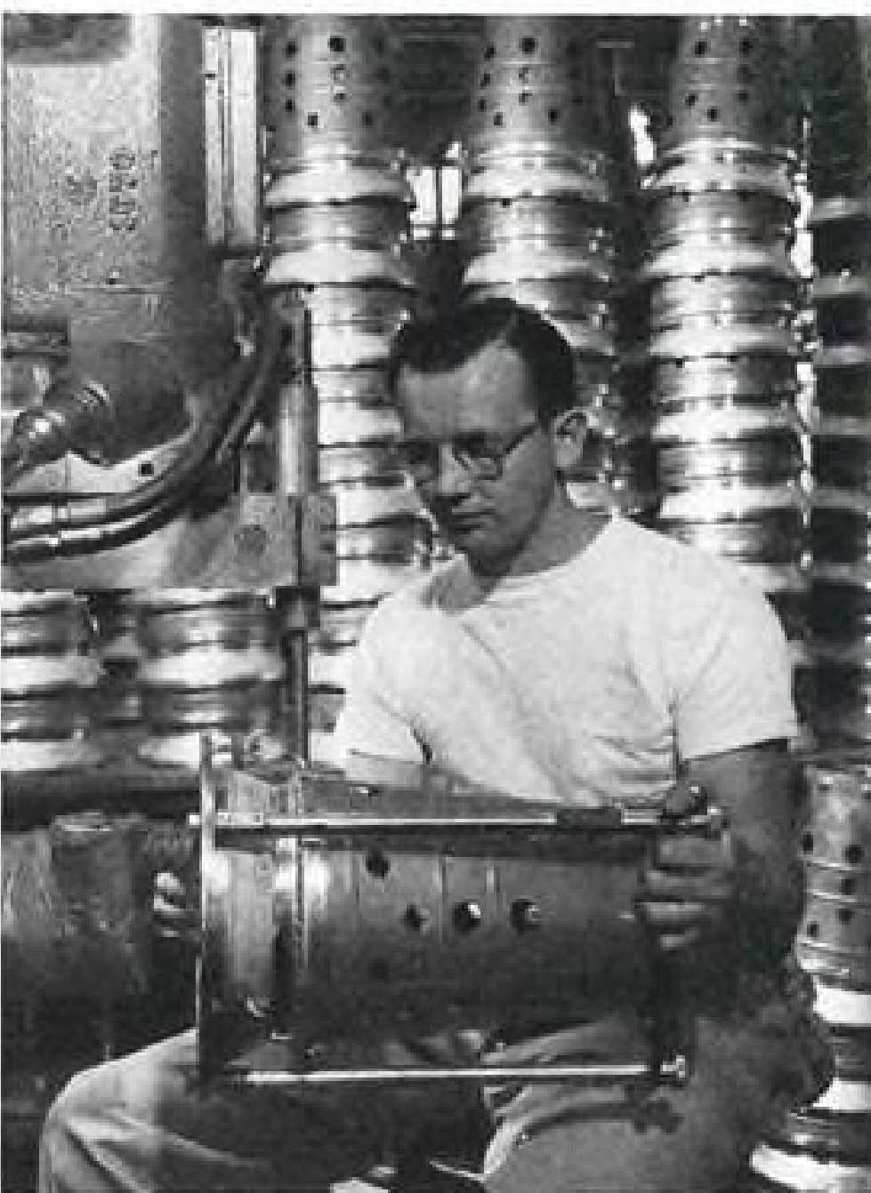
WELDING AID Special jig allows precise weld work. Tack welding is done on combustion chamber liner with no danger of position change.
