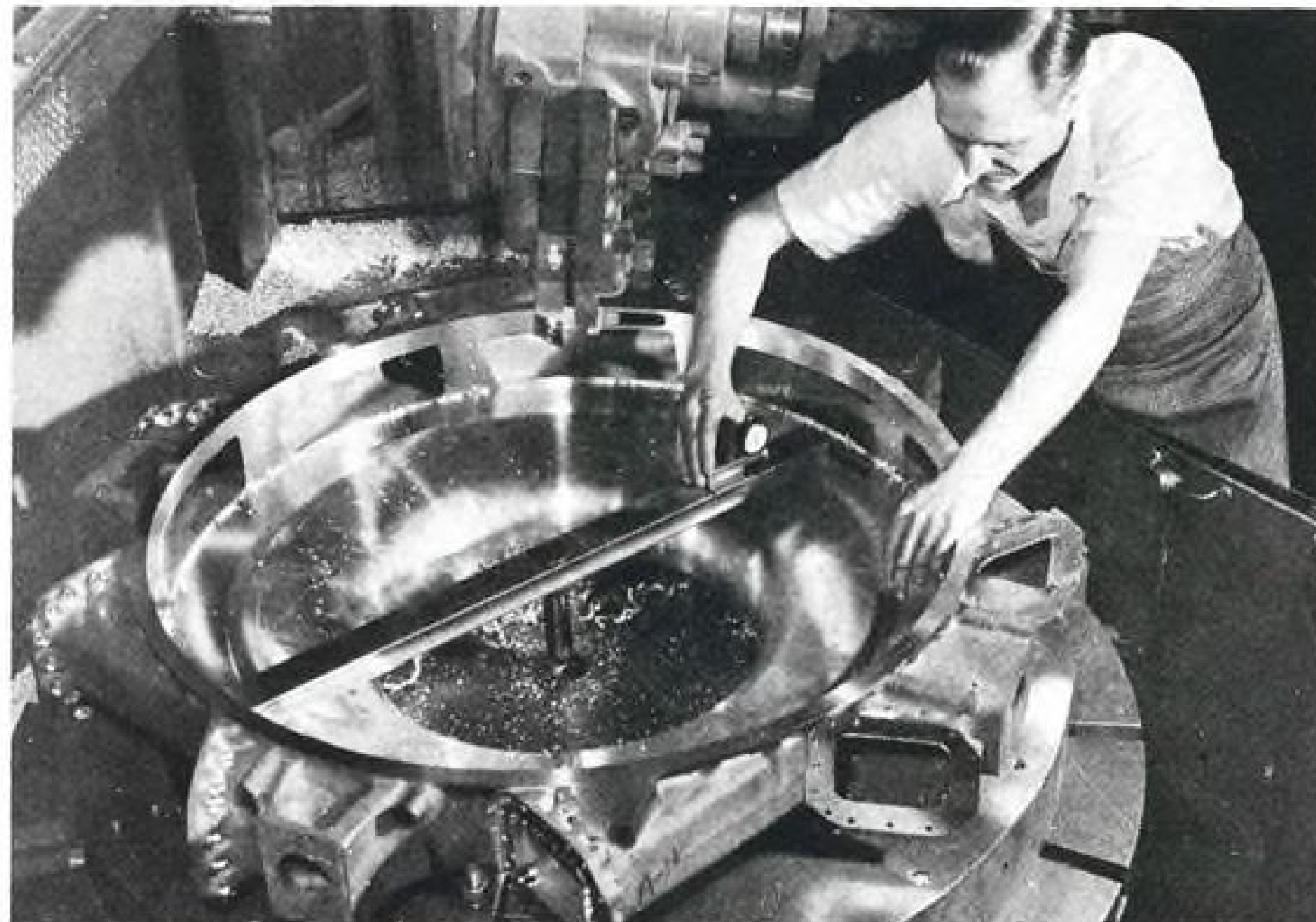
MIRROR SMOOTHNESS Compressor case receives highly machined surface accurate within 50/100,000 in. High velocity air from compressor is guided by this surface to the combustion chambers without inducing turbulence that would cut down engine efficiency, so close gaging is needed.
