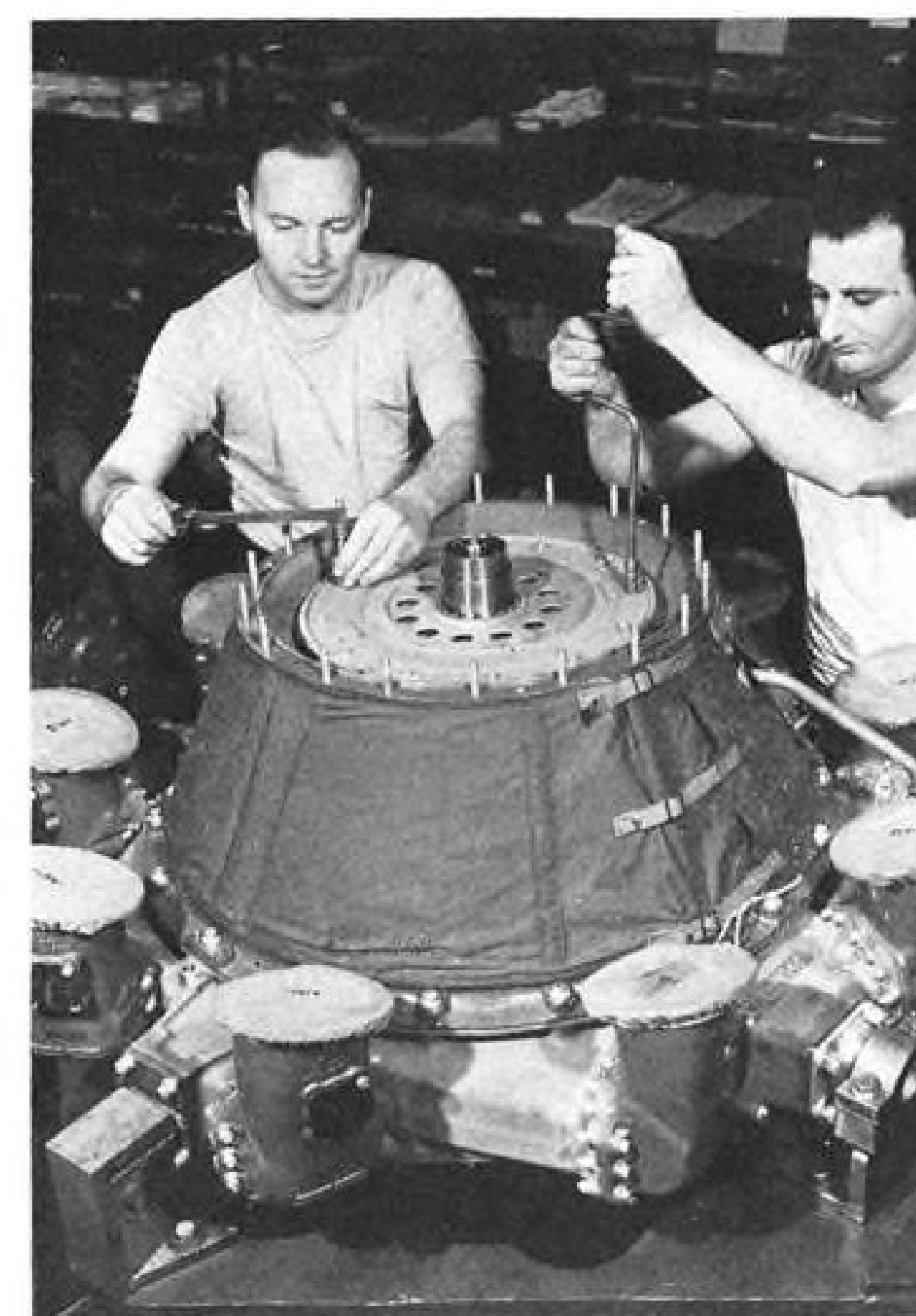
GREEN ASSEMBLY Compressor unit forms base on which engine assembly is built up. Covers are used to exclude dirt.
