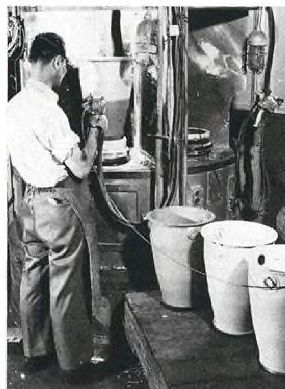
METAL SPRAY Low carbon steel chamber receives atomized aluminum protective coating. Wire is fed through torch for melting.
