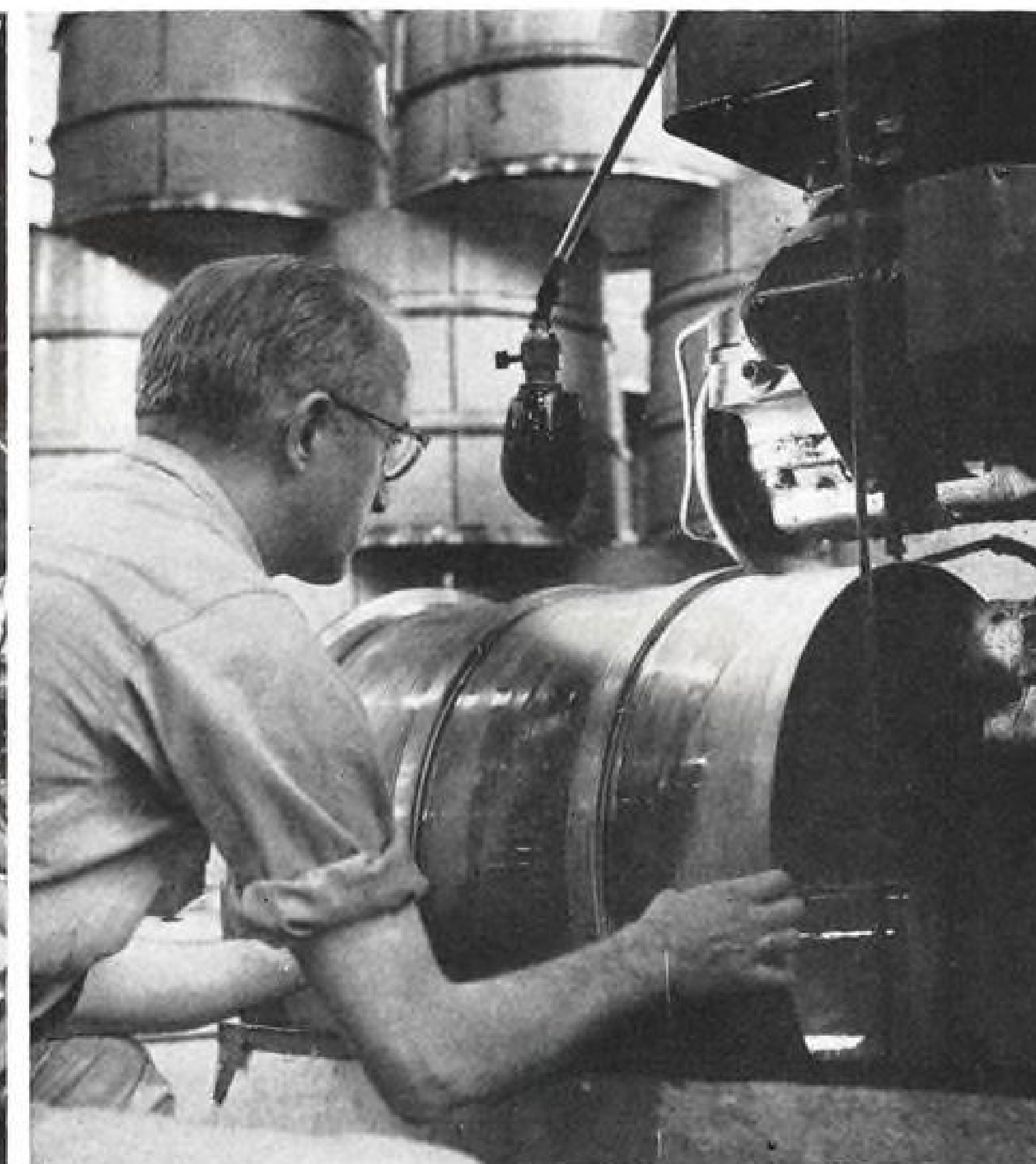
TAILPIPE WELD Here a craftsman puts seam weld on the outer stainless steel casing of the tailpipe. The welding machine is checked carefully for accuracy before production operation begins. Tube sprays cooling water over weld contact spot.
