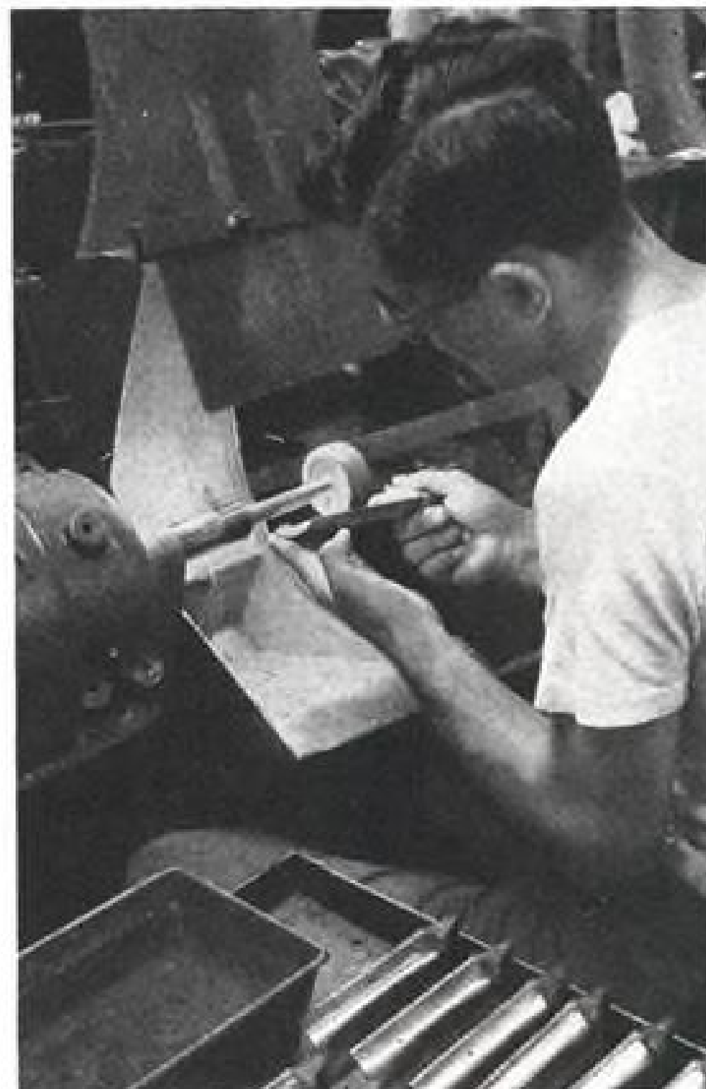
BUCKETS Before attachment to the rotor disk, each bucket gets careful polishing to give finish that will stand up under high turbine heat.
