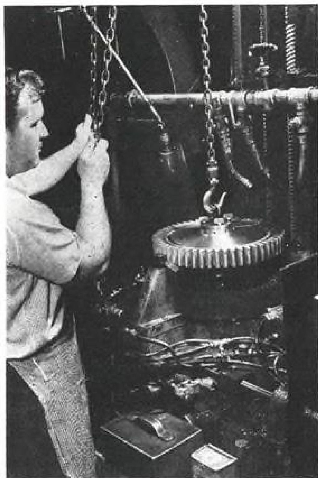
BROACHING The turbine wheel is readied for buckets. Setup of broaches cuts 54 precise pinetree slots in the solid turbine rotor.
