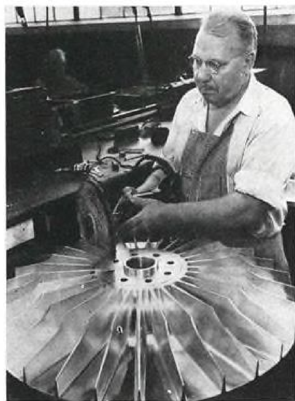
BUFFING High velocity airflow in the double-sided compressor also requires smooth finish. Each blade receives high polish with hand-held buffer.
