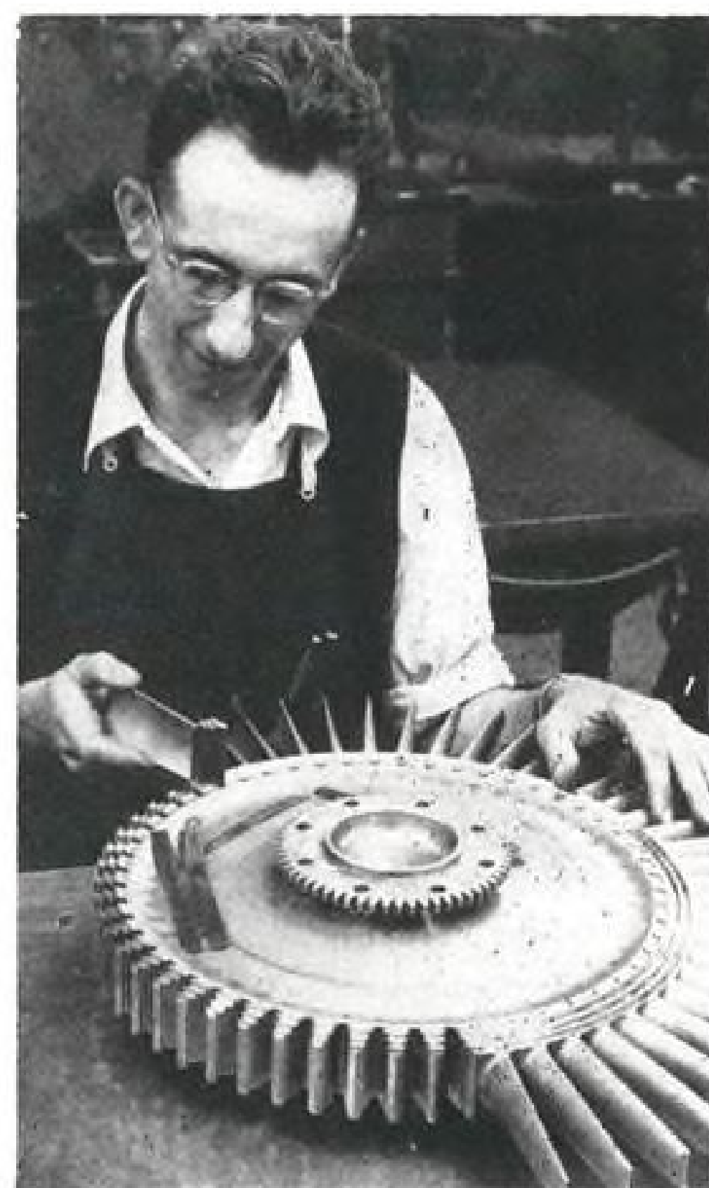
FITTING Assembled on rotor disk, buckets are fitted with a tip movement of 78/1000 in. to allow for expansion and contraction in service.
