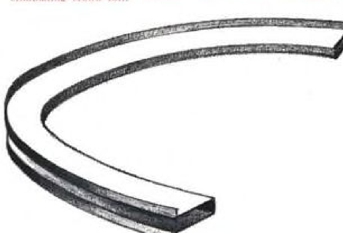
FUSELAGE FRAME Formerly made of two 1/2" sections welded together, this 10' long stainless steel frame is now stretch-wrap formed in one operation from a brake formed flat section.
