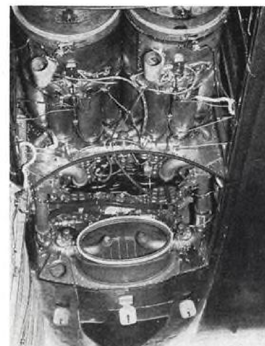
PAIRED POWER UNITS of the compact Allison XT40-A-4 turboprop, seen from the bottom, looking forward. Behind oil cooler rear face are bleed-air augmentors to improve on-the-water cooling.
