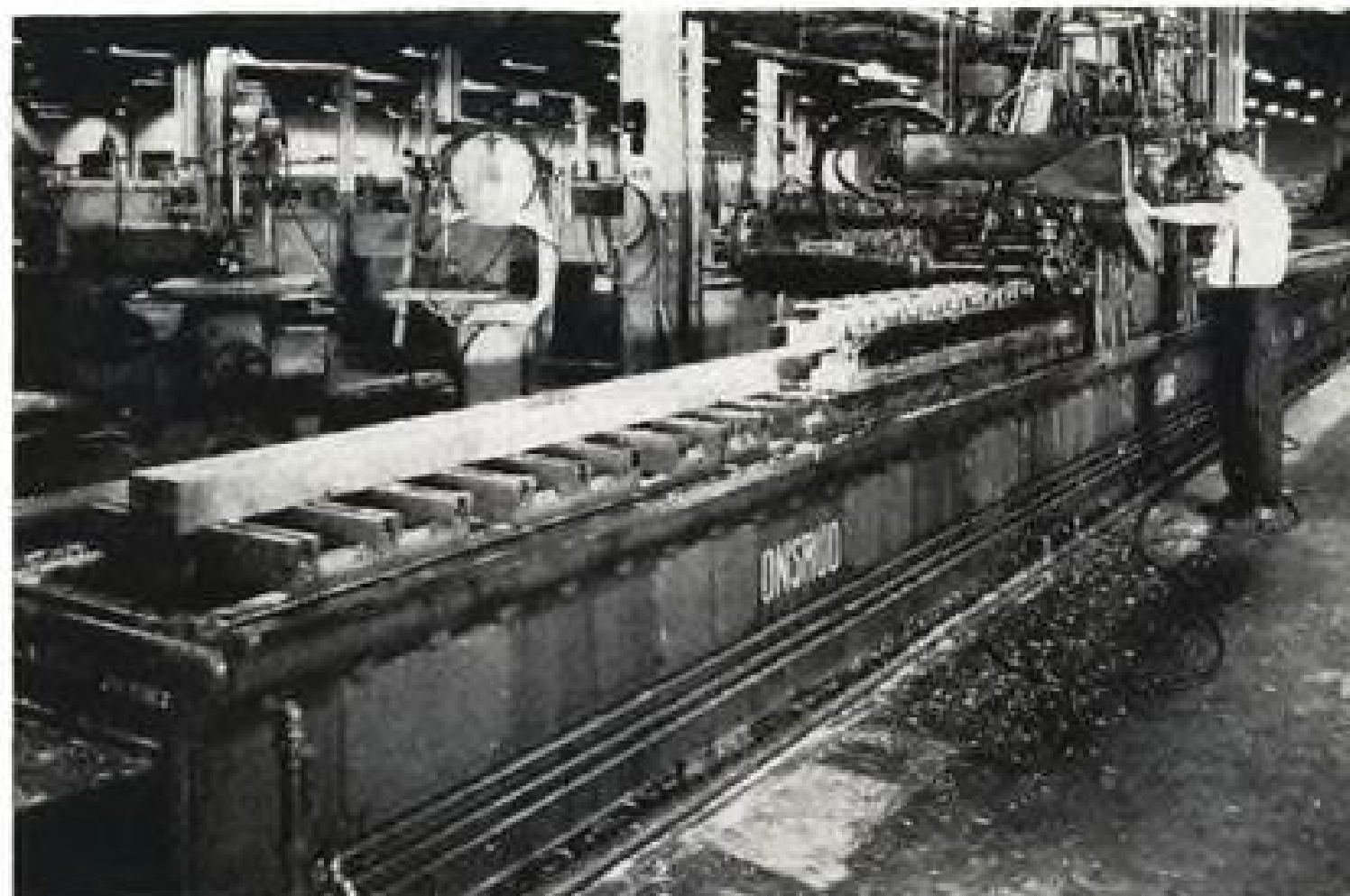
MILLING MACHINE at Boeing' Seattle plant can handle 85-ft. long spar; automatic joggler will replace three punch presses.
