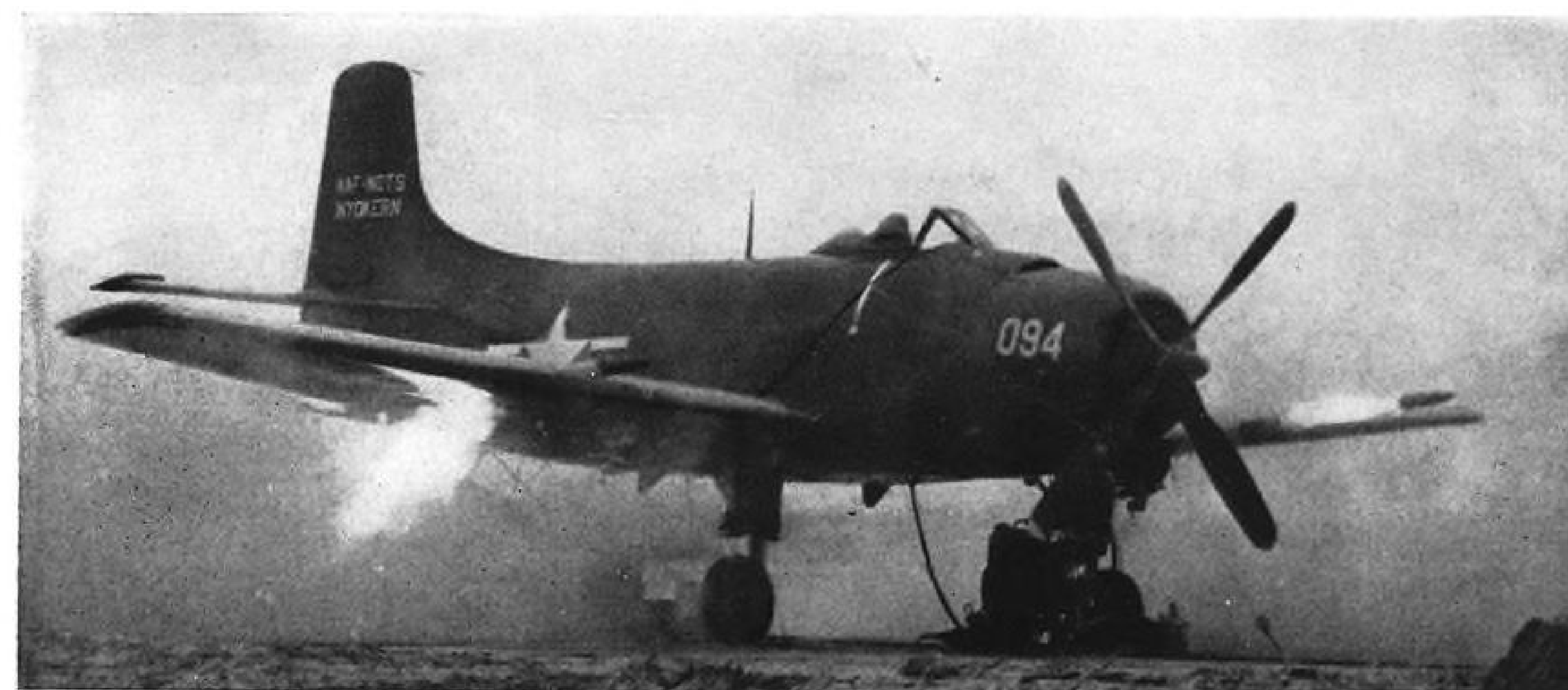
SUBMERGED LAUNCHER for 5-in. spin-stabilized rockets replaces externally hung projectiles, trebles firepower of Skyraider.
