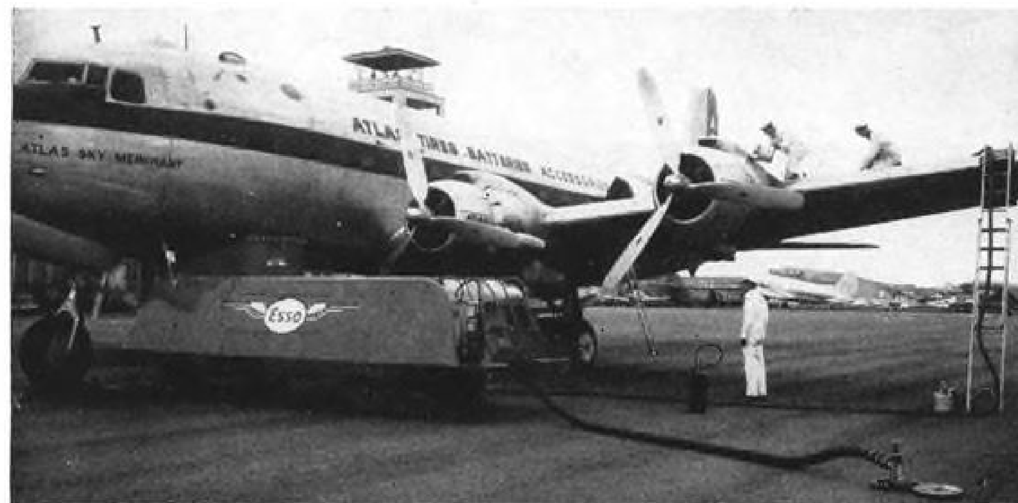
COMPACT servicer in use. Fuel from flush hydrant is delivered through two hoses.
