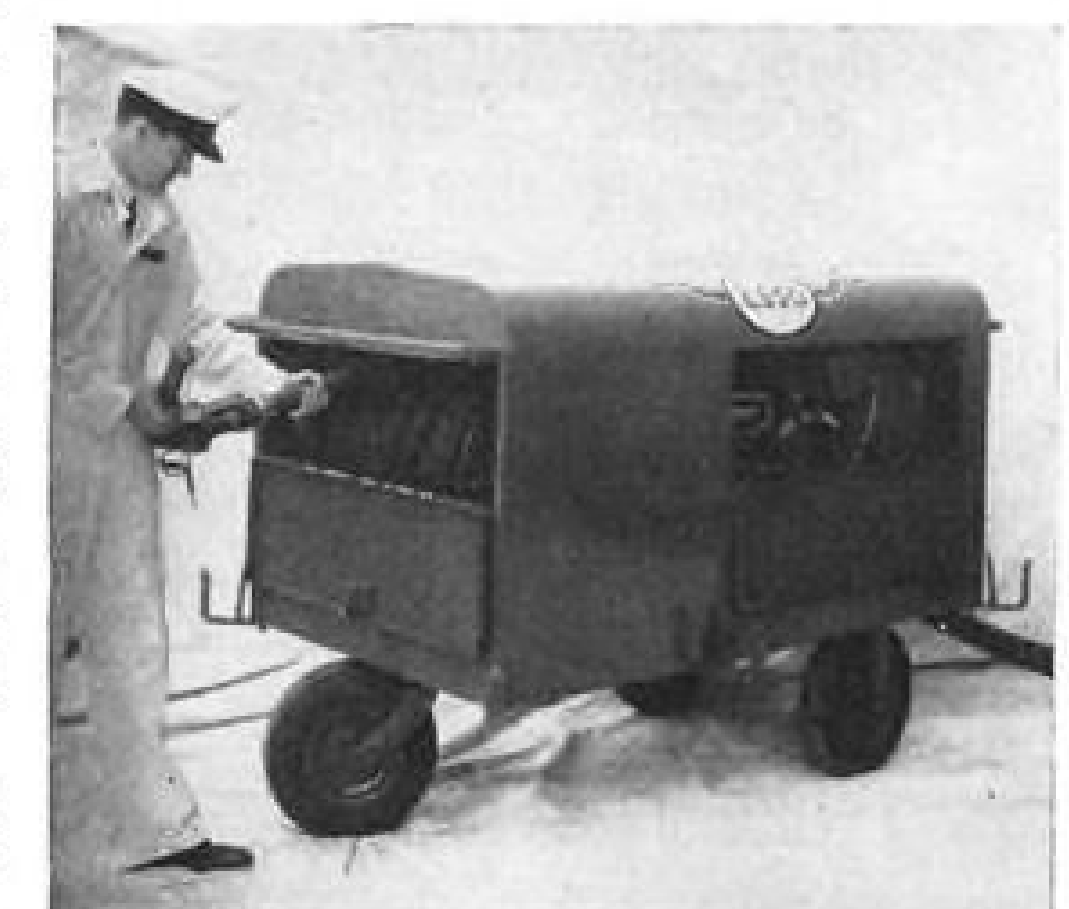
HYDRANT cart can pump 100 gpm.
