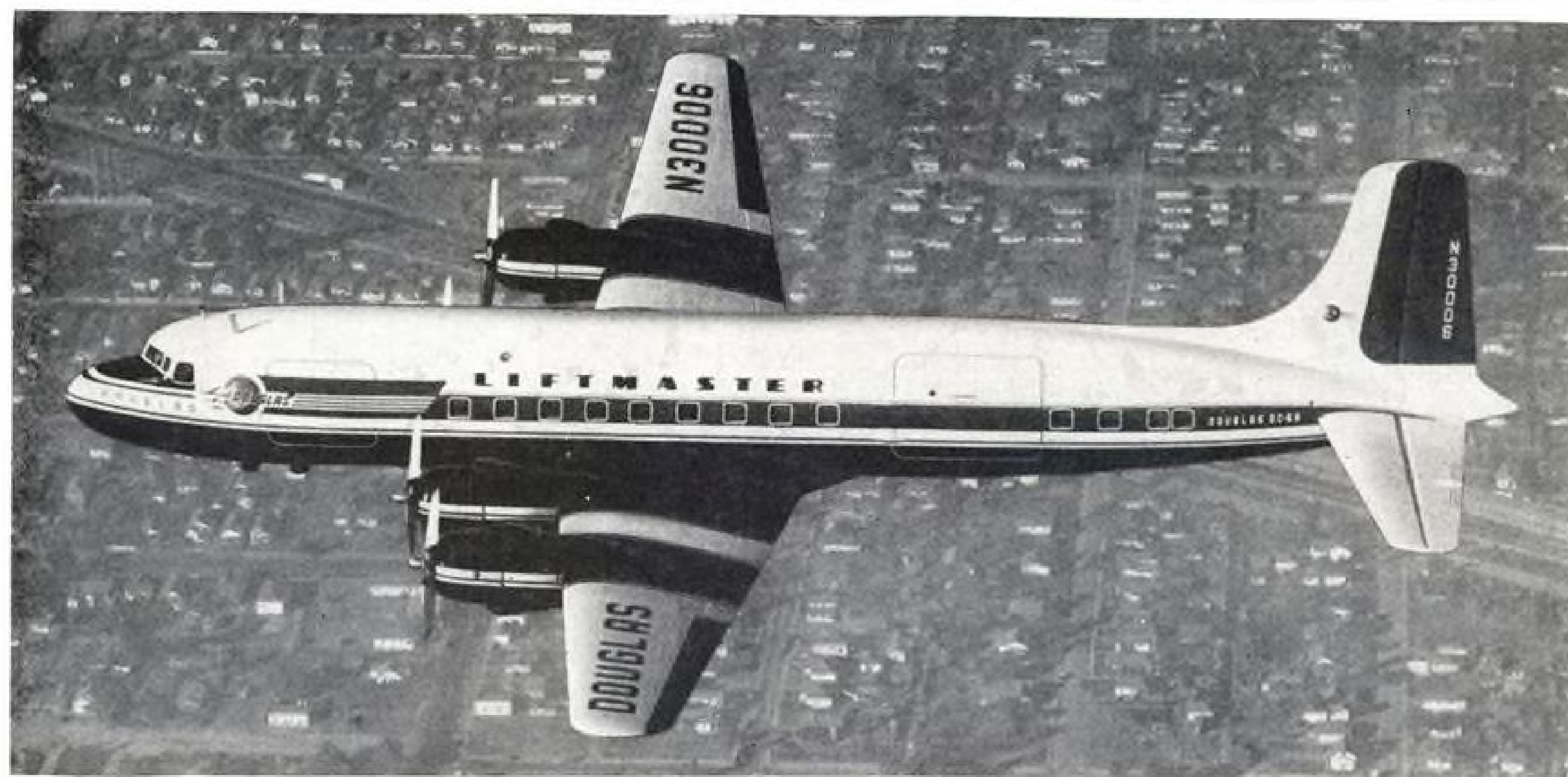
DC-6A illustrated Douglas' ideas on commercial cargo plane design: Proven performance, high speed, very large aft door.
