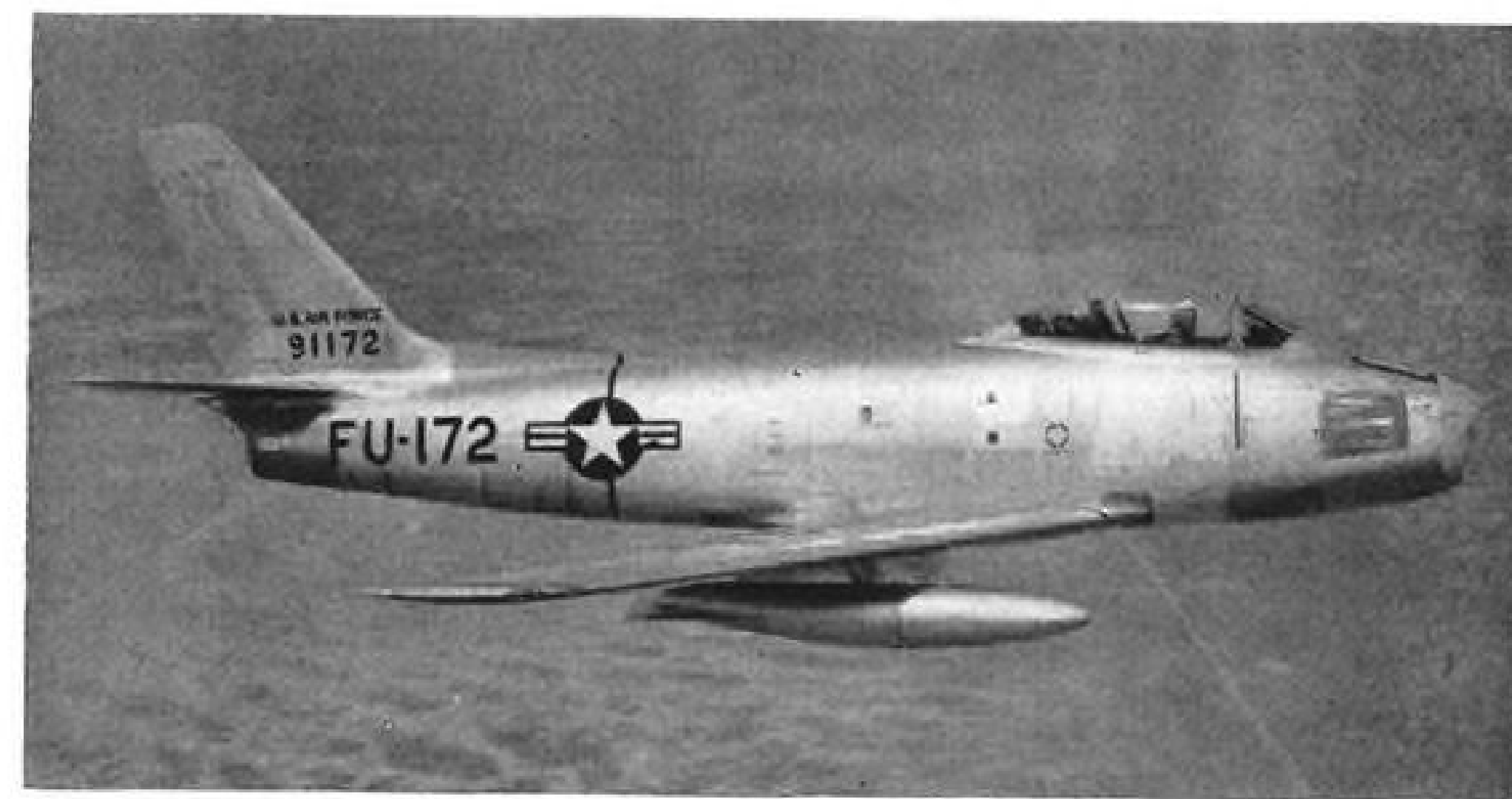
EXTRA TANKAGE is supplied on the F-86 Sabre from two non-droppable "banana" tanks.
