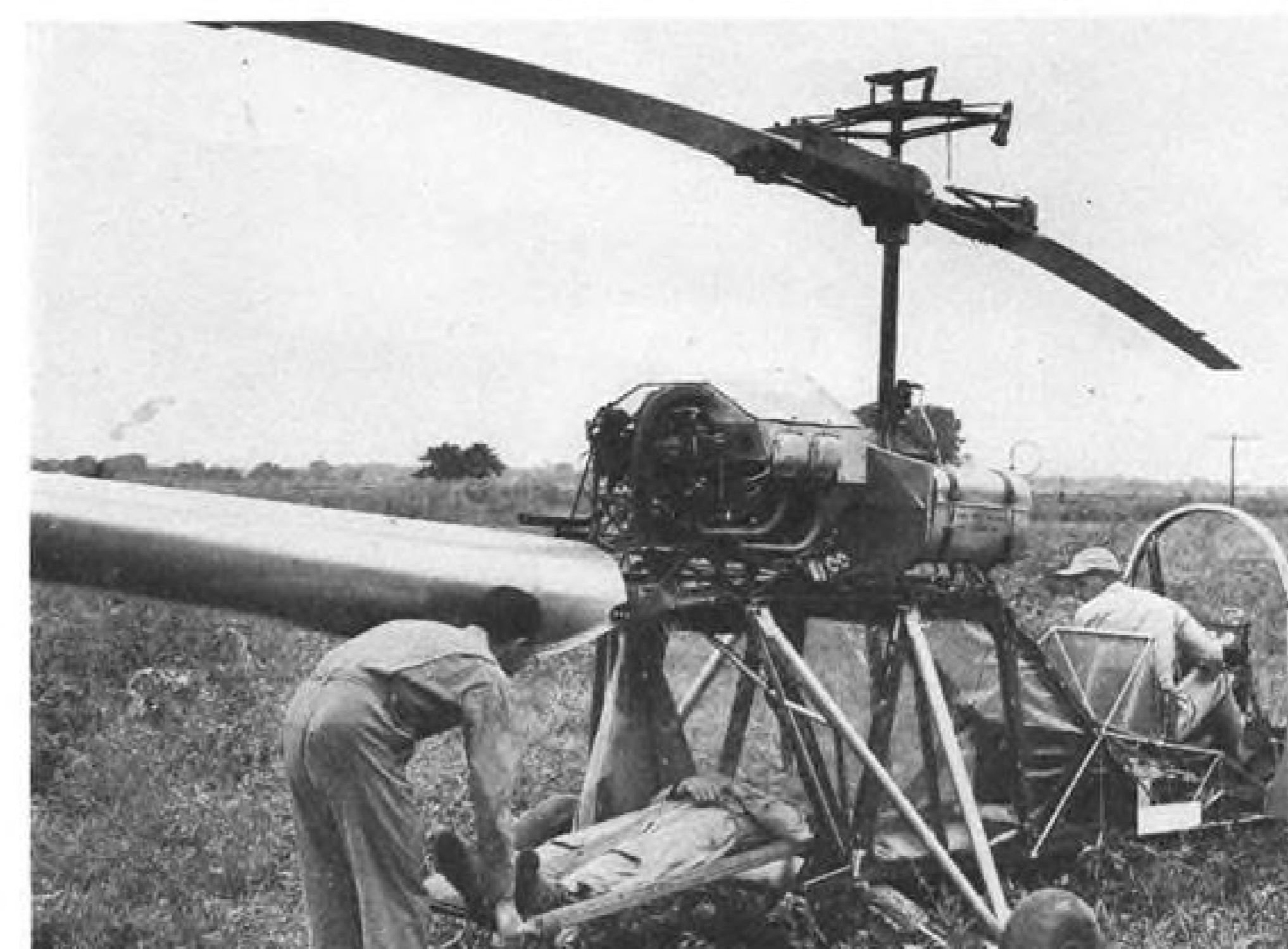
LITTER HANDLING is facilitated by location of the deck close to the ground.
