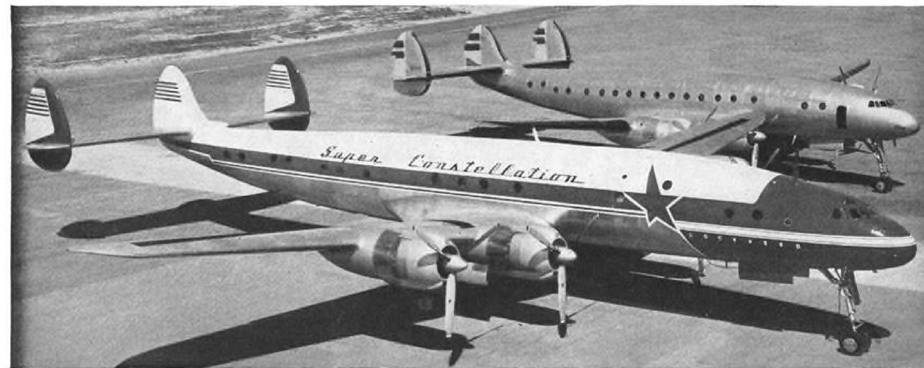
SUPER-CONNIE shows its greater length when parked on the Lockheed ramp beside a conventional Model 749.
