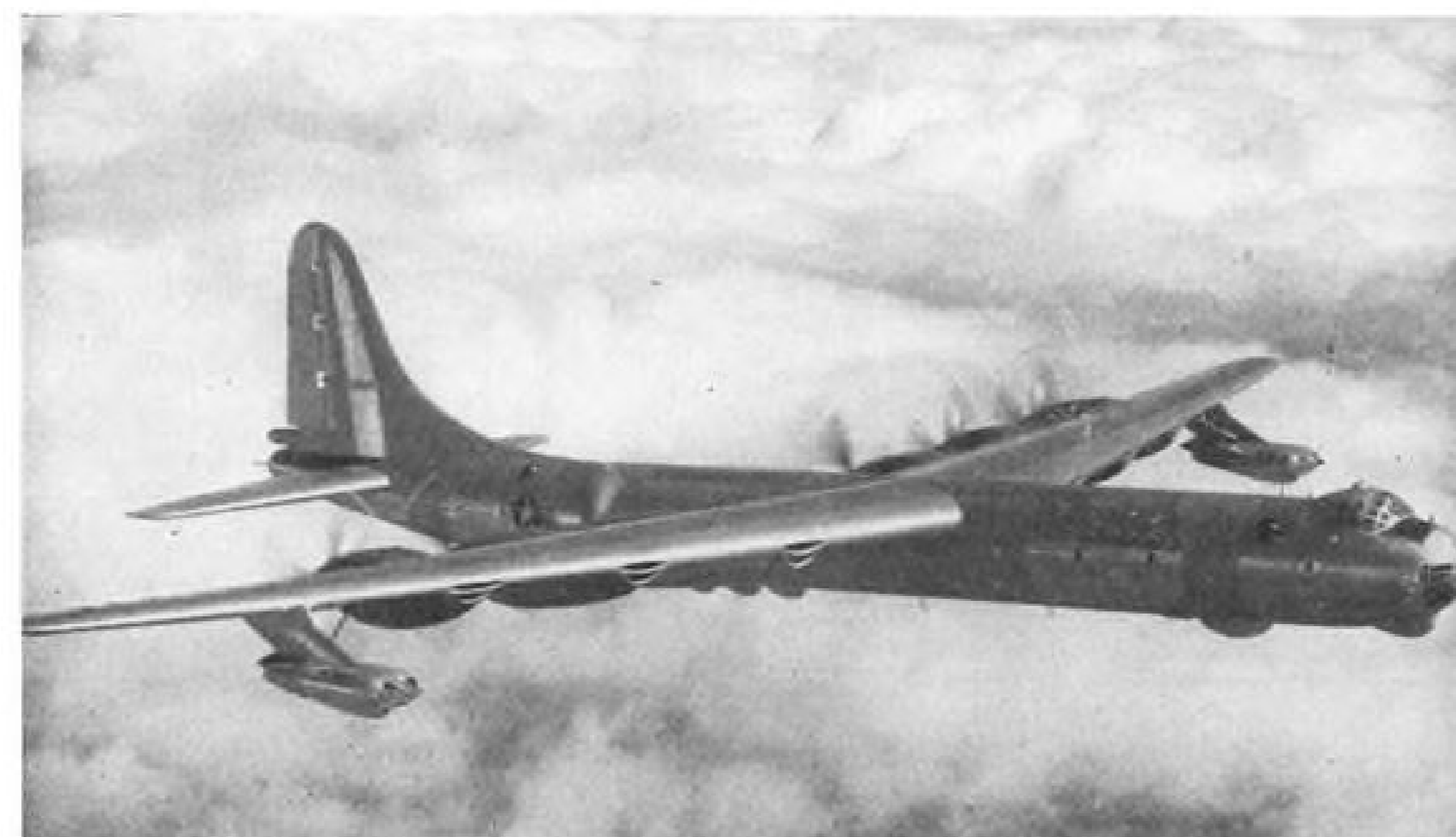
BIG EYES —Newest flight of Convair's RB-36 reconnaissance version of the B-36 bomber shows the variety of special housings along the underside of the fuselage. For photographic purposes, the RB-36 carries 14 cameras in the forward bomb bay, one with a 42-in. focal length lens.
