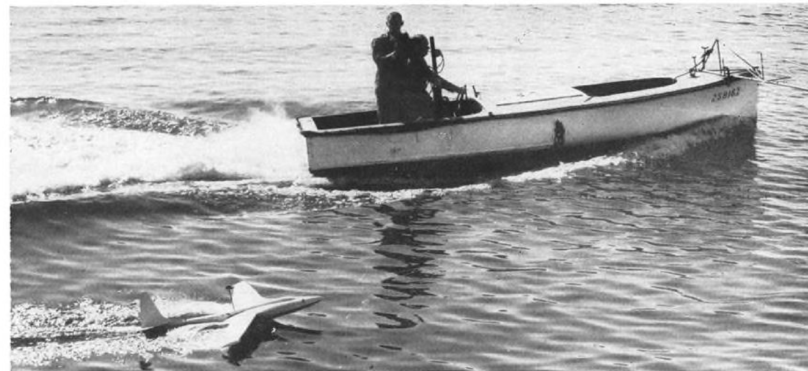
TOWED from bridle extending from power boat, with engineers photographing the model of the plane as it cut through water.
