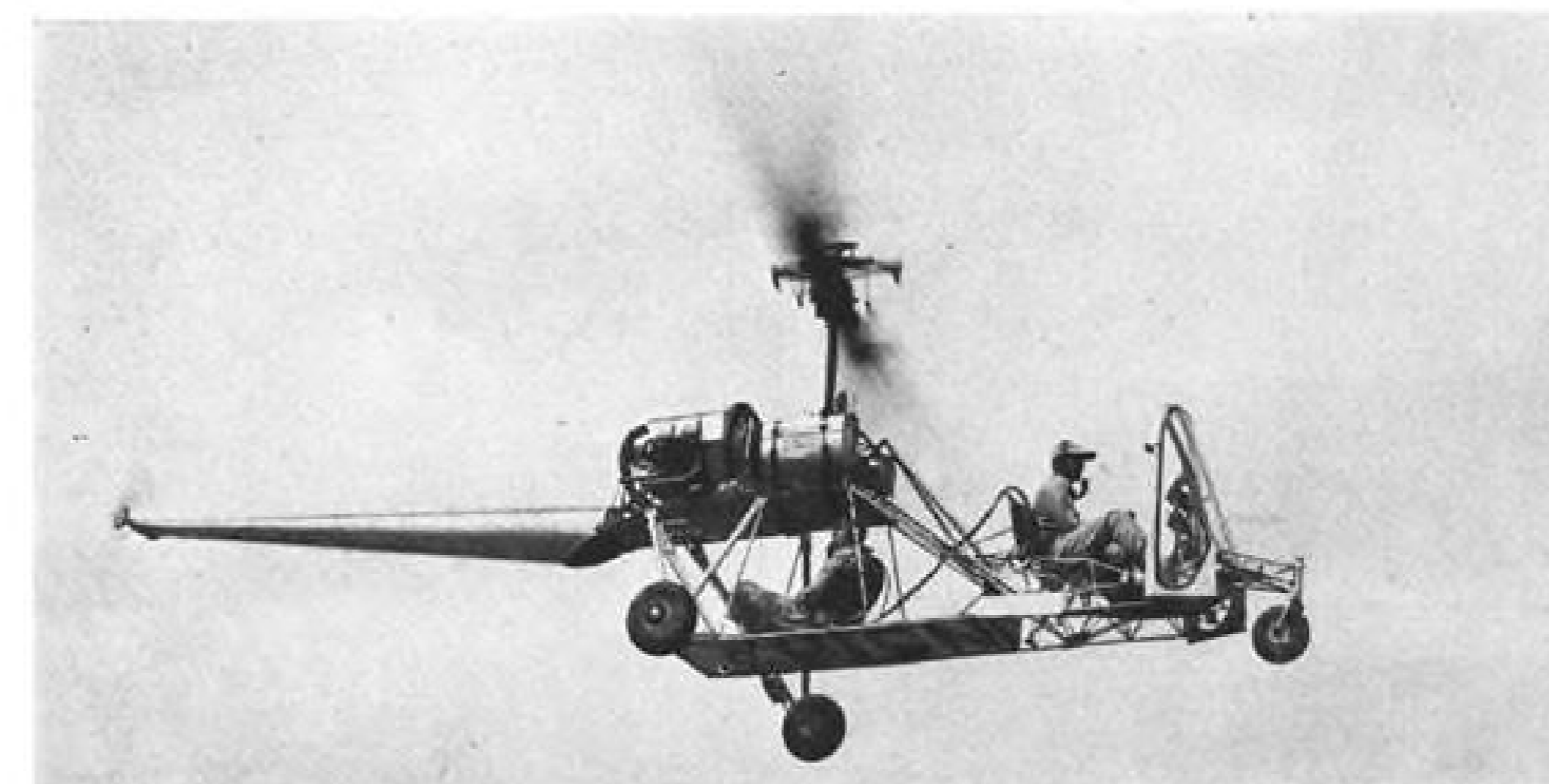
PASSENGER OR CARGO is accommodated on S-4's deck aft of pilot, while . . .
