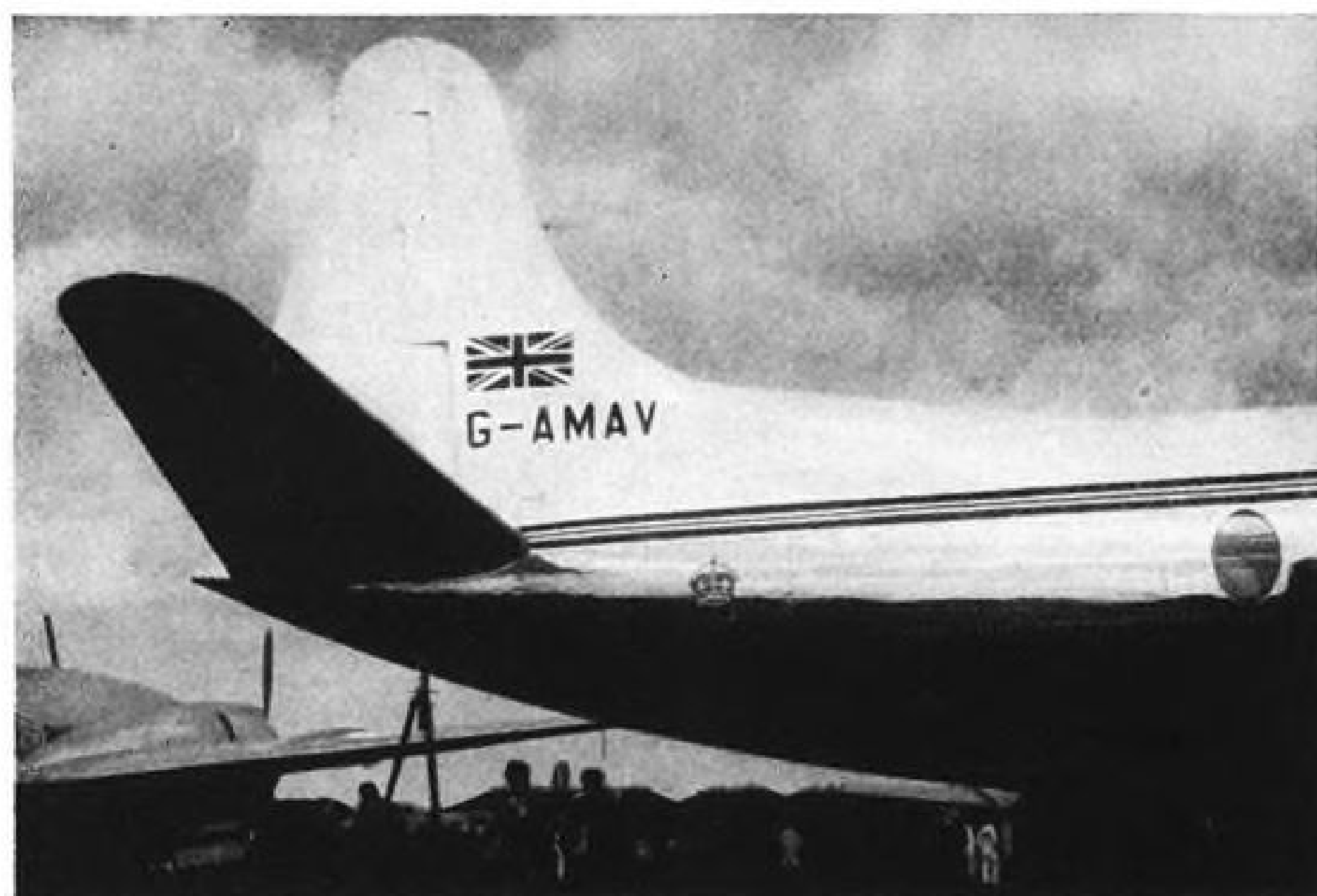
DORSAL FIN and dimensional changes from earlier prototype 630. Power units are...
