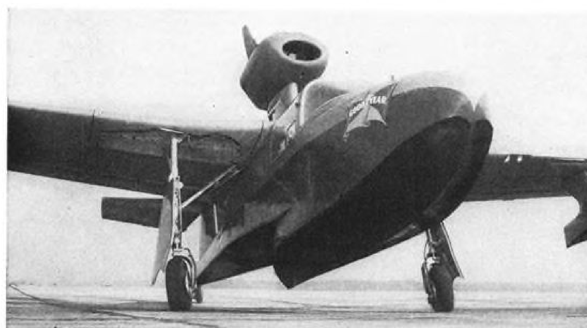
CROSS-WIND LANDING GEAR installation tucks into shoulder-high wing in two folds.
