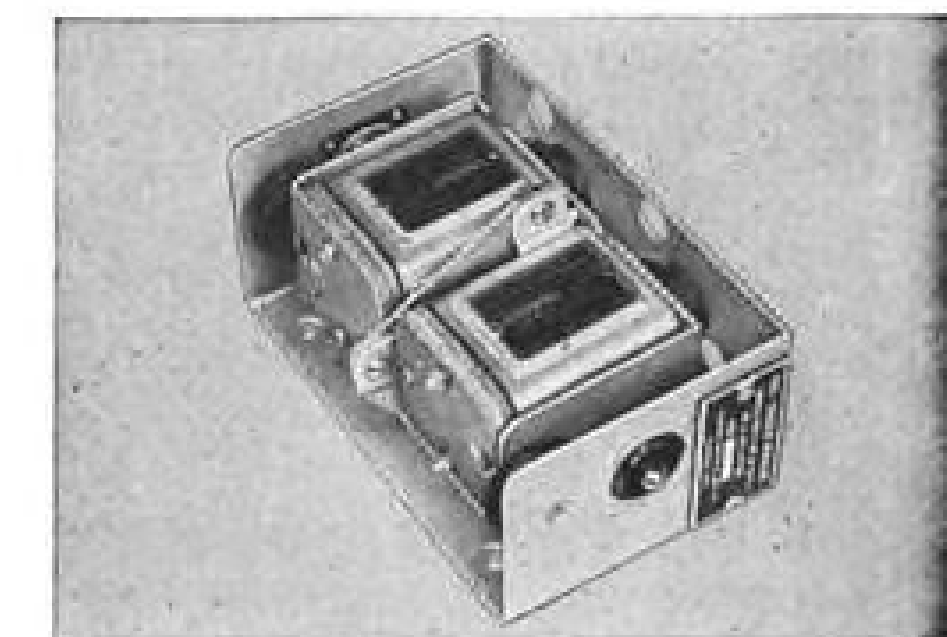
Overvoltage Relay—120 volts DC (USAF Spec. 32652, Type E-3)
