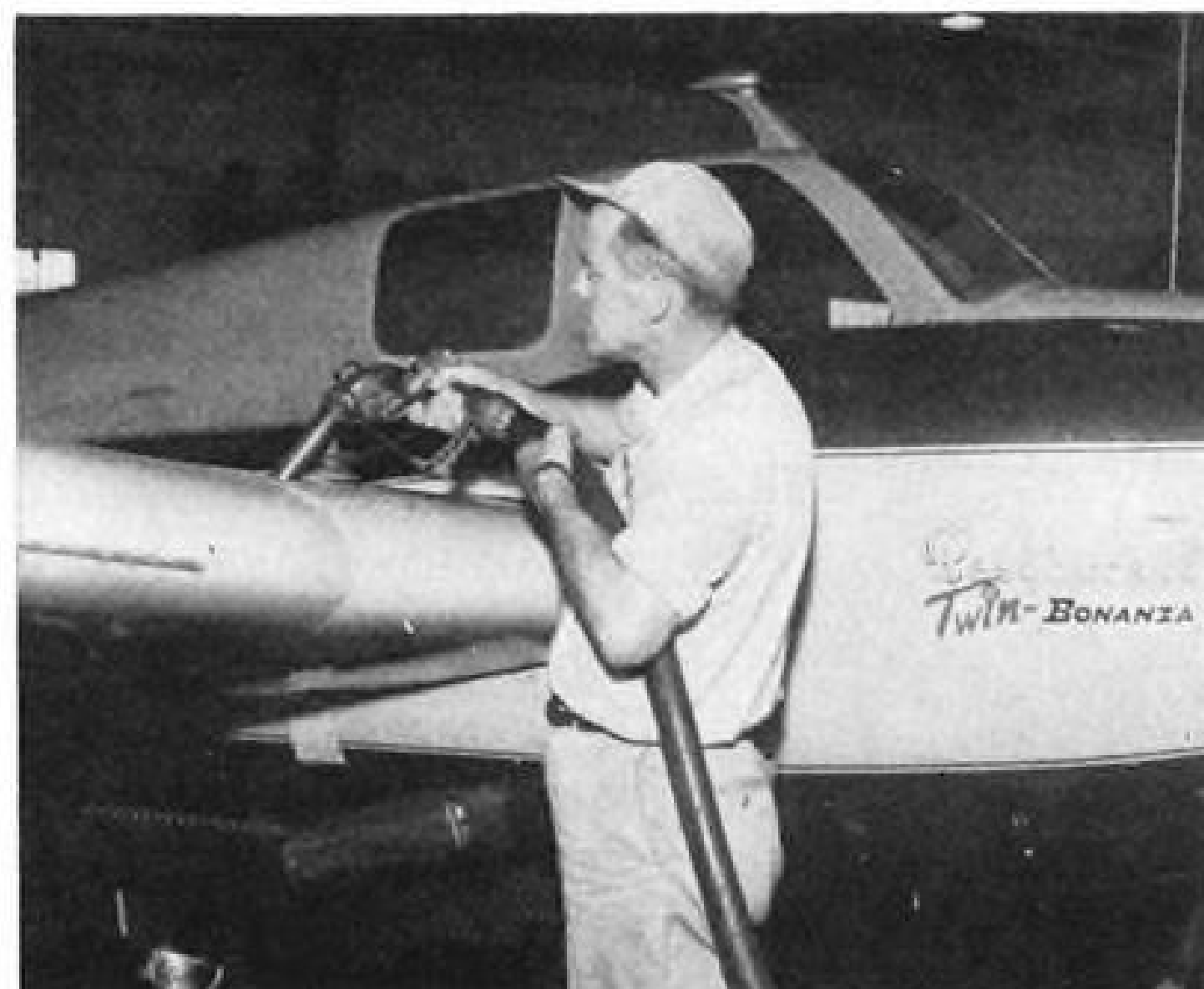
FUELING is easily accomplished through the wing leading edge from ground position or on low stand.
