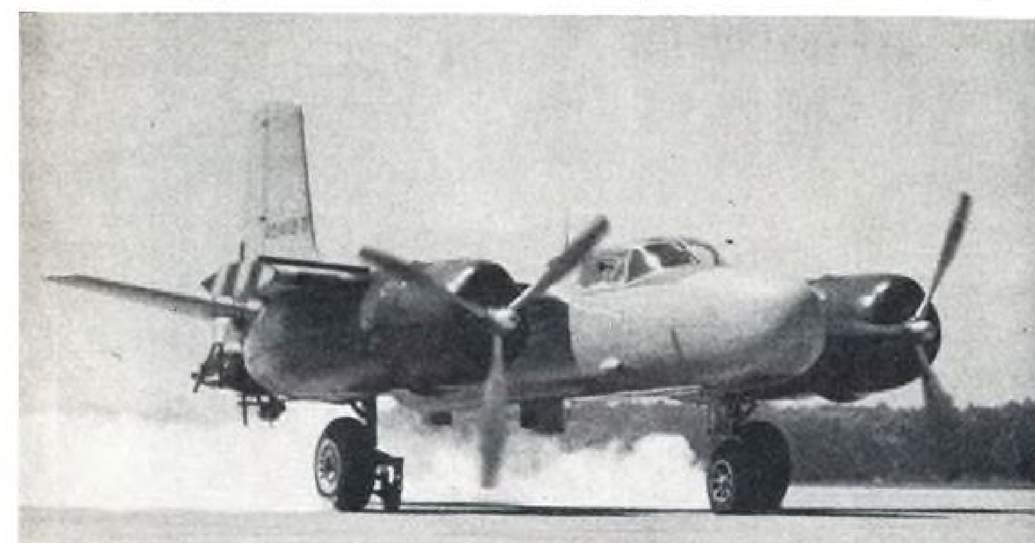
SKID TESTER —USAF Air Materiel Command is using this clipped-wing Douglas B-26 to gain valuable test data needed for design of stronger, lighter, smaller landing gears. In the left view,
