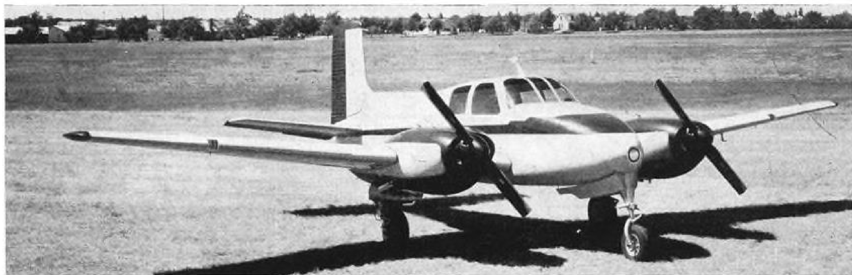
TWIN BONANZA multipurpose craft is designed for easy modification into trainer, photographic plane, ambulance or cargo ship. Outer wing panels have same geometry as Bonanza wing. The roomy cabin will accommodate six.
