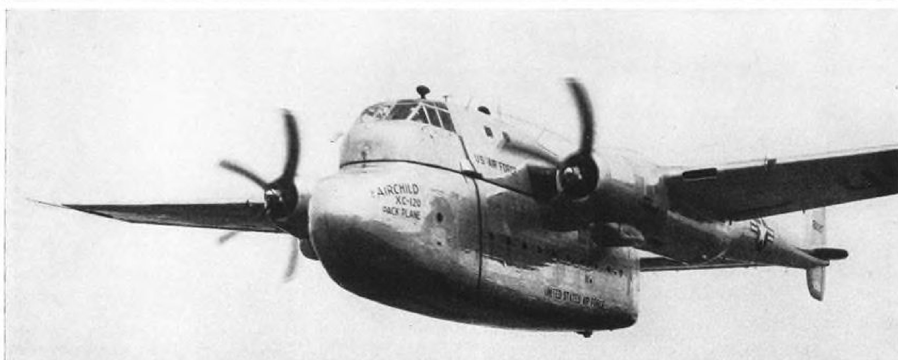
PACK PLANE is Fairchild's high-utility design combining huge detachable fuselage with quick-turn-around carrier. Gap between the two is closed by inflated deicer-boot-type seal. Craft is logical progression of C-82 and C-119B.
