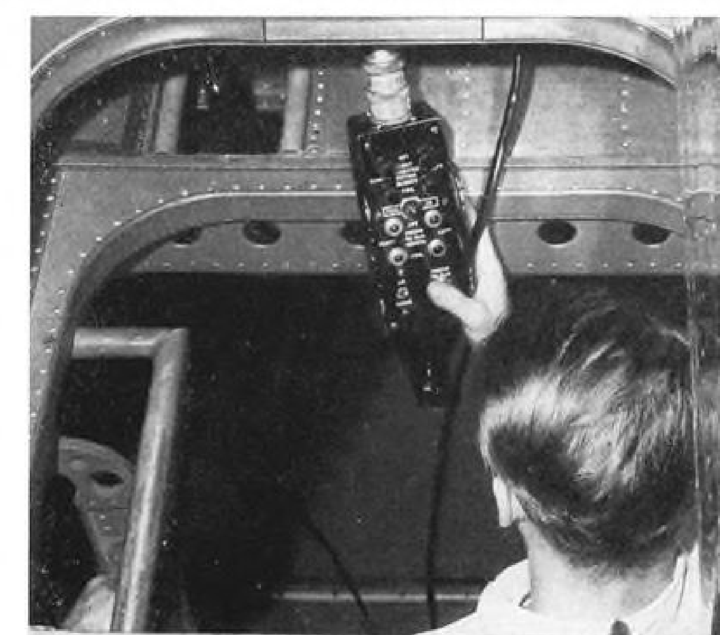
CLOSURE is controlled by main-switch operator standing in pack as he watches nacelle-pack alignment.
