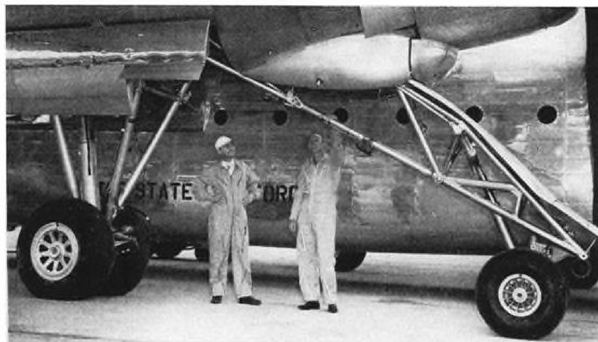
LANDING GEAR is quadricycle type, with 15-ft. 7-in. wheelbase. Main and auxiliary units are retracted aft simultaneously.
