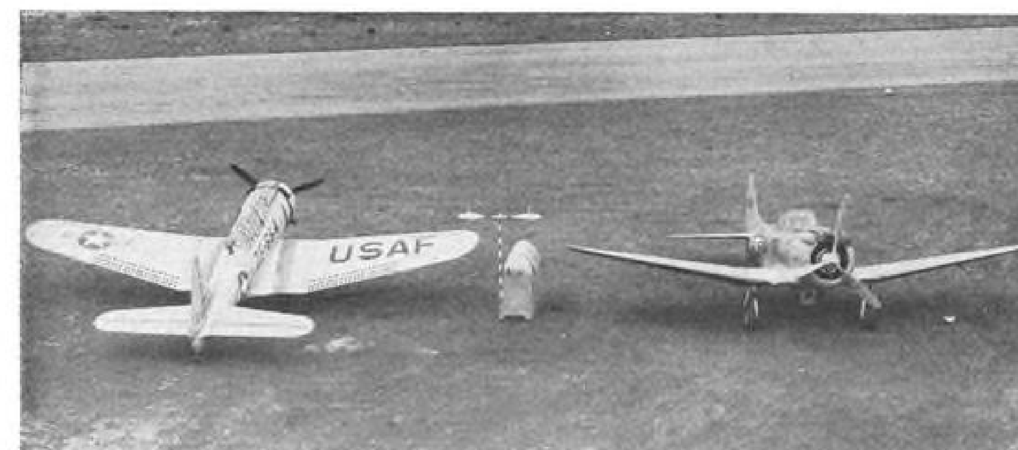
MOTHER & DRONE A-24s. Note horizon video camera under belly of drone (right). Test ground control unit is between planes. Right photo: drone control cockpit in mother ship. Upper television screens in pilot's line of sight monitor main video receivers (lower pair).
