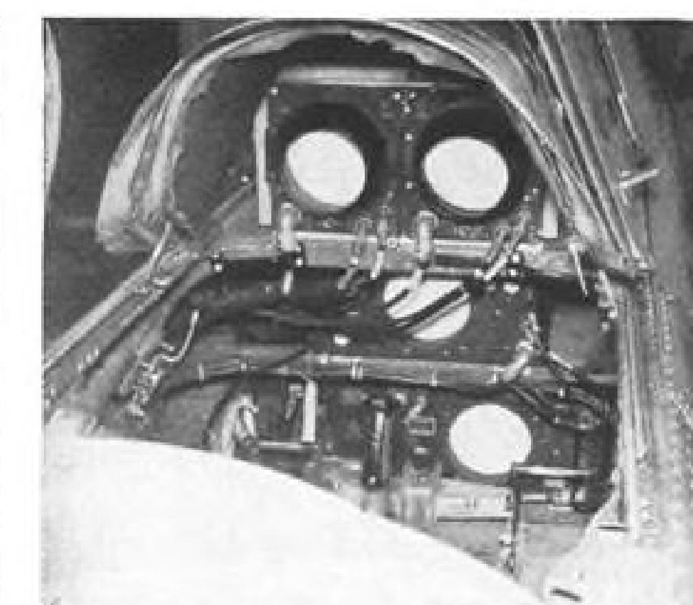
MOTHER & DRONE A-24s. Note horizon video camera under belly of drone (right). Test ground control unit is between planes. Right photo: drone control cockpit in mother ship. Upper television screens in pilot's line of sight monitor main video receivers (lower pair).
