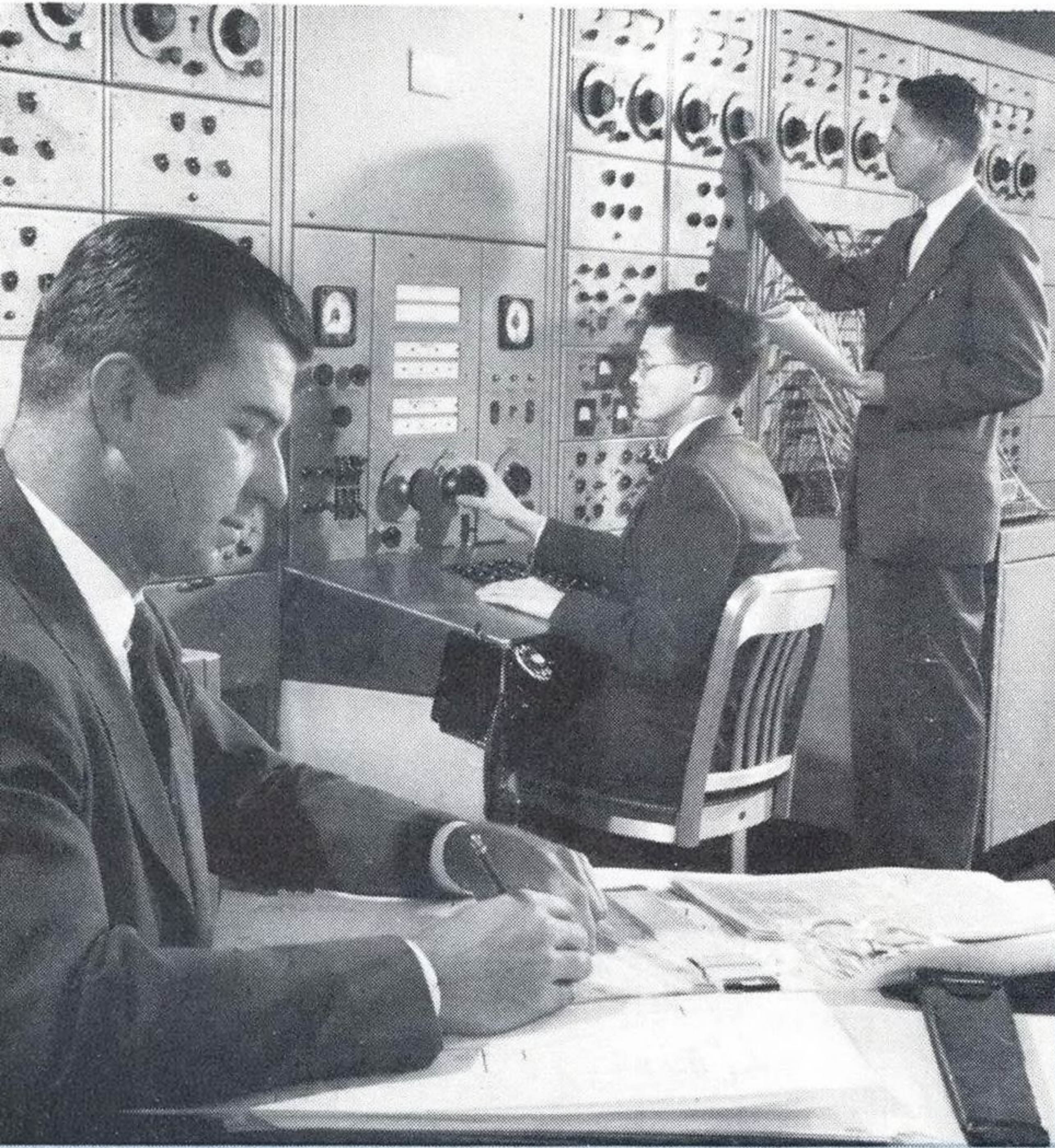
Complete electrical systems for any given aircraft can be simulated on this network analyzer.
