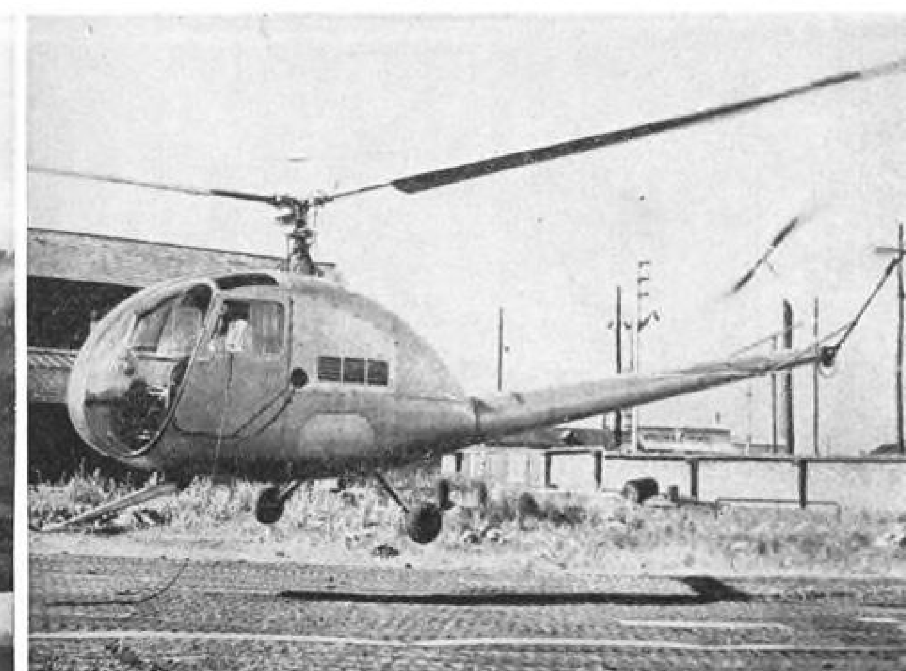
FRENCH COPTER —Sud-Est SE 3110 two seater has 203-hp. Salmson, butterfly tail rotors.
