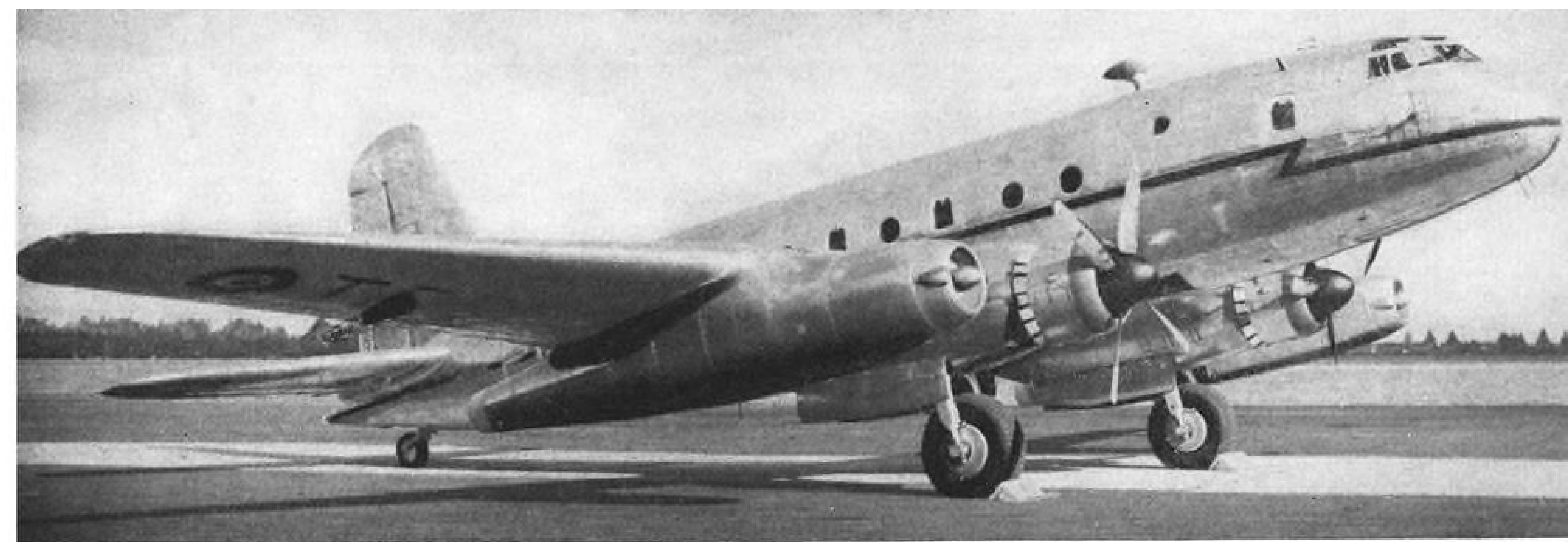
TRANSPORTING SAPPHIRES —Neatly fitted 7200-lb.-thrust Armstrong Siddeley Sapphire turbojets replace outboard Bristol piston engines on this four-engine Handley Page Hastings transport. On half the jet's power, plane reached 1000 ft. in 30 sec.
