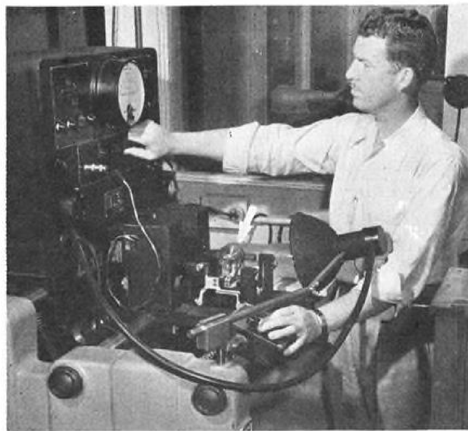
DYNAMIC BALANCING of air bearing gyro components is carried out in the dust-free rooms of North American's precision machine shop.
