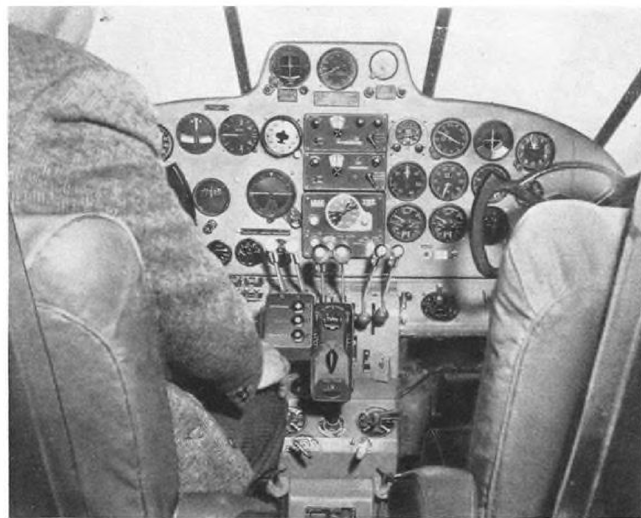
THREE BUTTON automatic approach coupler control box is visible just above the pilot's right hand. Directly to the right is the F-5 autopilot controller. Units are in Lear's Beech 18.
