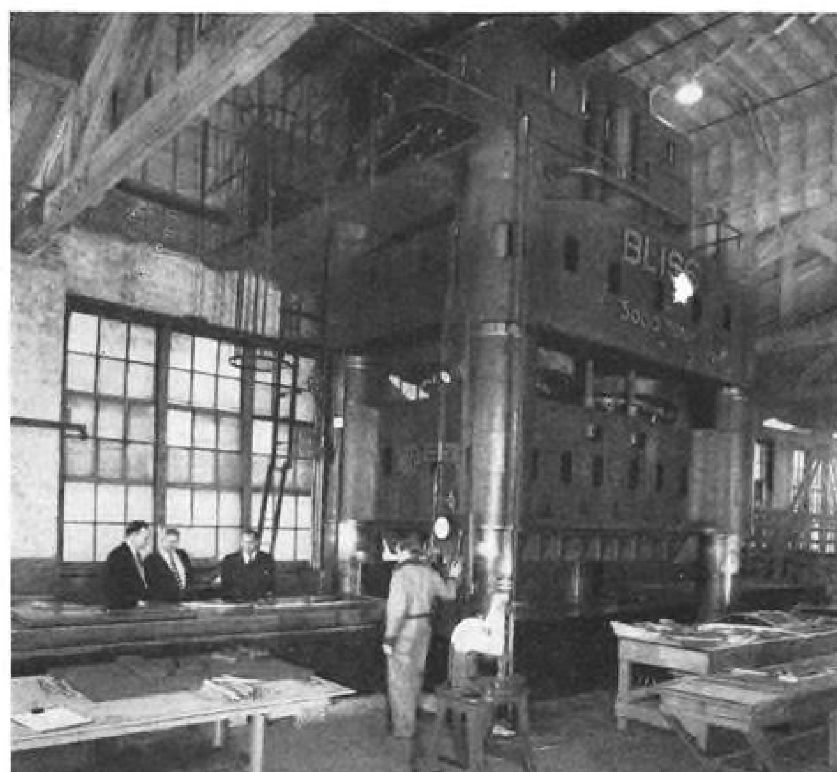
$410,000 was spent by Sikorsky for this 5000-ton Bliss hydraulic press. Considered a giant even then, this machine is dwarfed by this new . . .
