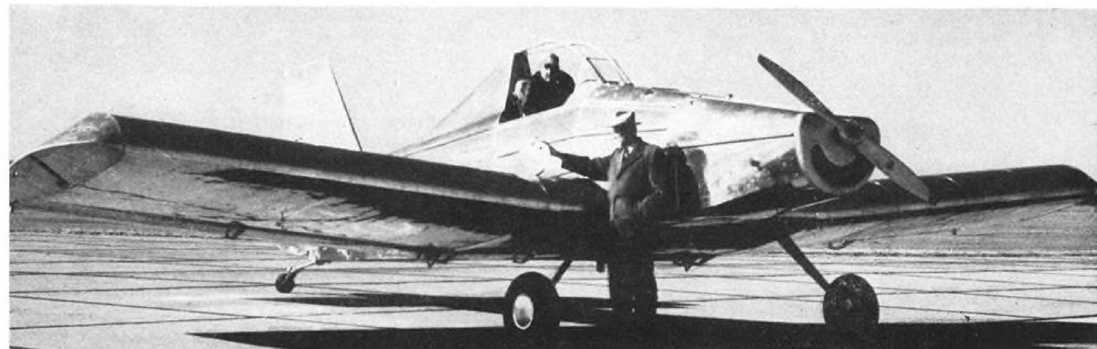
NEW FLYING FARMER —Texas A&M's designed-for-the-purpose agricultural plane is examined by designer Fred Weick prior to first flight (see also page 32). The 200-hp. Lycoming-powered plane features excellent visibility and spray tank storage within thick wings.
