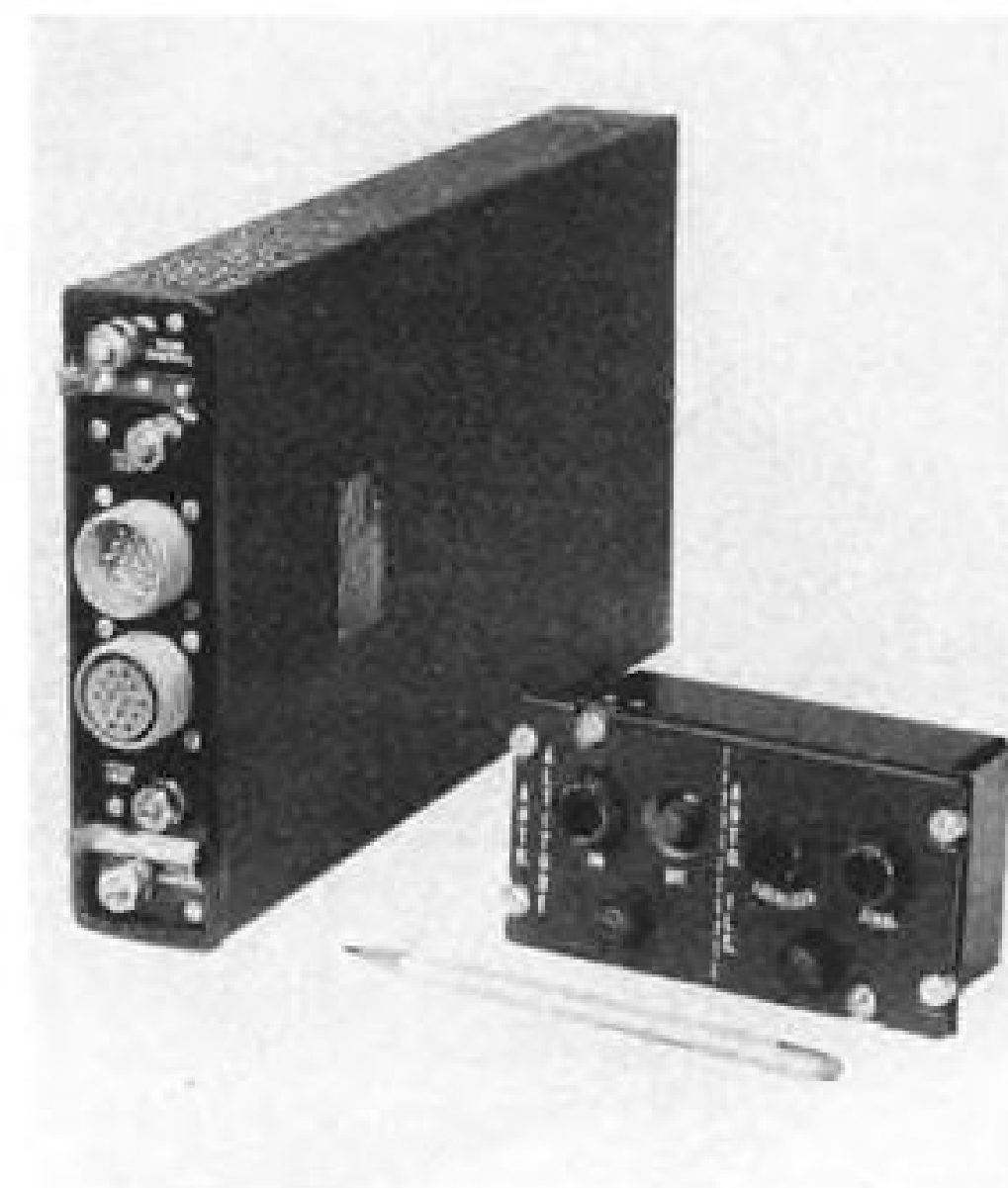
COMPACT APPROACH COUPLER is at the left—note thinness. Pilot's control box at right.
