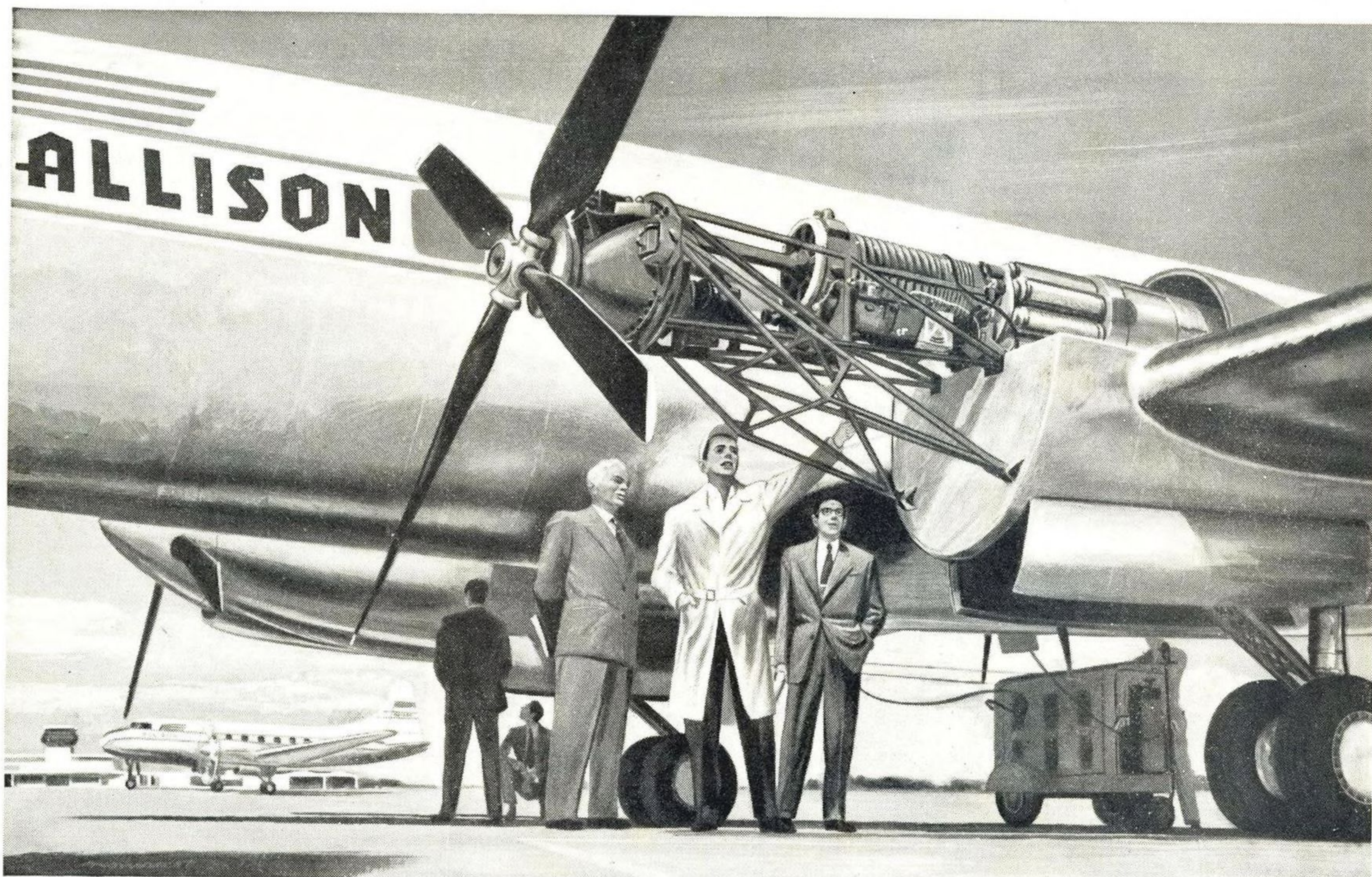
Allison "501" Turbo-Prop engines fit in nacelles of present commercial transports.
