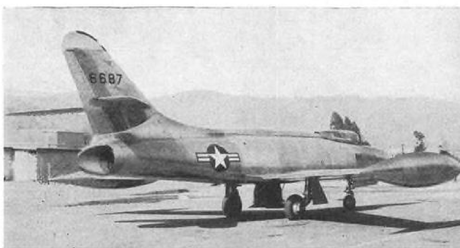
VERTICAL TAIL towers high, mounts swept stabilizer in controllable assembly. Nose detail shows radio bay, gun blast doors.
