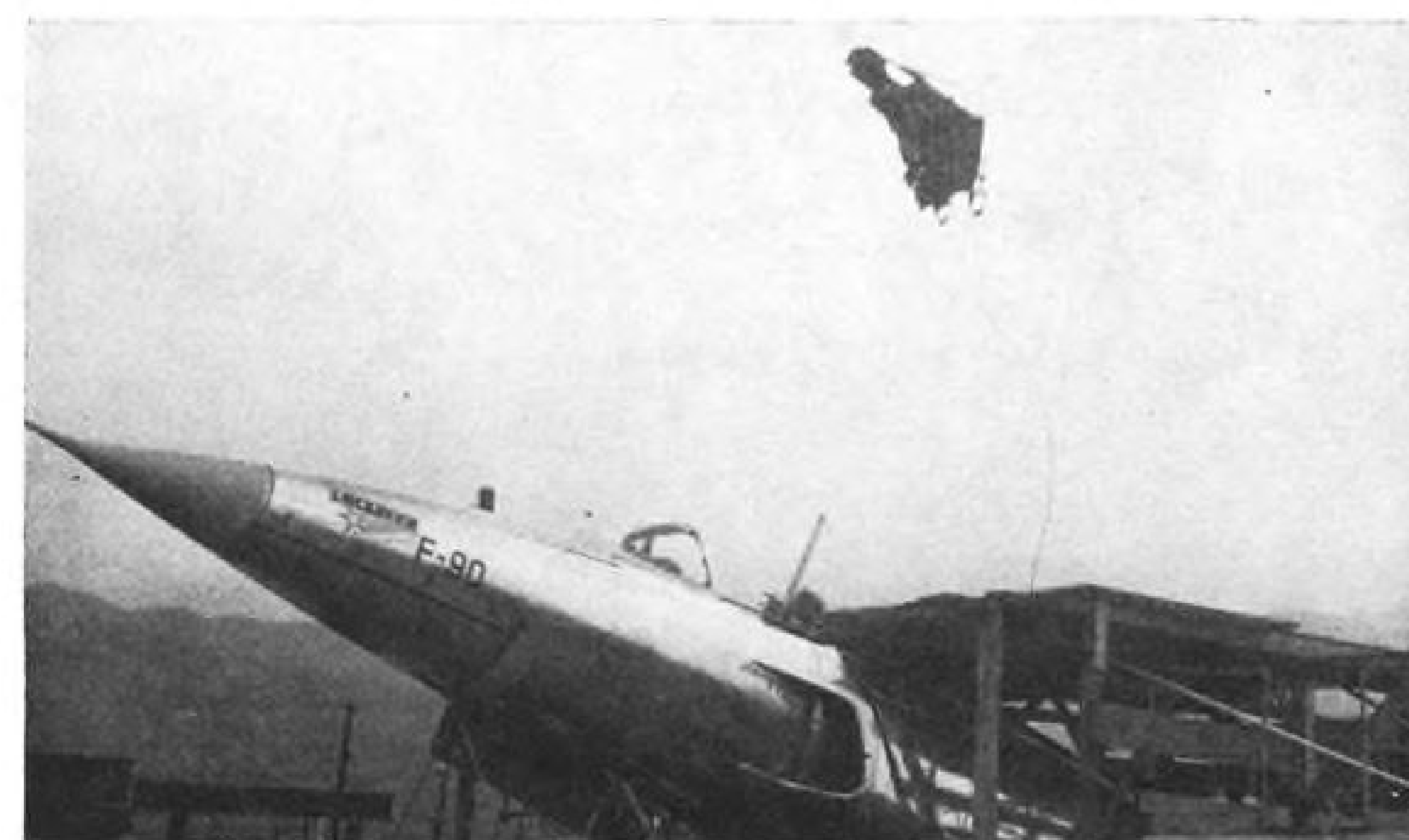
AIRBORNE SEAT takes off from ejection mechanism incorporated in cockpit design.
