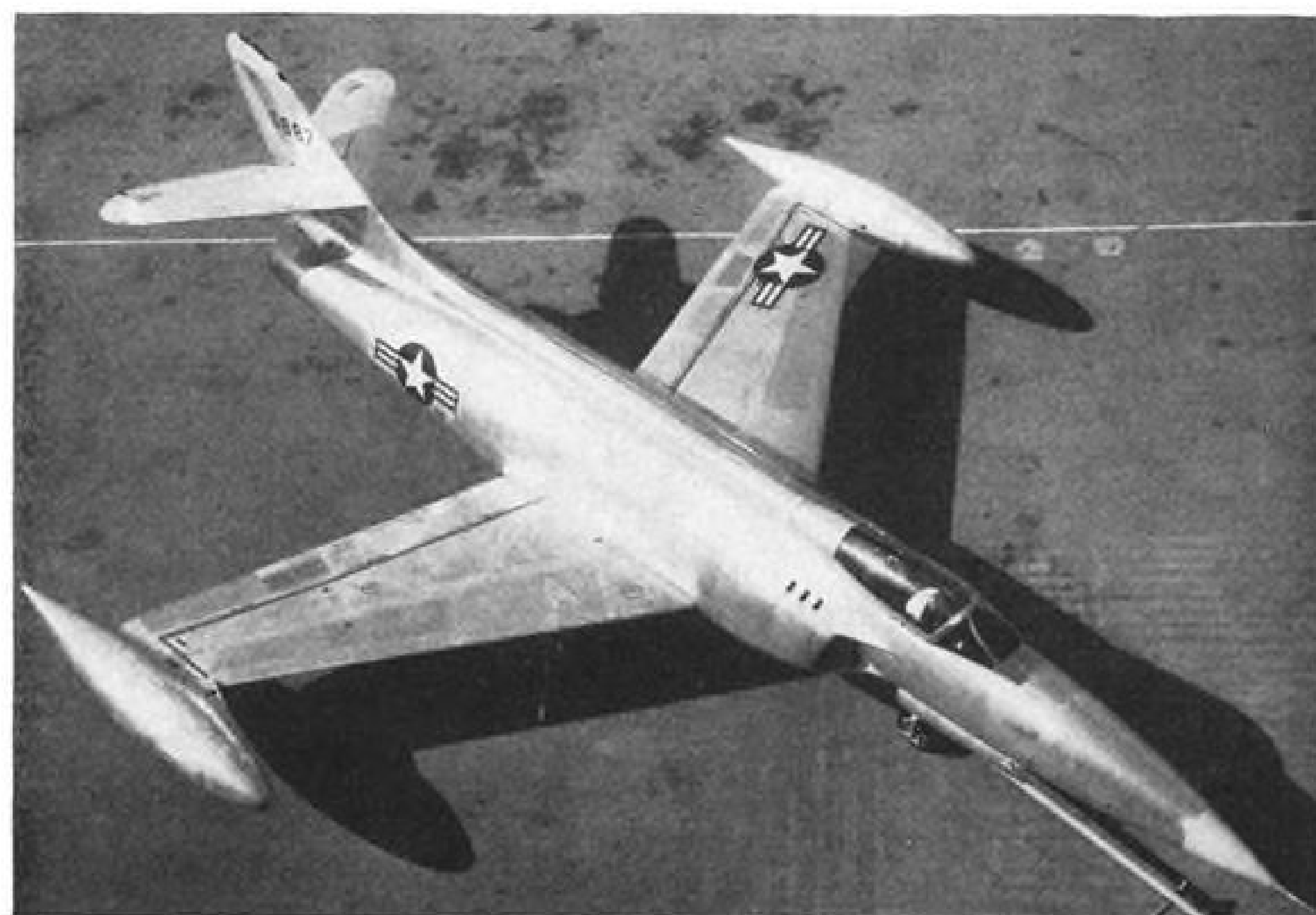
LOCKHEED F-90 in ground view shows needle-nose and aft position of swept wing.
