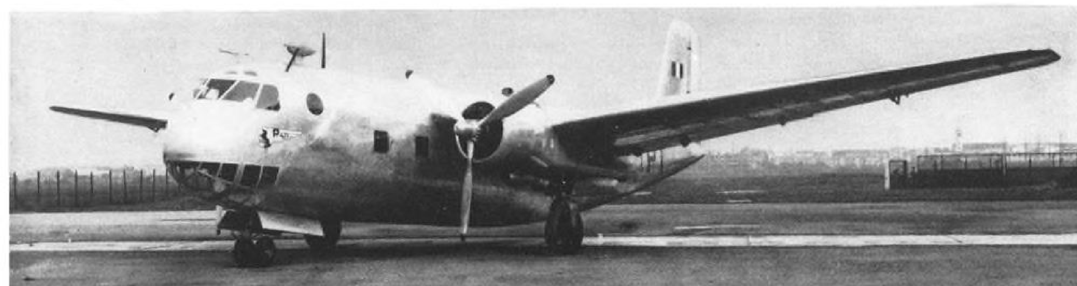
NEW BREDA TRANSPORT—Breda 471 (below) is a new 18-passenger transport being flight tested in Italy. Top speed of 286 mph. is planned with two P&W R-1830 engines of 1200 hp. each. Wing center section is of inverted gull configuration.
