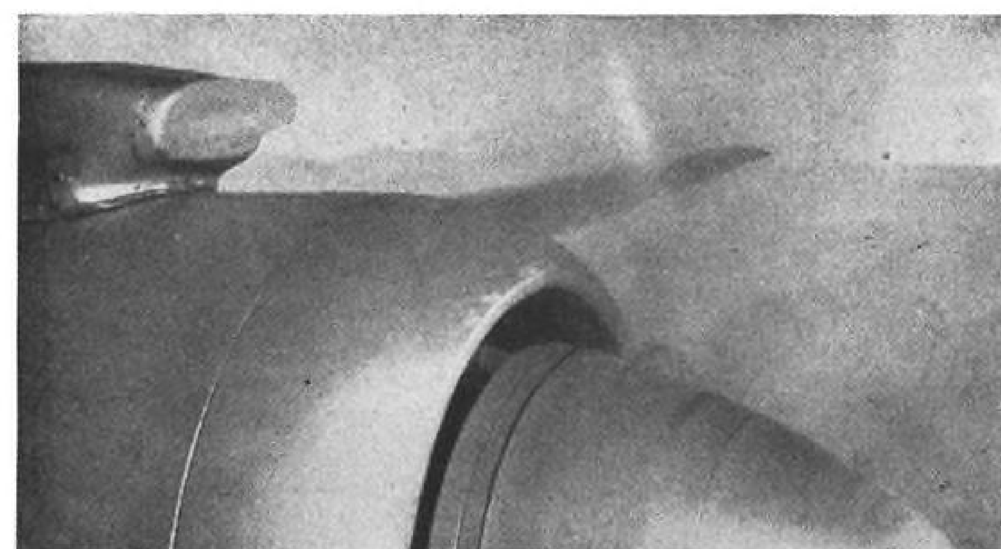
INTERESTING ice accretion completely blocking the carburetor air intake scoop which occurred during one of the test flights conducted to test the efficiency of Porosint units.
