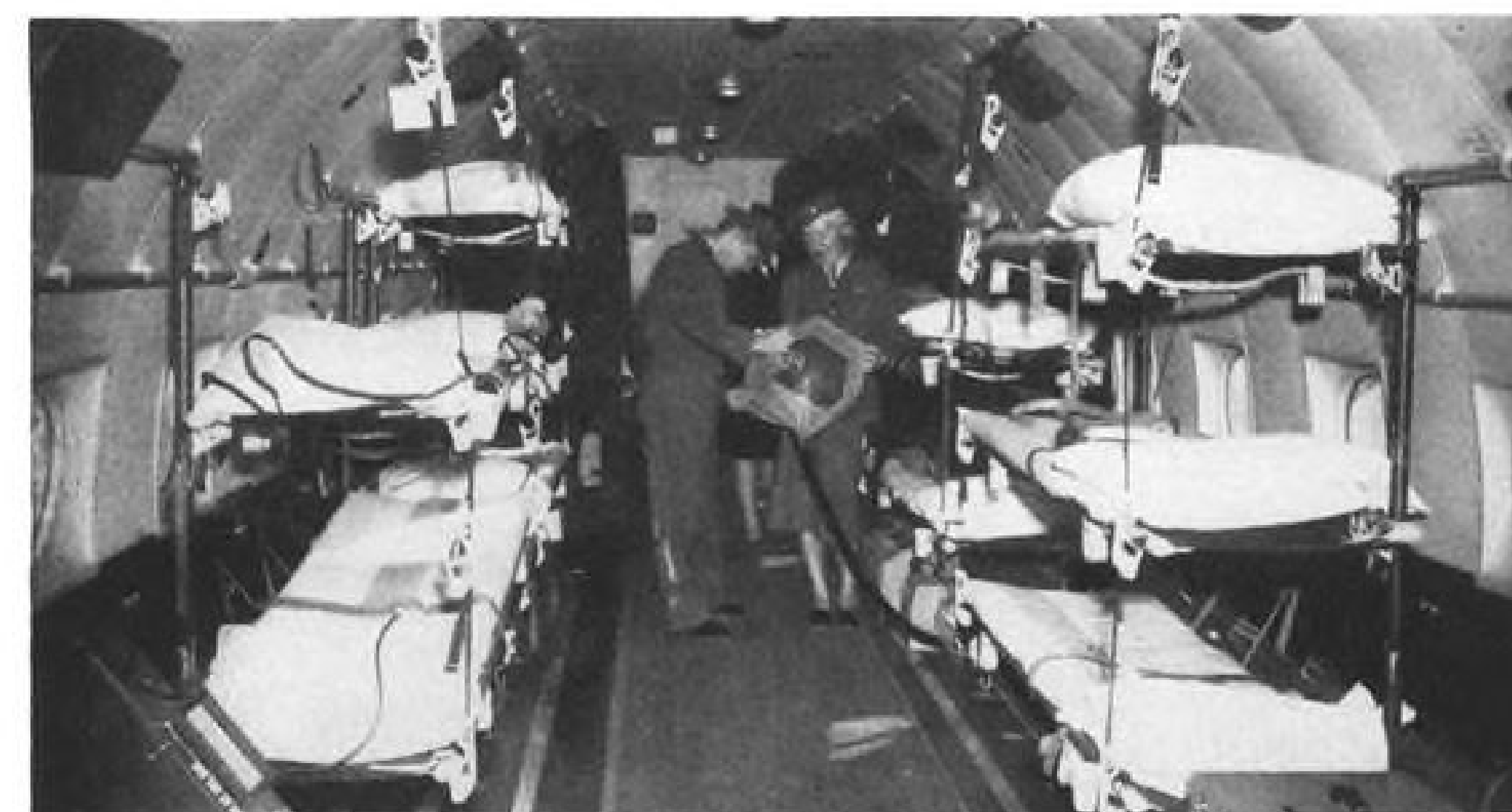
"AIR EVAC" C-54M can be converted from cargo plane to carry 32 patients in comfort.
