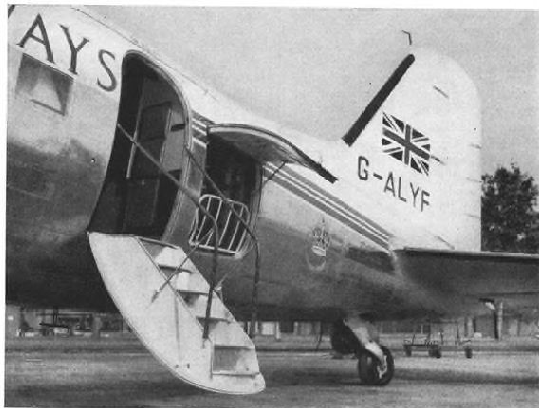
EASIER LOADING is provided by drop-down steps and up-swinging cargo door, and . . .
