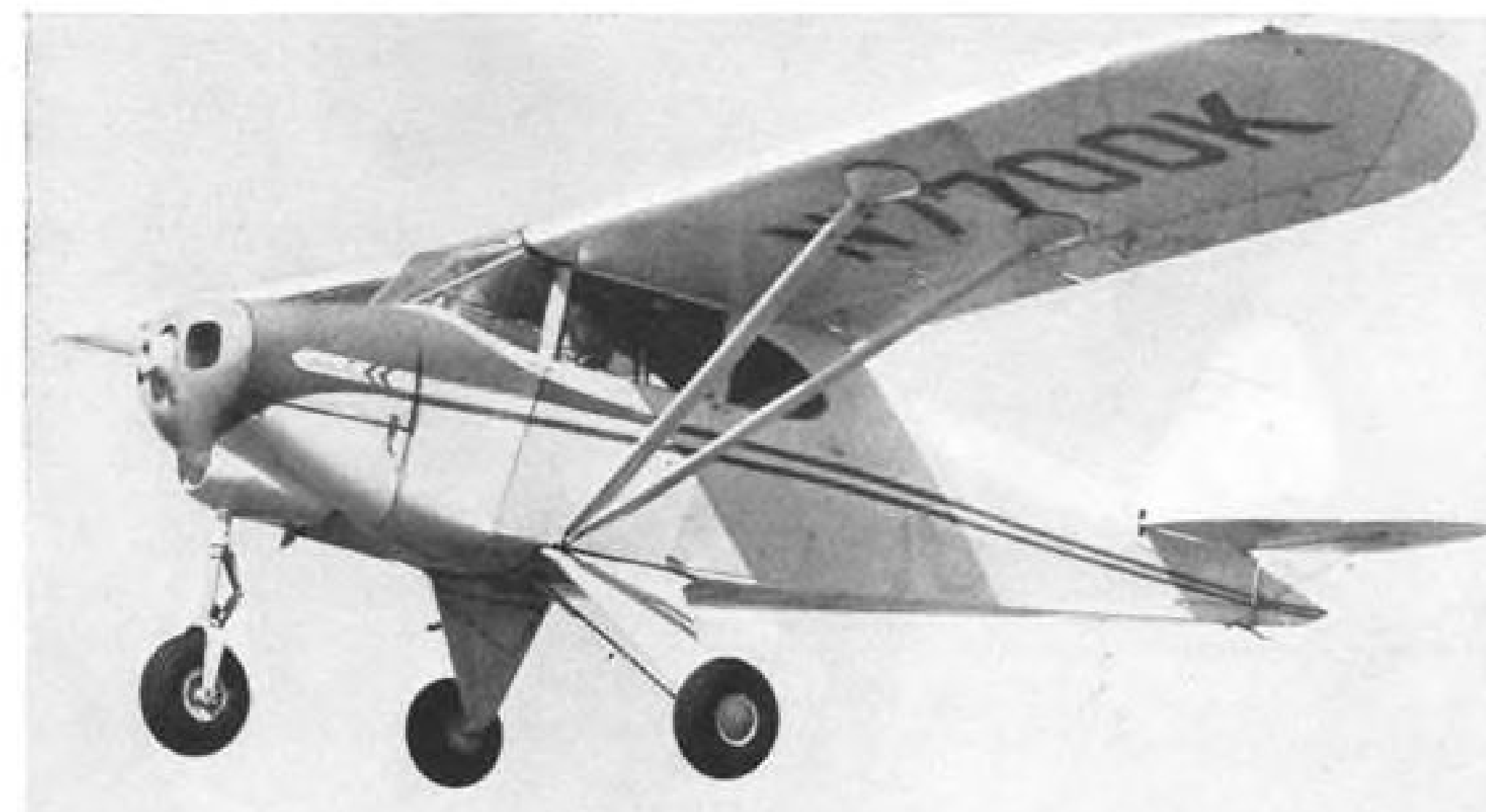
PIPER TRI-PACER shows off its new tricycle landing gear. All wheels are the same size.
