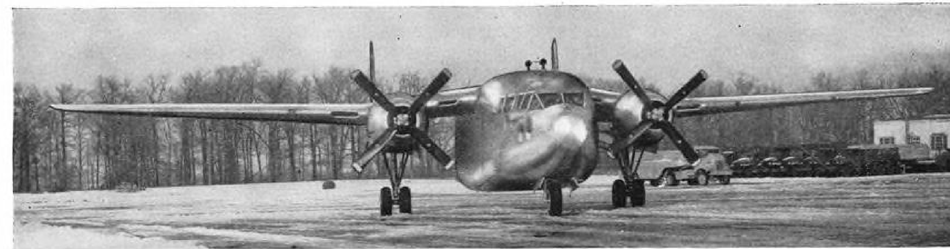
AEROPRODUCTS PROPELLERS, such as will be used on the new version of the Packet, are being tested on a C-119B furnished by AF.
