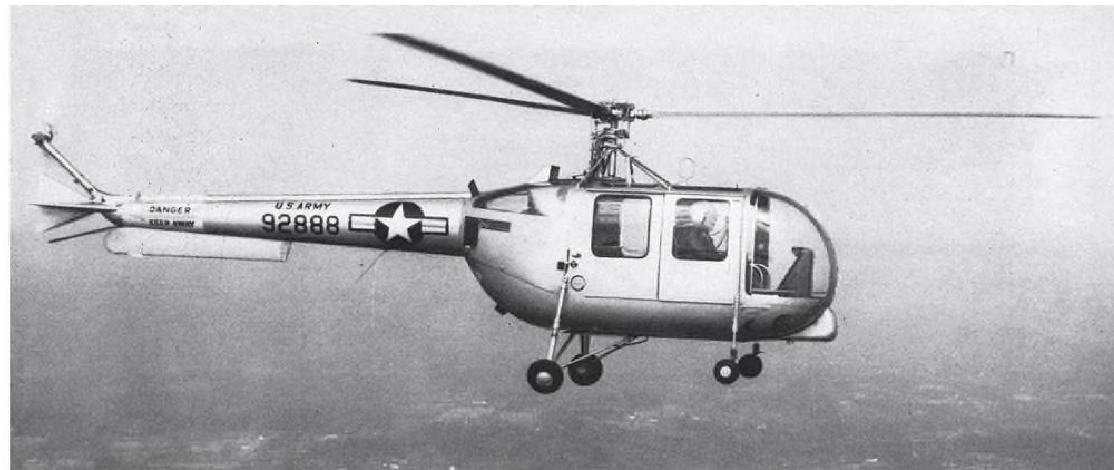
ANOTHER SIKORSKY CERTIFIED—CAA has granted Sikorsky its third commercial helicopter type certificate, this one for the S-52-2, military version of which (YH-18) is shown in this flight view. The 3-4 placer has a 245-hp. Franklin. Note new tail fins, landing gear.
