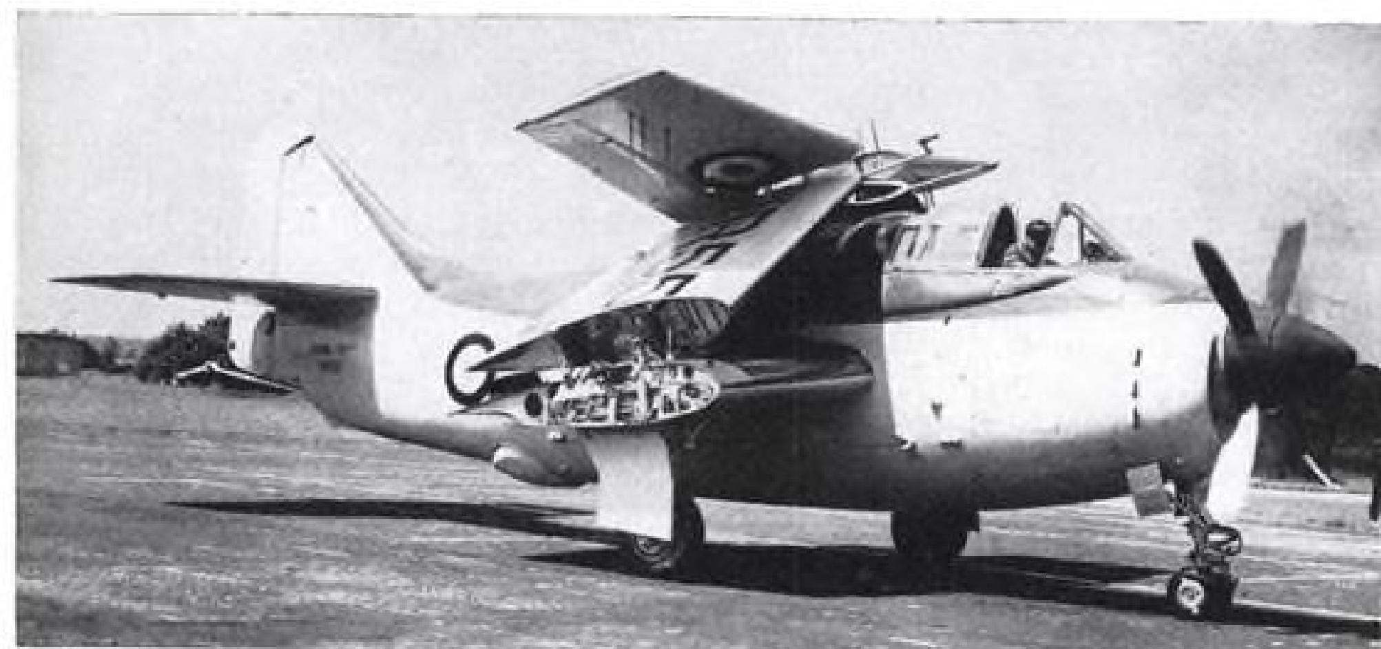
DOUBLE-FOLDED wings make Fairey 17 a small package for easy carrier handling.
