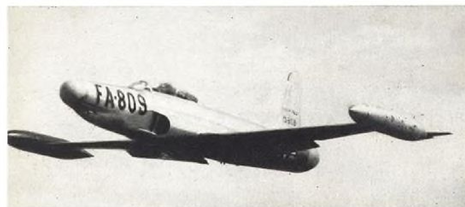
ALL-WEATHER PUNCH — Two-place Lockheed F-94B all-weather interceptor (above) sports new increased capacity wing-tip fuel tanks. Now in production, along with the F-94C (P&W J-48), the Allison J-33-powered B totes elaborate radar.
