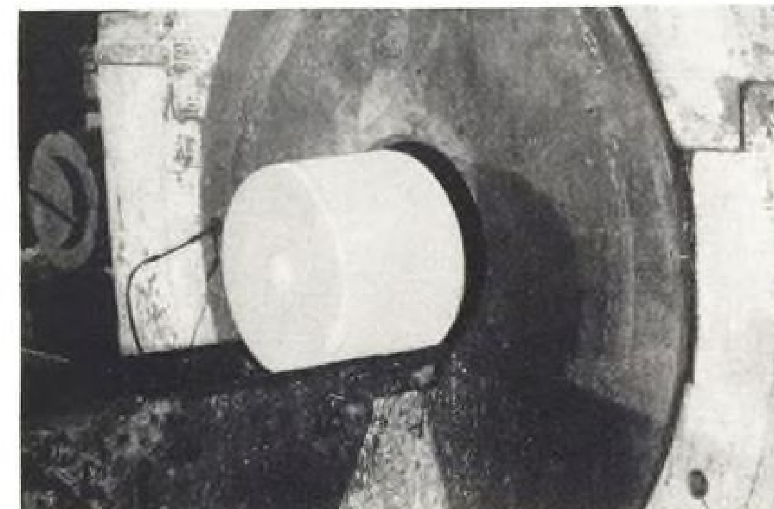
WHITE-HOT BILLET goes into 5500-ton press for shank formation. Reheated (right) it goes back for shank expansion and taper.
