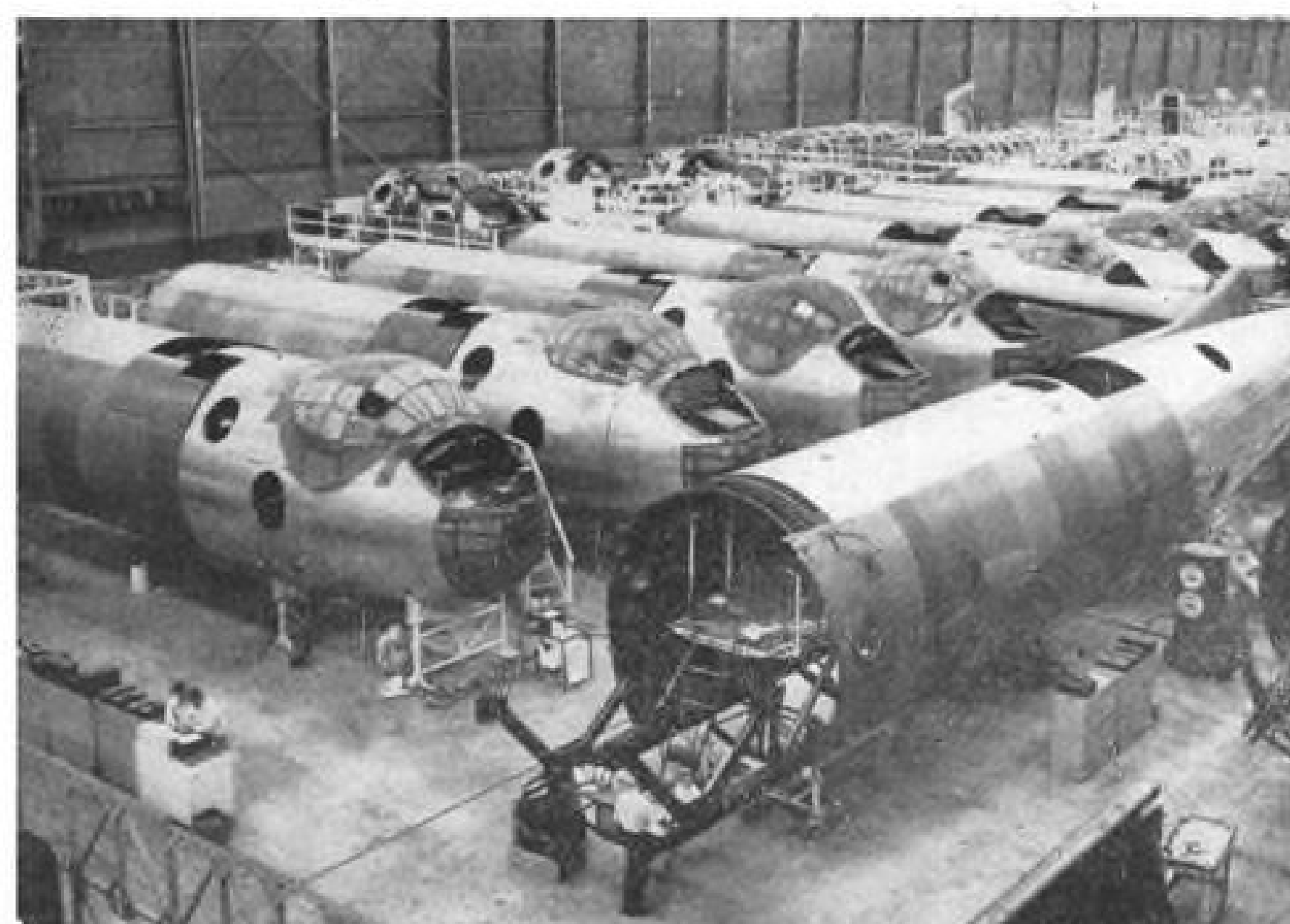
BUILDING THE BIG ONES—A portion of B-36 production (below) at Ft. Worth, showing nose, forward fuselage and tail sections being made and assembled.
