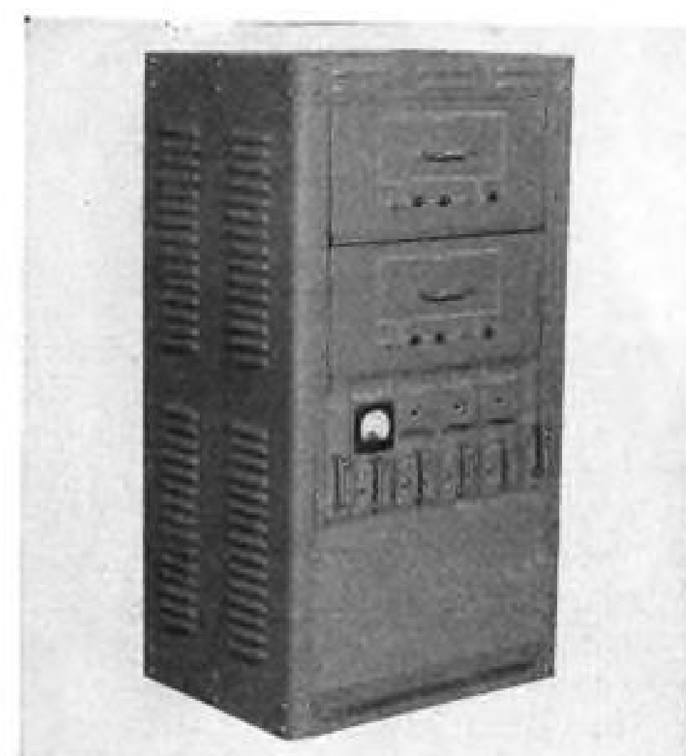
CONSOLE houses 4-channel continuous radio monitor developed by Brush.
