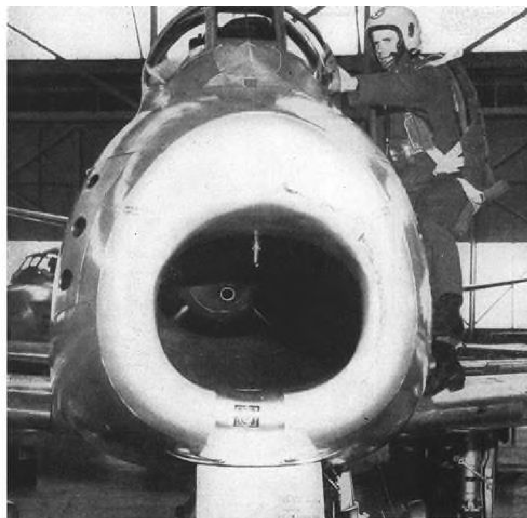
SABRE FORE AND AFT—Two detailed views of the nose and tail of the North American F-86 show oval inlet for the GE J-47 turbojet which can be seen deep in the fuselage, and the exhaust outlet. Rear view also shows extended fuselage dive brakes.
