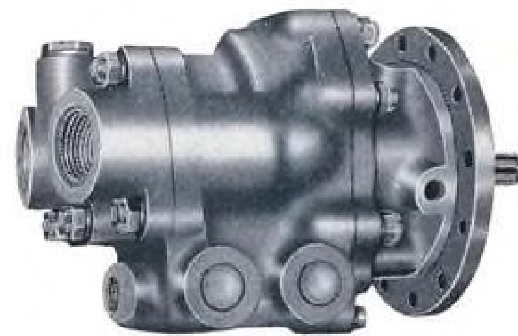
Pesco Model 011799 Unloading Gear Pump. Weight 8.6 lbs. Maximum continuous operating pressure 1500 p.s.i. Capacity 2 g.p.m. at 1500 r.p.m. Features Pesco's exclusive, patented "Pressure Loading" principle. Other models available for pressures to 3000 p.s.i.
