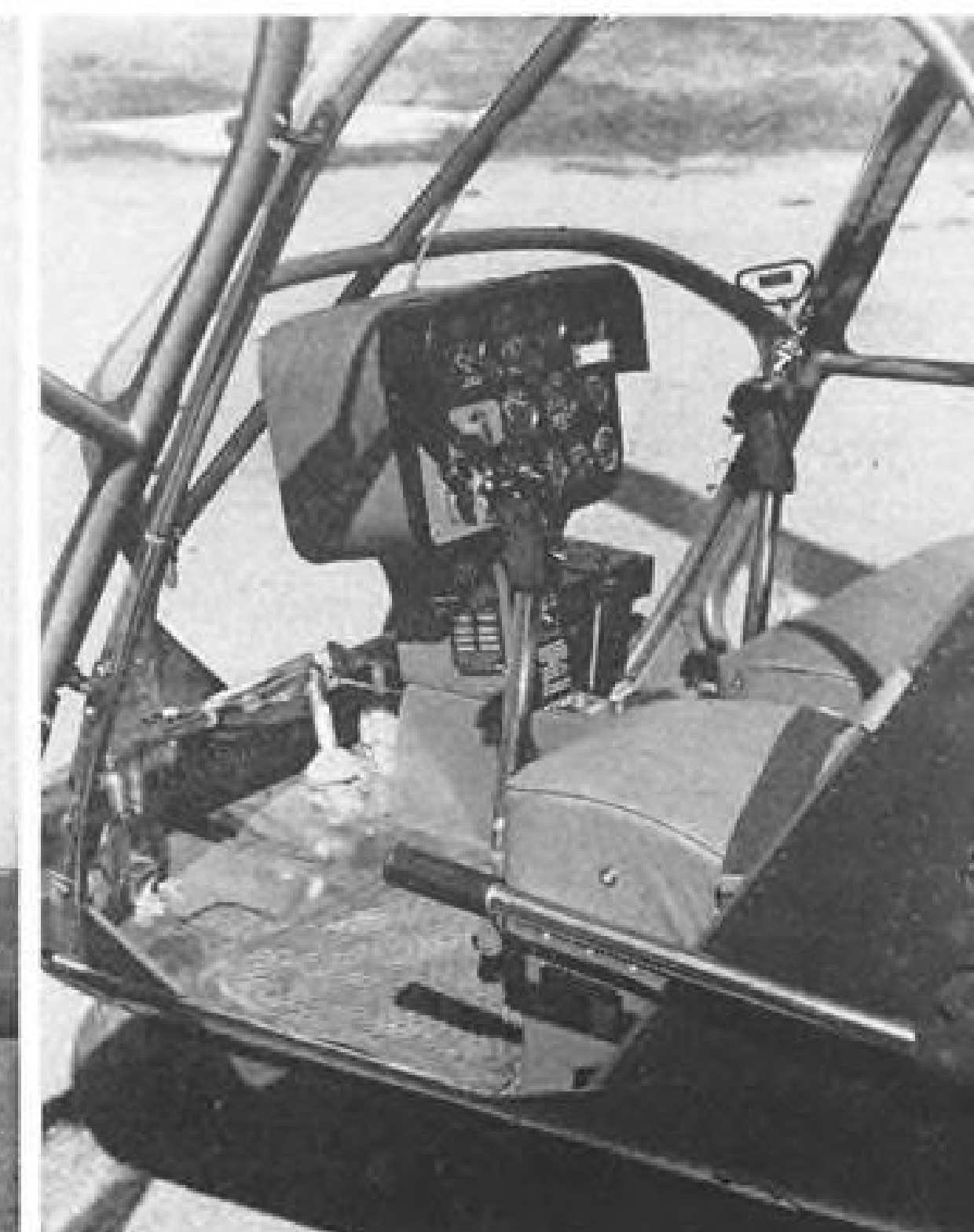
HILLER ARMY AMBULANCES —Two Hiller H-23A copters (below left) display their capacious externally mounted litters. The cockpit closeup details new placement of the control sticks (they were mounted overhead). The horizontal lever is for collective pitch control.
