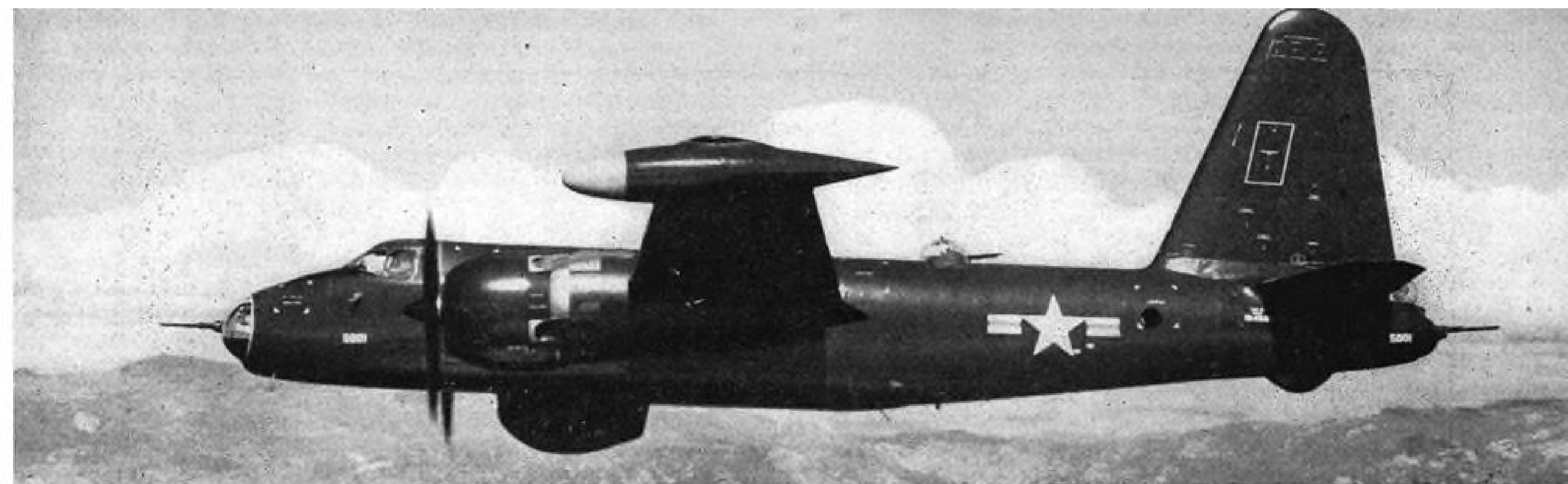
NEWEST NEPTUNE—Latest version of the Lockheed long-range Navy patrol bomber, the P2V-5, incorporates changes in nose armament—two flexible 20mm. cannon in place of earlier models' six fixed 20s—and increased and improved radar gear for tracking enemy naval craft. First P2V-5s will be delivered this month. The eight-place plane has two 3250-hp. Wright R-3350-30W compound engines.
