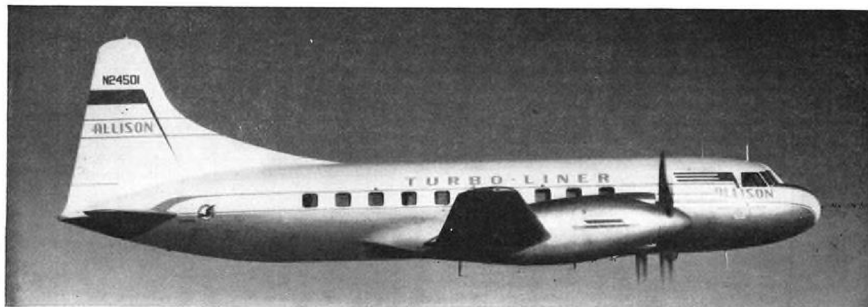
Turboliner, Allison's experimental turboprop version of the Convair-Liner.
