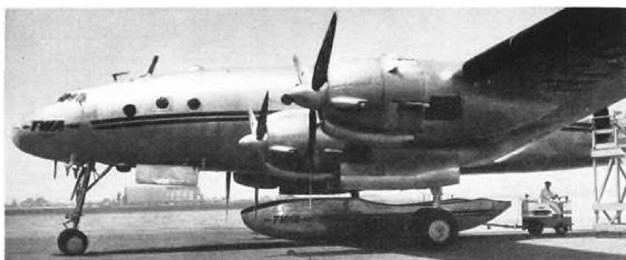
CARGO CONTAINER is towed under Constellation, hoisted by self-contained winch.
