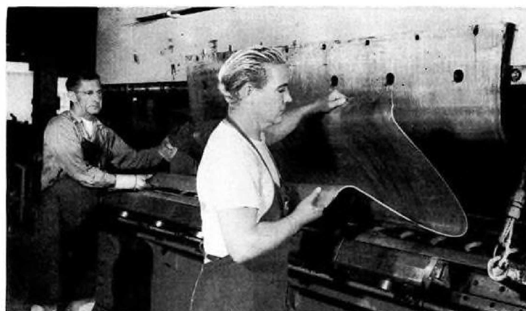
SKIN FORMED to leading edge contour is removed from hydraulic press brake.
