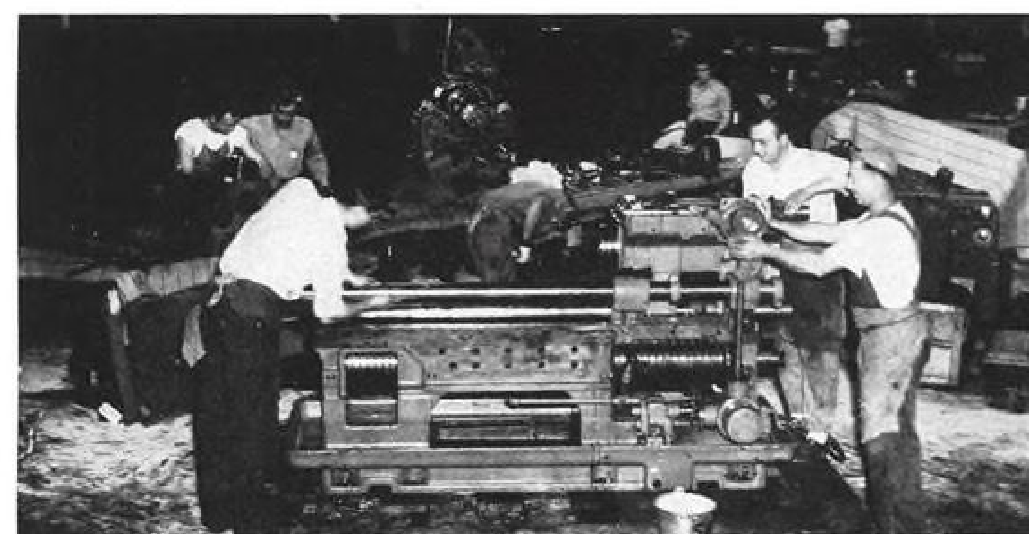
DISMANTLING GEAR HOUSING for thorough cleaning of shafts and interior parts.
