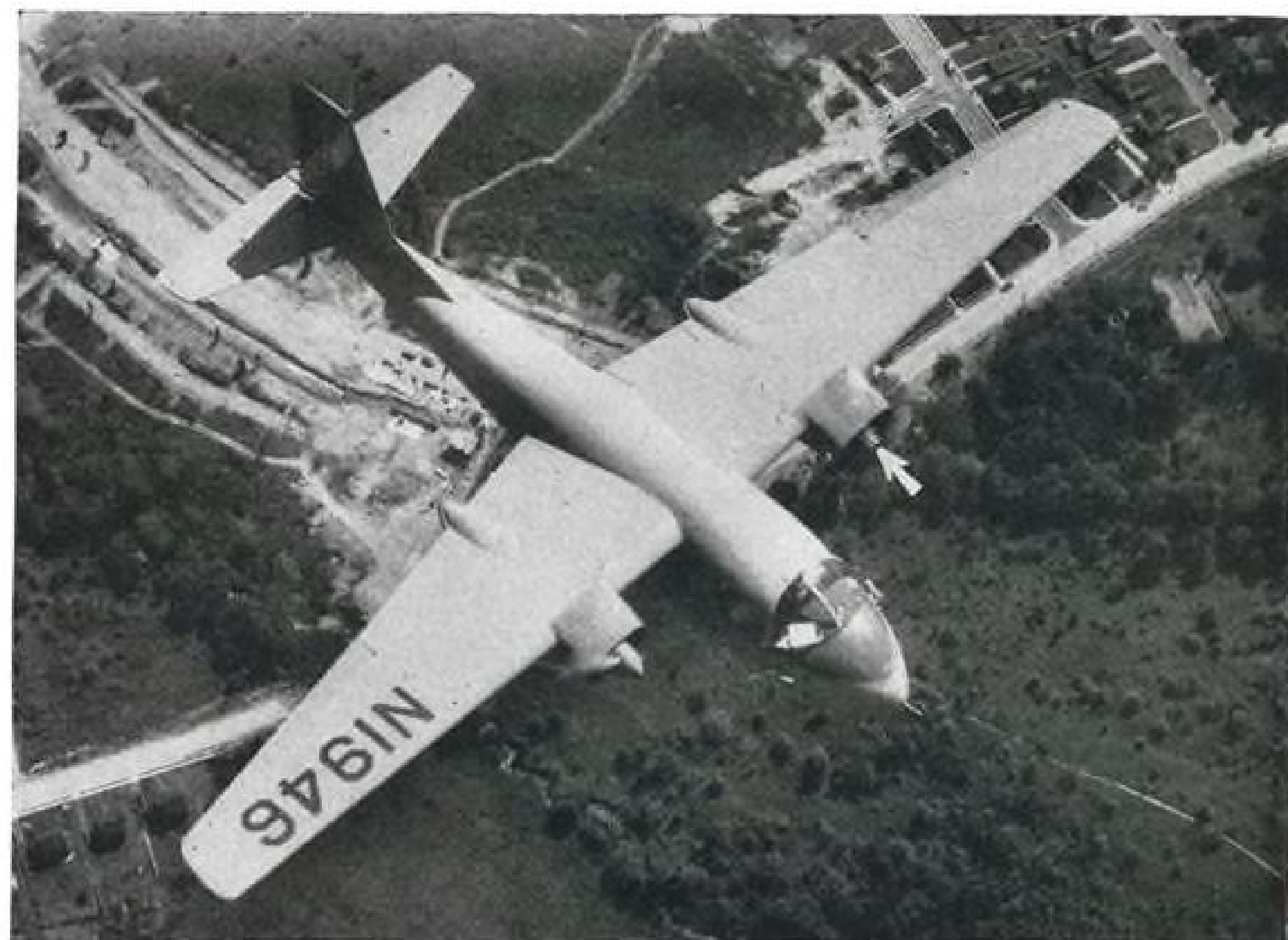
ONE PROP REMOVED, (arrow) the Aero Commander flies 1160 miles non-stop.
