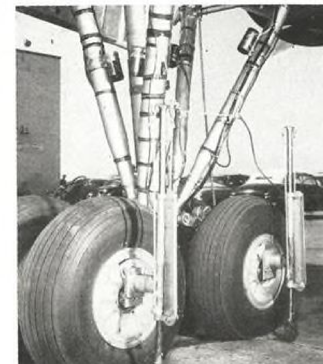
QUAD-WHEELED PACKET TESTED—Fairchild C-119 (below, left) has been fitted with new four-wheel bogie-type landing gear designed to improve plane's performance when operating on rough sod or soft-surface fields. The wheel truck is pivotal mounted. Test equipment includes rate-of-descent arms (right) to aid in measuring continuously the loads sustained during evaluation.
