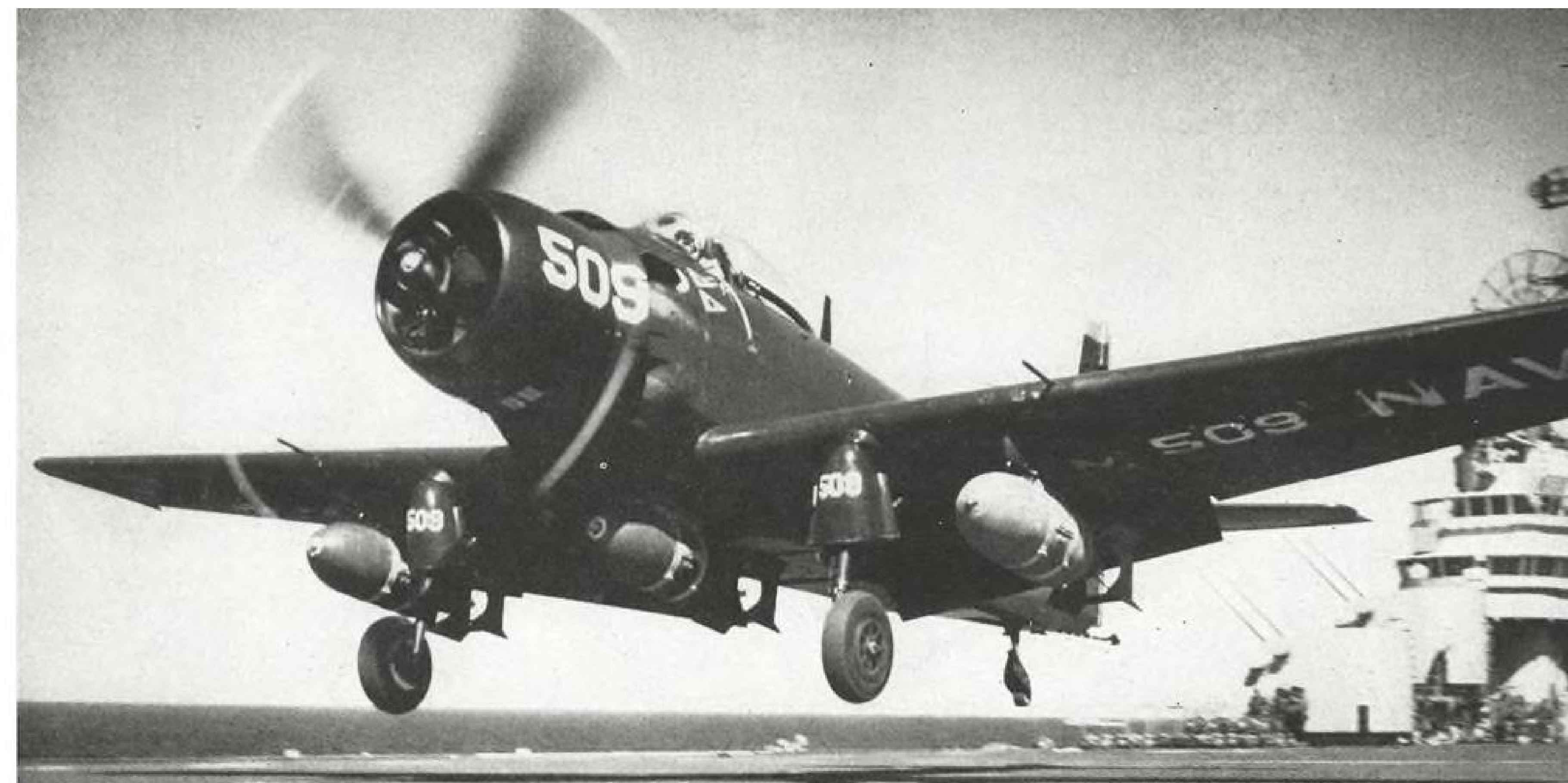
EGGS DUE TO DROP—Douglas AD Skyraider (Wright R-3350), carrying three 2000-lb. bombs, takes off from the 27,000-ton USS Valley Forge to strike enemy in Korea. Combat photo shows pilot is using considerable flap and right rudder in his takeoff.
