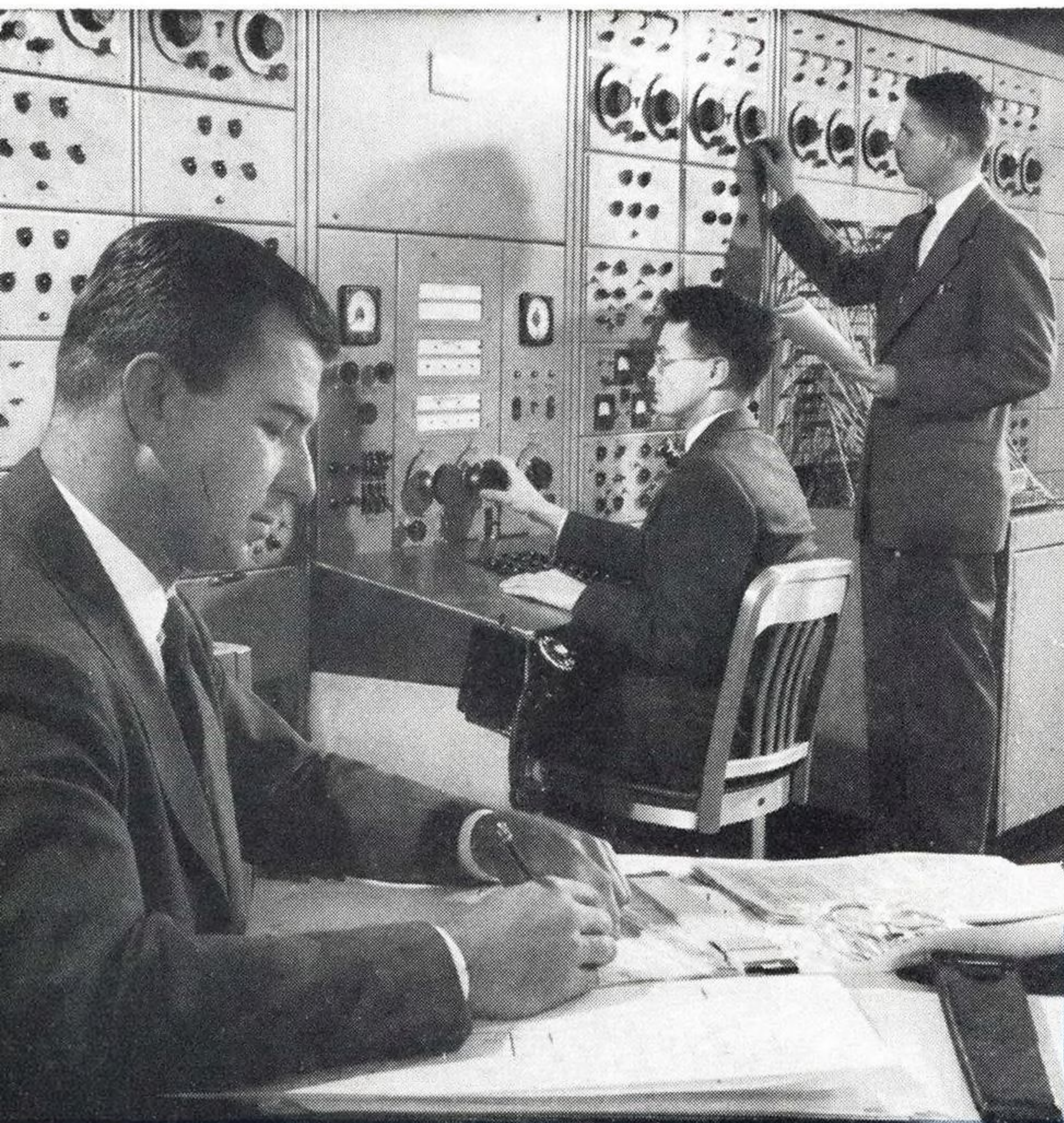
Complete electrical systems for any given aircraft can be simulated on this network analyzer.
