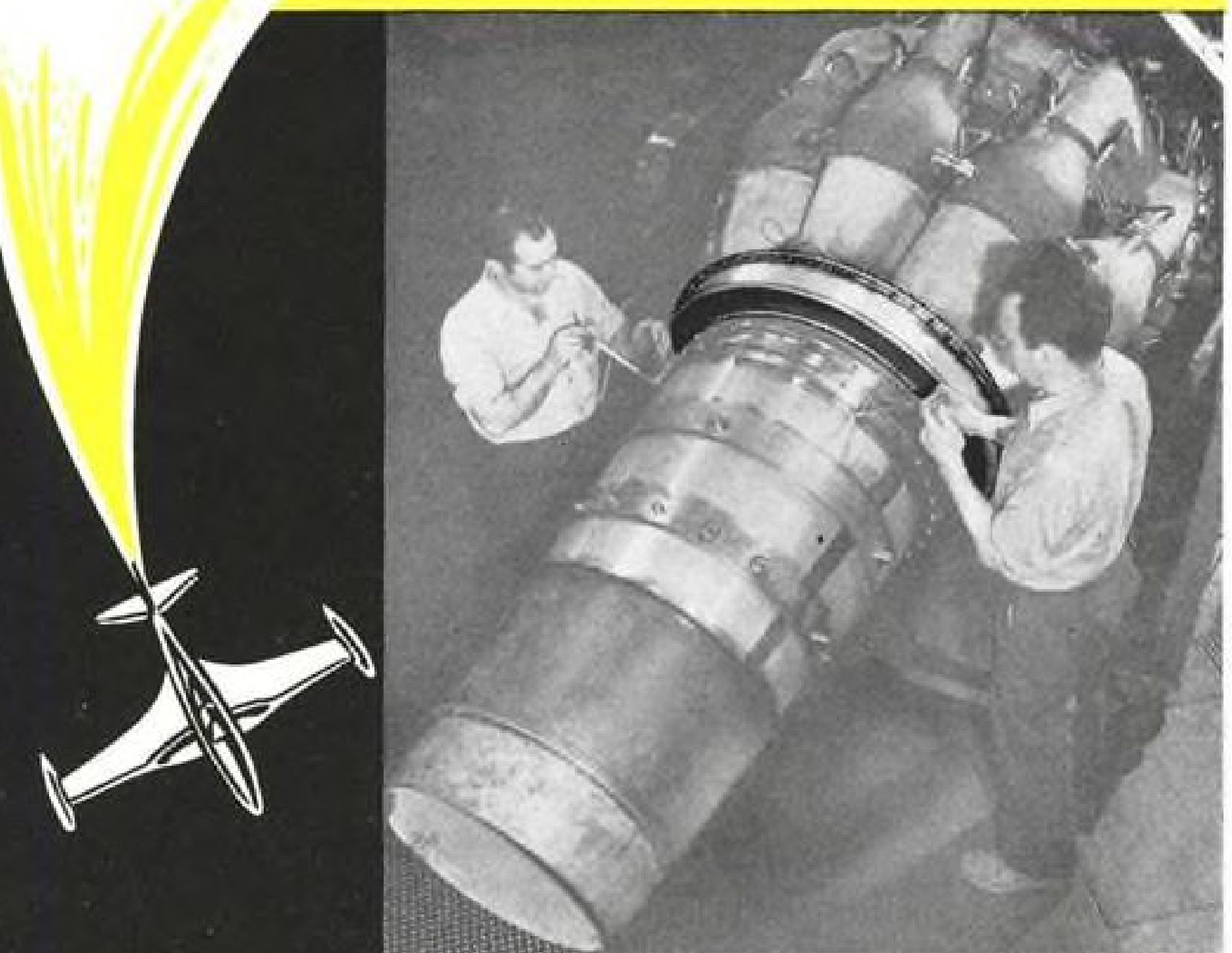
Hundreds of Air Manifold Cases for the Pratt & Whitney J-48 Turbo-Wasp are being turned out by Smith-Morris
