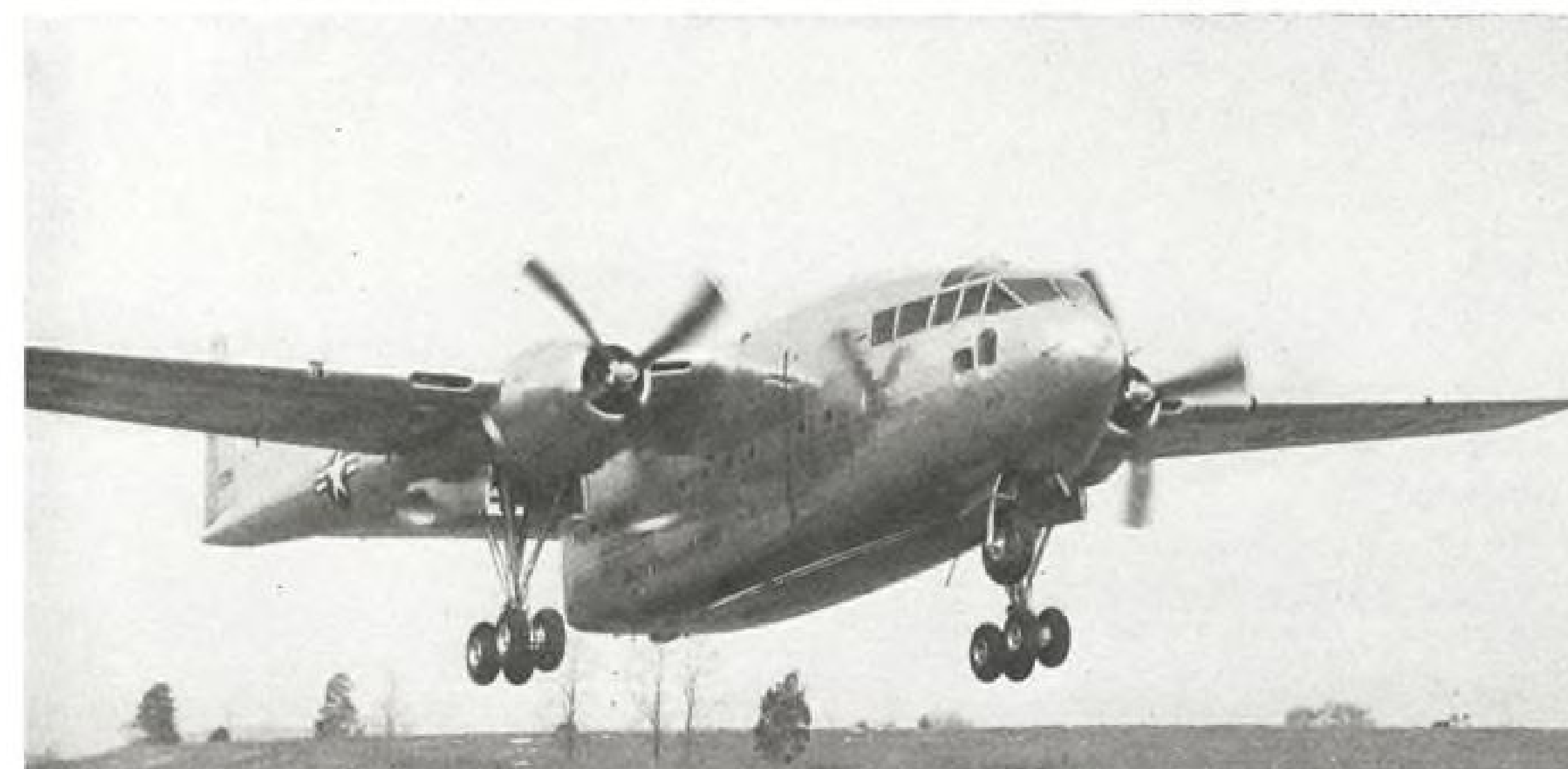
QUAD-WHEELED PACKET TESTED—Fairchild C-119 (below, left) has been fitted with new four-wheel bogie-type landing gear designed to improve plane's performance when operating on rough sod or soft-surface fields. The wheel truck is pivotal mounted. Test equipment includes rate-of-descent arms (right) to aid in measuring continuously the loads sustained during evaluation.
