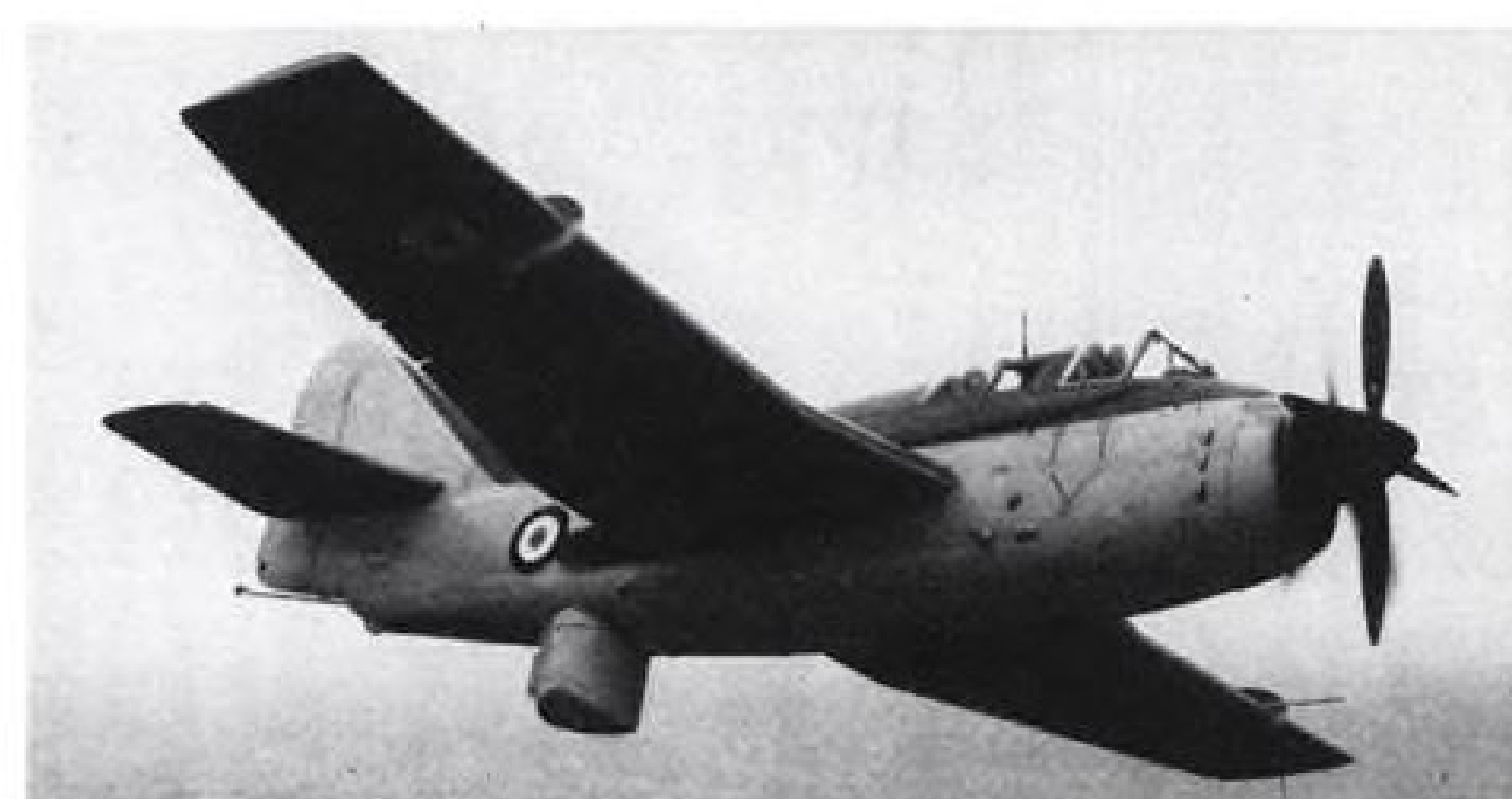
BRITISH SUB-HUNTERS —Production-type Fairey 17 turboprop plane (above left) has front cockpits revised, a rear cockpit added (hidden by wing) and wing fences. Rolls-Royce Griffon powered Fairey Mk. 7 (right) carries two radar men in new rear cockpit.
