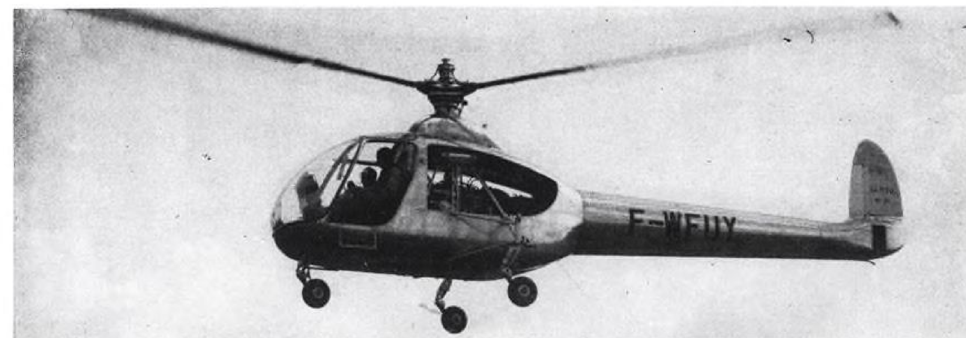
ARIEL III shows clean lines in this proving flight. Turbine exhaust may be deflected by pedal action for rudder control.
