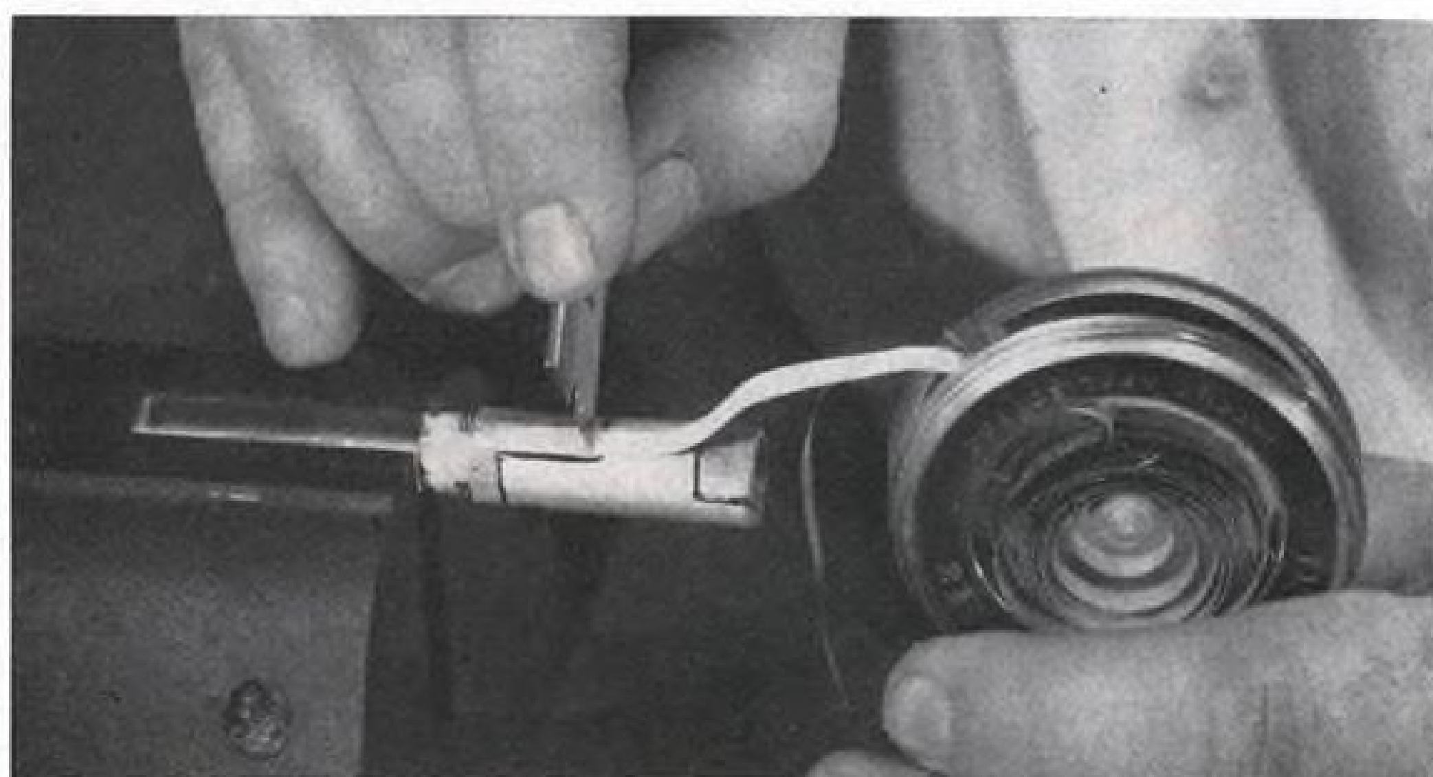
APPLYING tape resistor to miniature chassis. Tape is cut off with razor blade.
