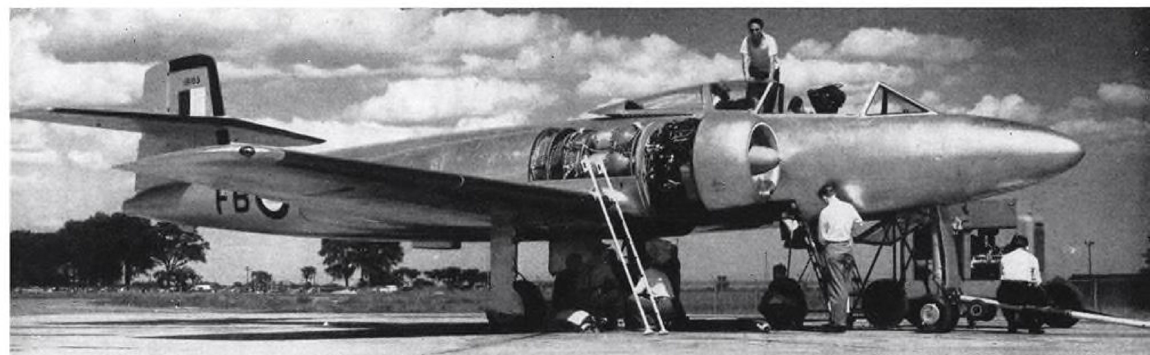
CANUCK GETS ORENDAS —First all-Canadian jet fighter, the A. V. Roe Canada CF-100 Canuck with new 7,000 lb. thrust A. V. Roe Canada Orenda turbojets gets last-minute check prior to first flight in mid-June. Previous CF-100s had British-built Rolls-Royce Avons.
