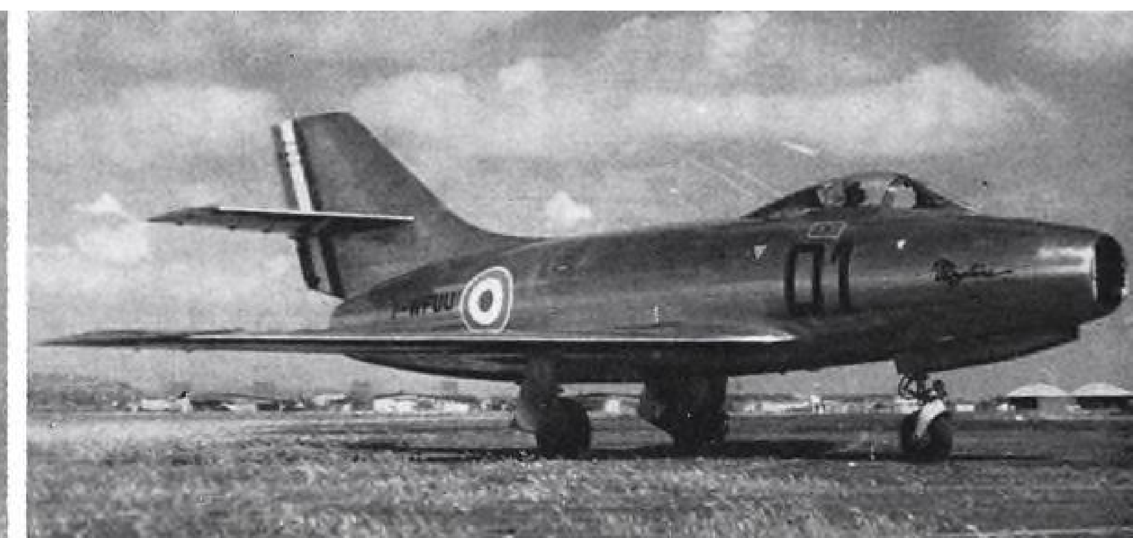
FIGHTING FAMILY —Straight-wing Dassault MD-450 Ouragan (Hurricane), above left, and its sweptwing development, the MD-452 Mystere, (right) figure importantly in French Air Force fighter build-up. Both use Rolls-Royce Nene. MD-452 has done over 625 mph.
