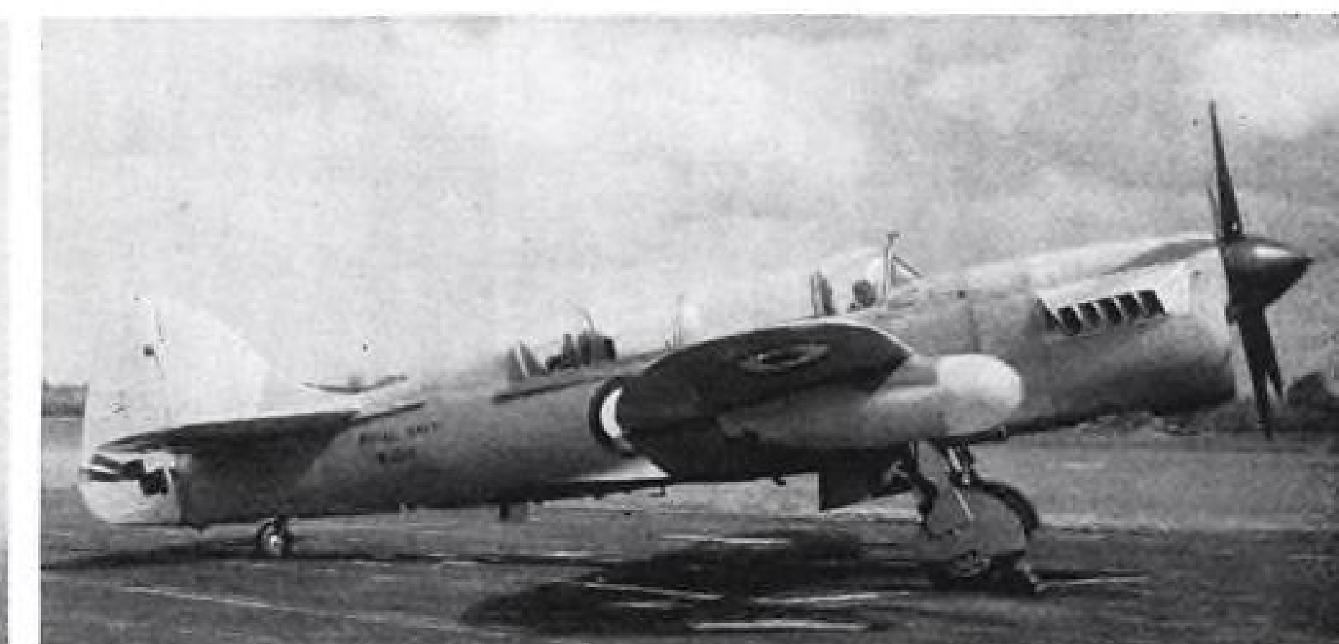
BRITISH SUB-HUNTERS —Production-type Fairey 17 turboprop plane (above left) has front cockpits revised, a rear cockpit added (hidden by wing) and wing fences. Rolls-Royce Griffon powered Fairey Mk. 7 (right) carries two radar men in new rear cockpit.
