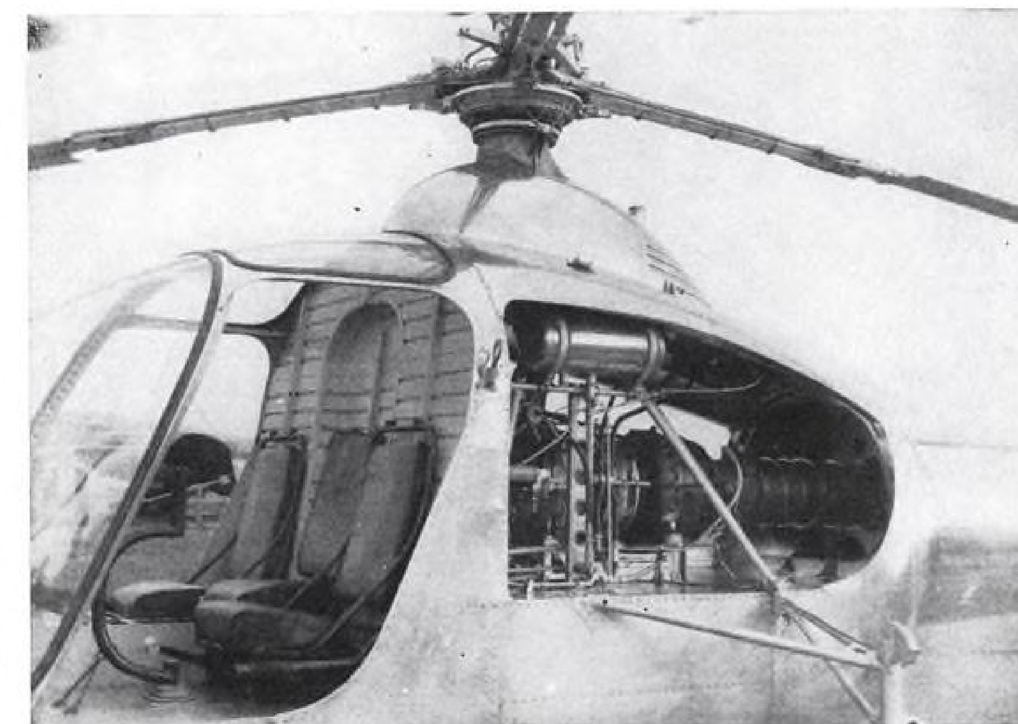
ROOMY COCKPIT accommodates three, with controls at each outside seat. Residual thrust from turbine is tailpiped through boom.
