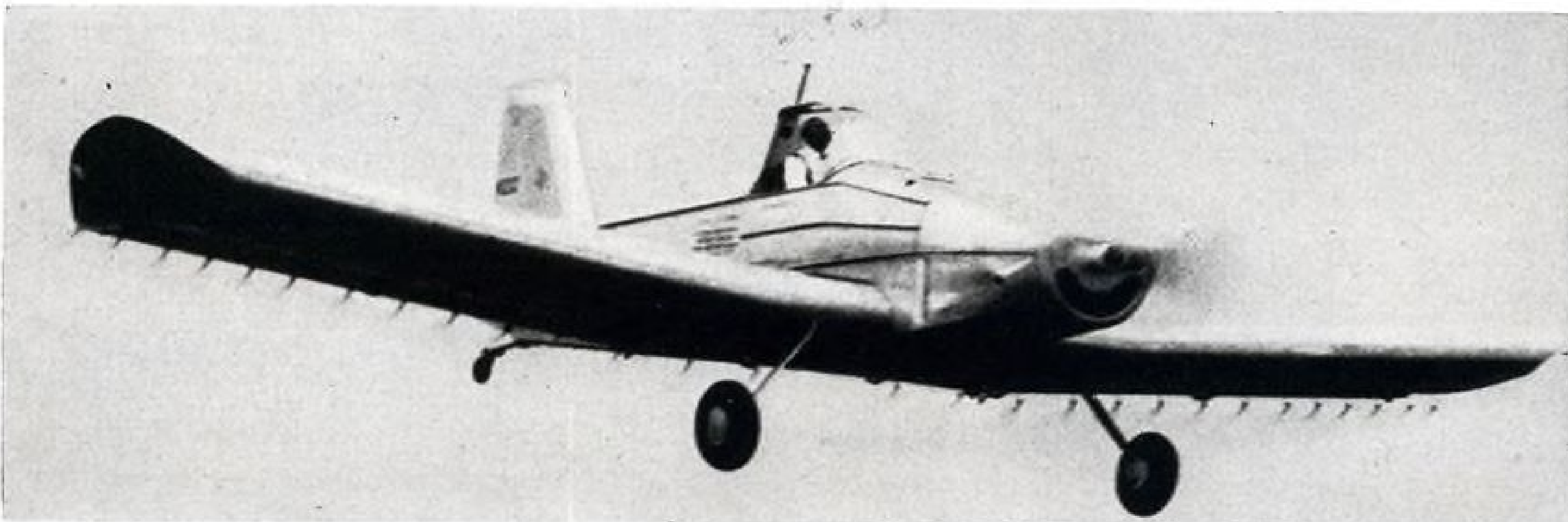
SPRAY EQUIPMENT which, running full span of wing, gives maximum distribution. Dusting equipment will fit behind engine.
