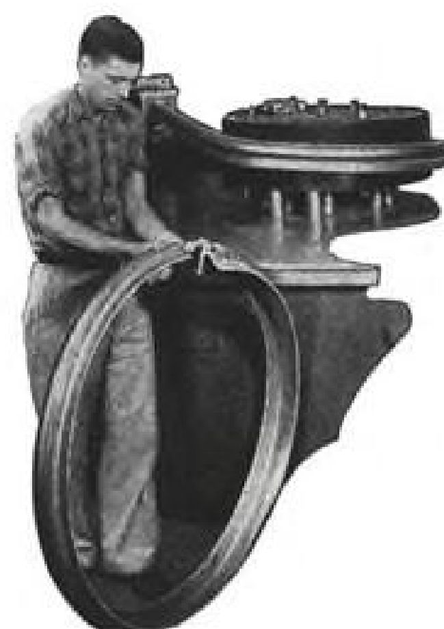
Aluminum gun turret rings accurately formed to complete circle.
