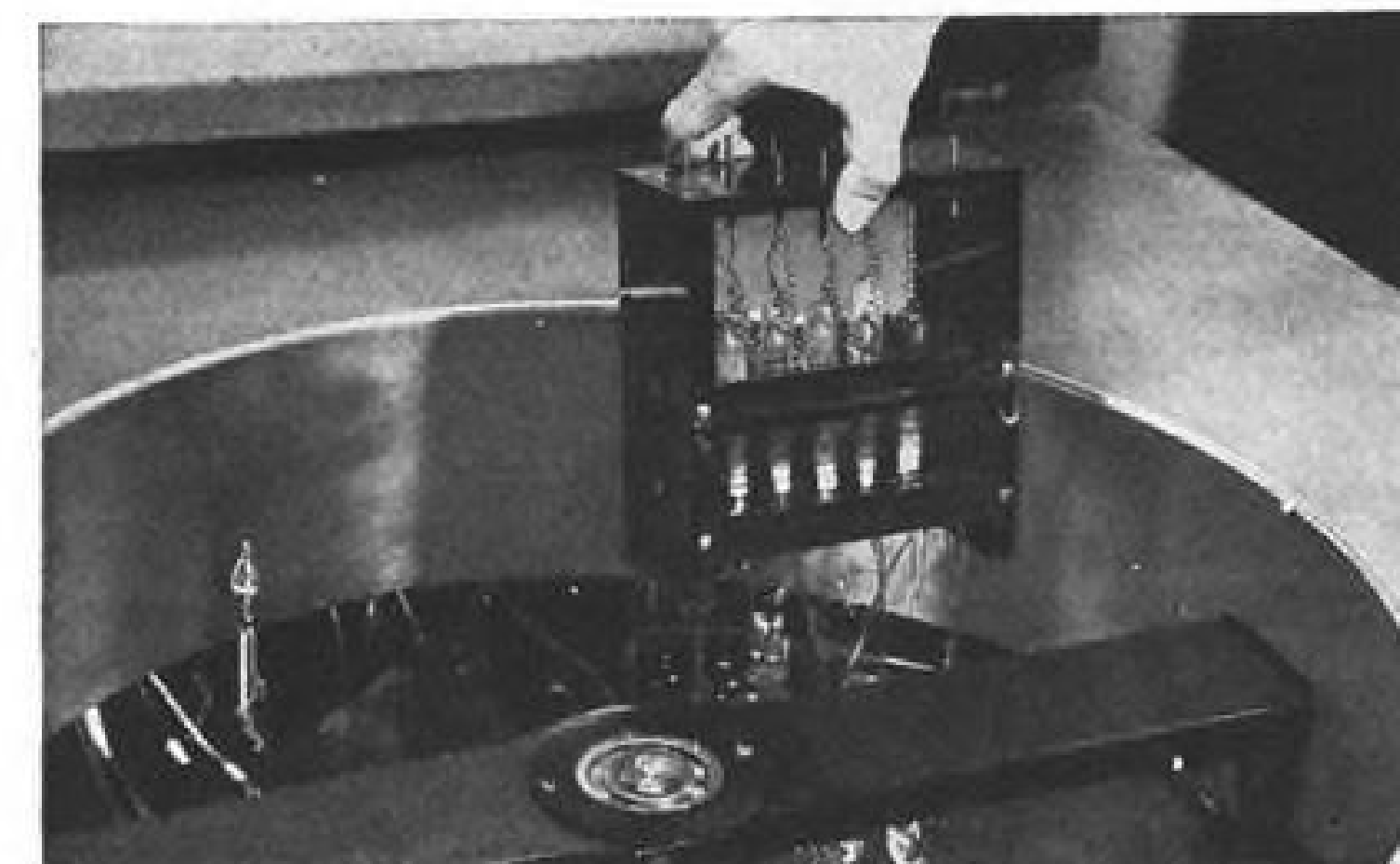
VOLT STANDARD is periodically compared with that of the National Bureau of Standards in Washington, D. C. to within 0.000001 volt.
