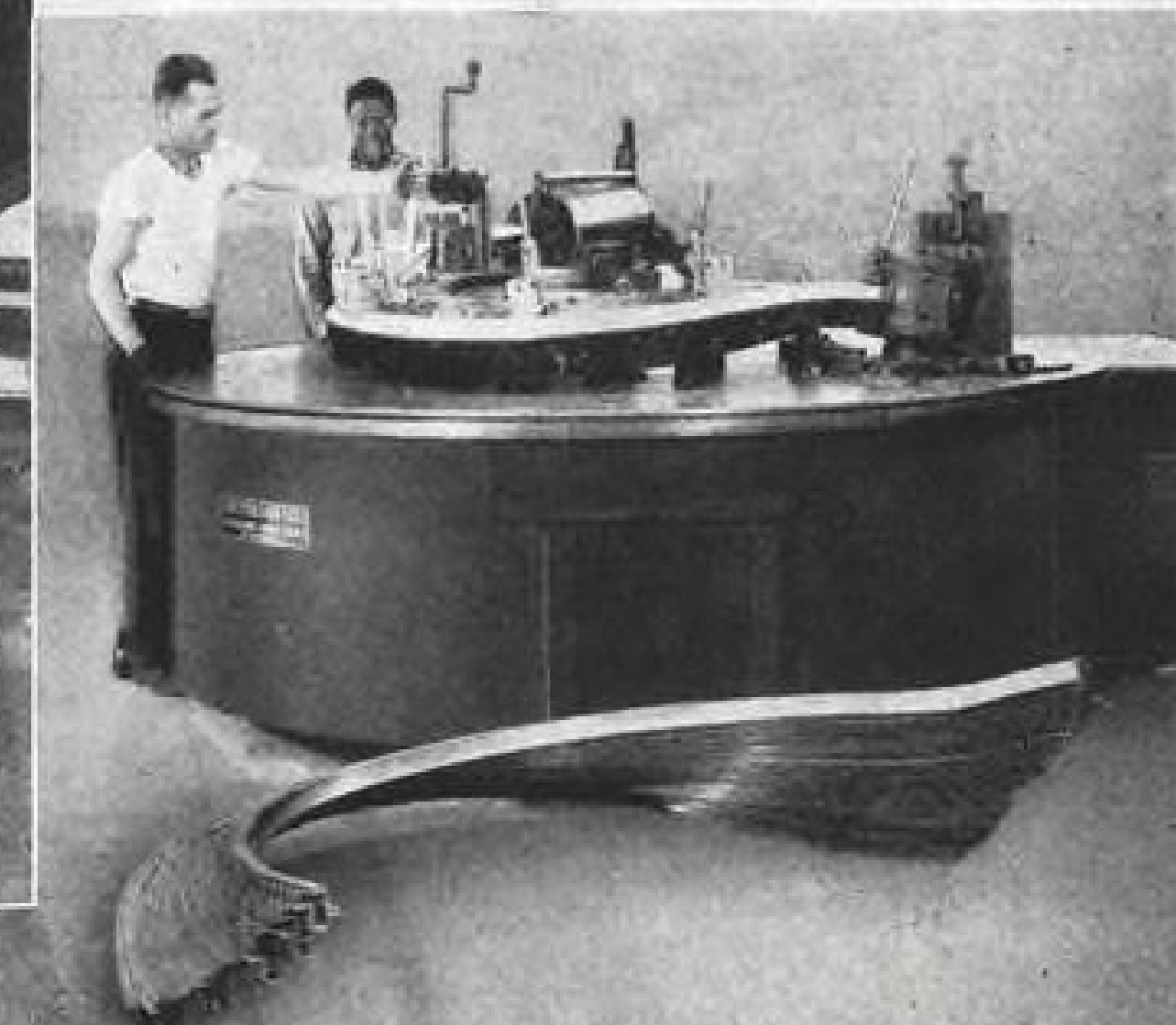
Showing aluminum "Z" extrusion being formed in both horizontal and vertical curves.
