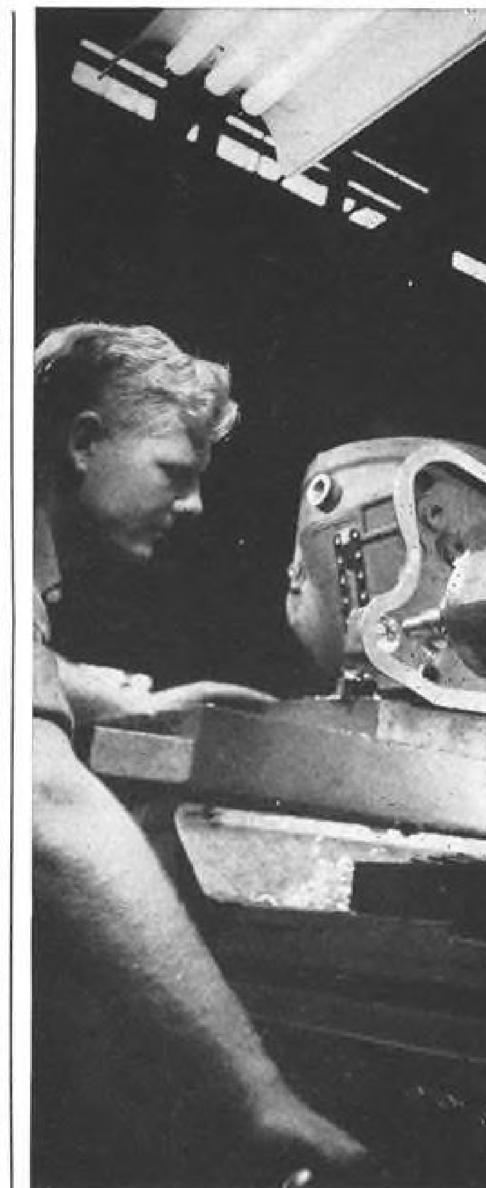
FIXED JIG is located over pit for two-side access. Panel is then transferred to . . .
