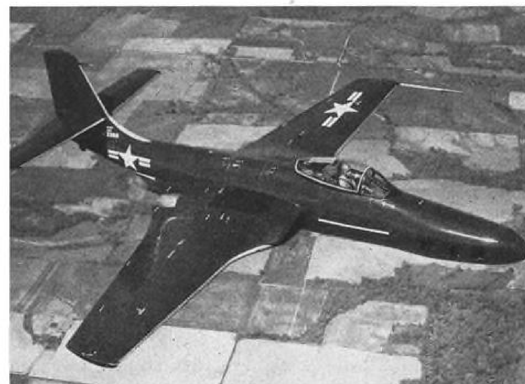
PHOTO BANSHEE —McDonnell F2H-2P has had its nose extended and enlarged to take six different types of cameras for photo reconnaissance at 50 to 50,000-ft. altitudes.
