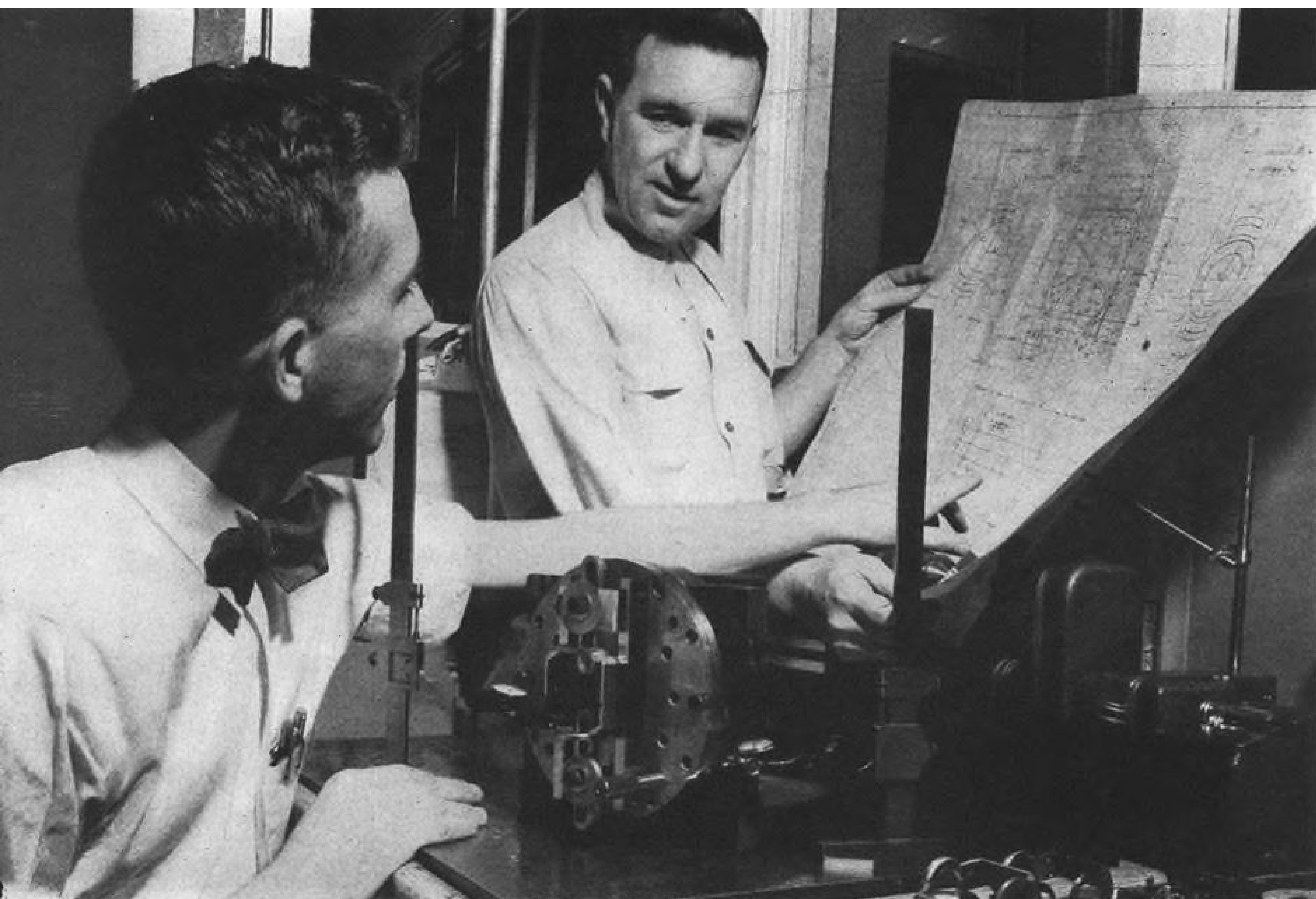
GAGE INSPECTORS MAKE COMPLETE DIMENSIONAL ANALYSIS OF GYRO GIMBAL PARTS. THIS WORK IS DONE IN TEMPERATURE CONTROLLED ROOMS.
