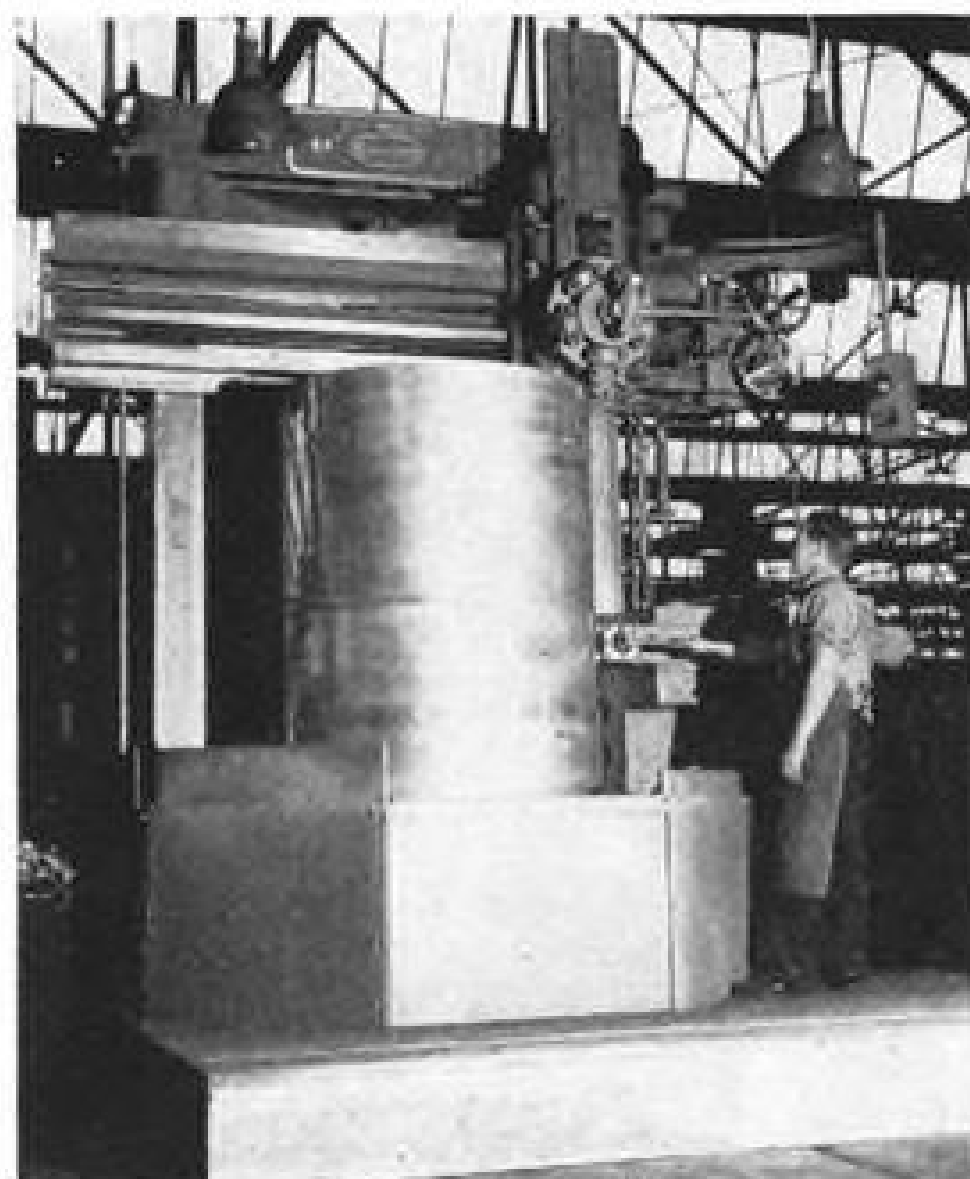
BULLARD VERTICAL TURRET LATHE (left) features high boring mill with raised bed; Turchan hydraulic duplicator (right) converts Bullard vertical turret lathe into an automatic production tool.
