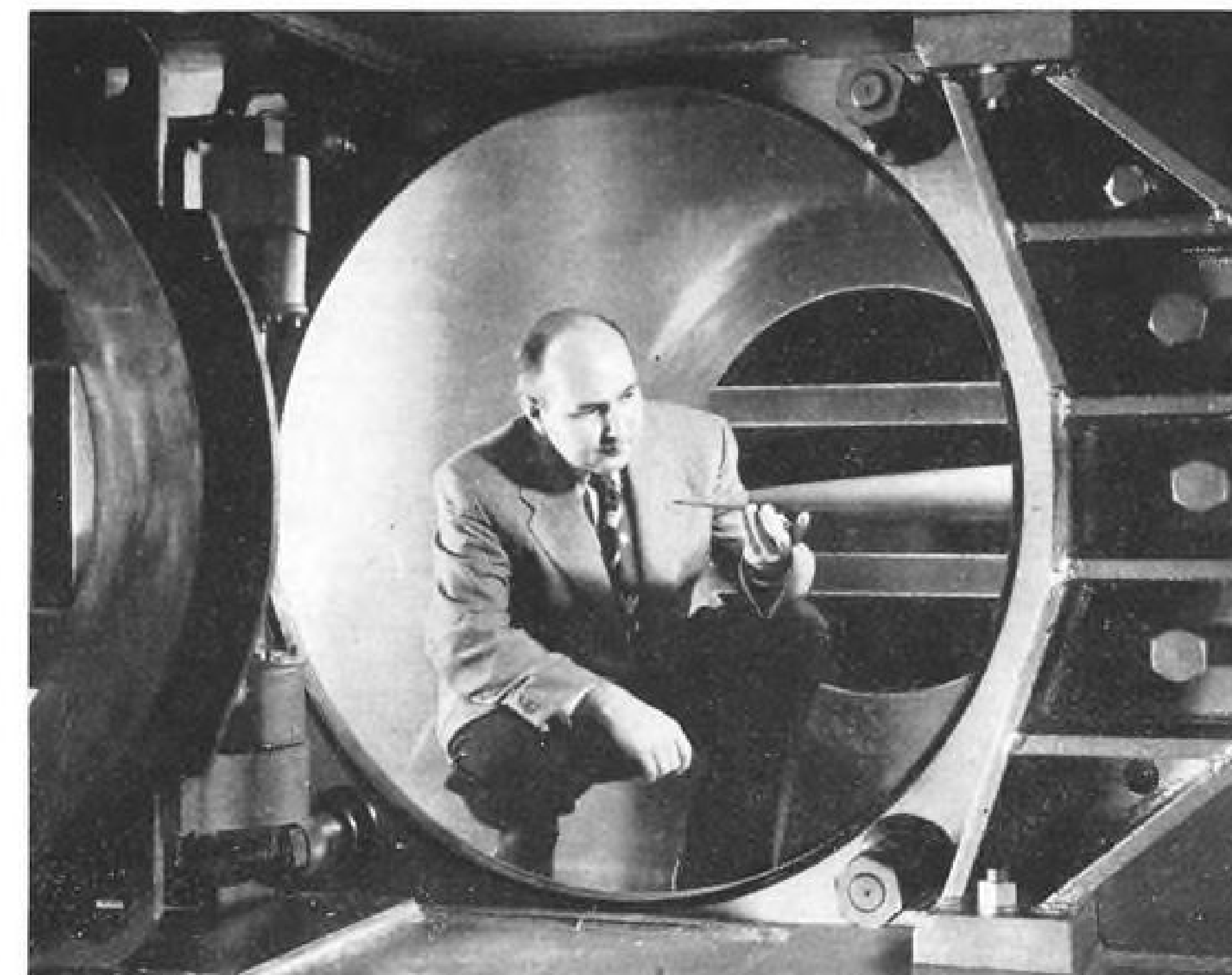
AIR LOCK, (above left), a guillotine-type valve, seals windtunnel test section so that technicians can work under normal pressure. Remainder of dry air stays at different pressure in rest of tunnel. Pneumatically operated valves bleed or add air, are part of pressure control system, and not related to air lock. Donald D. Baals (right) head of 4- by 4-ft. supersonic tunnel, crouches in test section housing missile model.
