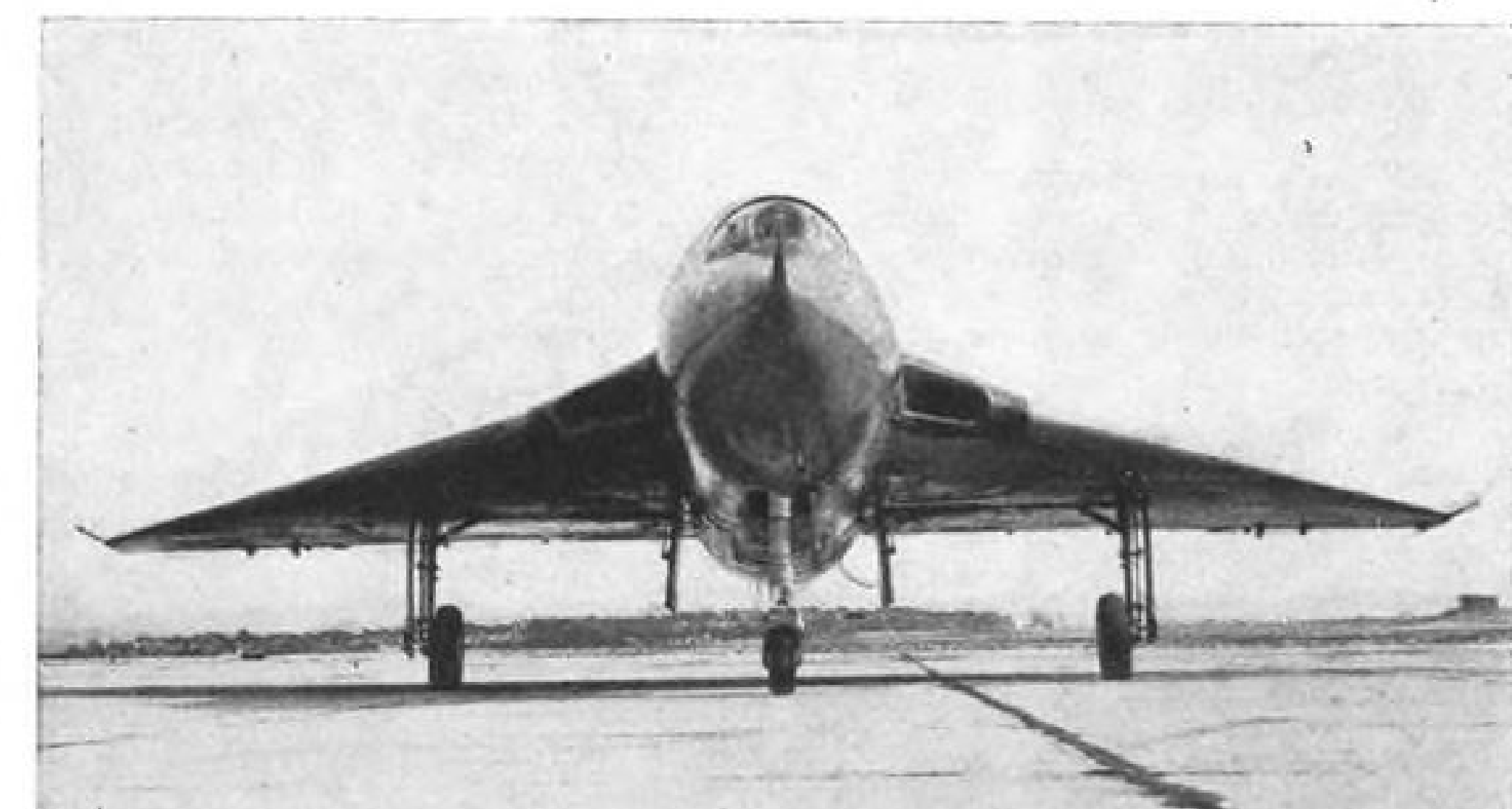
NEW DELTA CONFIGURATION, British Avro 707A, has a high, sweptwing; wide landing gear tread and sharply tipped wing.
