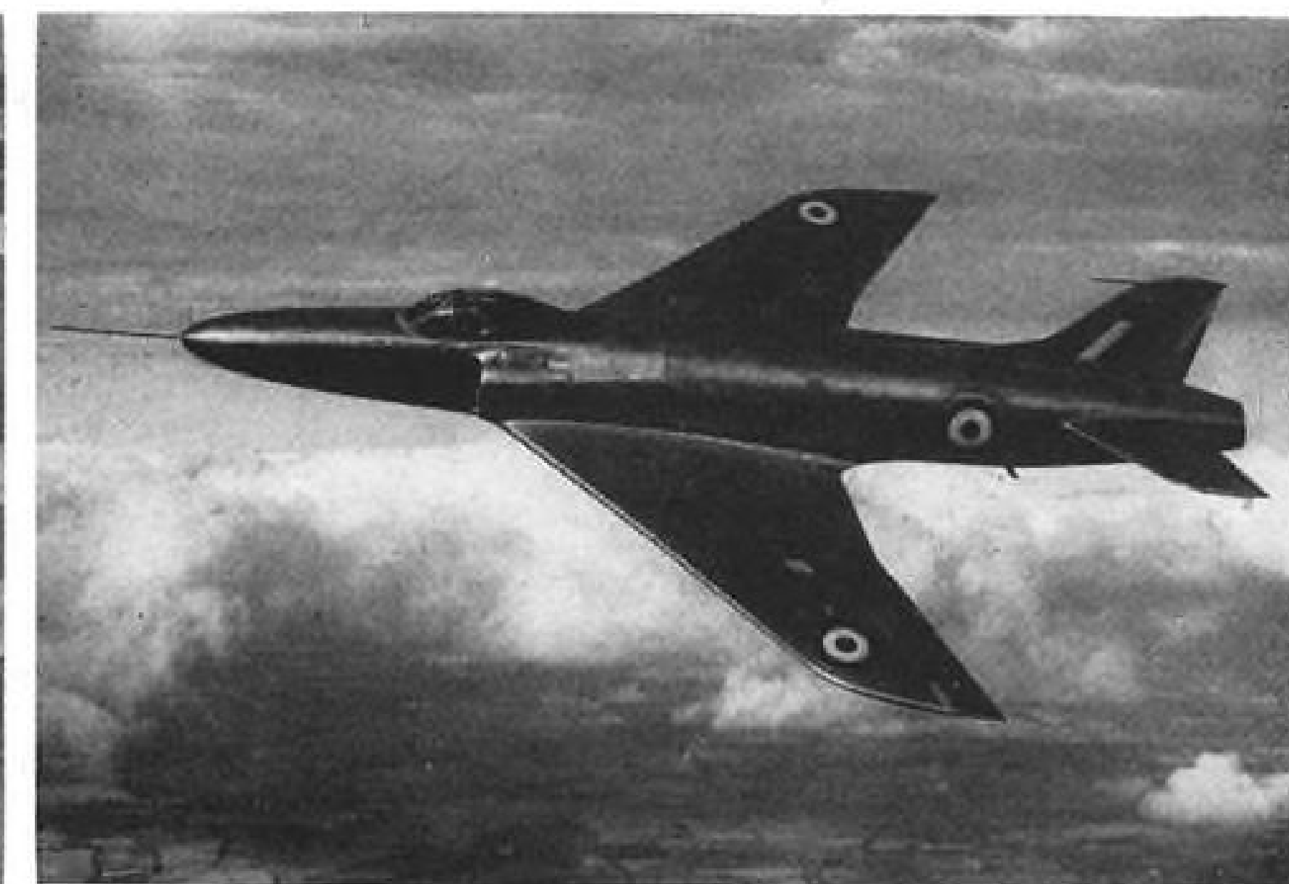
RAF'S NEW SWIFT —In quantity production for RAF fighter squadrons, the new Rolls-Royce Avon-powered Supermarine Swift shows its irregular planform, sweptwing while in a bank.
