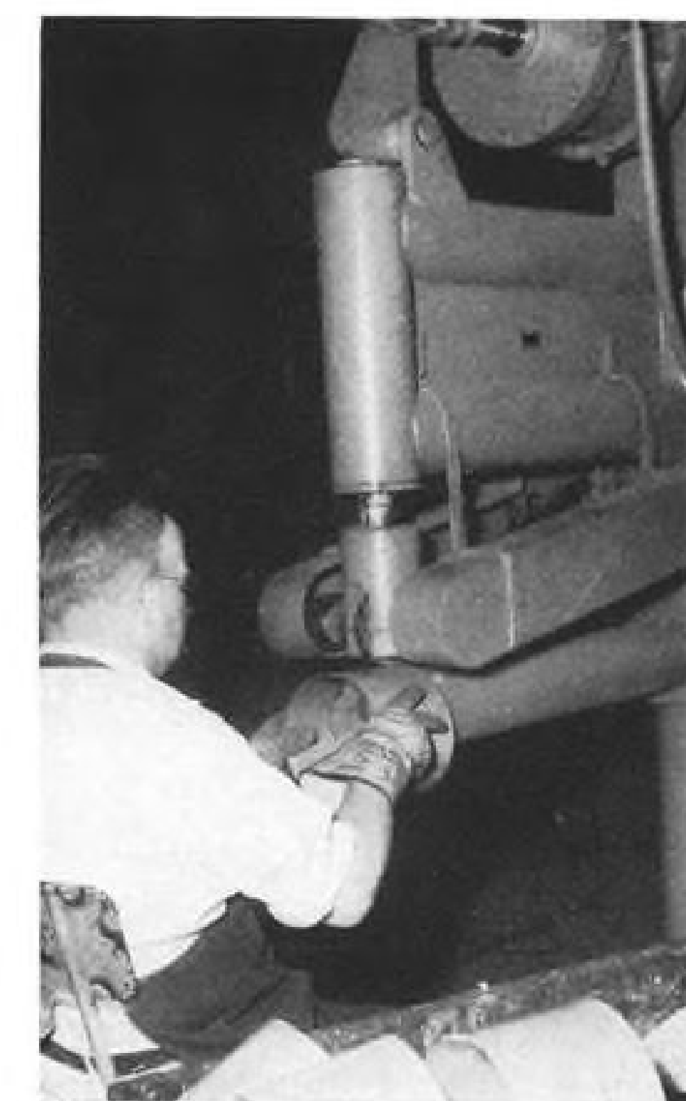
RYAN-BUILT SEAM ROLLER flattens Heliarc welded seams in a matter of seconds.
