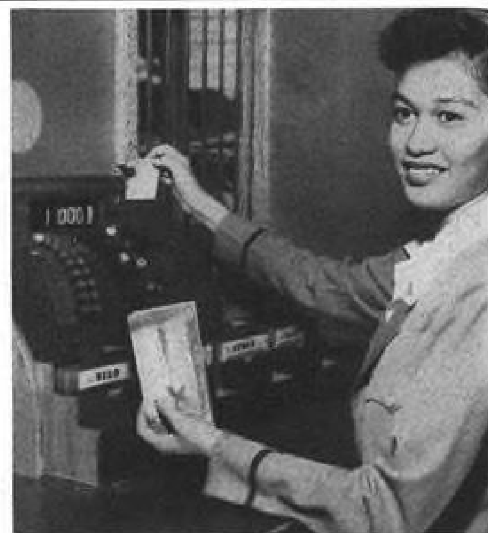
HAWAIIAN AIRLINES' modified cash register quickly checks in passengers and baggage.
