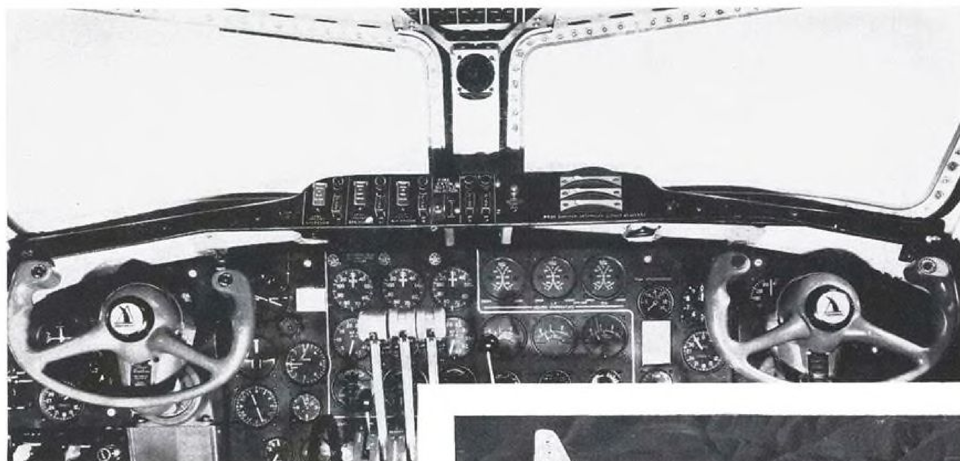
High-strength, high-impact panels of Pittsburgh Flexseal are used in connection with the warm-air de-icing system in the windshield of the C-125 "Raider," built by Northrop Aircraft, Inc., Hawthorne, Calif.
