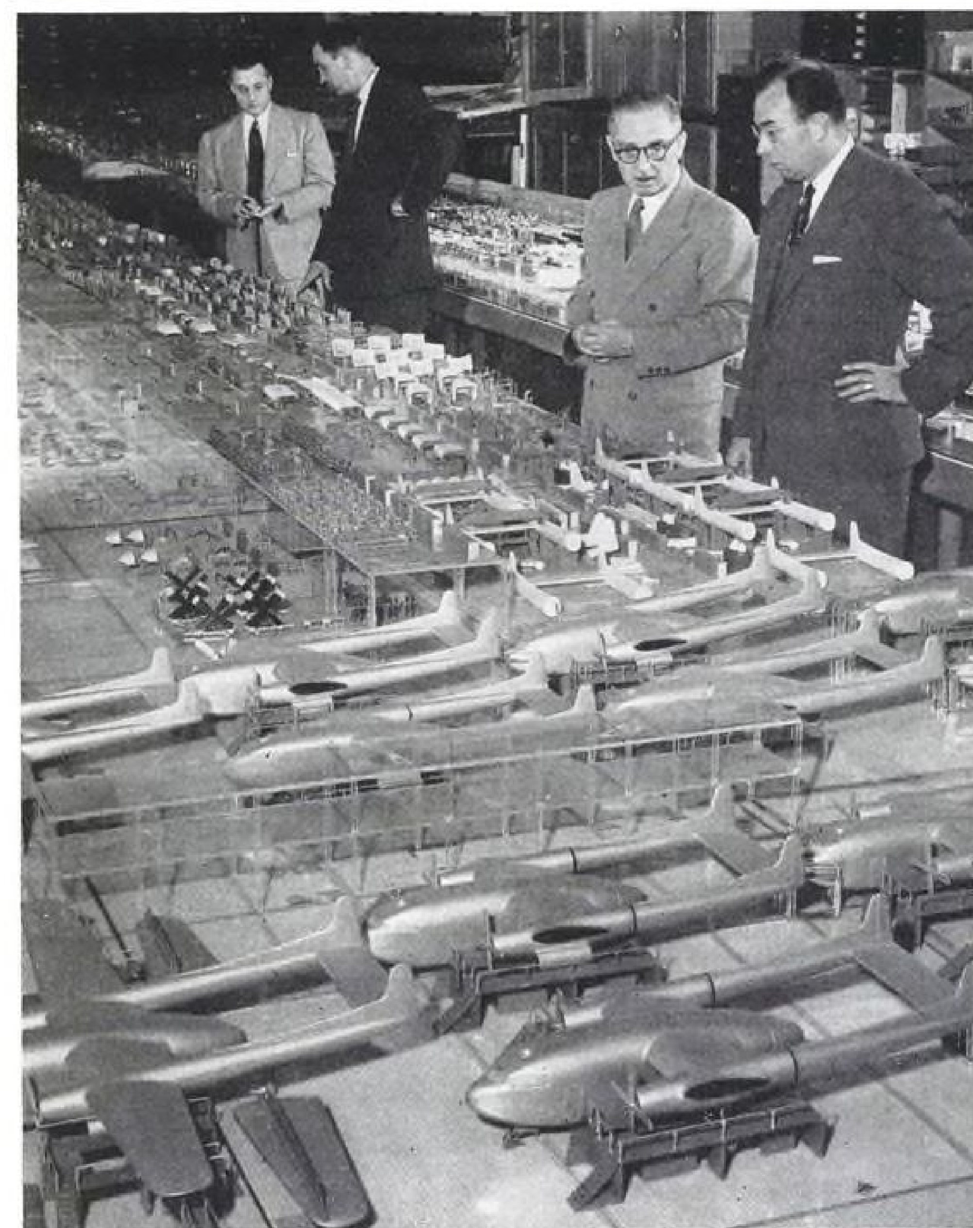
NOT A TOY but a production aid is this 1:48 scale model of Kaiser-Frazer Willow Run plant, with replicas of Fairchild C-119 on assembly line. K-F President Edgar Kaiser (right) inspects 70 x 35-ft. layout with other K-F executives.
