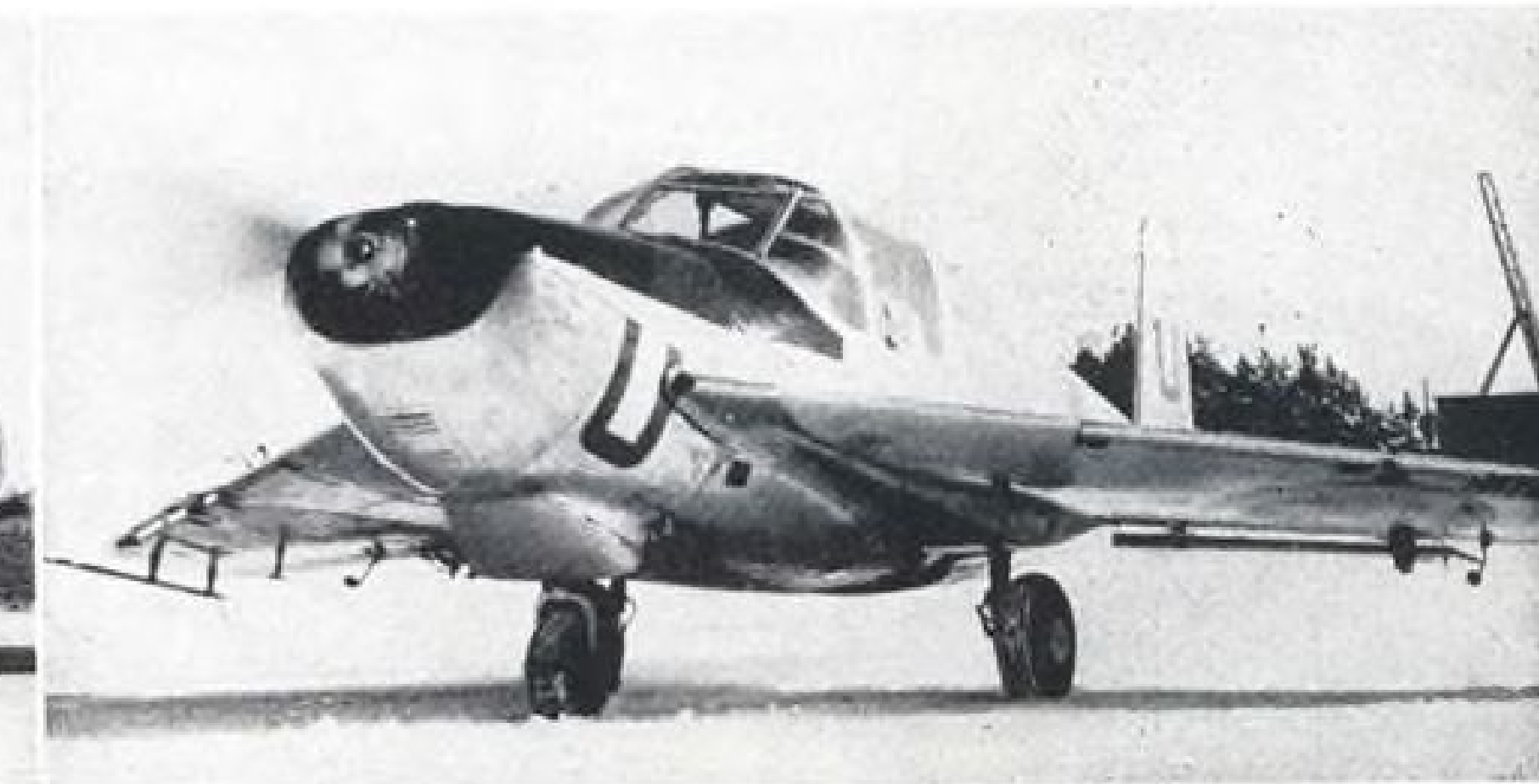
SPECIAL SAFIR 91B mounts half-scale swept wing for studies of configuration. Leading-edge slots and special flaps are fitted.
