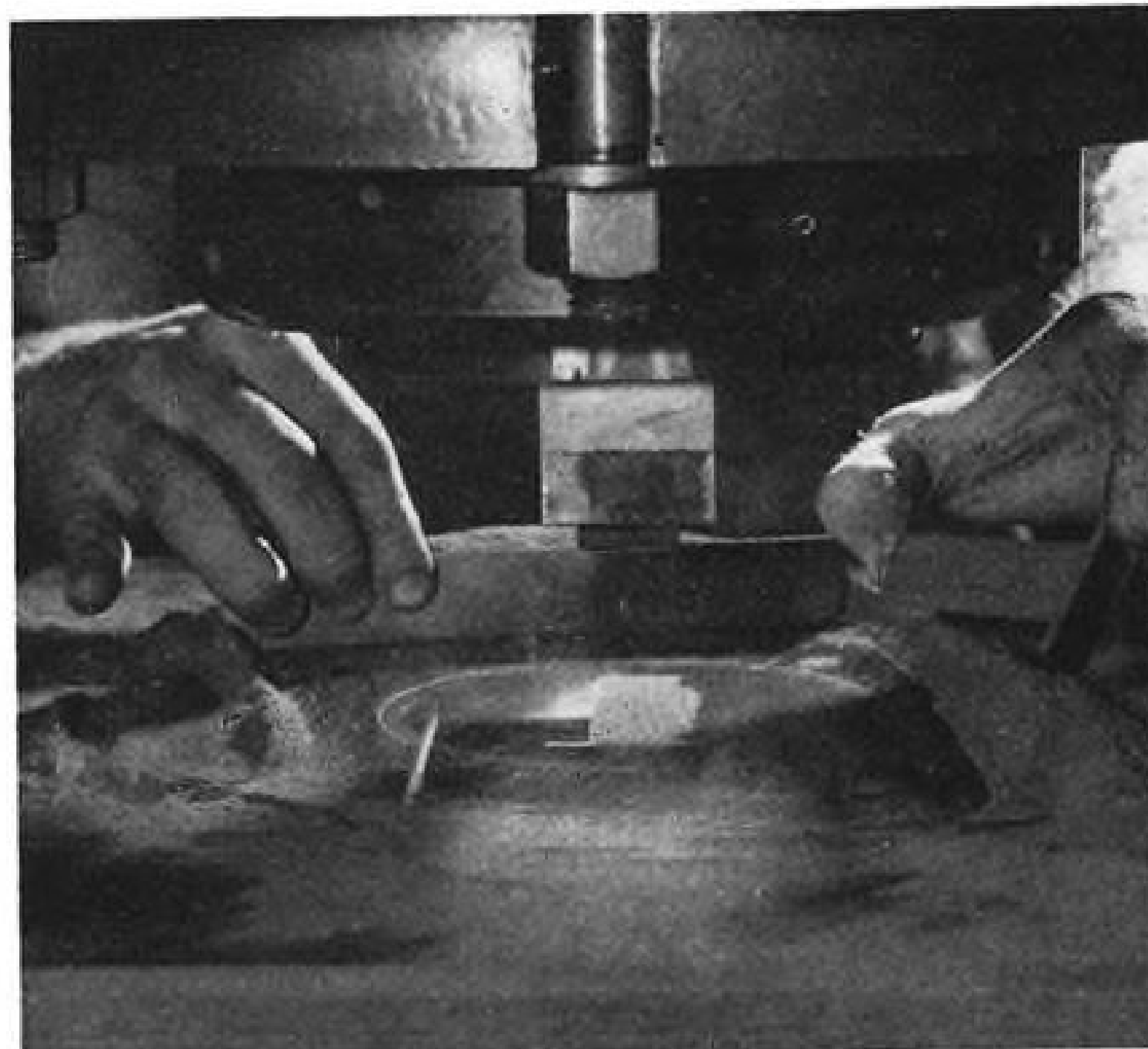
MOLDING takes place after cavity is filled with powder metal. Dies last 30-50 times longer than drop forge dies. COINING follows molding and sintering, gives blade additional strength by further compression.
