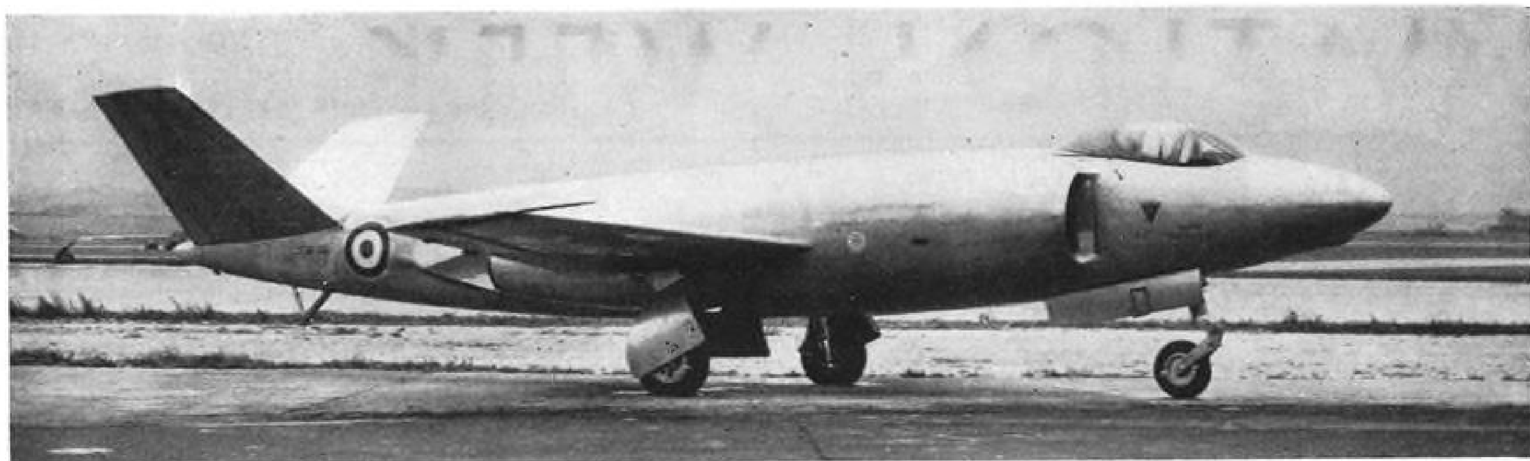
SUPERMARINE 508 features a Vee tail, is said to be the fastest and most powerful fighter ever designed for naval operations, which may well be a valid claim since it is powered by two Rolls-Royce Avon turbojets. Main wheels of tricycle landing gear retract.
