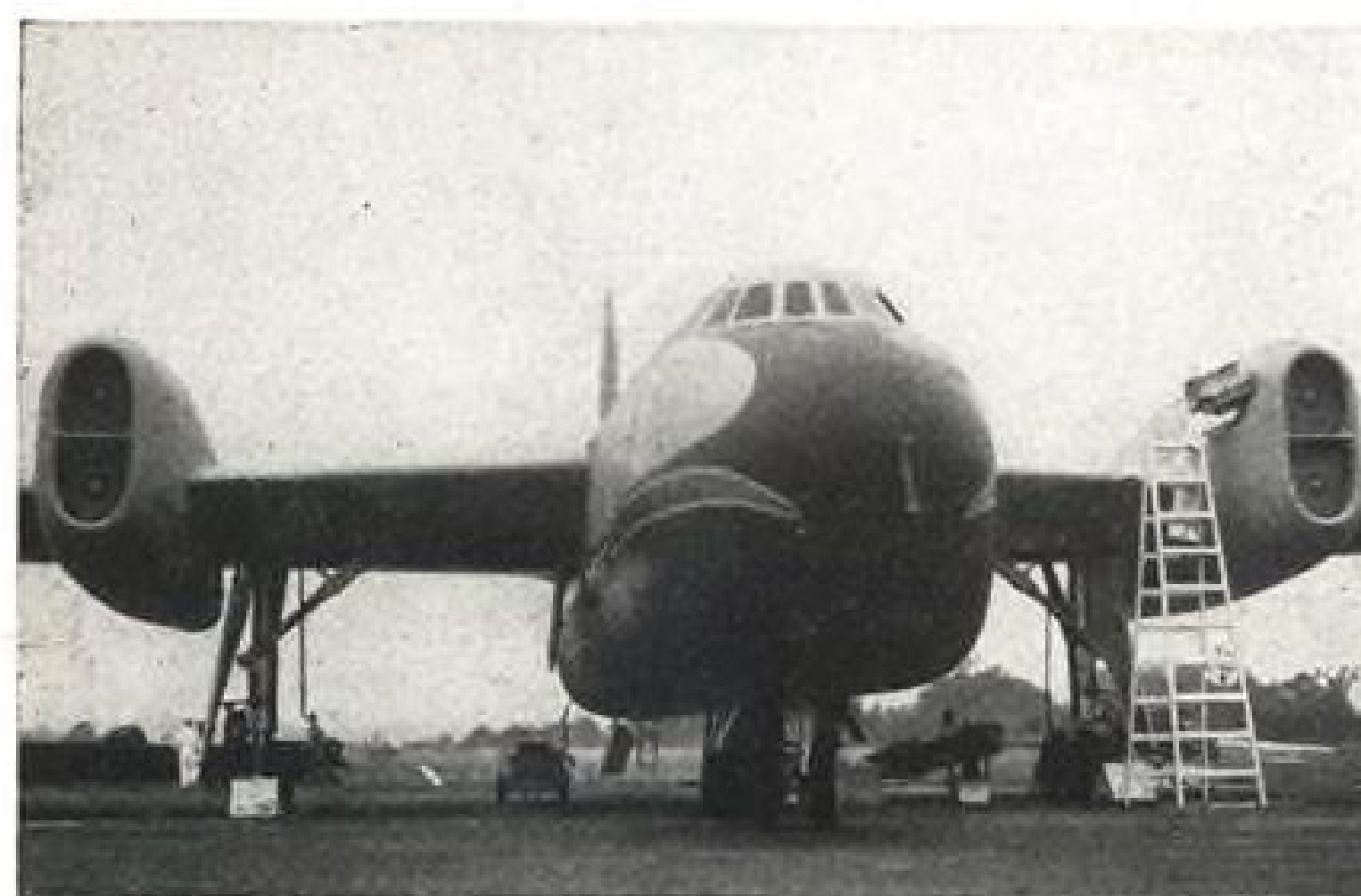
SHORT S.A.4 four-jet bomber shows double engine nacelles, each having two Avons. Note deep fuselage and four-wheel landing gear.
