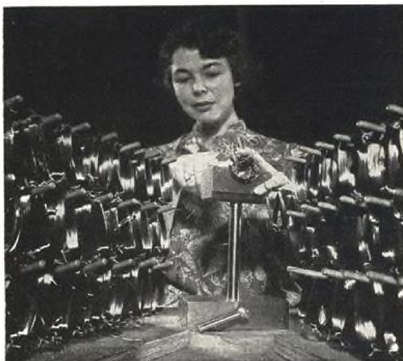
COILS FOR TACHOMETER GENERATORS are prewound and inserted in stator slots. They are specially formed and inserted to withstand extreme environmental conditions and excessive vibration.
