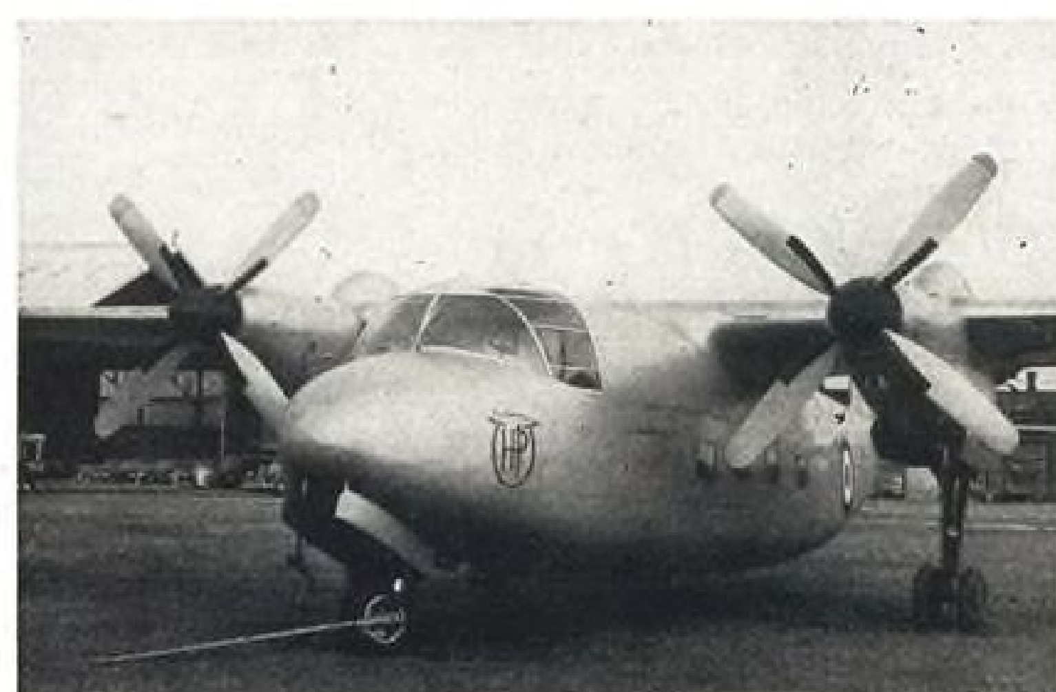
HANDLEY PAGE MARATHON II transport in closeup displays new de Havilland four-blade reversible pitch props.
