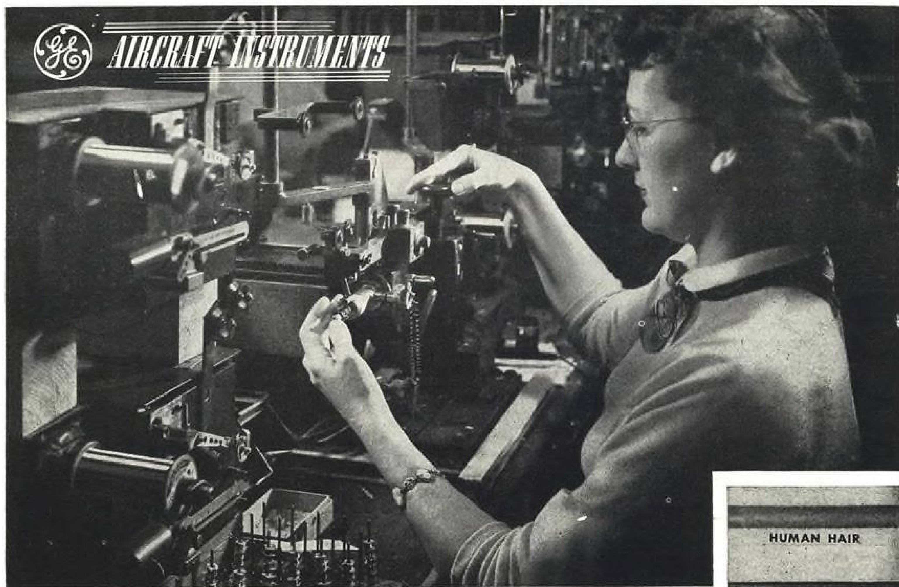
OPERATOR WINDS POSITION-INDICATOR COILS—WIRE FEEDS AT 600 RPM AROUND SQUARE COIL FORMS.
