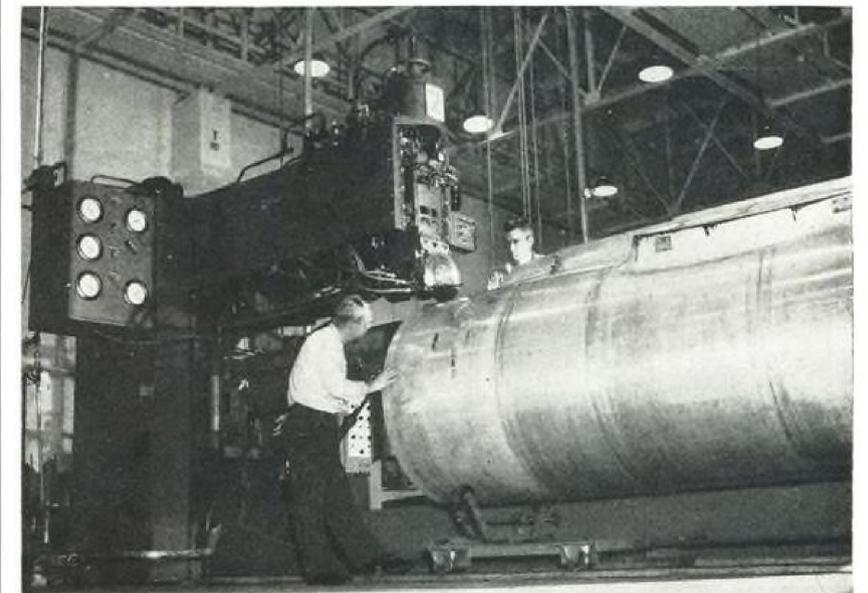
HUGE WELDER with 60-in throat easily handles giant external fuel tank.
