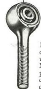
Fafnir Ball Bearing Rod Ends, one of the Fafnir Ball Bearing units regularly specified by Northwest Airlines. Light, compact design . . . outer race ground directly on shank member. Special heat treatment, an exclusive Fafnir feature, insures shank toughness — eliminates brittleness and cracking. Inner race extension beyond face obviates need of spacers.
