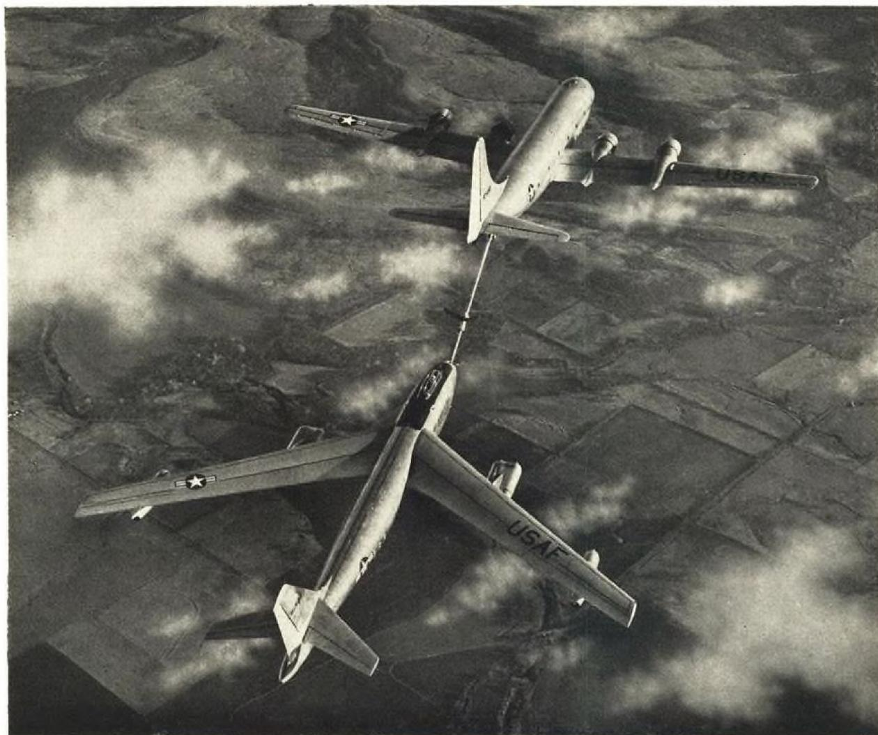
Fuel is pumped through "flying boom" into Stratojet from Stratofreighter tanker plane at high altitude.
