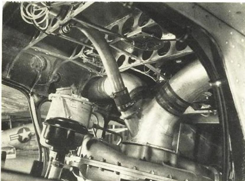
BLOWER leading air from wing ducts is compressor stage of B-29 supercharger.
