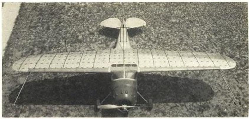
WOOL TUFTS on wing "paint picture" of air flow, which camera records.
