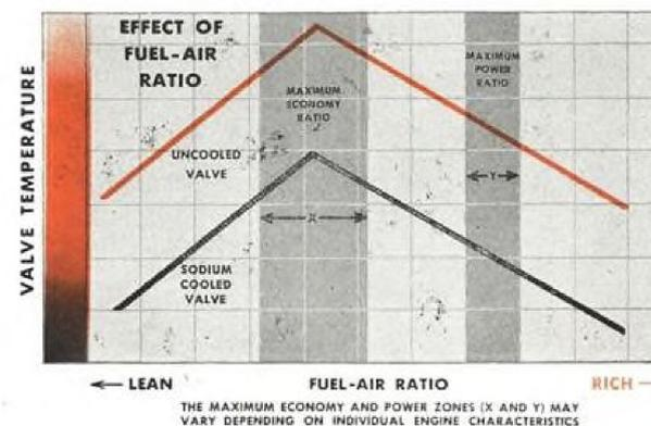
The trend in modern engine operation is toward higher speeds and more economical fuel-air ratios, resulting in higher temperatures for many operating parts.
