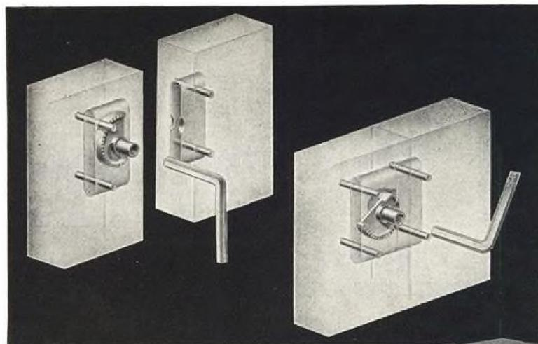
Serrated, tapered cam in male component engages lip of female. Panels are drawn tightly together when cam is turned by hex wrench, screwdriver, or any hand tool.
