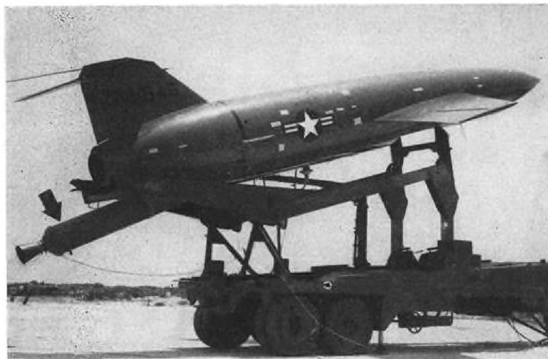
MARTIN MATADOR AF's B-61 missile, is poised on truck launching cradle. Weapon is about 30 ft. long, has thin swept wing. Basic power is supplied by Allison jet, but initial push is by RATO unit (arrow) as . . .
