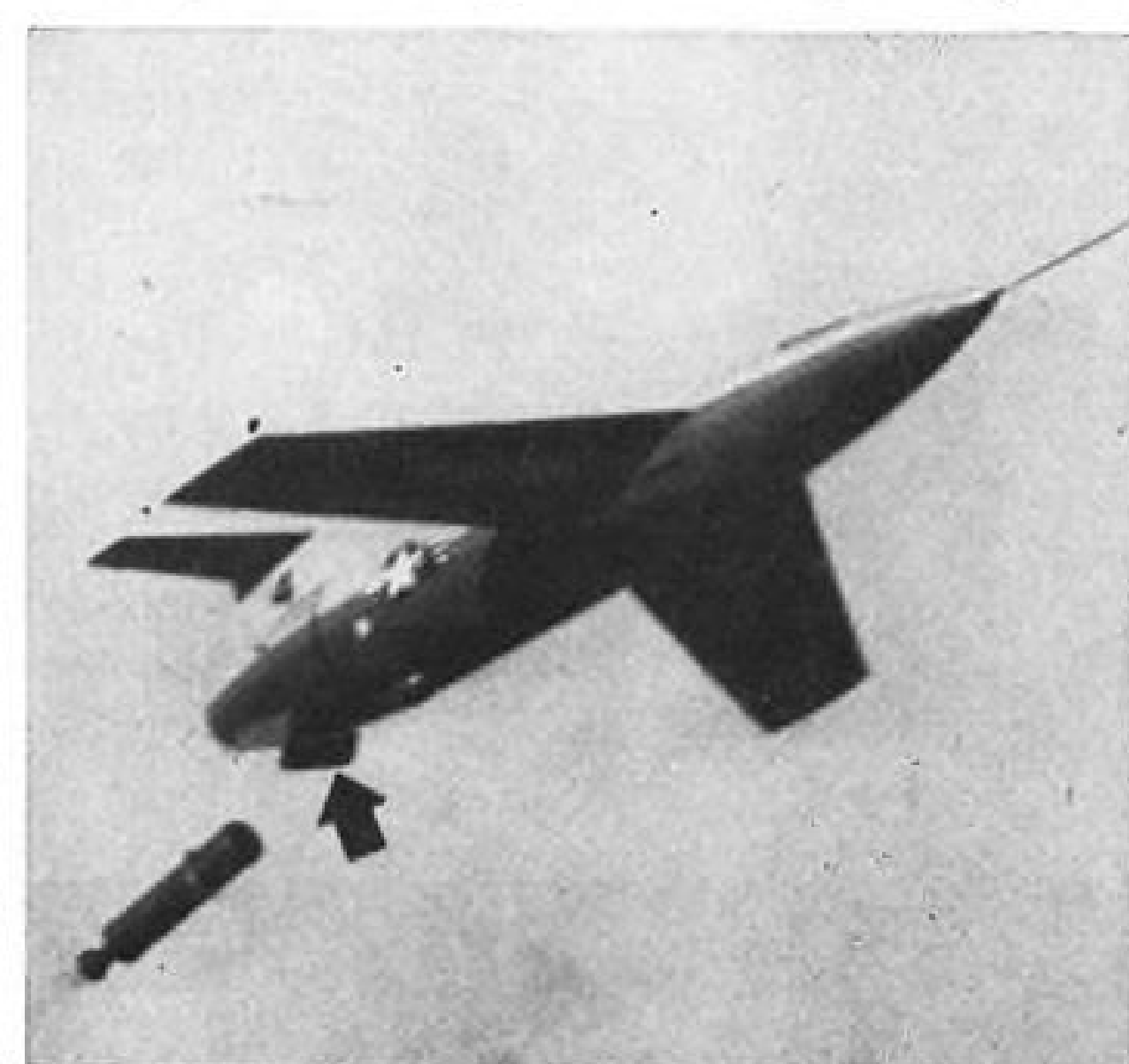
ROCKET FALLS away, with fairing doors (arrow) beginning to close and turbojet taking over.
