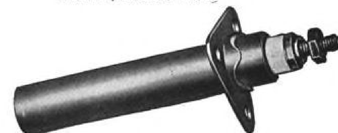
FIRE AND OVER-HEAT DETECTOR. 17343-11 Range +300°F to +1000°F. Fixed setting, non-adjustable, factory set. Hermetically sealed.
