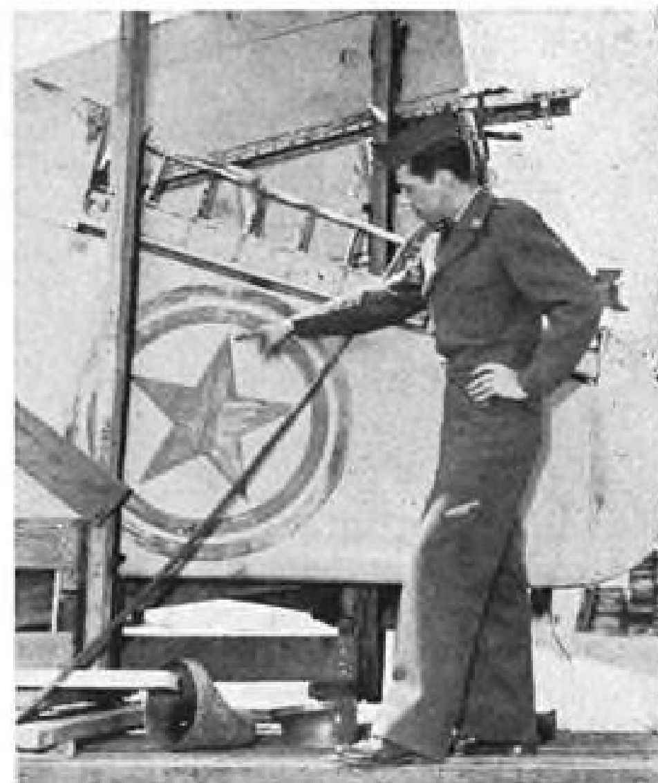
WING SECTION of a YAK-11 shot down over Korea is inspected. Although only a trainer gun mounts were provided in plane.
