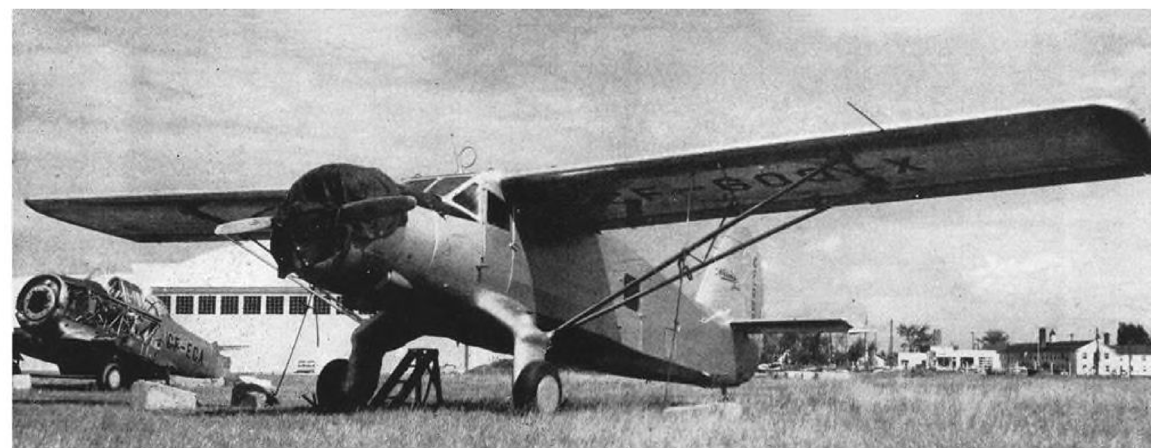
REVAMPED NORSEMAN —Being tested by Canadian Car & Foundry at Cartierville, Montreal, is new Norseman Mk. VII, which differs from earlier models by having longer, flat-sided fuselage and all-metal wings. Cabin access door has been moved aft.
