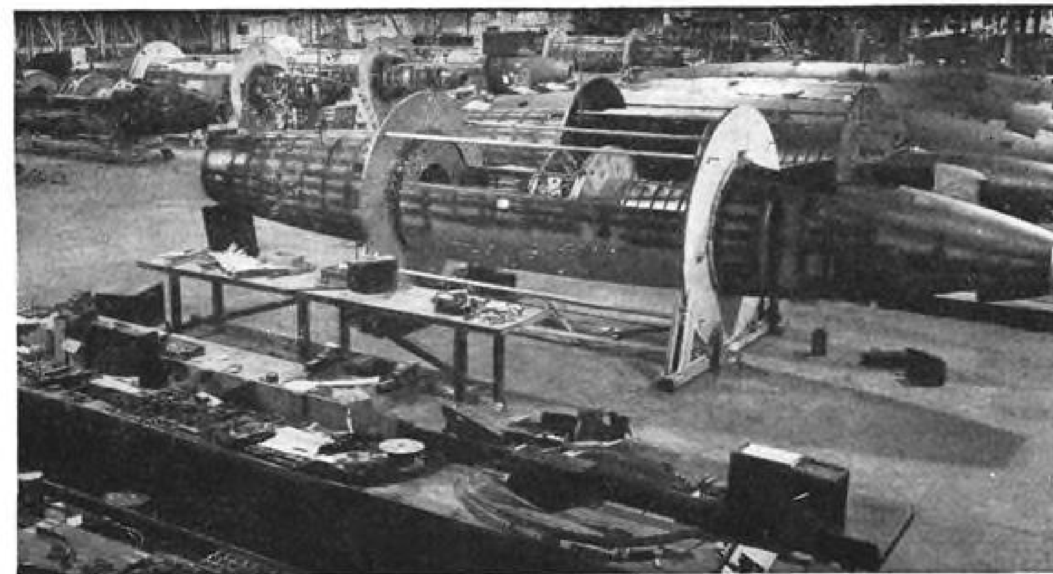
REVOLVING jig is used for fuselage work after main components are assembled.
