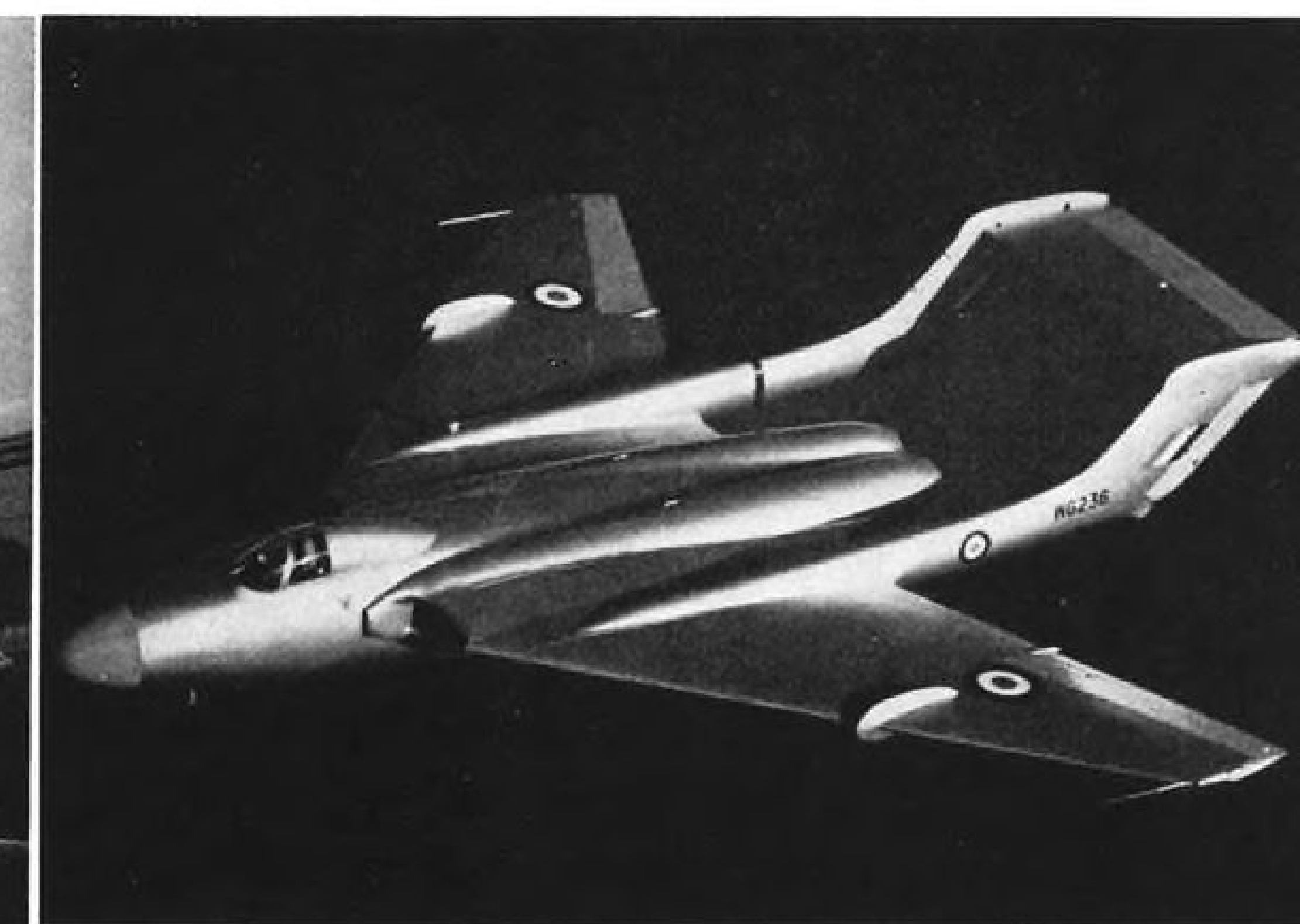
NEW DH NIGHTBIRD —First flight view of the new DH 110 multi-seat, twin-jet (2 Rolls-Royce Avons) night-fighter highlights craft's swept surfaces, close grouping of powerplants. Note very high stabilizer-elevator placement.
