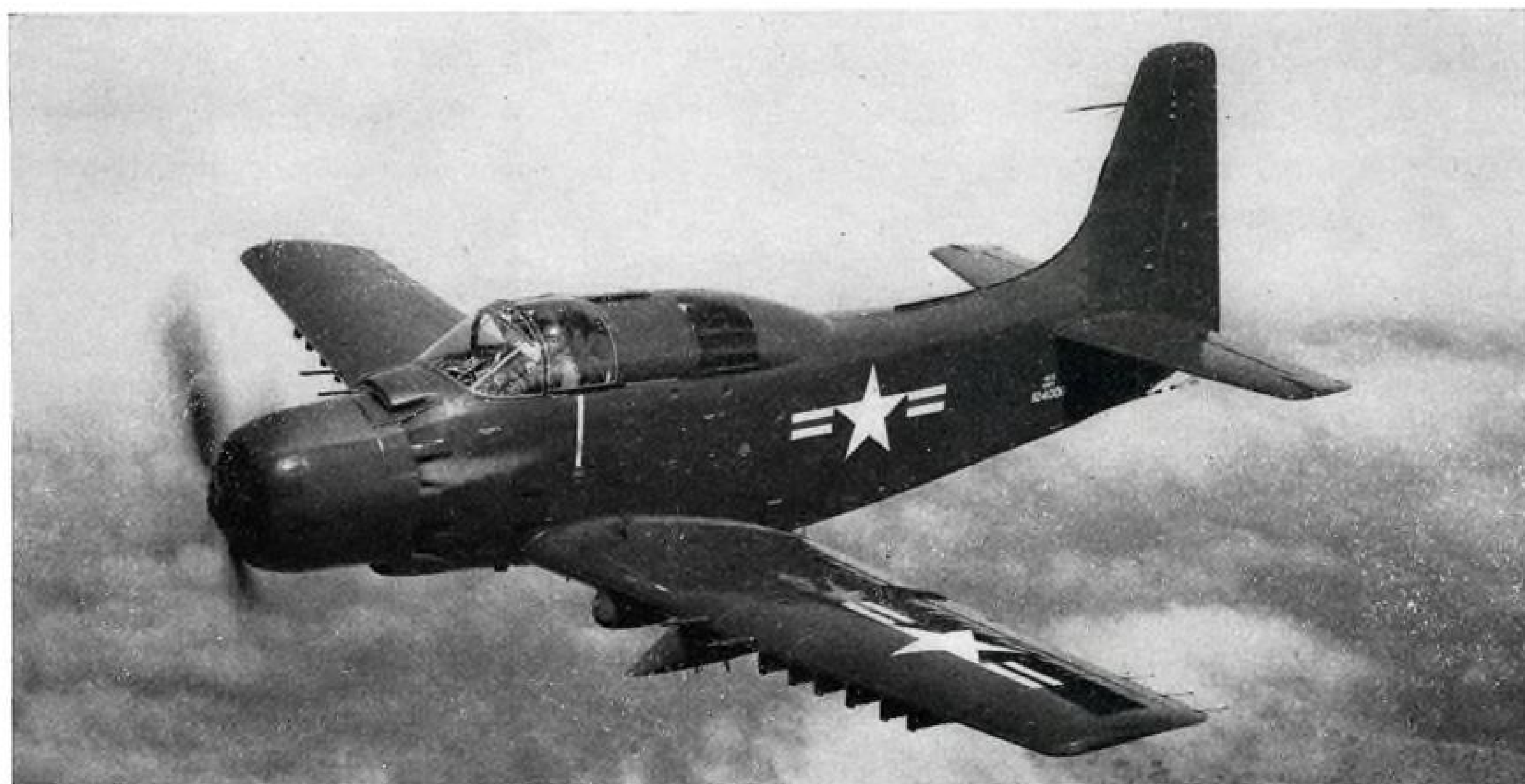
DOUGLAS AD-5 SKYRAIDER has been engineered as a one-plane air force, conversion kits adapting the basic structure to many duties.
