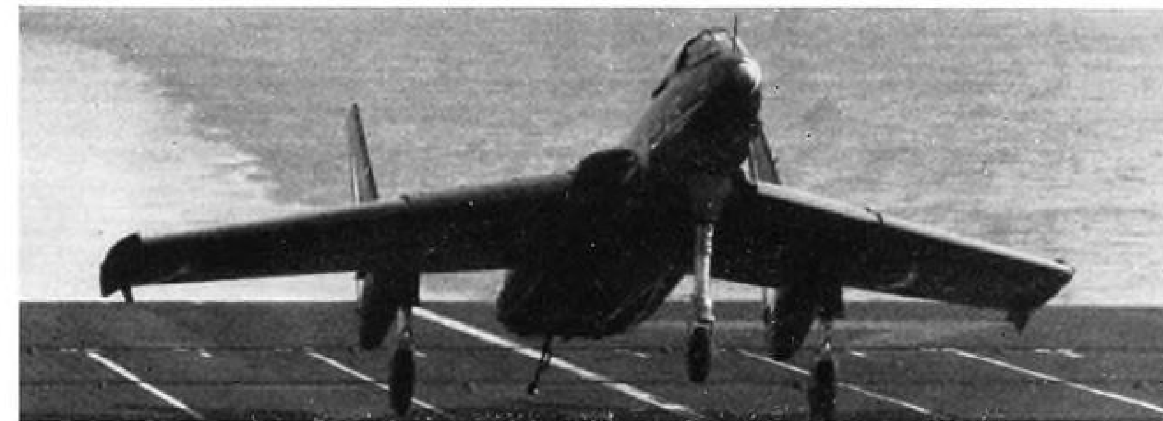
CUTLASS SCORES TOUCHDOWN—Still nose-high, a Patuxent-based Vought F7U-1 Cutlass (left) twin-jet Navy fighter drops onto the deck of the USS Midway during carrier evaluation trials, its hook picking up an arresting wire early in the landing (the 31,540th landing on the big CVB carrier). The novel, 700-mph.-class F7U is now in production for service use, has two Westinghouse J-34s fitted with afterburners for extra speed during combat and in emergencies.
