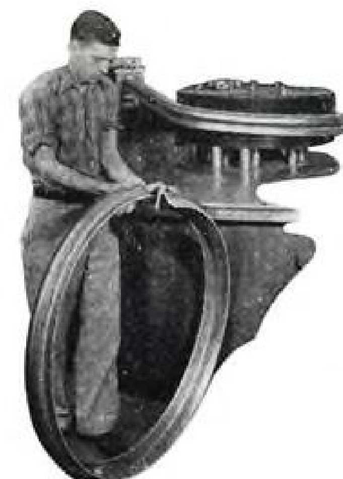
Aluminum gun turret rings accurately formed to complete circle for various aircraft.
