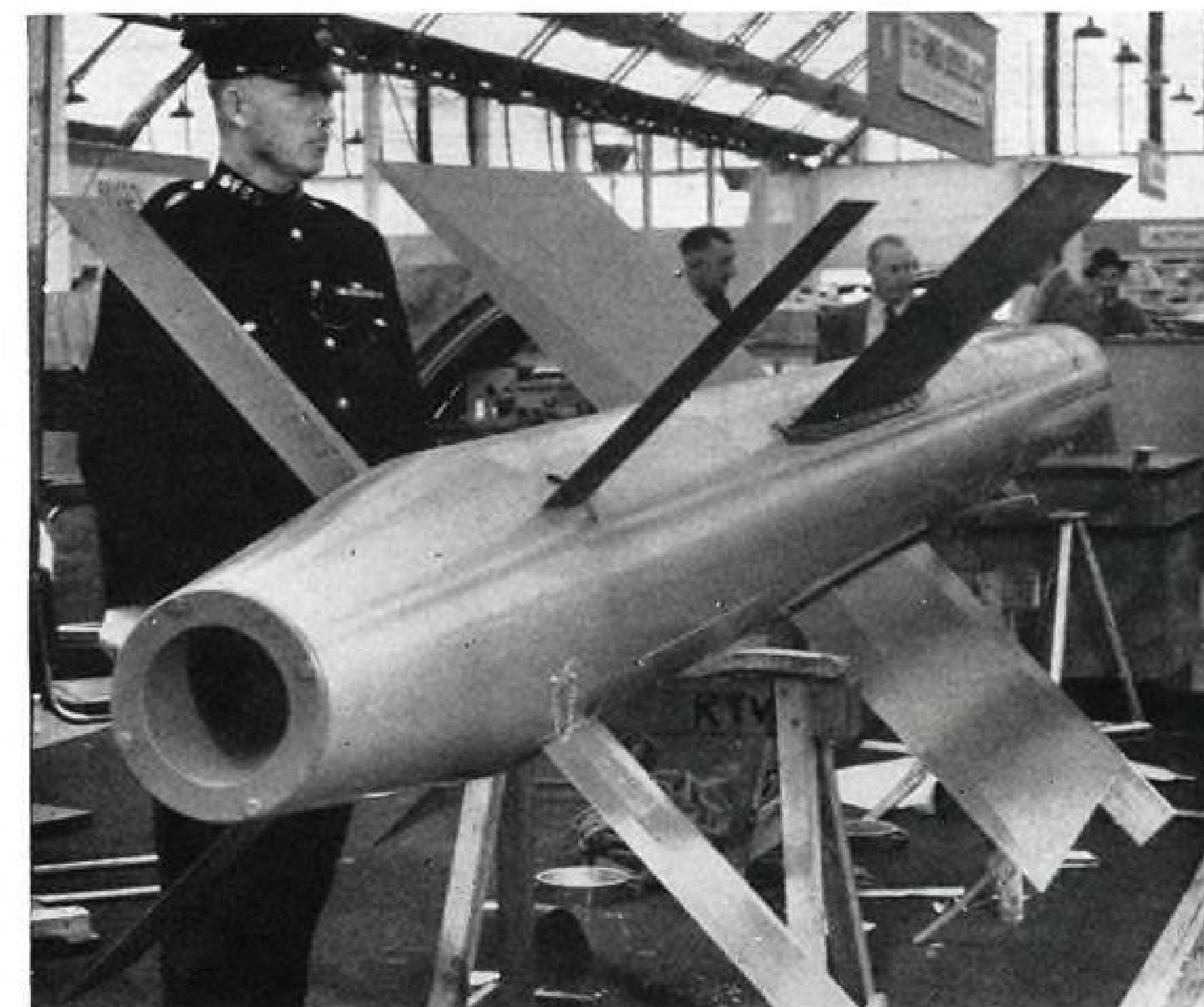
RAE RESEARCH ROCKET mounts four fixed wings and four movable tail surfaces.
