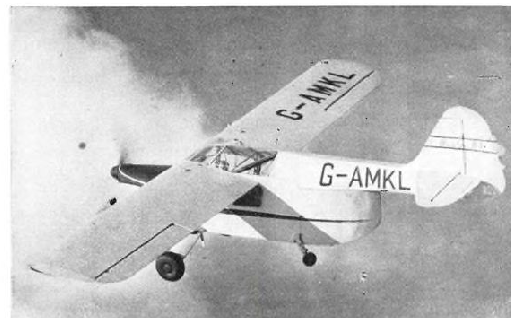
FLIGHT view of Auster B4 shows cargo area in boom-and-pod fuselage, featuring . . .
