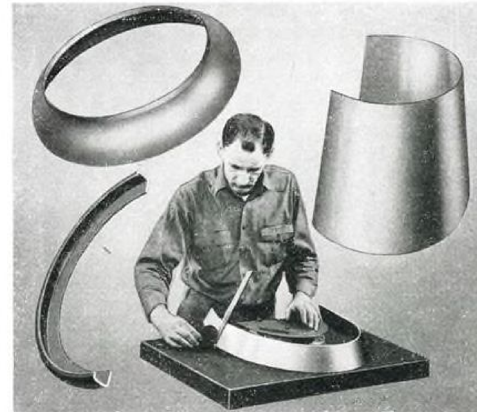
Above: Jet flange rings, shrouds, cases, flame tubes, stiffeners and casings are formed in either full circles or segments.
