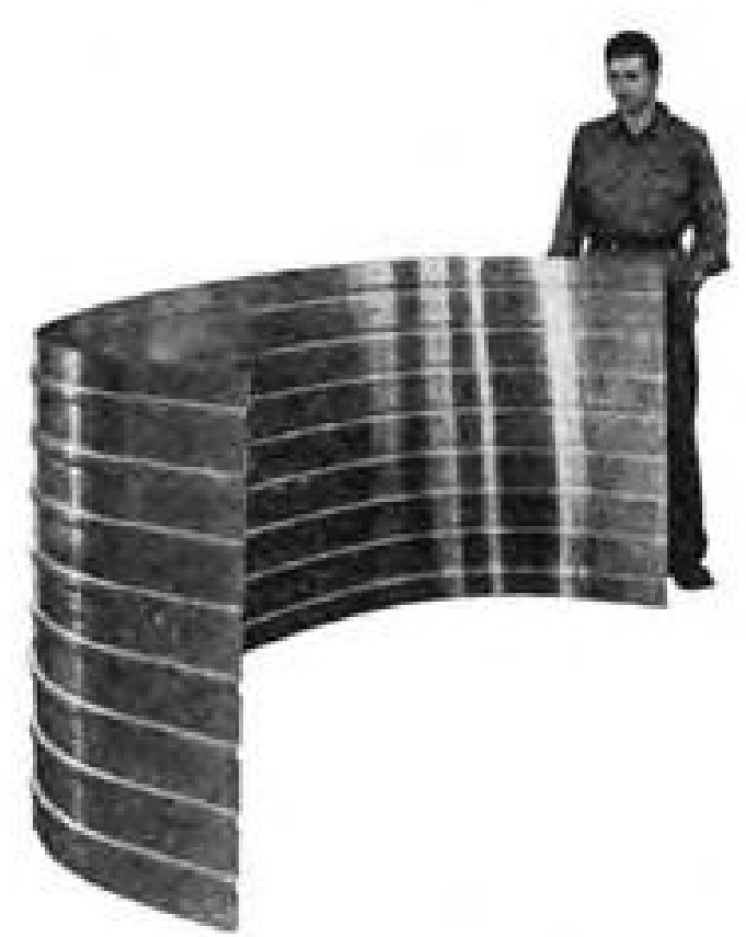
Large corrugated aluminum sheets accurately formed on the BATH machine.
