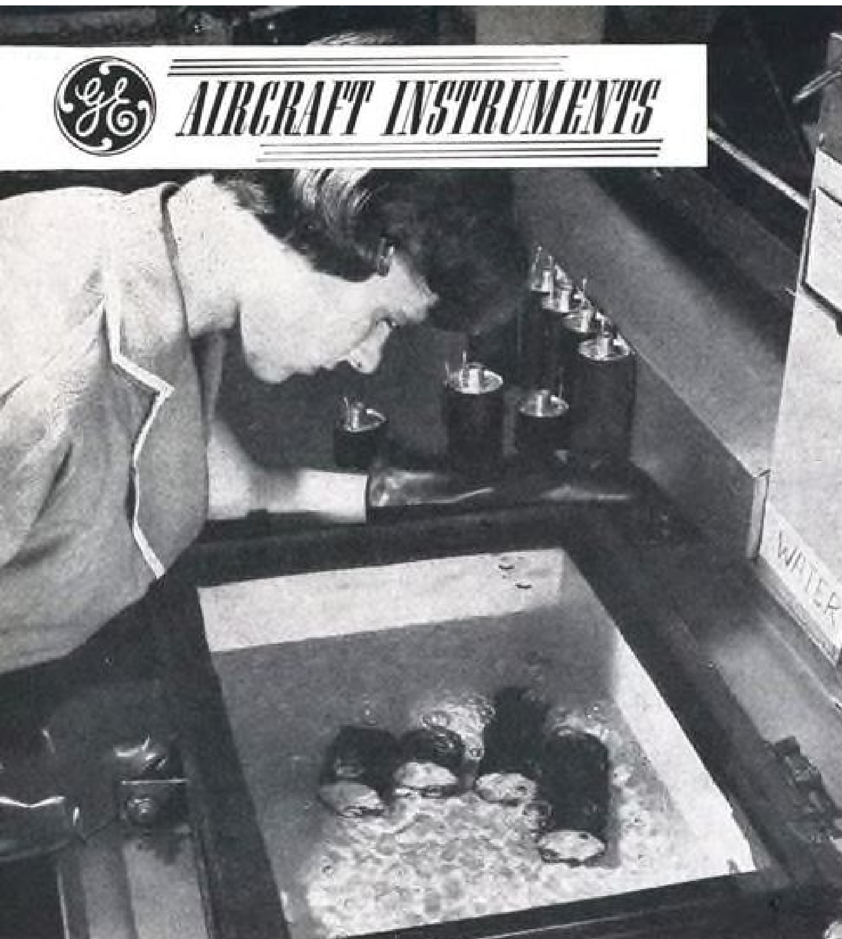
INSPECTION FOR LEAKS is done in a vacuum test bath after the air bubbles caught on the instruments are boiled off at 29" vacuum.
