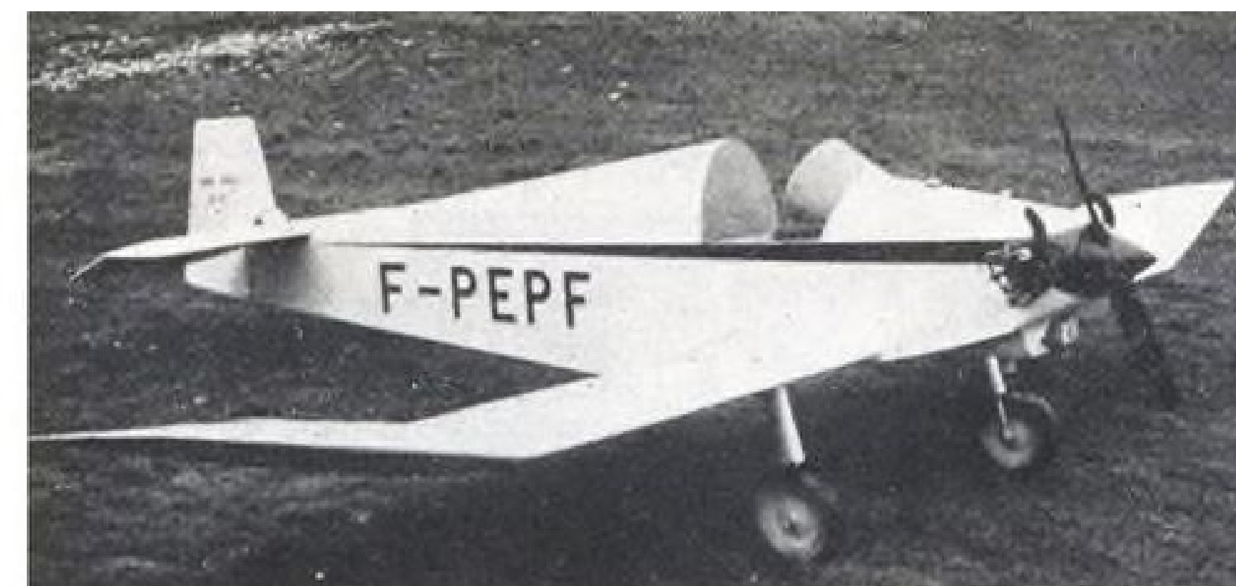
FRENCH ULTRA LIGHTS —Trim lightplanes above, the D.9 (left) and the D.111 (right) are products of Avions Jodel. Single-seat D.9 has 34-hp. ABC Scorpion, weighs 594 lb. gross; later, two-place D.111 has 75-hp. Minie. Both are designed to be built from kits.
