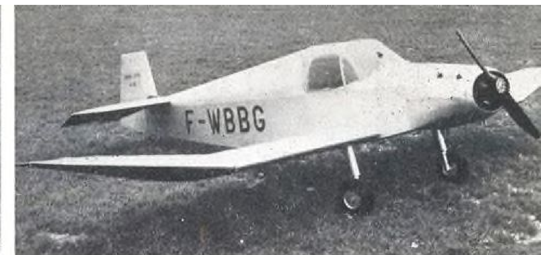
FRENCH ULTRA LIGHTS —Trim lightplanes above, the D.9 (left) and the D.111 (right) are products of Avions Jodel. Single-seat D.9 has 34-hp. ABC Scorpion, weighs 594 lb. gross; later, two-place D.111 has 75-hp. Minie. Both are designed to be built from kits.
