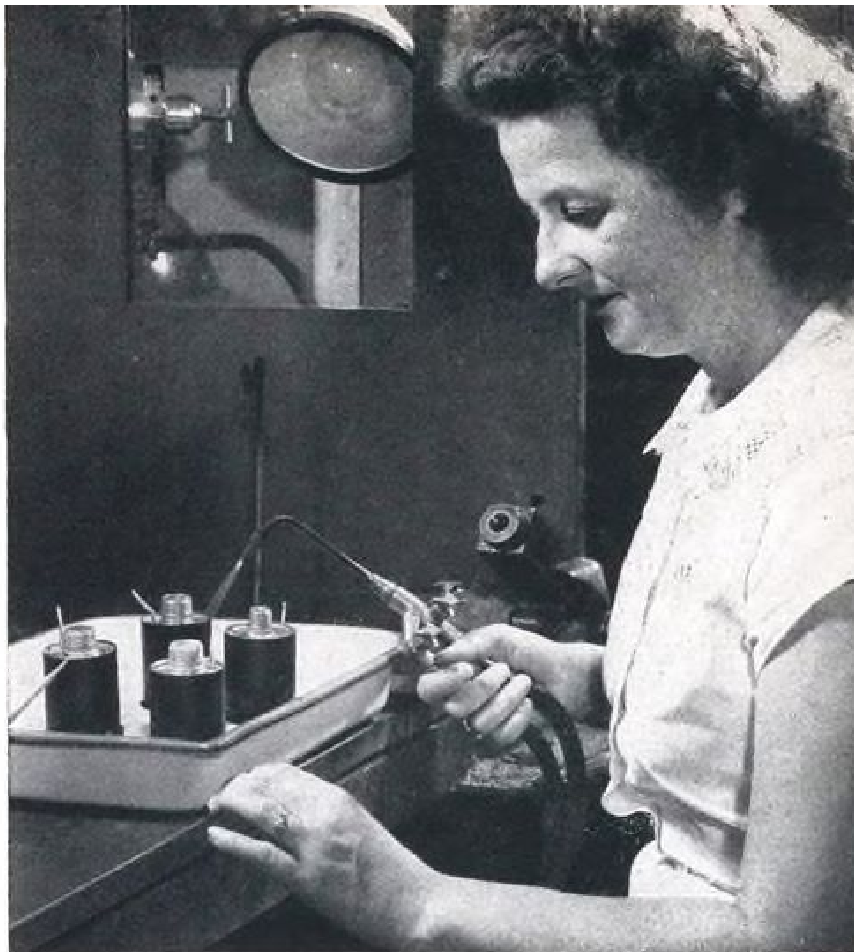
INSTRUMENT MECHANISM is flame soldered into the can. Even cooling is assured by keeping the instrument faces under water.
