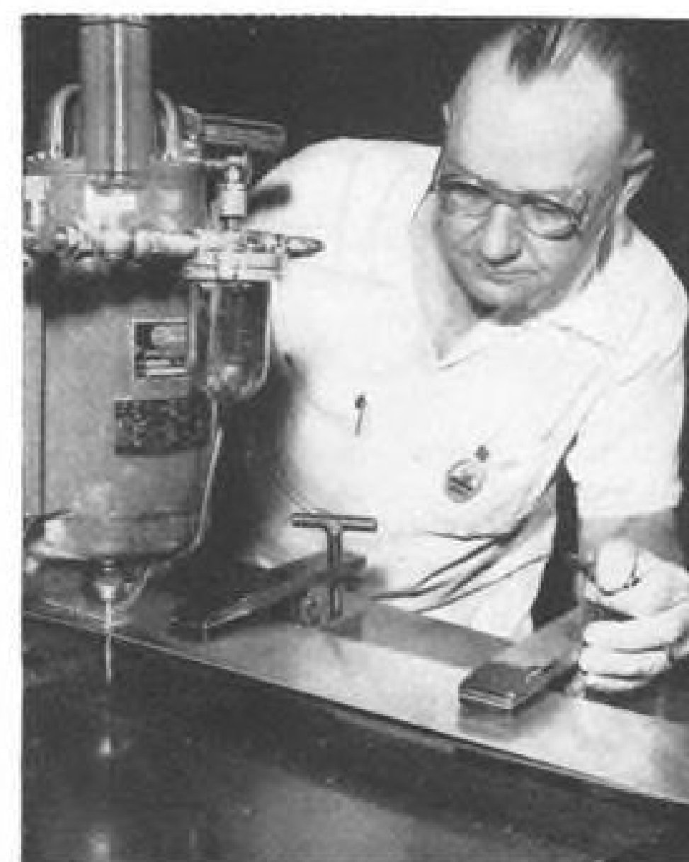
AIR pressure forces oil through tube to router head on this new router-oiler system.
