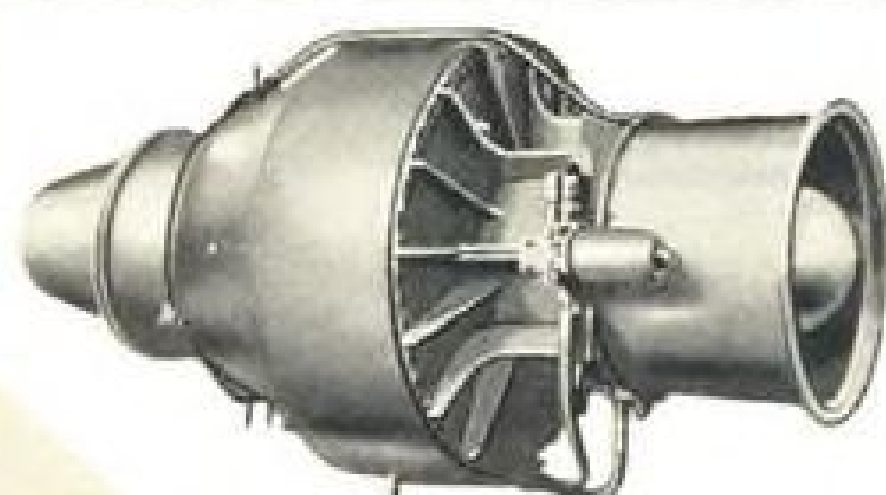
JET POWER for target and trainer aircraft or as booster power on bombers and transports. 300-900 lbs. thrust.
