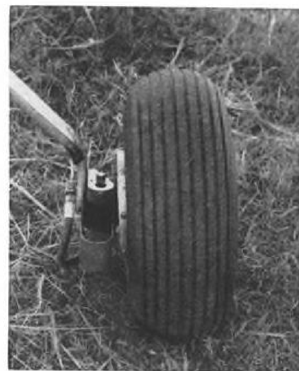
FRONT view of "barn-door hinge" swivelling device, with small spring in front of hinge to snap wheel back to regular tracking position for takeoff.
