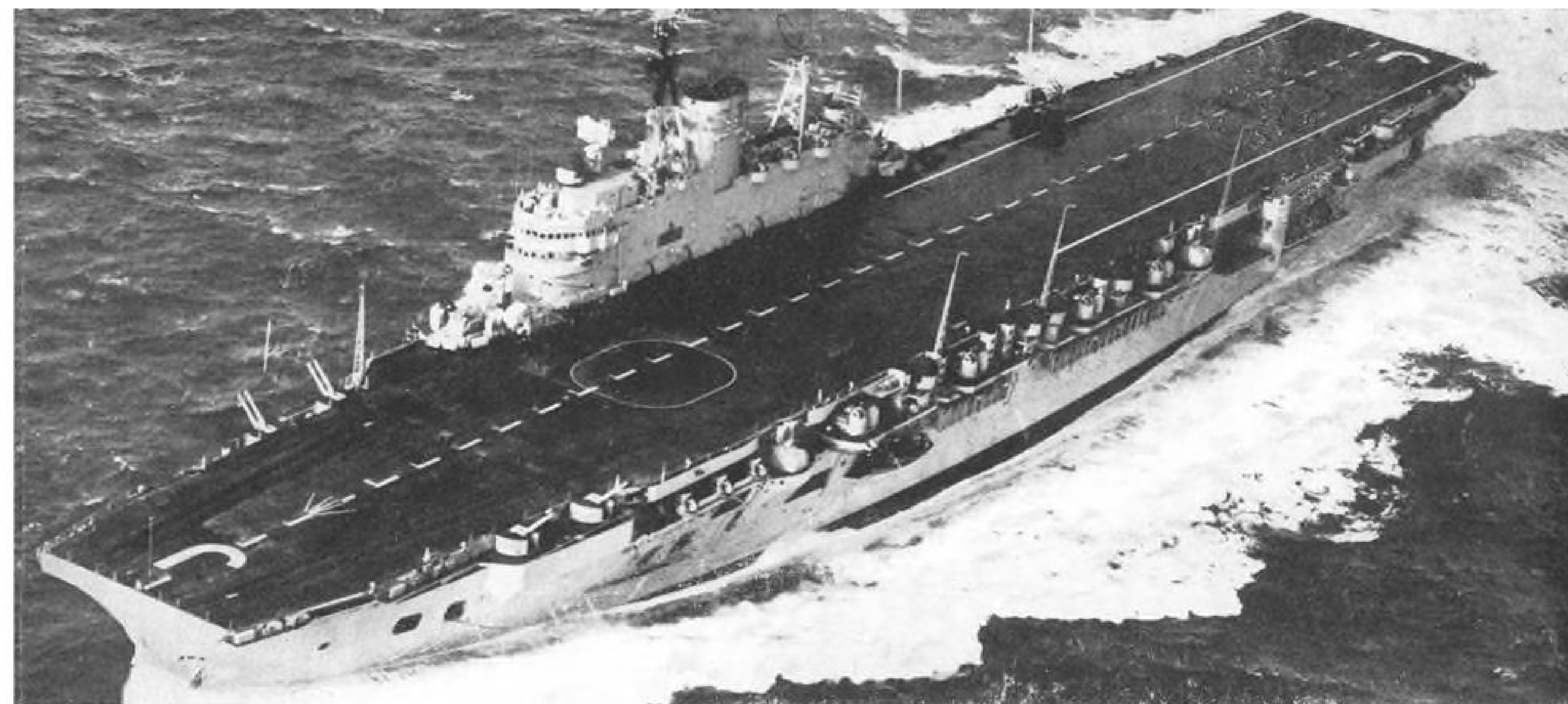
NEW ROYAL NAVY FLAT-TOP —HMS Eagle, big, new 800-ft. carrier for the Royal Navy, weighs 36,800 long tons and can carry 100 aircraft. Eagle roughly compares with U. S. Essex-class flat-tops. Royal Navy's present carrier strength is seven ships, plans call for 18.
