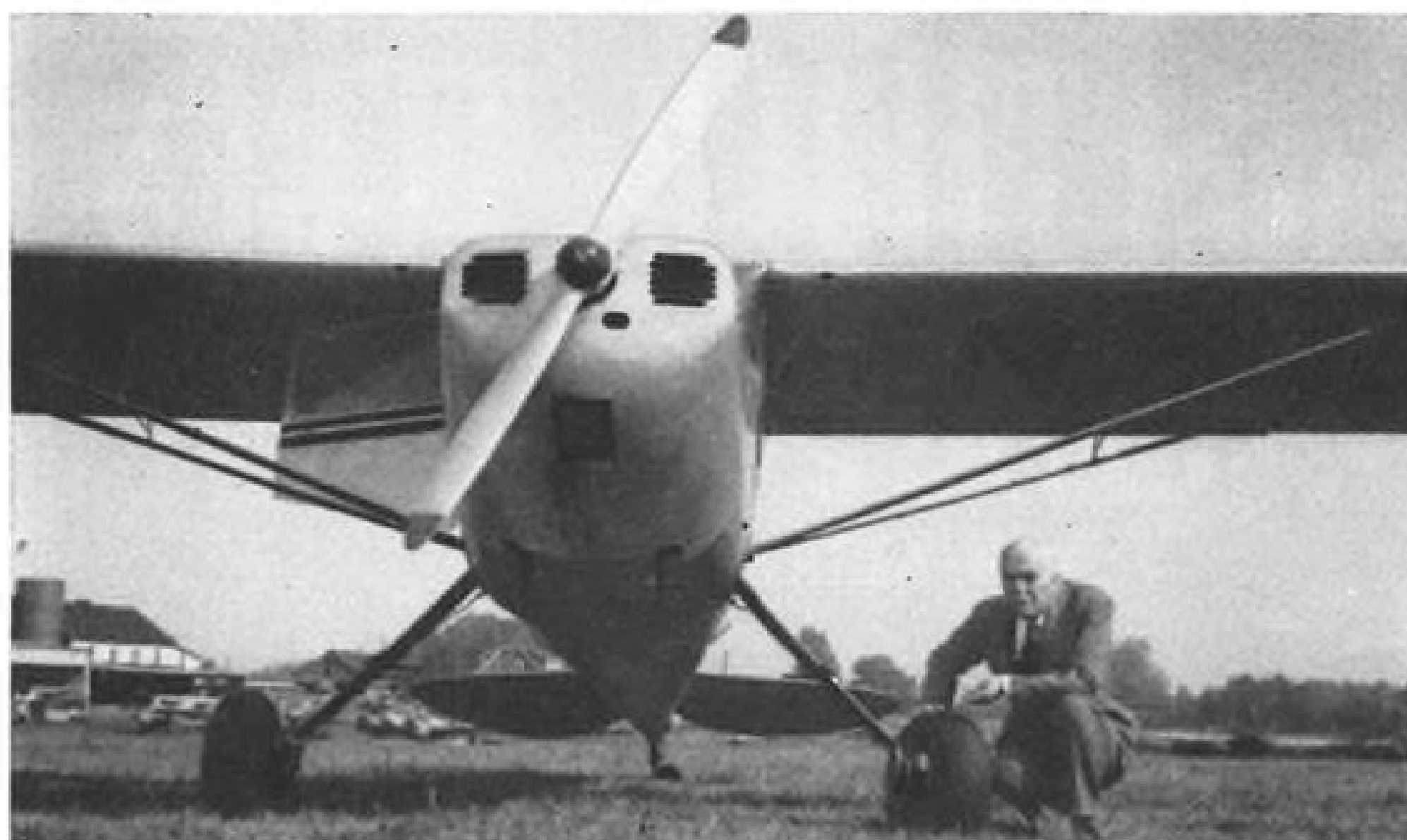
NEW crosswind gear on Cessna 140 is checked by John Geisse, developer. Note wheel at right turned at outward angle, can't turn inward.
