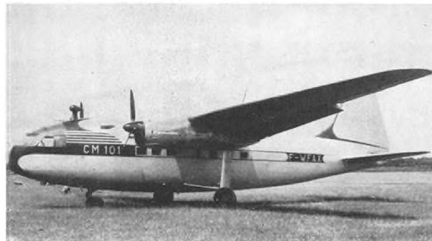
FOUGAS DUET —Two recent Fougas designs built in France for different purposes are the CM-101-R transport (left) and the Bemaux III light research plane (right). Former carries 14 passengers, has two 580-hp. Sncma piston engines and two auxiliary Turbomeca Pimene jets of 485-lb. thrust, arranged in tandem pairs in each engine nacelle. Gross weight is 18,982 lb., empty weight 13,825 lb. Gemeaux III is a two-place light plane with a single 740-lb.-thrust Turbomeca Marboire turbojet between the twin fuselages.
