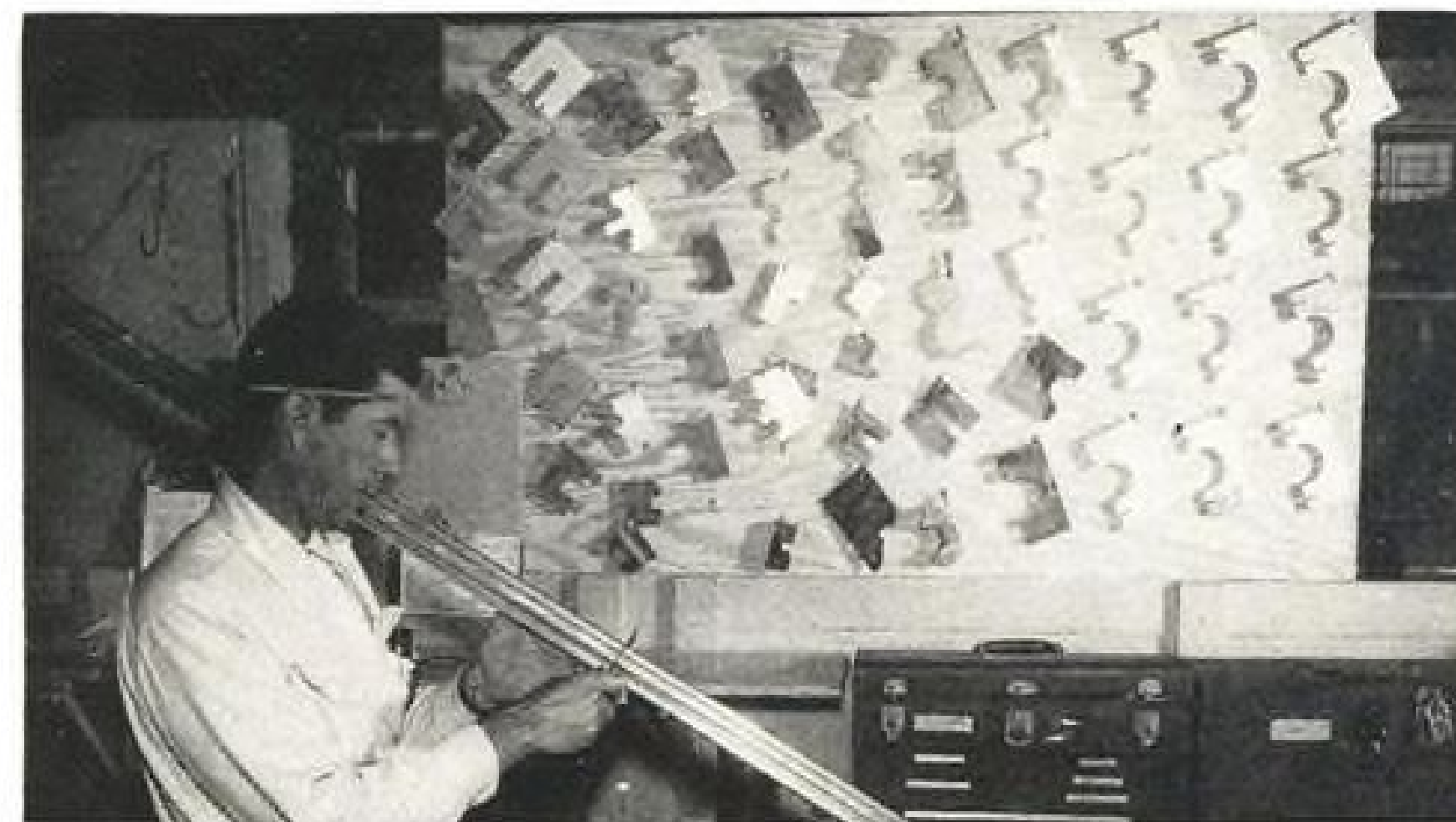
3 Checker who slides template along sample part to pass on dimensions and shape. From Yoder rolls, part goes for further treatment up . . .
