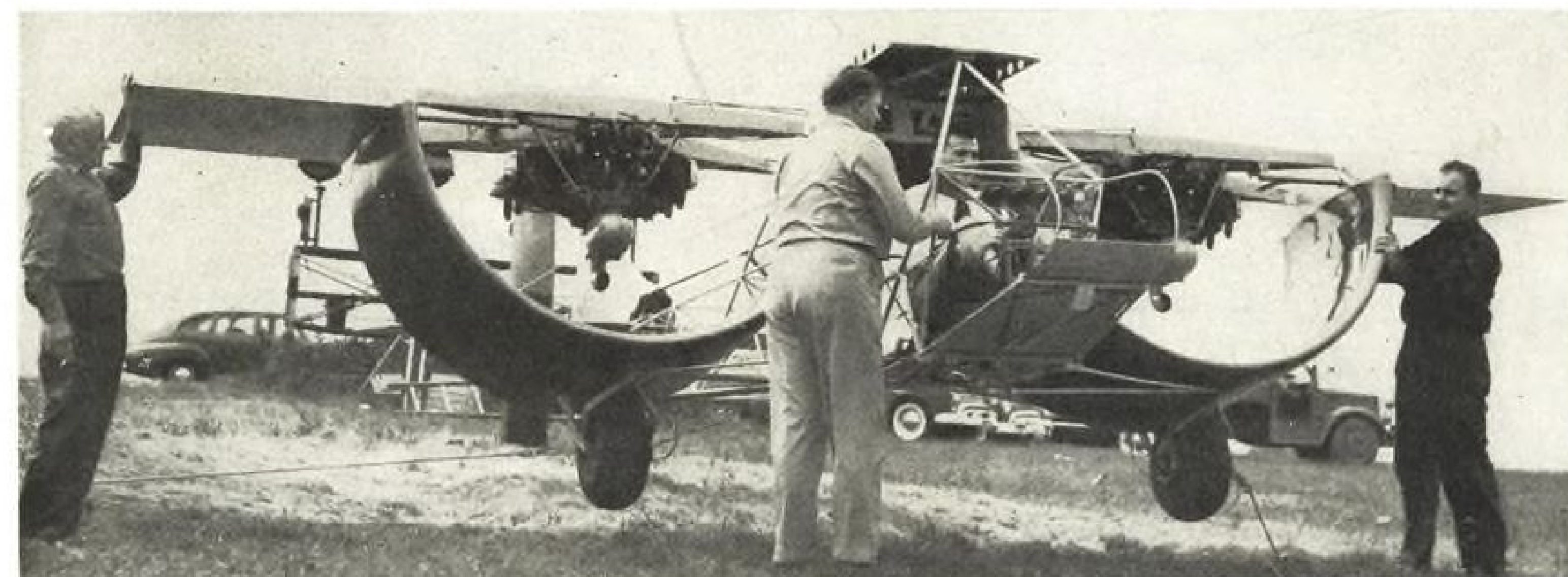
THROUGH CHANNELS, Custer's wing gets its lift. It rose off the ground when tethered, but there are still unanswered questions.
