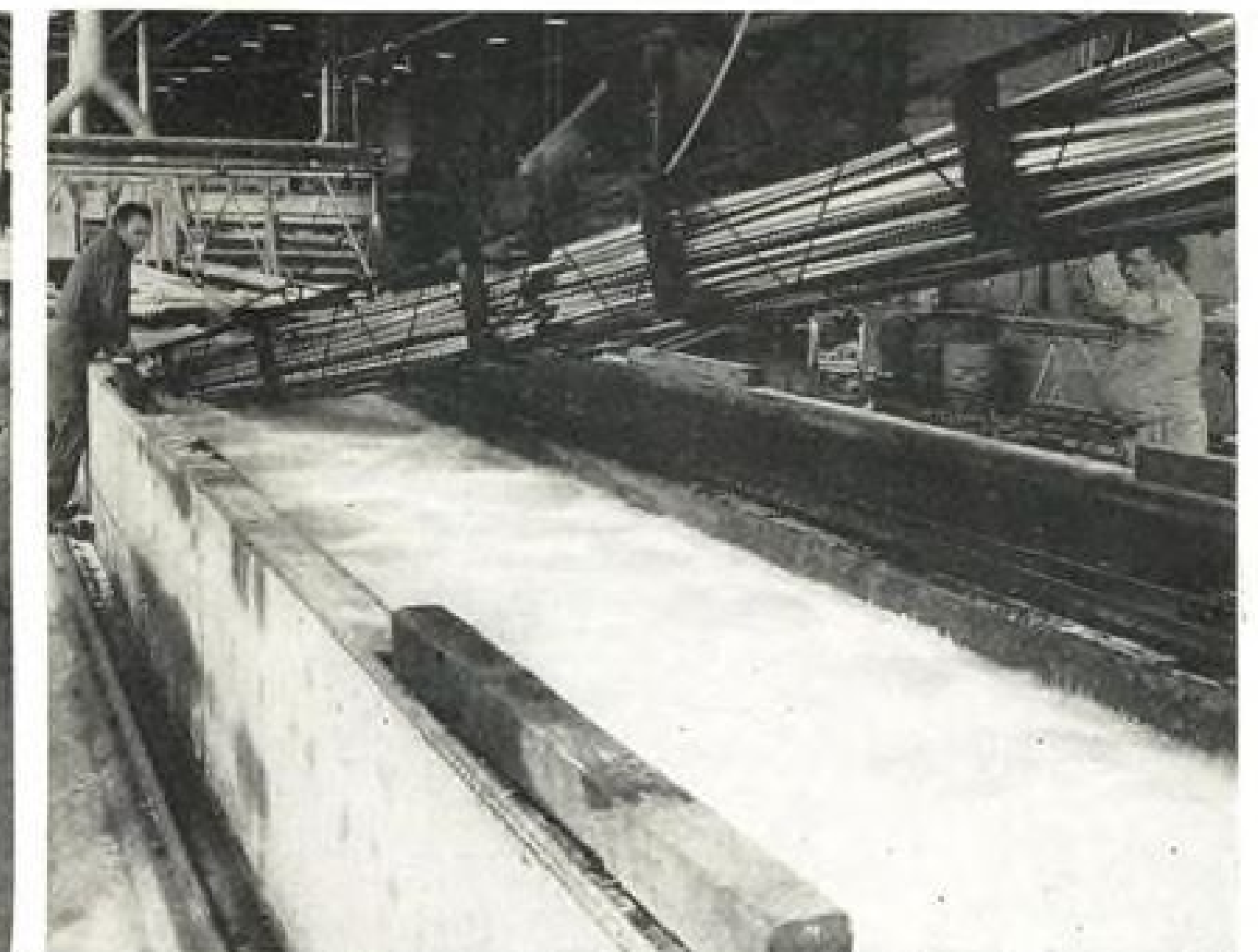
6 Quench and cleaning bath (nitrate tank abuts it, upper left rear). This takes but a few seconds. Next step is to . . .
