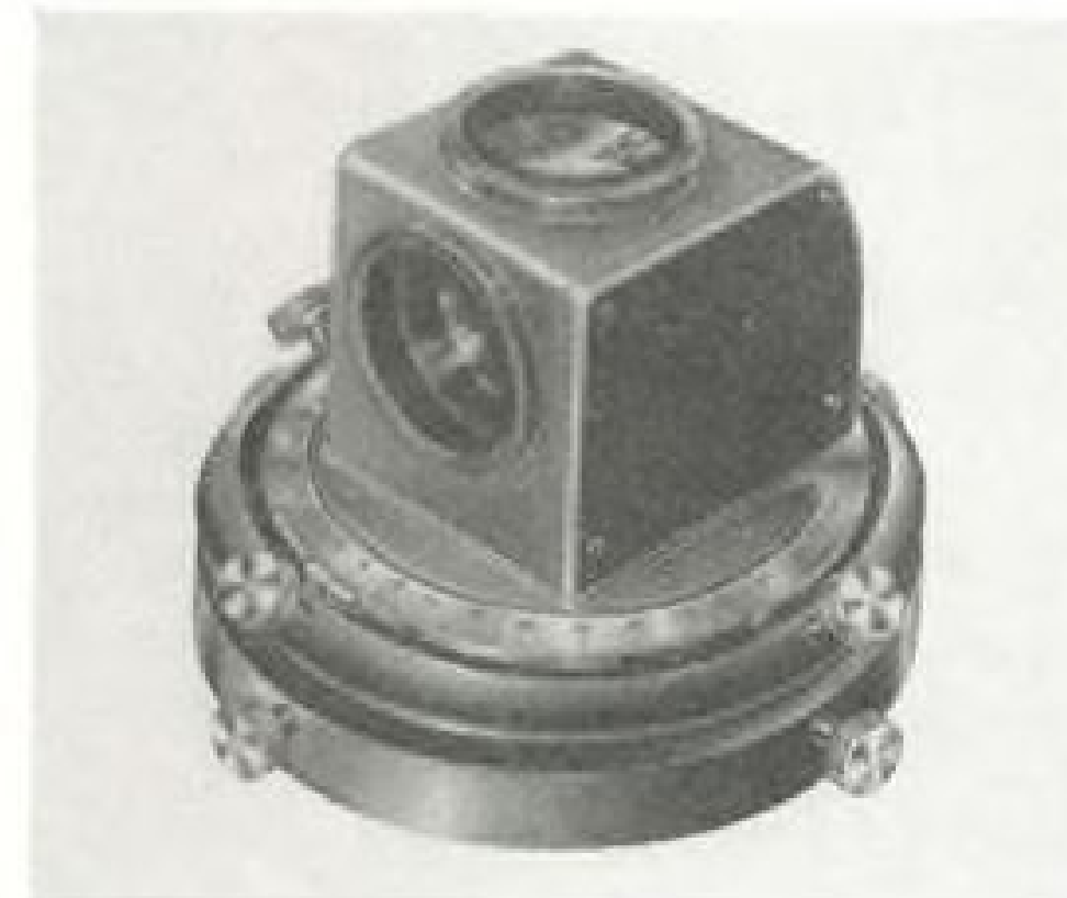
OPTICAL tooling alignment scope (top) has built-in autocollimating illuminator, and optical square (bottom) establishes plane at right angles to scope's line of sight, which were shown at Convair meeting.
