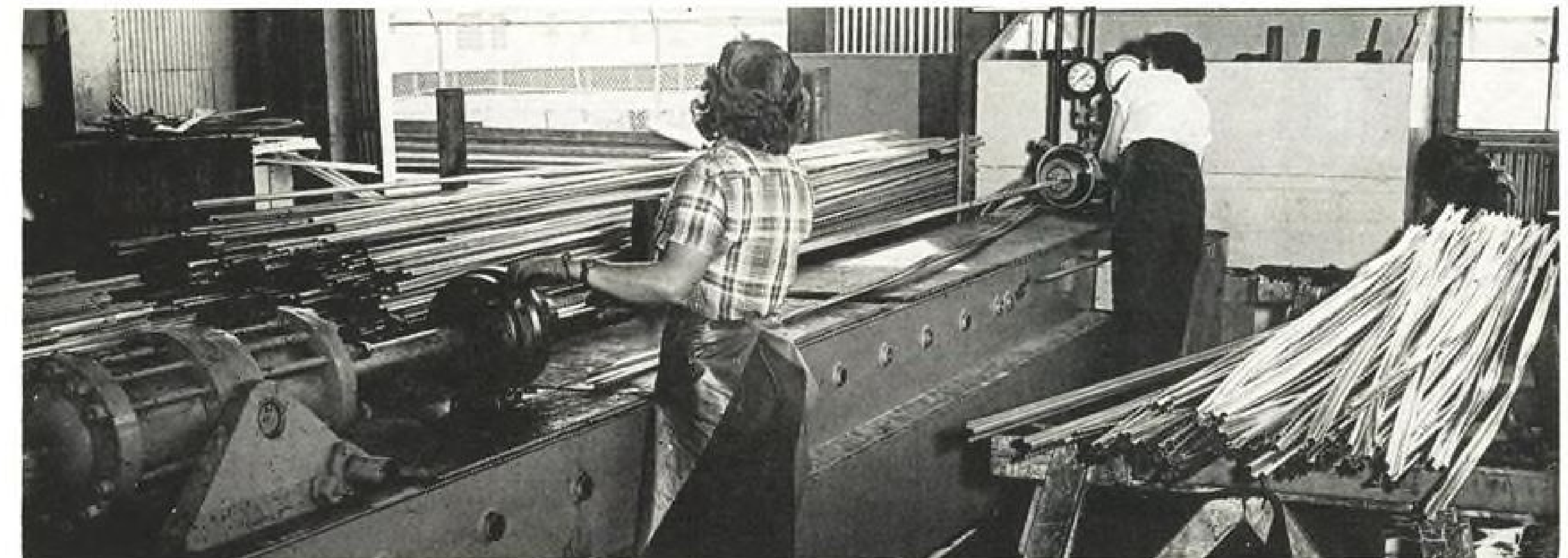
7 Hufford stretch-leveler, about 25 ft. from the quench bath. Kinked strips are pulled into straightness by the two jaws on the stretch-leveler. Occasionally strips which fall short of strength specifications fail during this process. Last stop is . . .
