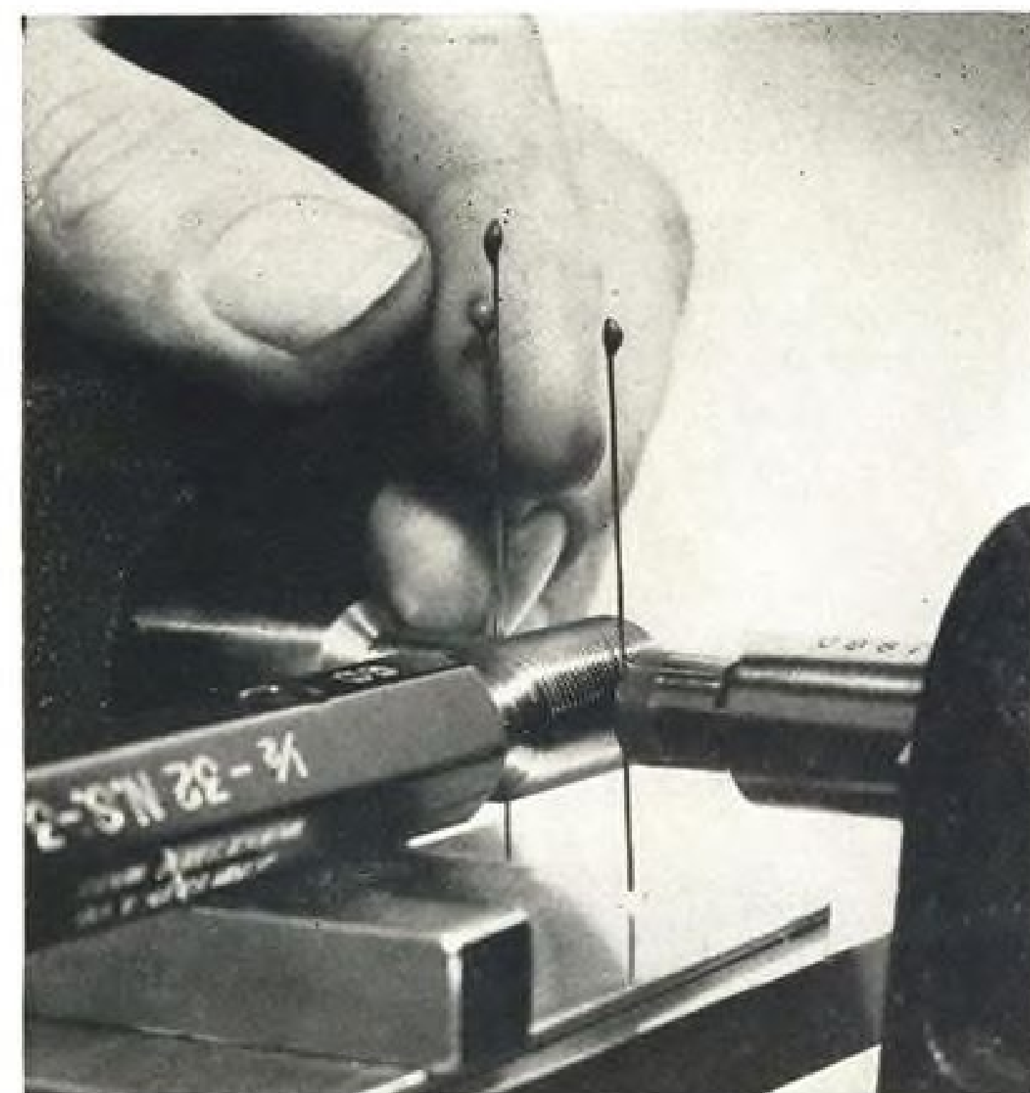
PLUG GAGE STANDARDS are checked every other day with this supermicrometer which measures to six decimal places—0.000010.
