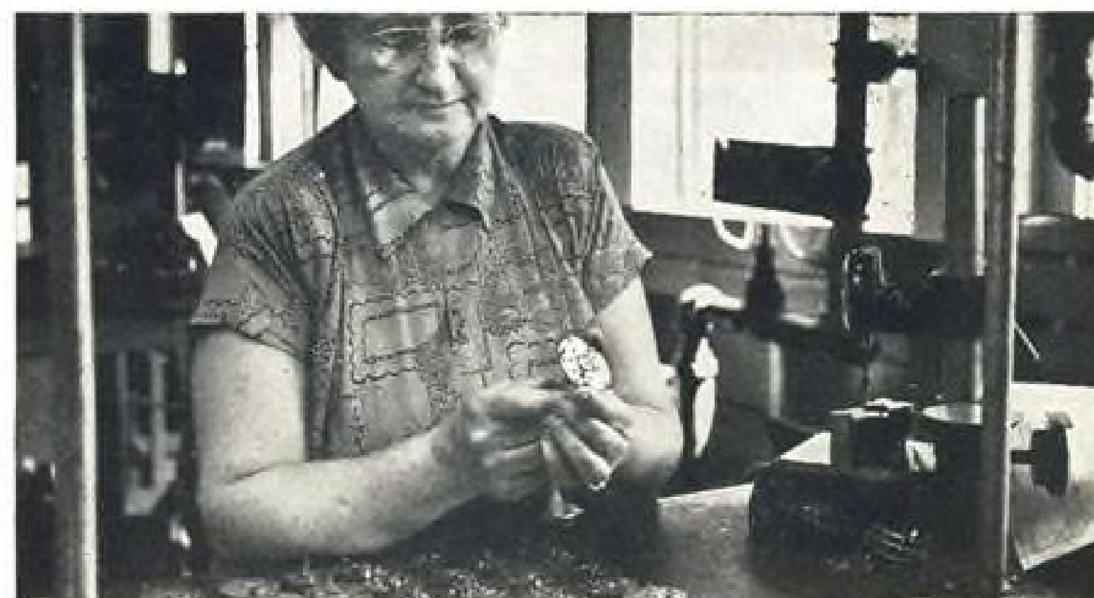
FINISHED PARTS are checked right on the assembly floor with plug gage standard pictured at left. Tolerances as close as 0.0001 in. are maintained.
