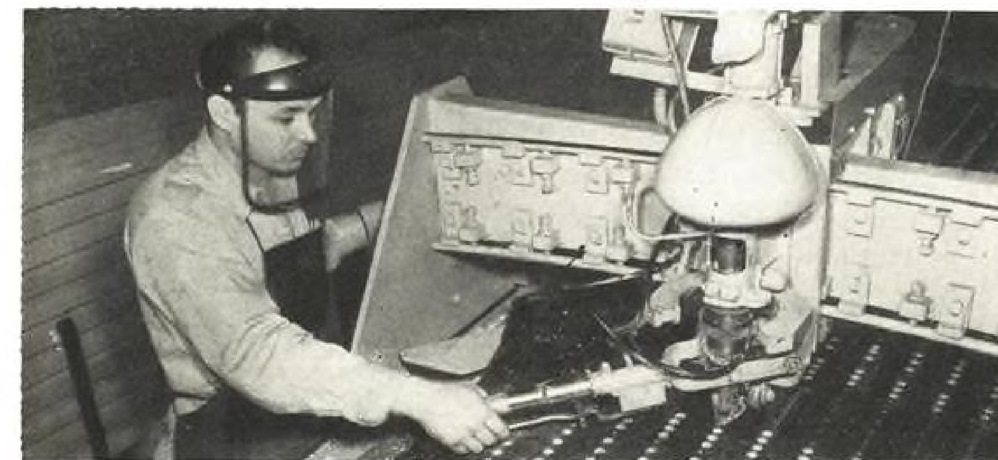
OLD METHOD of drilling rivet holes through the template, required . . .
