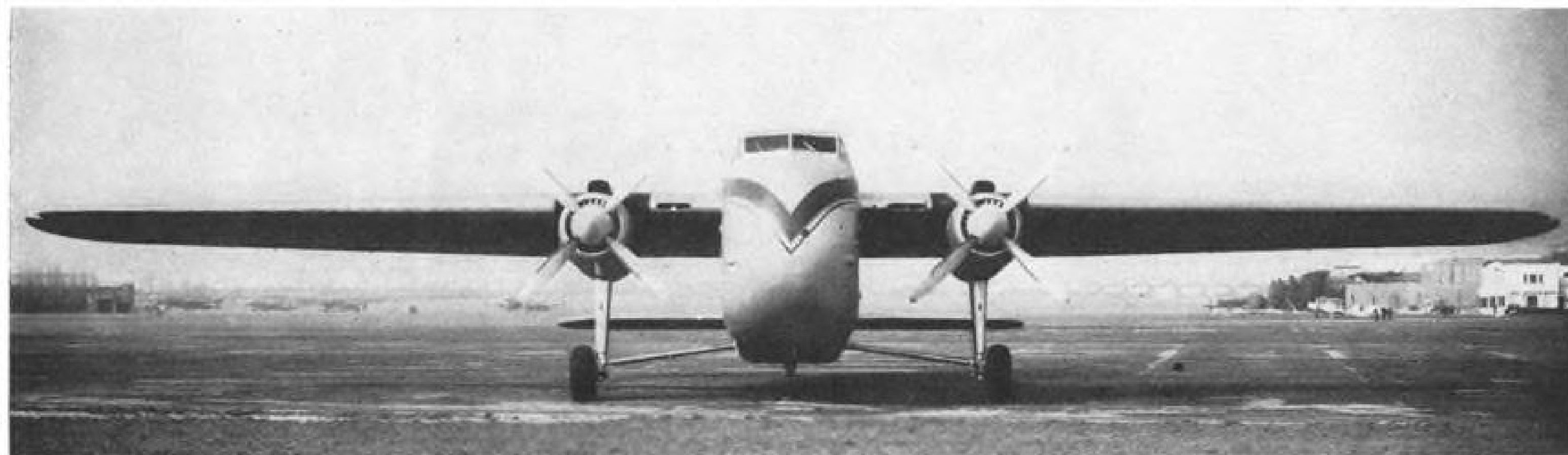
MEDIUM CARGO CARRIER is the Mk. 31 version of Bristol's Type 170 Freighter, with increased power from twin Hercules 734 powerplants. Fixed landing gear has been strengthened to handle increased gross weight.
