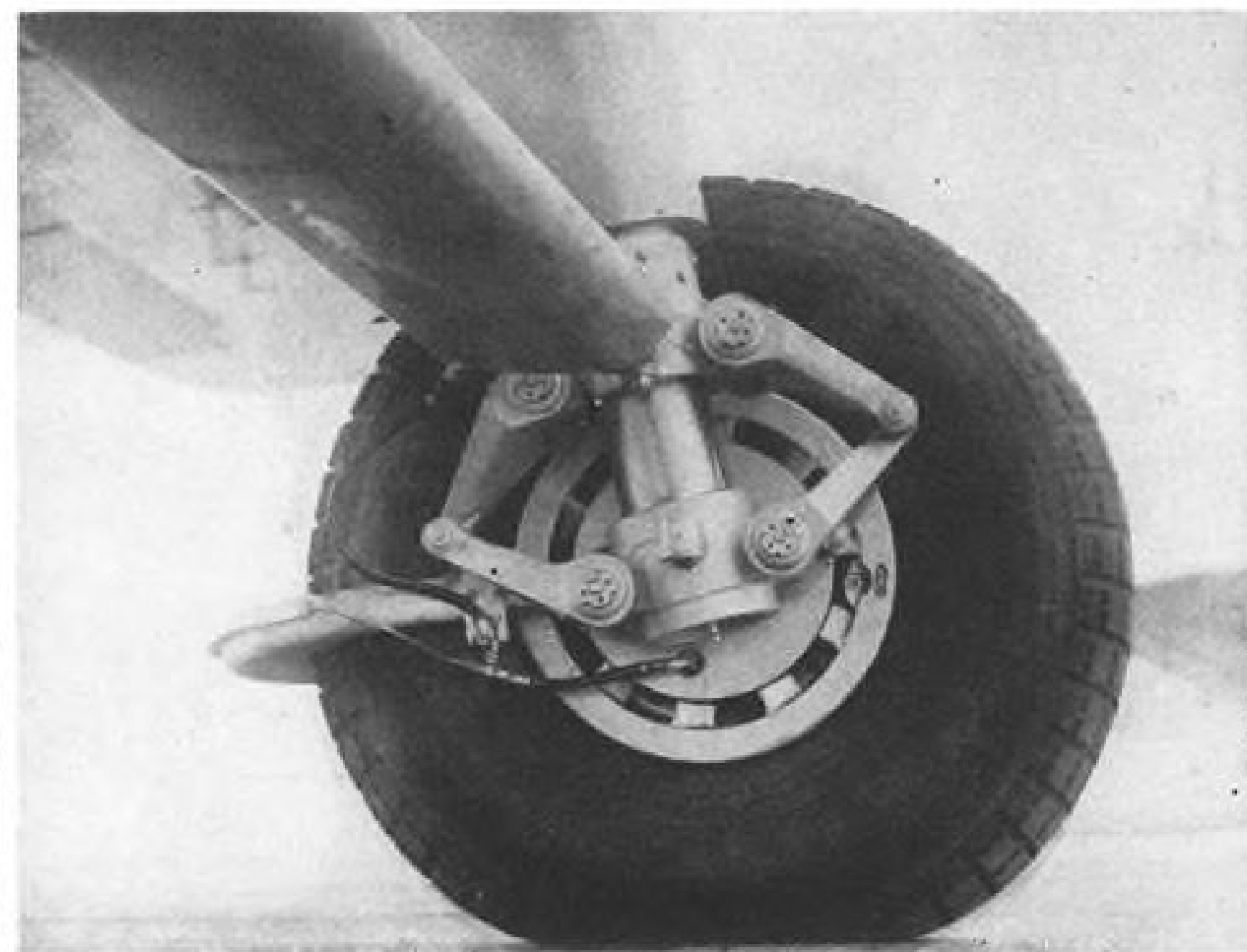
MEDIUM CARGO CARRIER is the Mk. 31 version of Bristol's Type 170 Freighter, with increased power from twin Hercules 734 powerplants. Fixed landing gear has been strengthened to handle increased gross weight.
