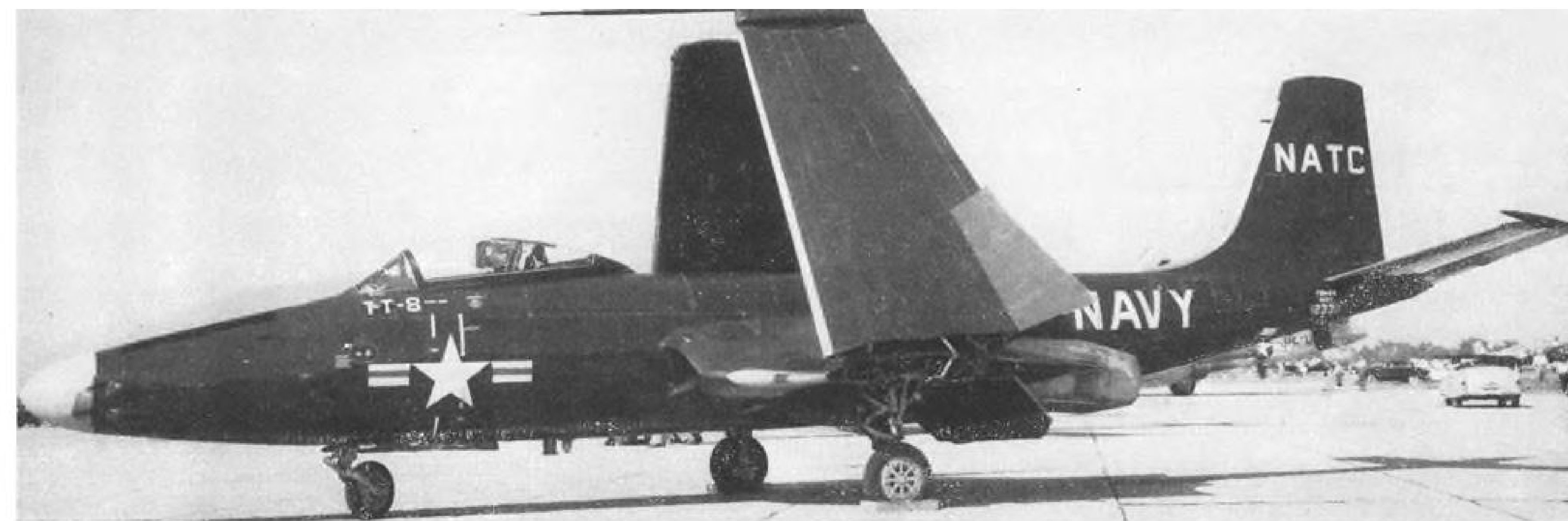
EXTRA BOOST ON BANSHEE—This McDonnell F2H-2N Banshee all-weather fighter has been fitted with short afterburners to provide extra boost on demand. Plane is assigned to test section at Navy's Patuxent Air Station. It does not have its large tip tanks.
