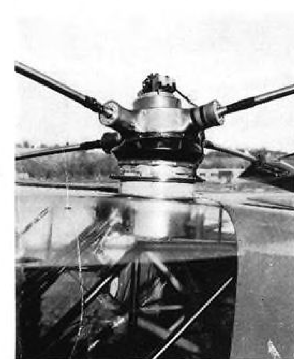
ROTOR HEAD, four hingeless blades.
