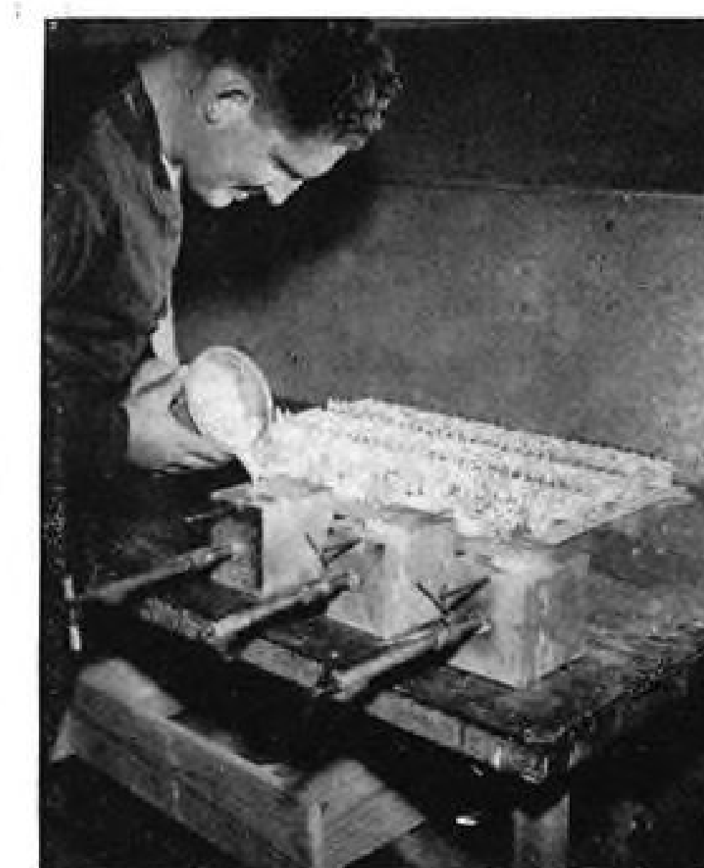
CORES formed in plastic molds are . . . PERFECT when removed. Note slick finish.
