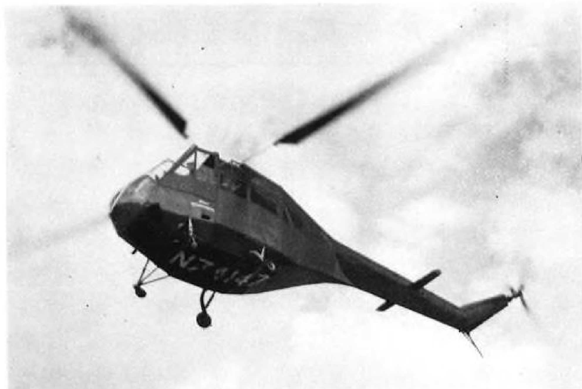
DOMAN LZ-4 was built specifically for use as a military rescue craft. It features . . . ENGINE set below side-by-side cockpit . . .
