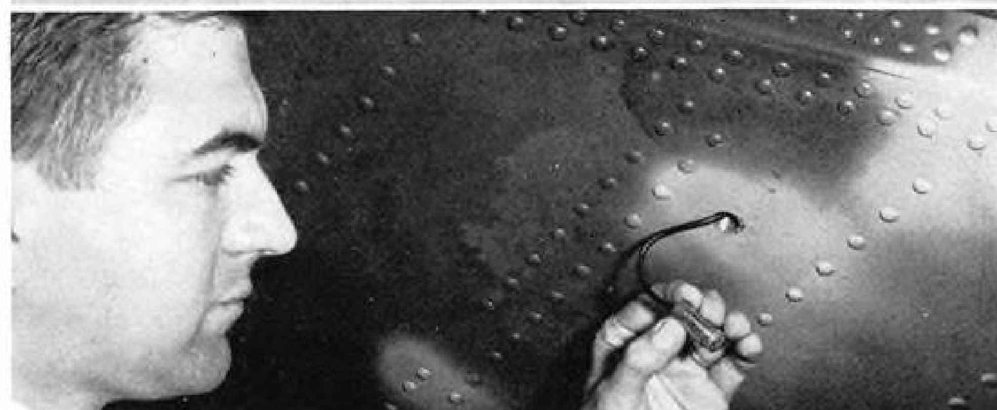
EASY INSTALLATION is assured by using dummy phenolic plug during plane fabrication. To put transducer in, flush dummy is removed and wiring attached to pick-up.
