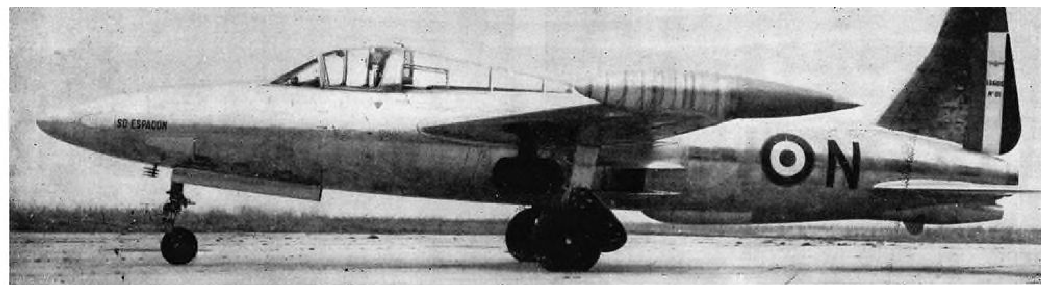
FRENCH JET MODIFIED —SNCASO 6026 Espadon (Swordfish) jet rocket fighter has new air intakes behind landing gear wells, rocket motor installation under the tail, and has tiptanks. Armed with six 20-mm. or four 30-mm. cannon, SO-6026 does about 650 mph.
