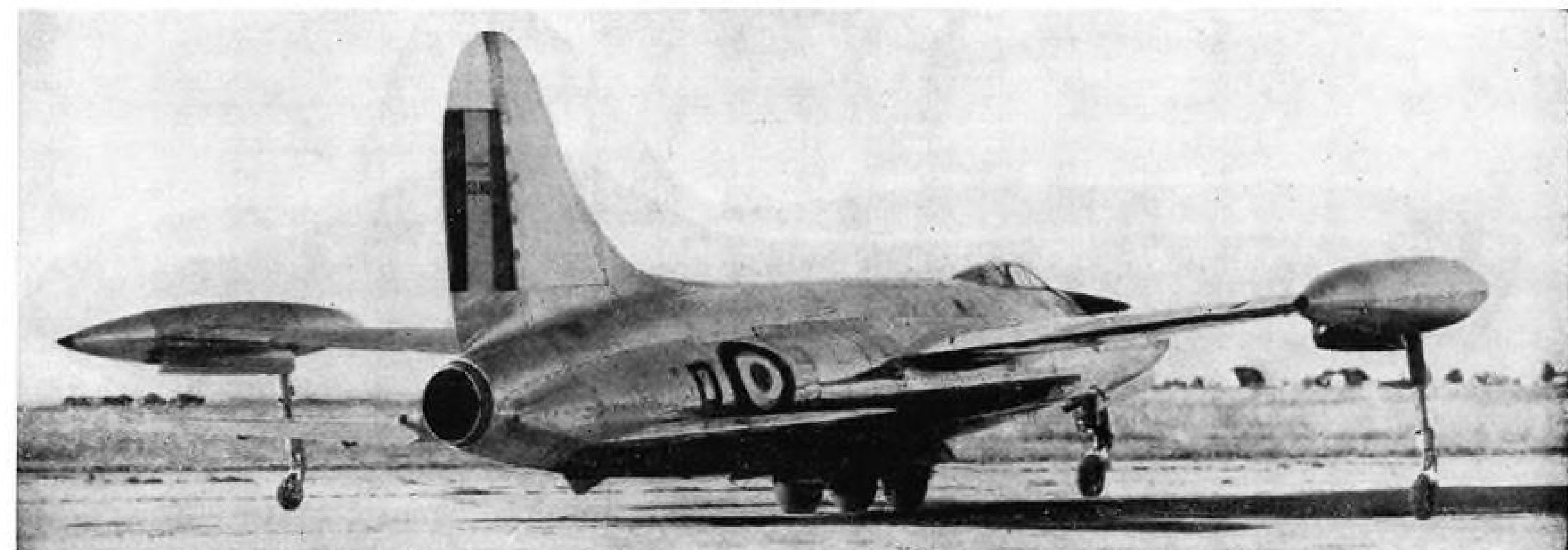
RESUMES TESTS —French SNCASO M2 research plane (above and below) is flying again with new tiptanks housing outrigger landing gear, modified servomechanisms. It is now powered by a 3,500-lb.-thrust Rolls-Royce Derwent, but installation of rockets is being considered. Speed is over 600 mph.
