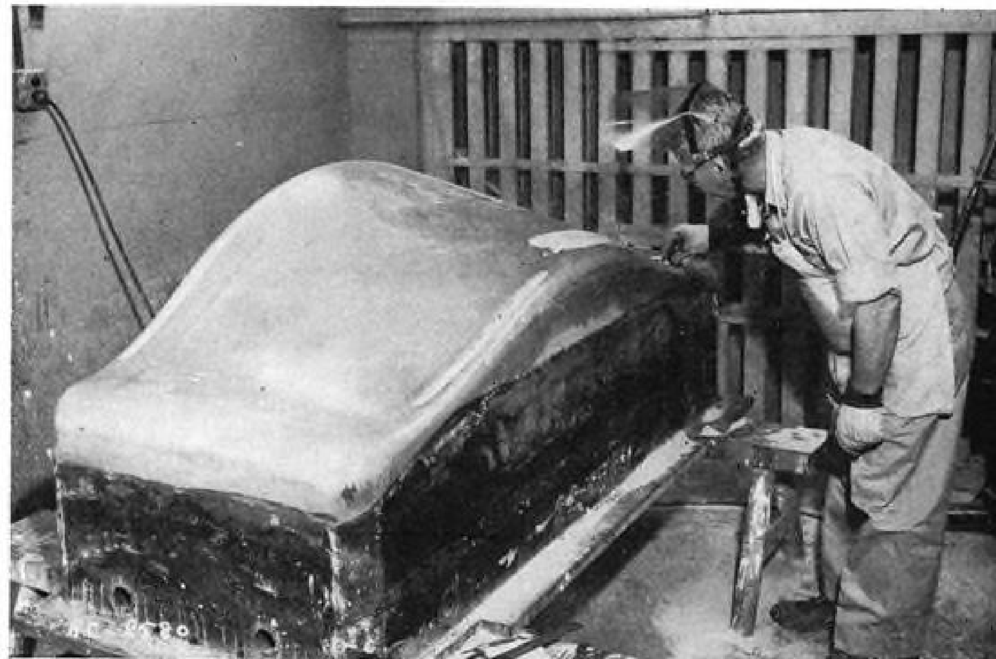
LOCKHEED technician installs gripper beads on plastic double-action die, while . . . WORKERS mount plastic drill guide.
