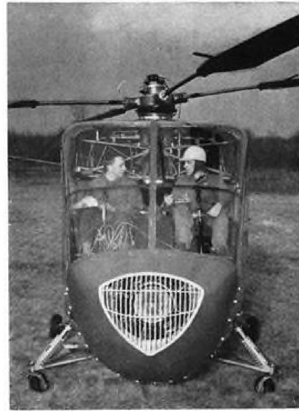
DOMAN LZ-4 was built specifically for use as a military rescue craft. It features . . . ENGINE set below side-by-side cockpit . . .
