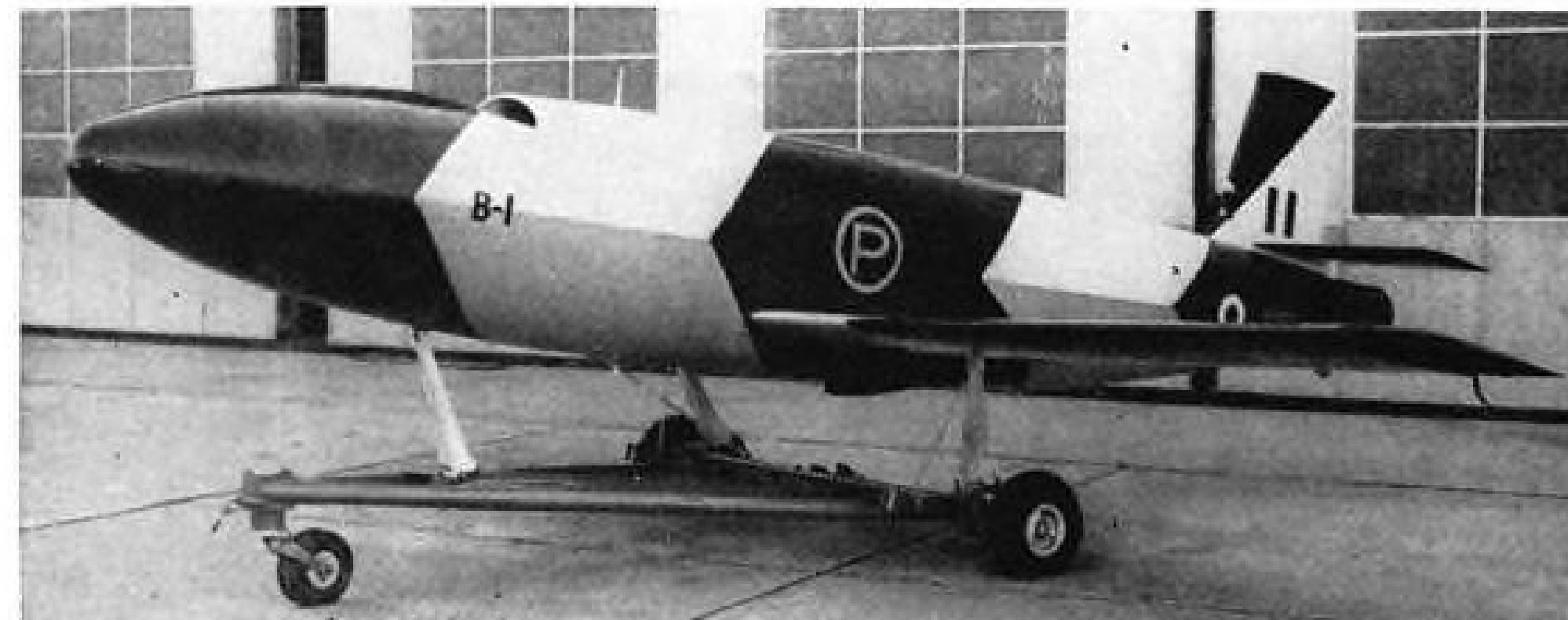
PILOTLESS TARGET DRONE takes off on jettisonable trolley, lands on central skid.
