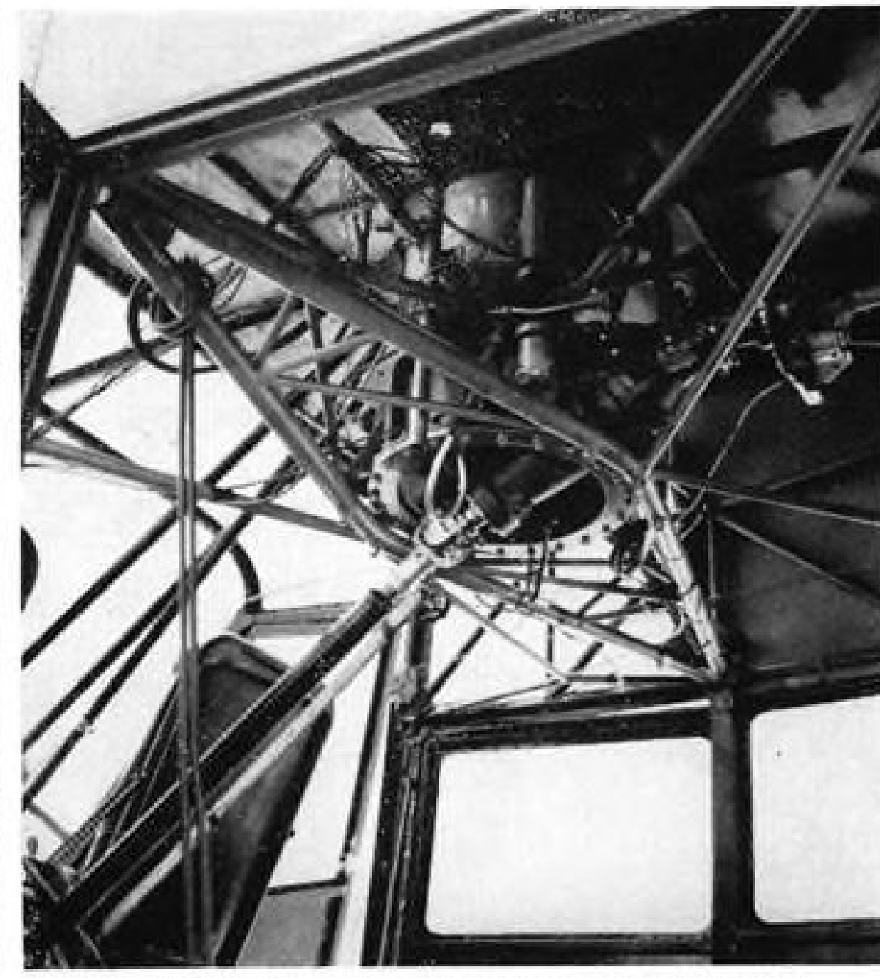
BIG CABIN, demonstrated by Glidden S. Doman. Between seats . . . SHAFT is linked to rotor. Projecting through roof is . . .
