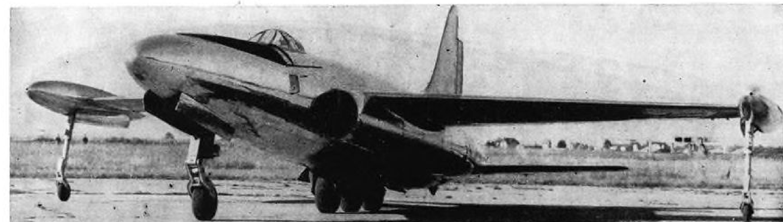
RESUMES TESTS —French SNCASO M2 research plane (above and below) is flying again with new tiptanks housing outrigger landing gear, modified servomechanisms. It is now powered by a 3,500-lb.-thrust Rolls-Royce Derwent, but installation of rockets is being considered. Speed is over 600 mph.
