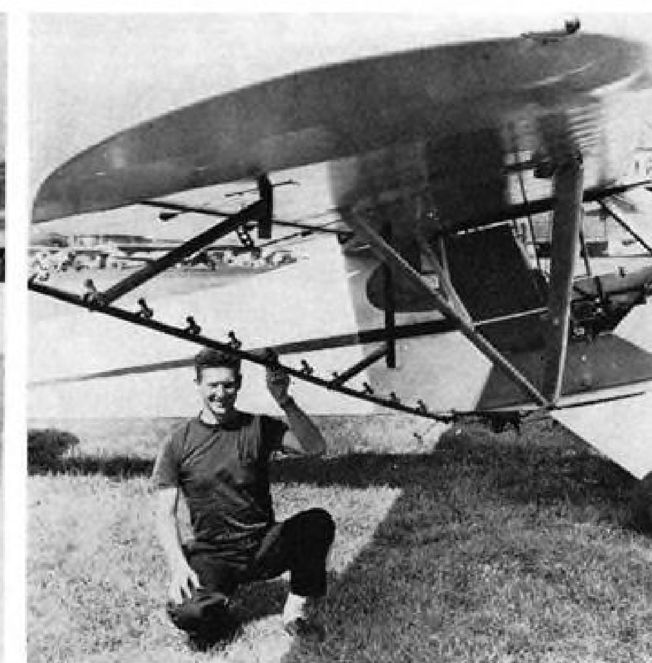
PIPER PA-18-A's dust dispersal unit provides wide, penetrating swath; spray booms (right) are hinged for safety.
