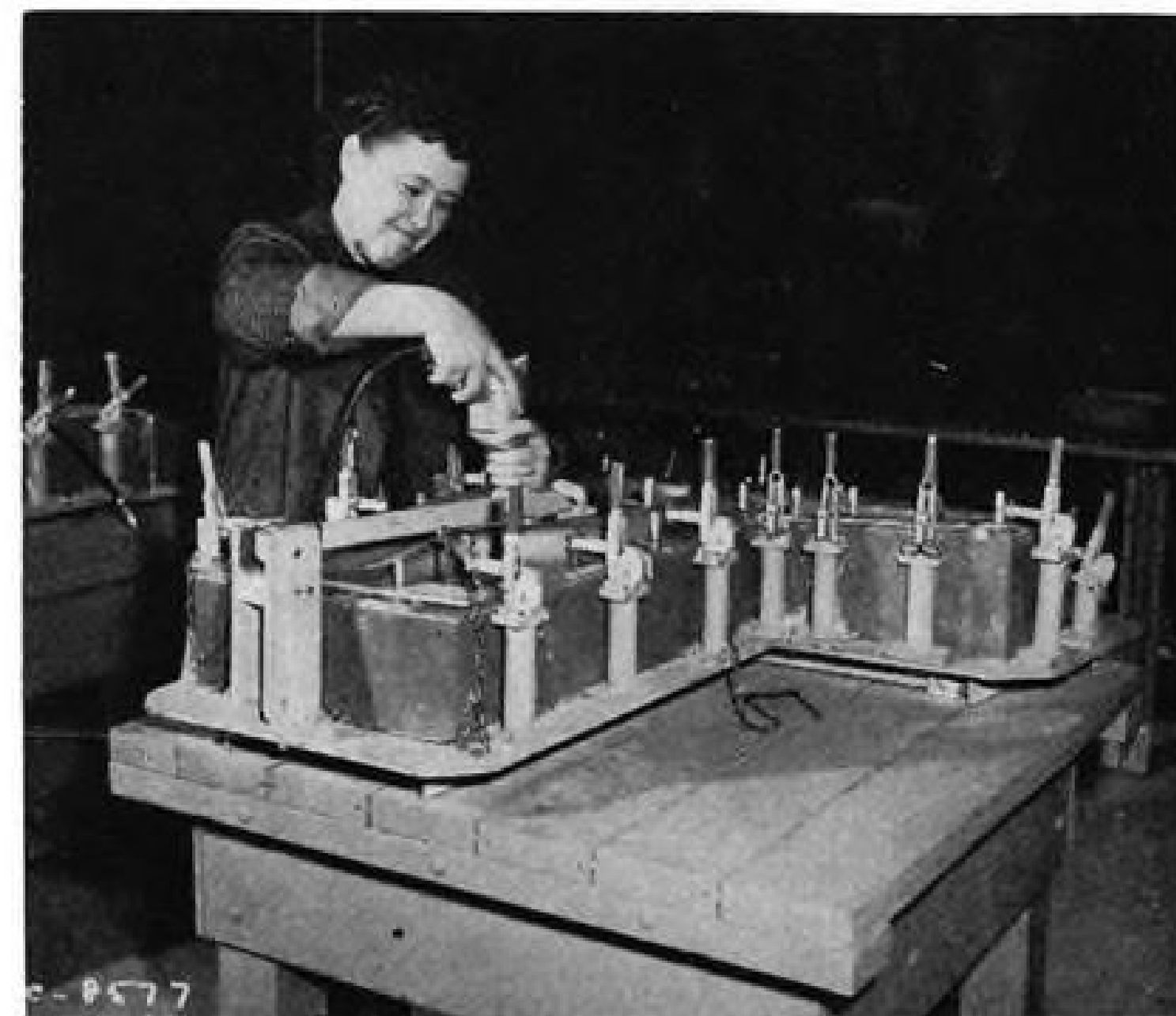
DRILLER uses plastic contour jig on metal part. Typical . . . JIGS are made of Rezolin plastic (top) and Fiberglas (bottom).
