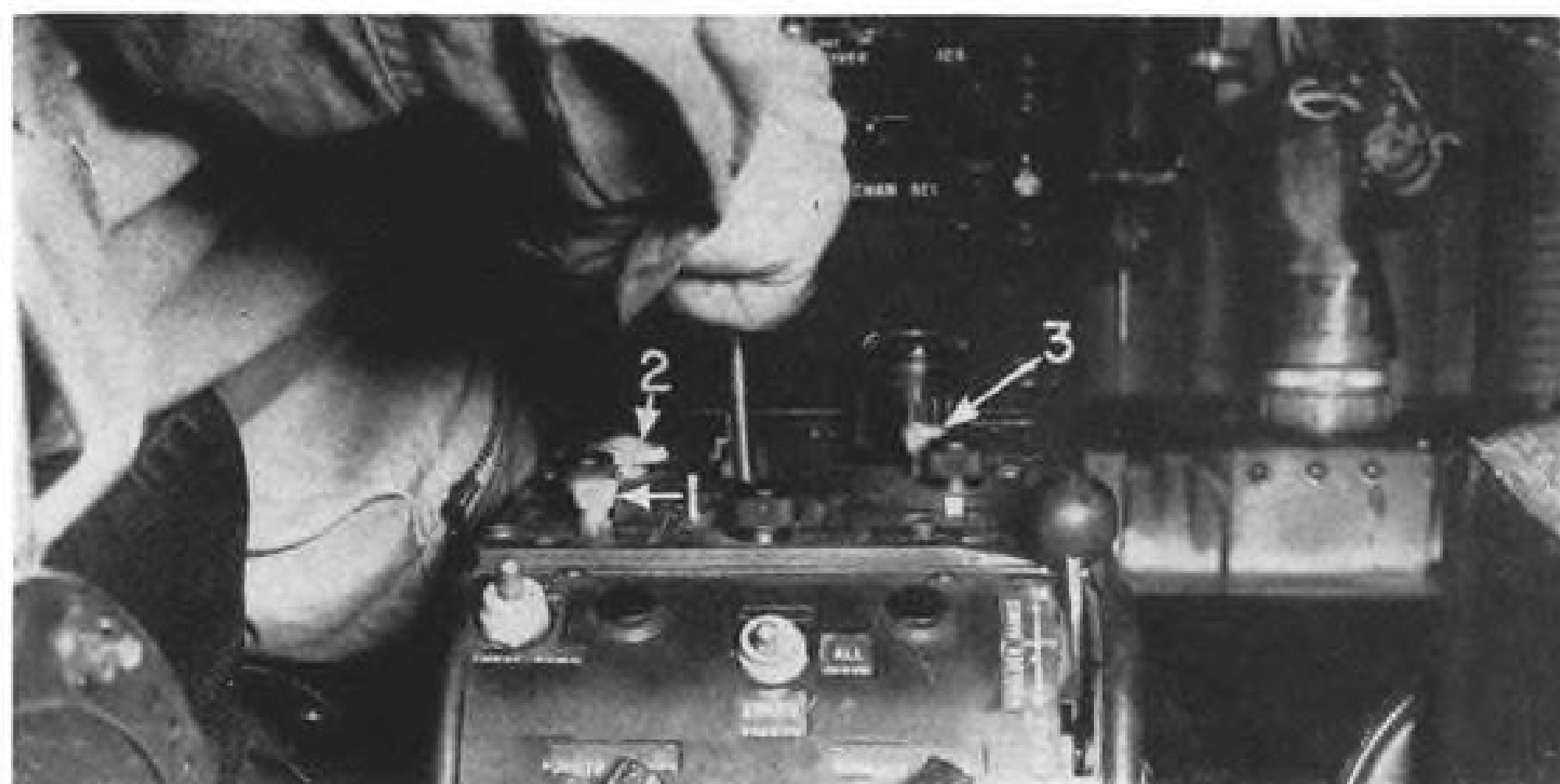
AUTOPILOT CONTROL by stick is preferable to knobs, BuAer feels, but knobs (1, 2 and 3 above) are still used for engagement, trim changes and altitude.
