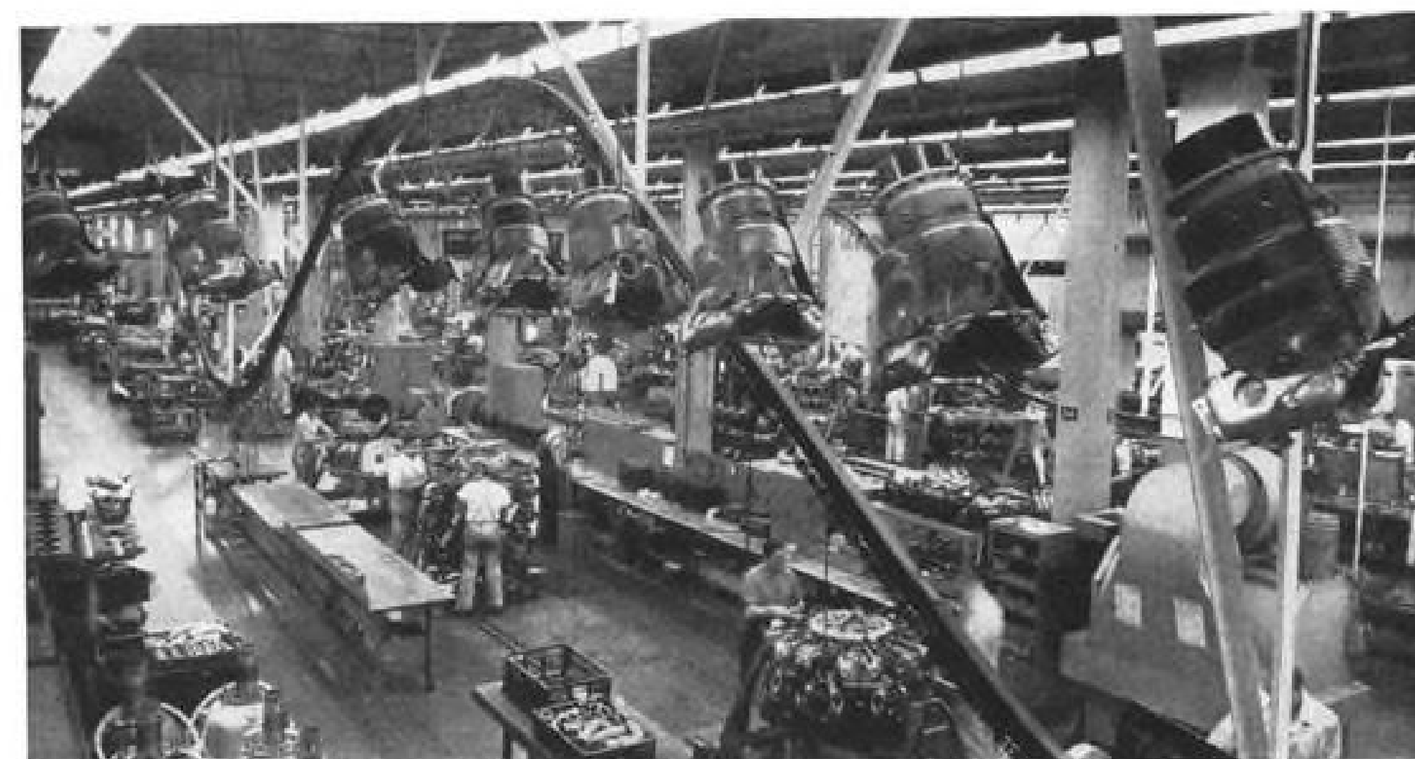
OVERHEAD conveyor system for cylinders in its modern engine overhaul shop.
