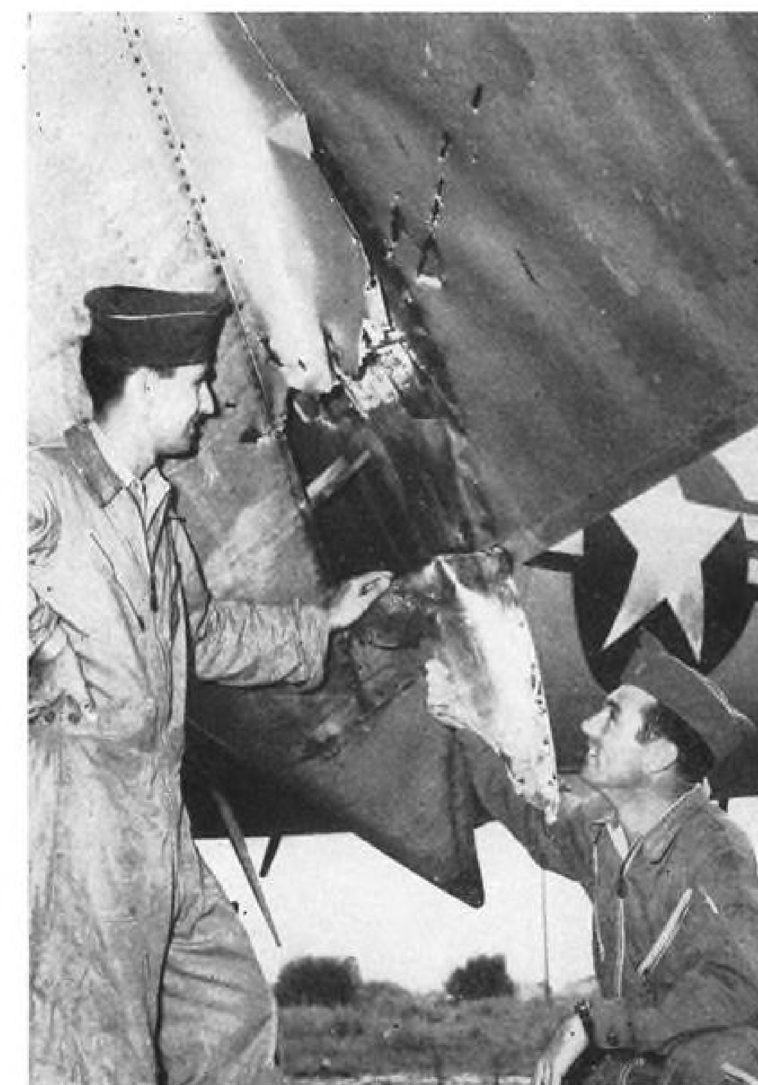
FLAP of B-29 (left) was badly damaged and fuselage section of an F-86 (right) ripped away by MiG fire. Both returned, as did . . .
