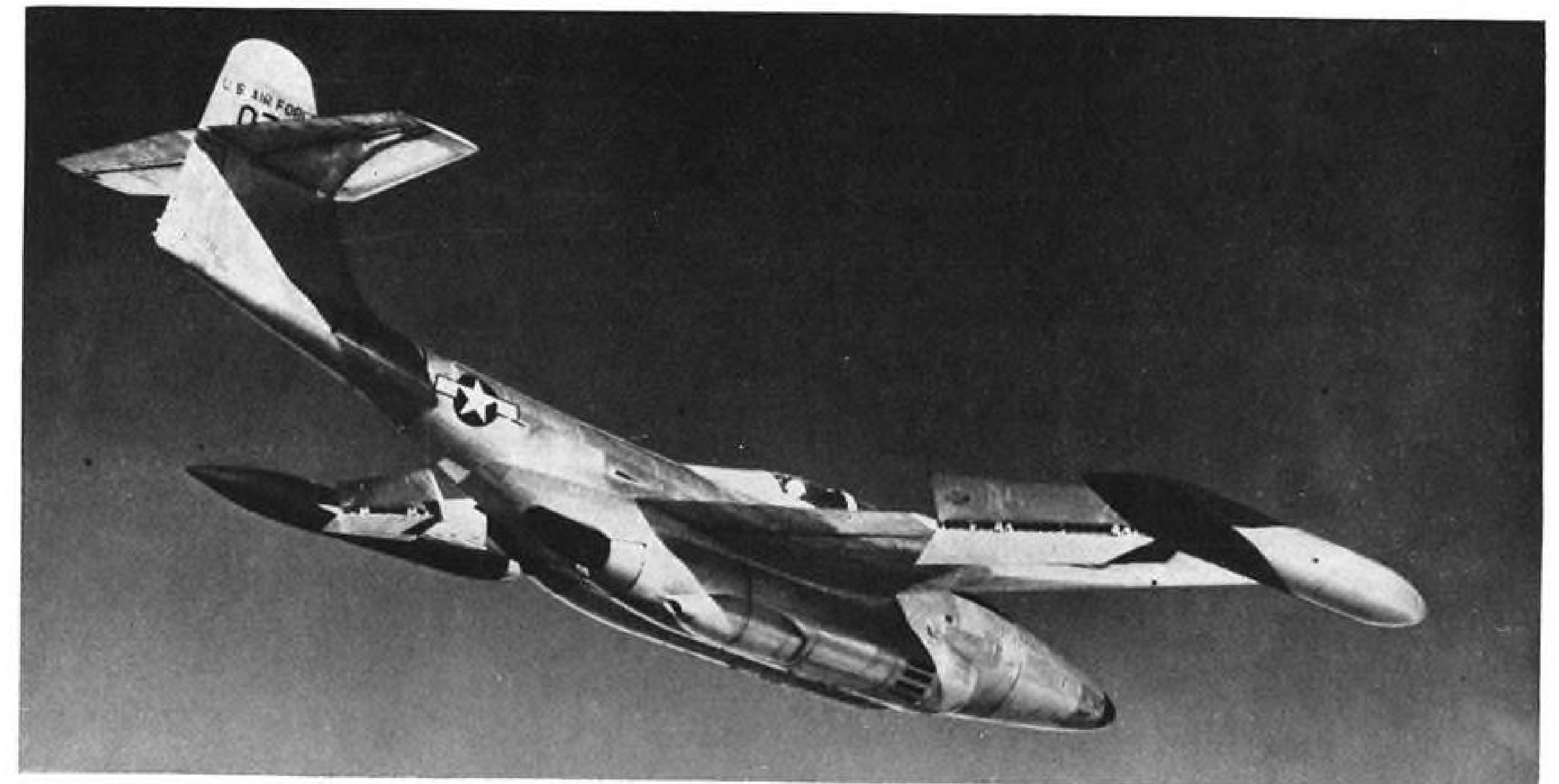
SCORPION'S AIR BRAKES OPEN —Northrop F-89D (above) demonstrates action of its clam-shell "decelerons" which serve dual function as ailerons and speed brakes. Their considerable area permits pilot to vary speed rapidly when engaging target, allows steep descents without exceeding Mach redline.
