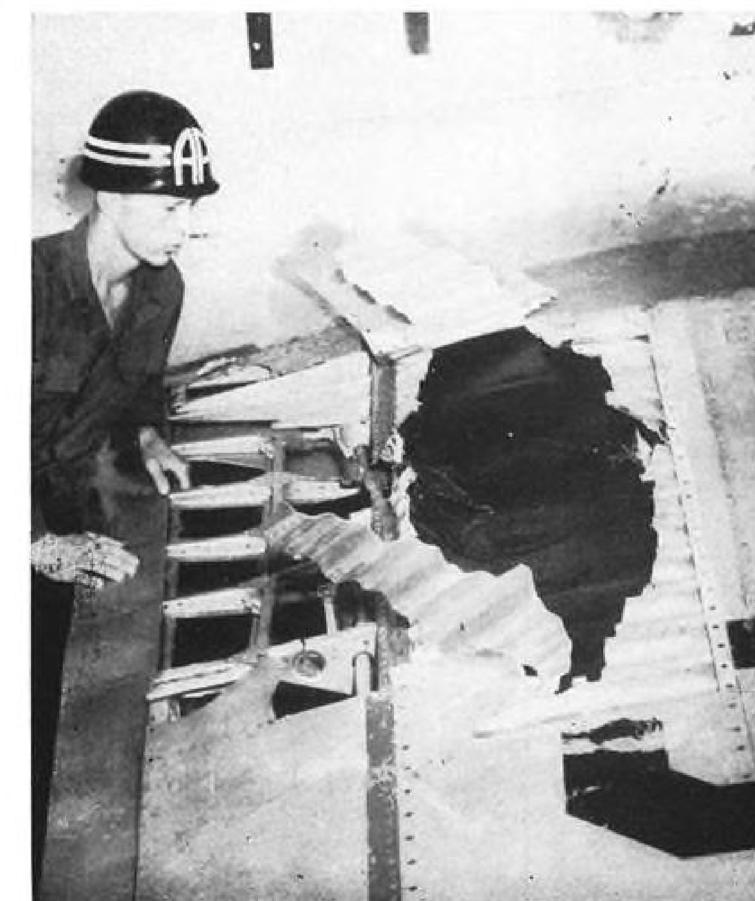
RF-80 (left), with gaping hole in wing, and another battlescarred Sabre (right). Most damage is done by MiG 37mm cannon.
