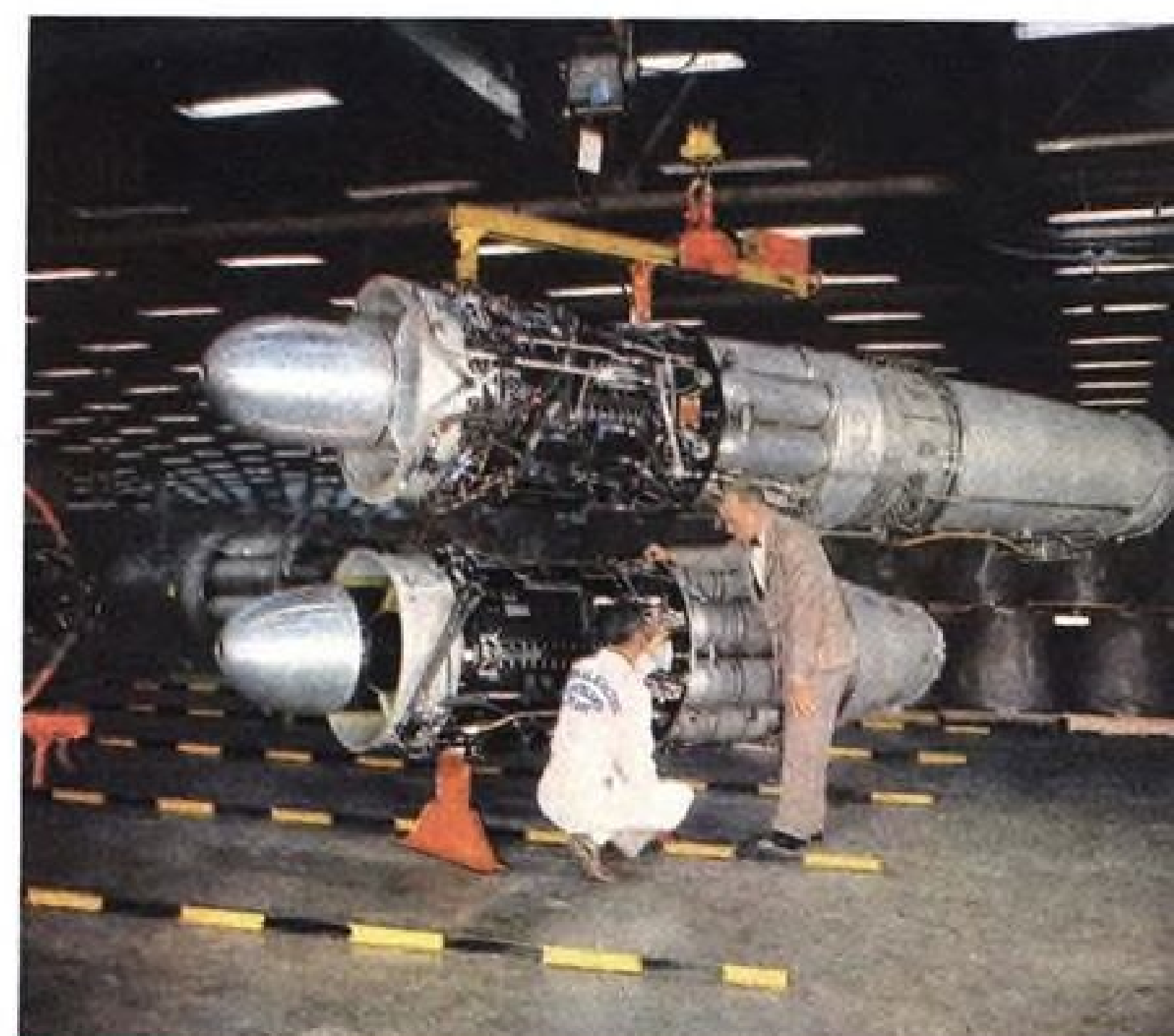
THRUST or "push" of G-E jet is increased by afterburner, shown on the top engine. Pilot can climb faster, gets greater bursts of speed in combat.
