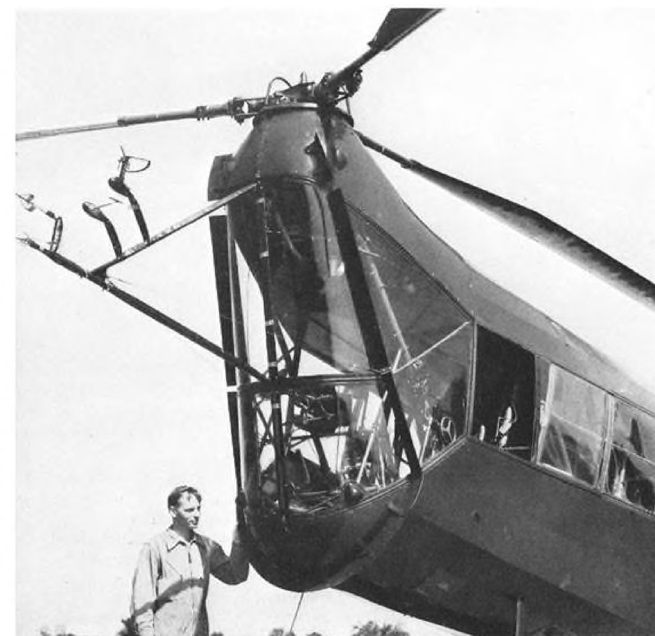
HORSECOLLAR is metal spoiler strip to create turbulent flow along HRP fuselage for increased directional stability. Temporary boom on nose carries devices to measure airspeed, angle of attack and sideslip angle. Copter is being flown by NACA pilots.
