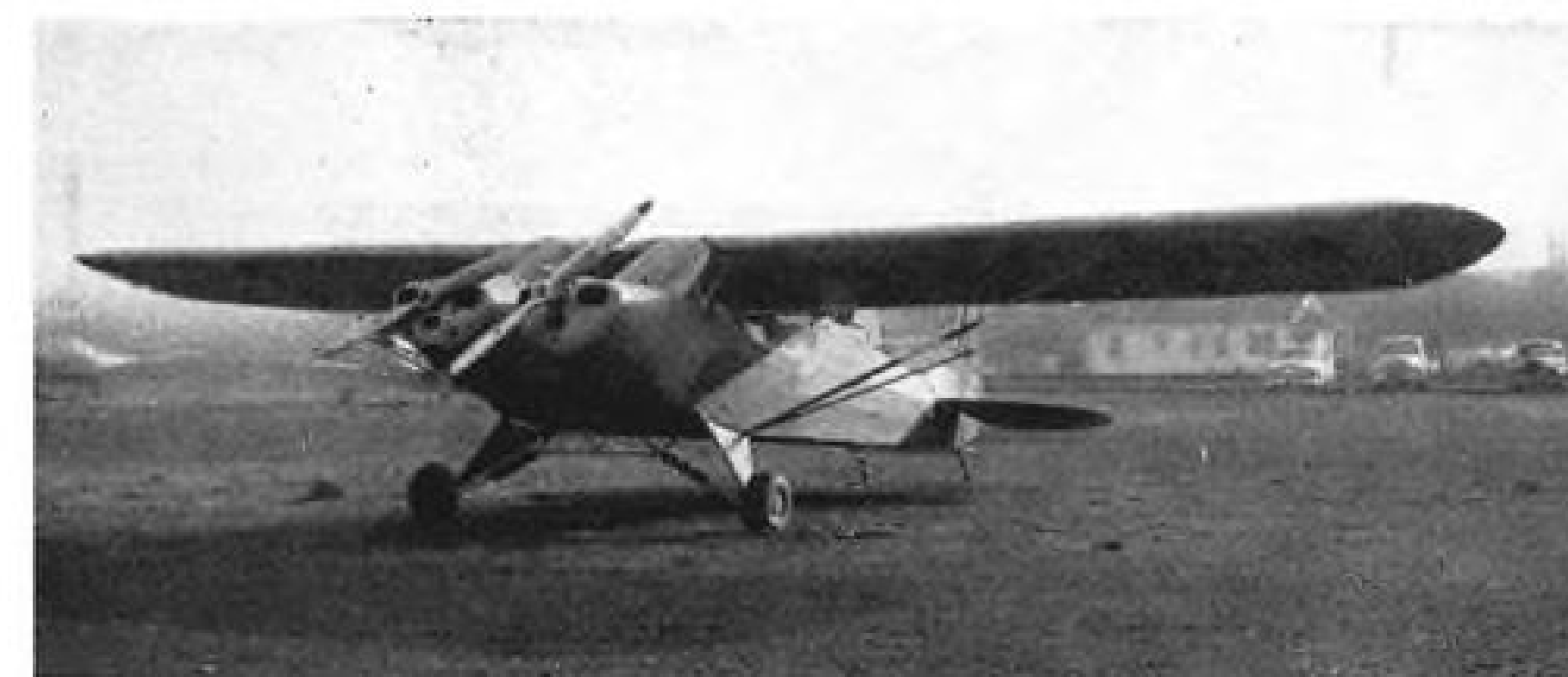
SIAMESE PIPER —This peculiar creation (above) is the handiwork of Harold Wagner, Portland, Ore. It's two Piper Cubs, with port prop shaft reworked for clearance with starboard prop. Wing span is 38½ ft.; top speed is 120 mph. Plane has racked up 30 hr. flight time.
