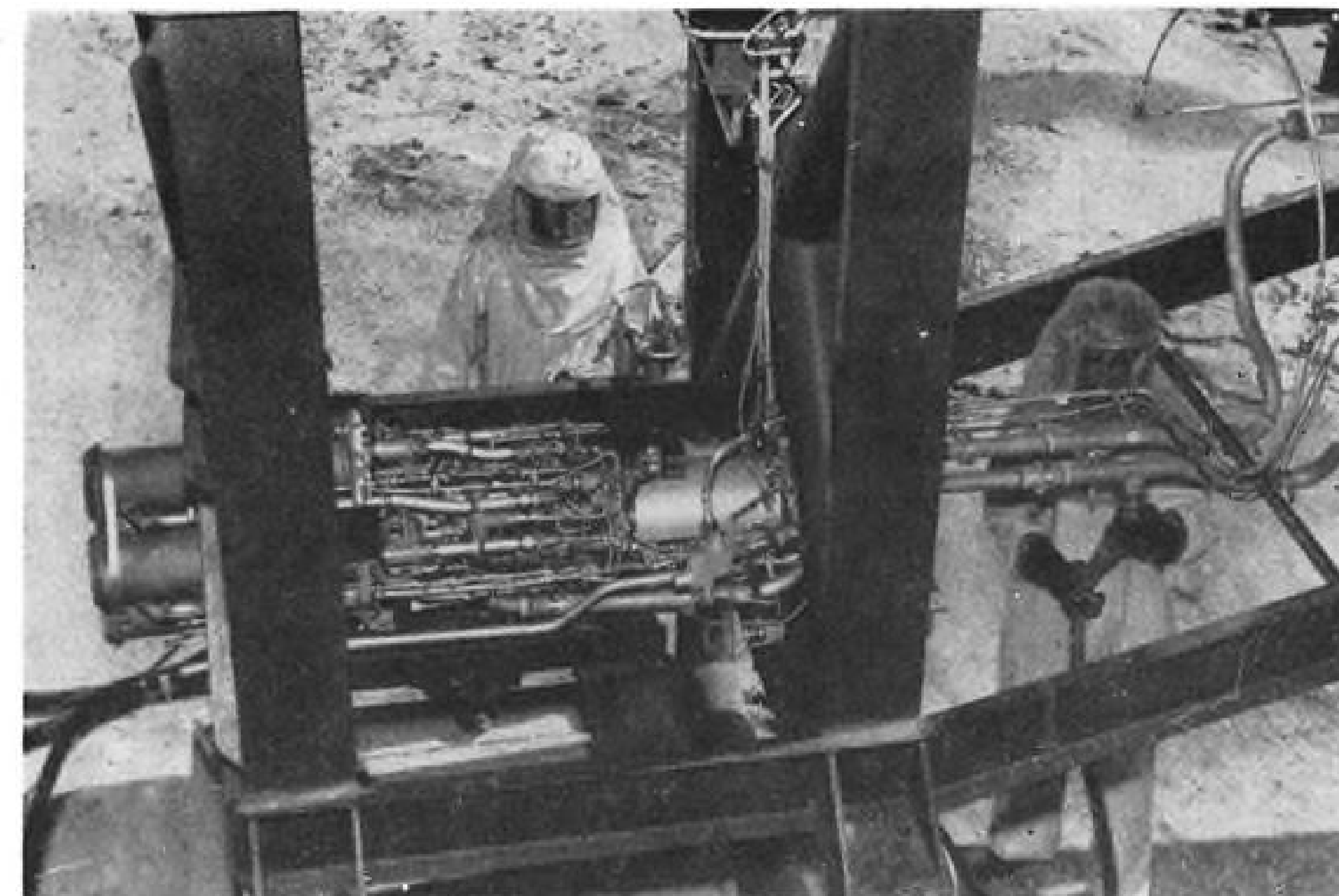
REACTION MOTOR rocket engine for Republic's XF-91 is set up here just as in the aircraft. Four-cylinder engine develops 6,000-lb. thrust, powered Bell X-1 and Douglas D-558-II on their record-breaking speed flights.
