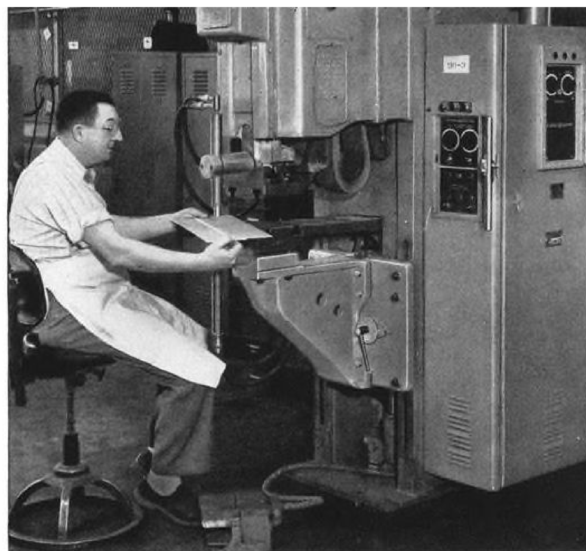
H. C. Wolfe, of the General Electric Electronics Laboratory Welding Section, says, "Tests in our Laboratory and in other General Electric Welding Laboratories showed that single-phase a-c welding using Slope Control was as good as three-phase welding on aluminum. So, for Class A spot welding of aluminum, the use of our a-c machine with Slope Control certified to Military Specification MIL-W-6860 for .125-.125" 52S \frac{1}{4} H aluminum has resulted in a considerable saving of money and time."
