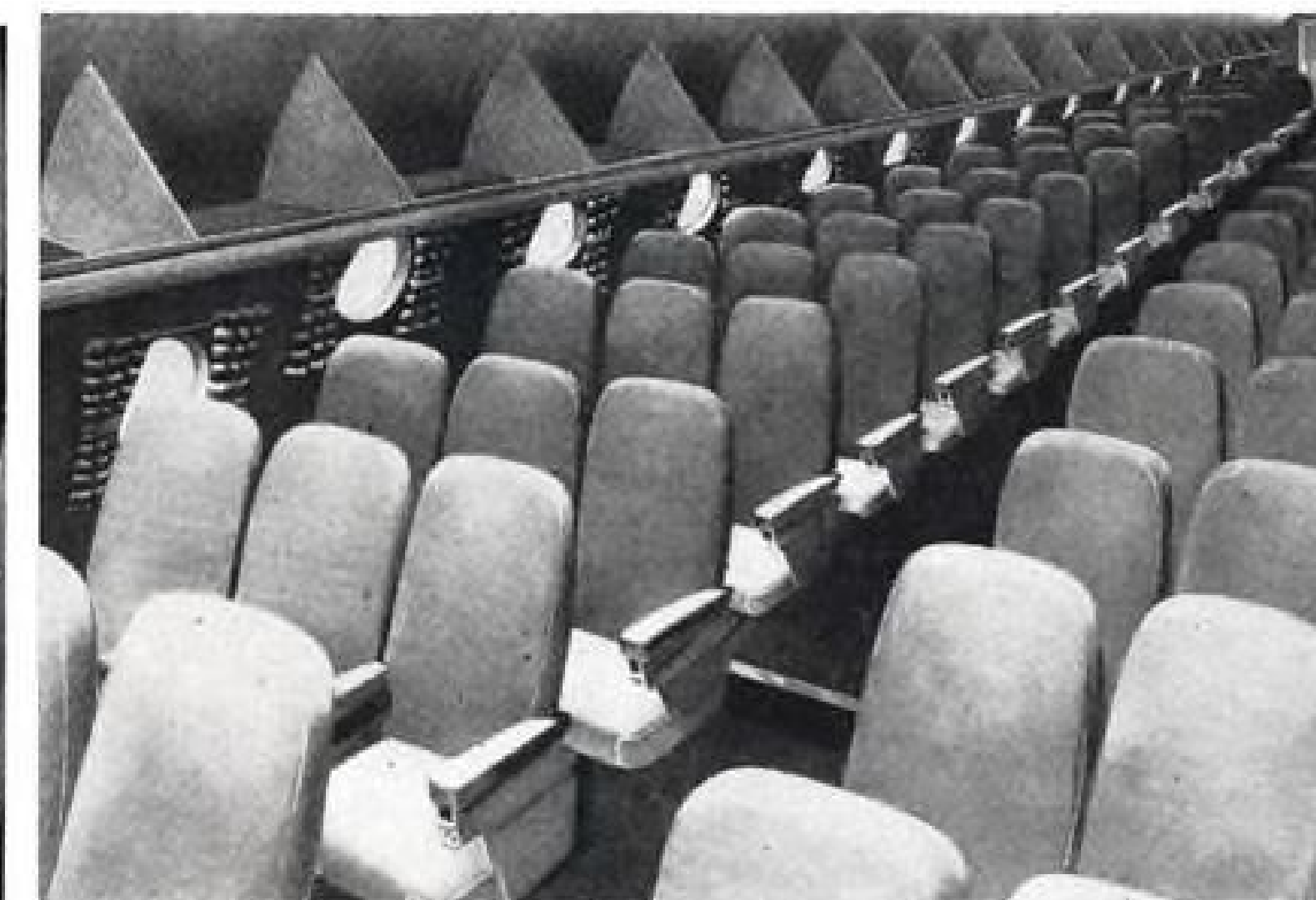
LOCKHEED is converting six A-26s (left) to transports for oil firms and five BOAC Connie interiors to the 3-2 seating arrangement (right).
