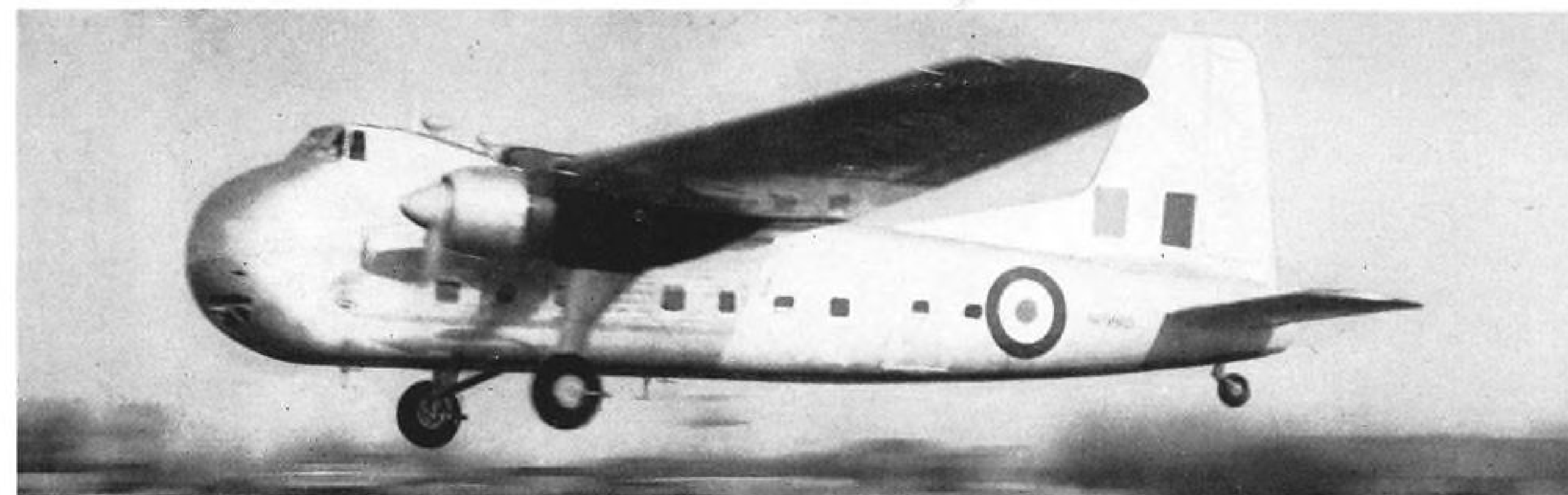
FERTILIZING FREIGHTER —Third Bristol Freighter ordered by the Royal New Zealand Air Force takes off from Filton, England, on its delivery flight. Plane is fitted with three 2-ton fertilizer hoppers for aerial top-dressing of hill pastures.
