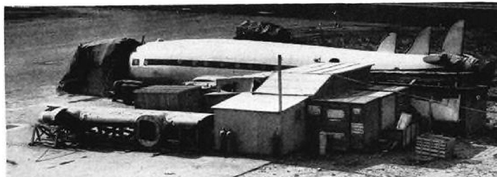
OUTDOOR station was set up to repair wrecked Connie as space saver at Idlewild.
