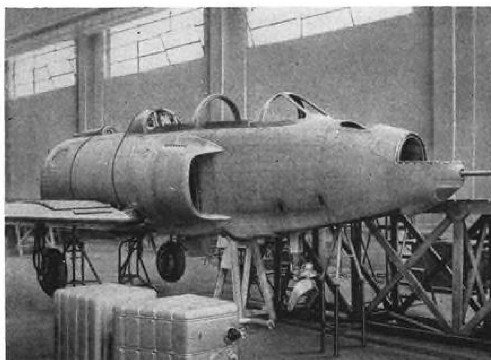
FORWARD FUSELAGE is reminiscent of Lockheed T-33. Interesting points: boundary layer removal scoops, light cockpit framing.
